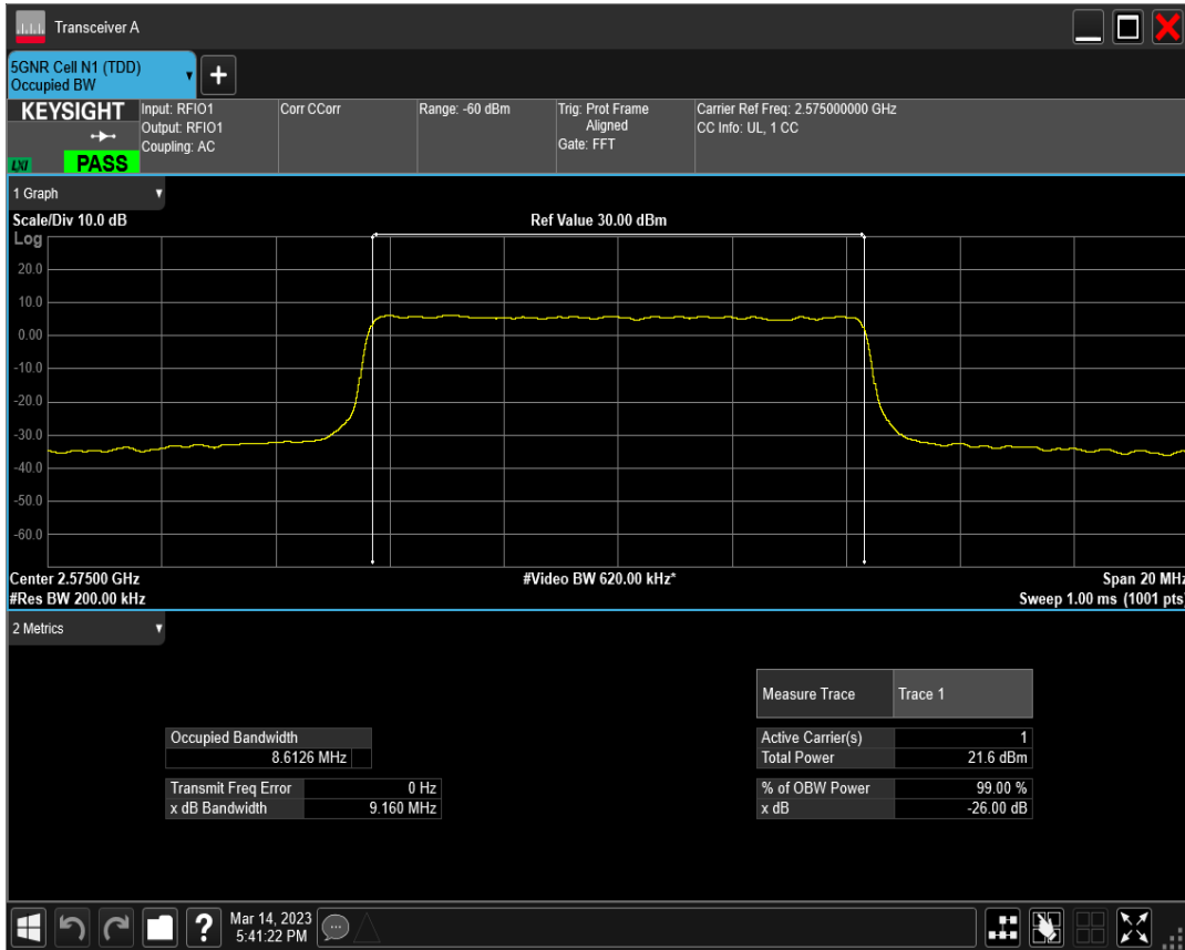
n38 SCS=30kHz DFT_QAM64 BW=10MHz Channel=515000 RB=24@0
