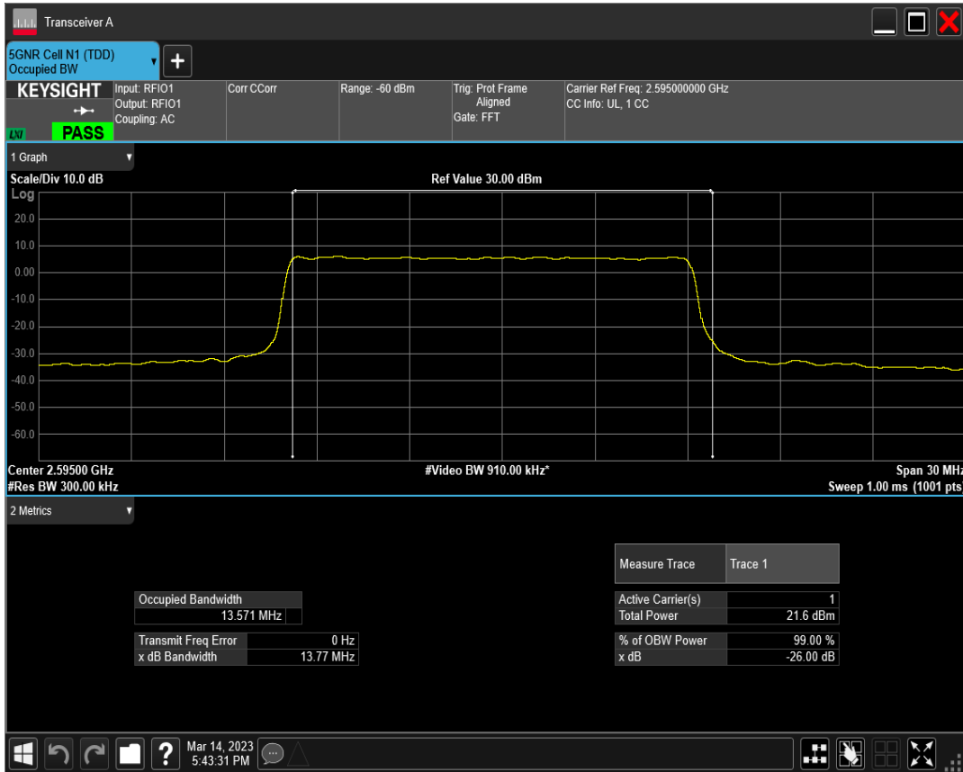
n38 SCS=30kHz DFT_QAM64 BW=15MHz Channel=519000 RB=36@0
