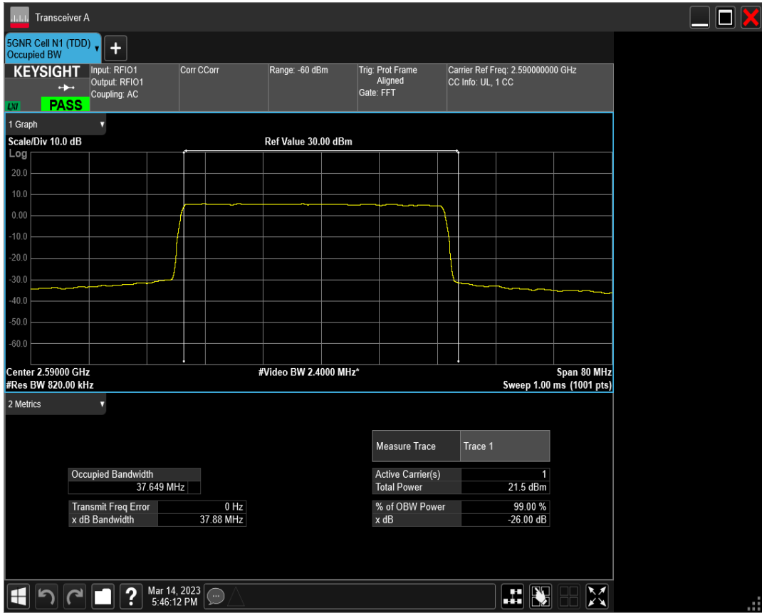
n38 SCS=30kHz DFT_QAM64 BW=40MHz Channel=518000 RB=100@0
