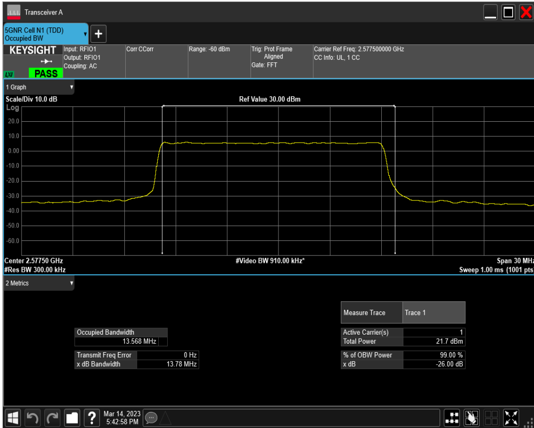
n38 SCS=30kHz DFT_QAM64 BW=15MHz Channel=515500 RB=36@0
