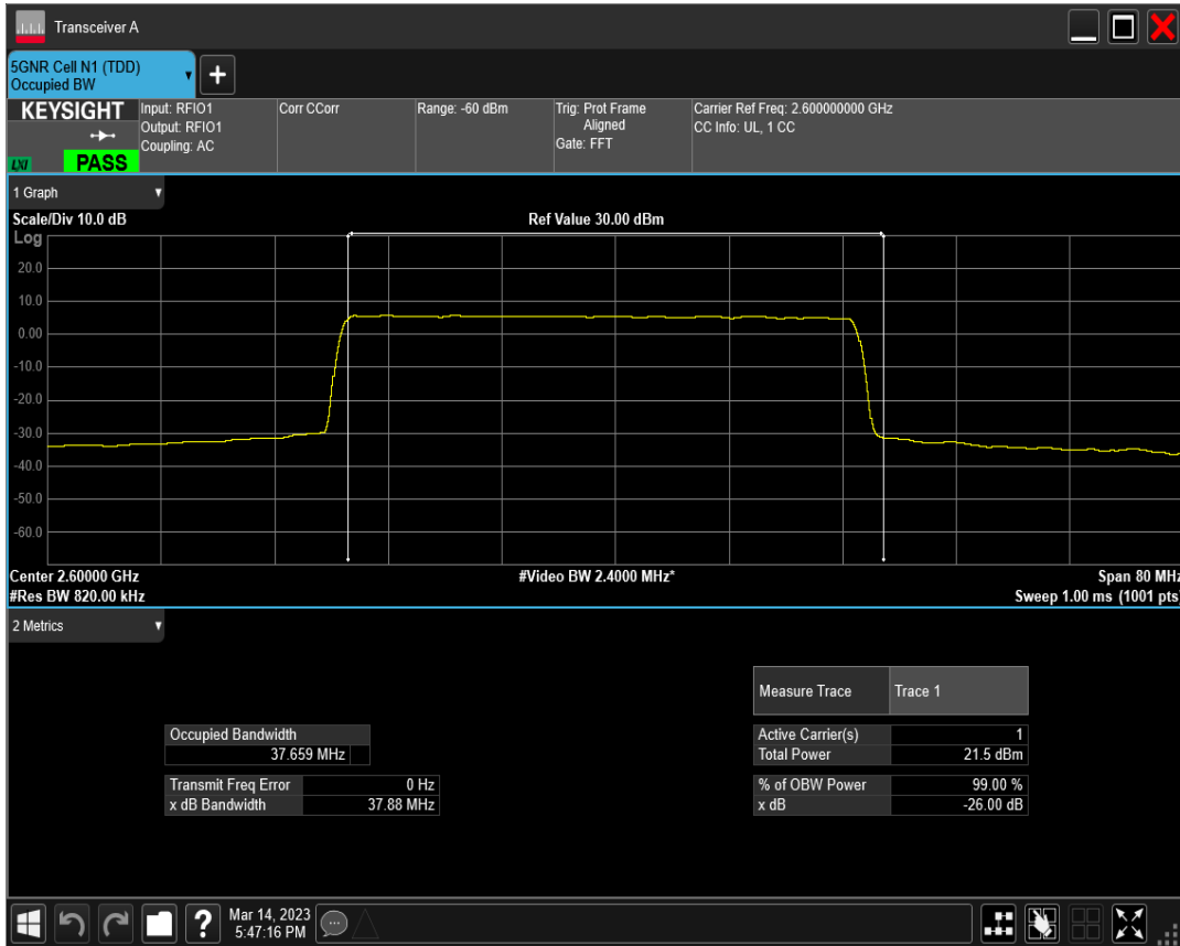
n38 SCS=30kHz DFT_QAM64 BW=40MHz Channel=520000 RB=100@0
