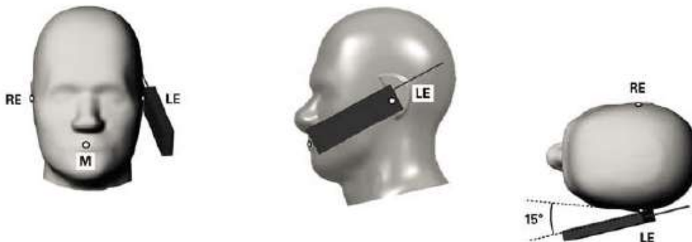
Fig.11.4 Illustration for Tilted Position
