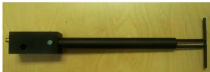
Figure 1 – MVG COMOSAR Validation Dipole
