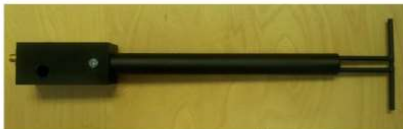
Figure 1 – MVG COMOSAR Validation Dipole
