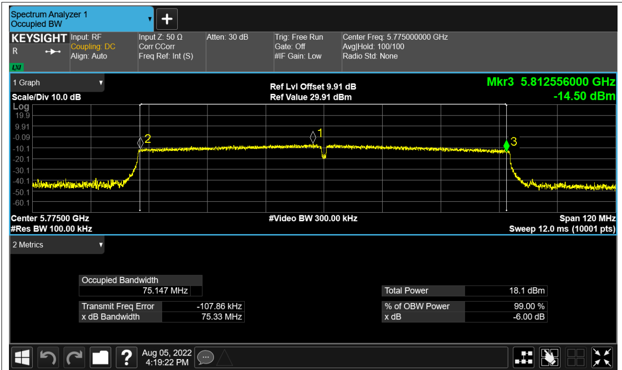
-6dB Bandwidth NVNT n20 5745MHz Ant1
