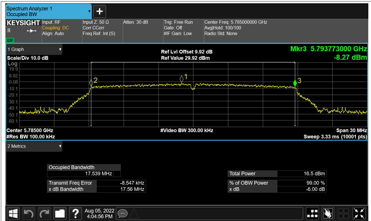
-6dB Bandwidth NVNT ac20 5825MHz Ant1
