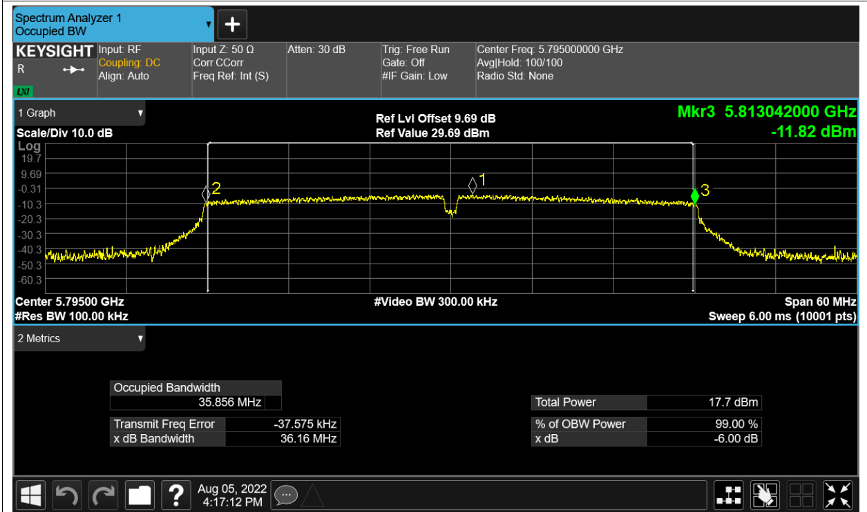
-6dB Bandwidth NVNT ac80 5775MHz Ant1
