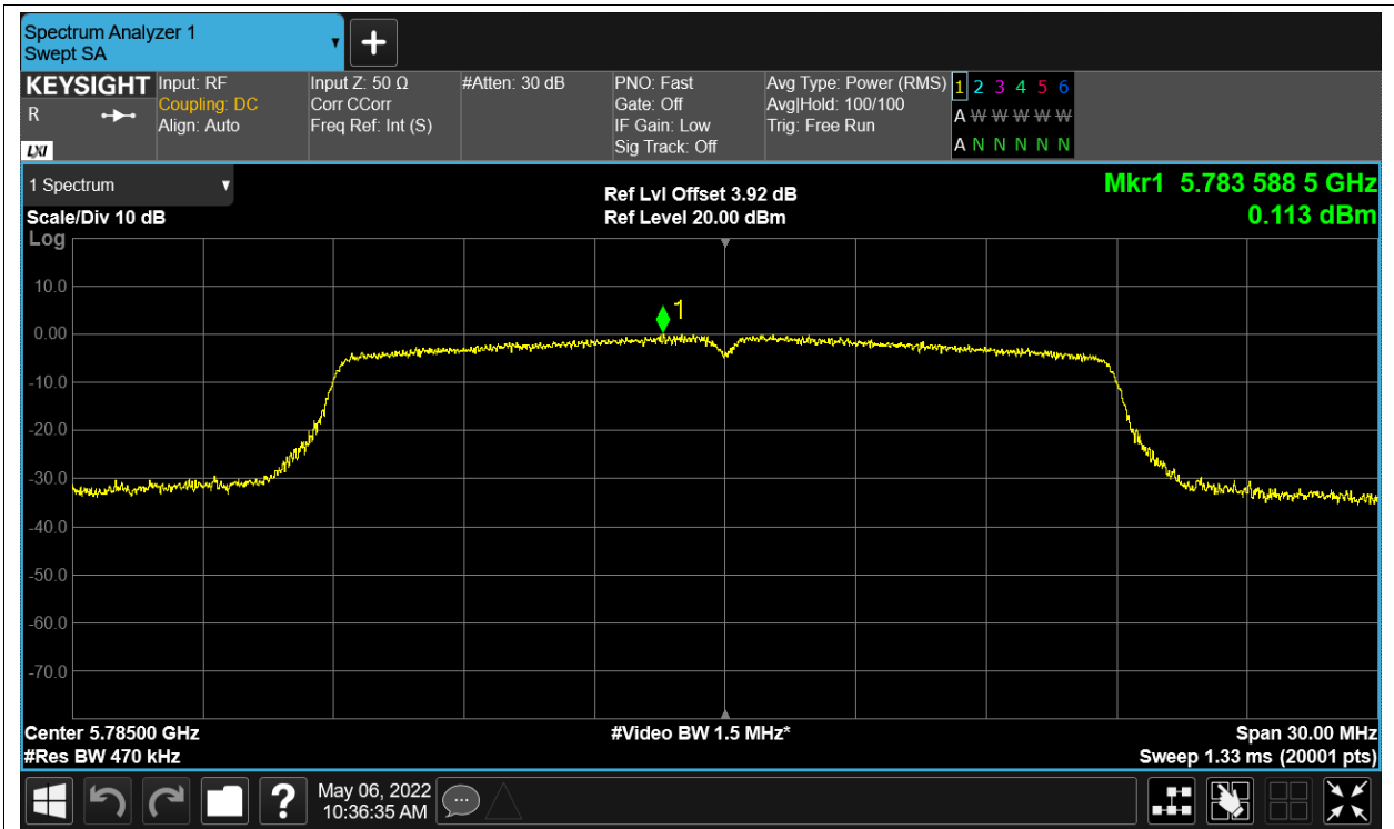
PSD NVNT ac20 5825MHz Ant1
