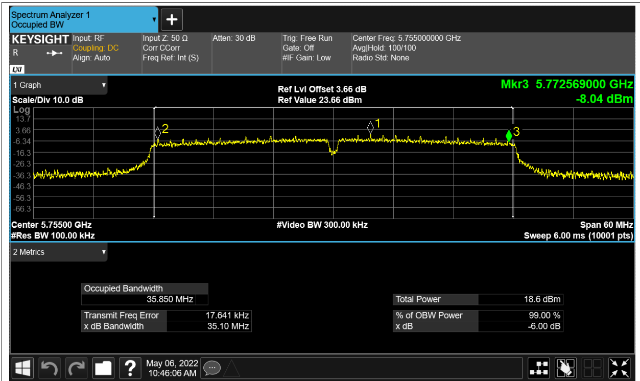
-6dB Bandwidth NVNT ac40 5795MHz Ant1
