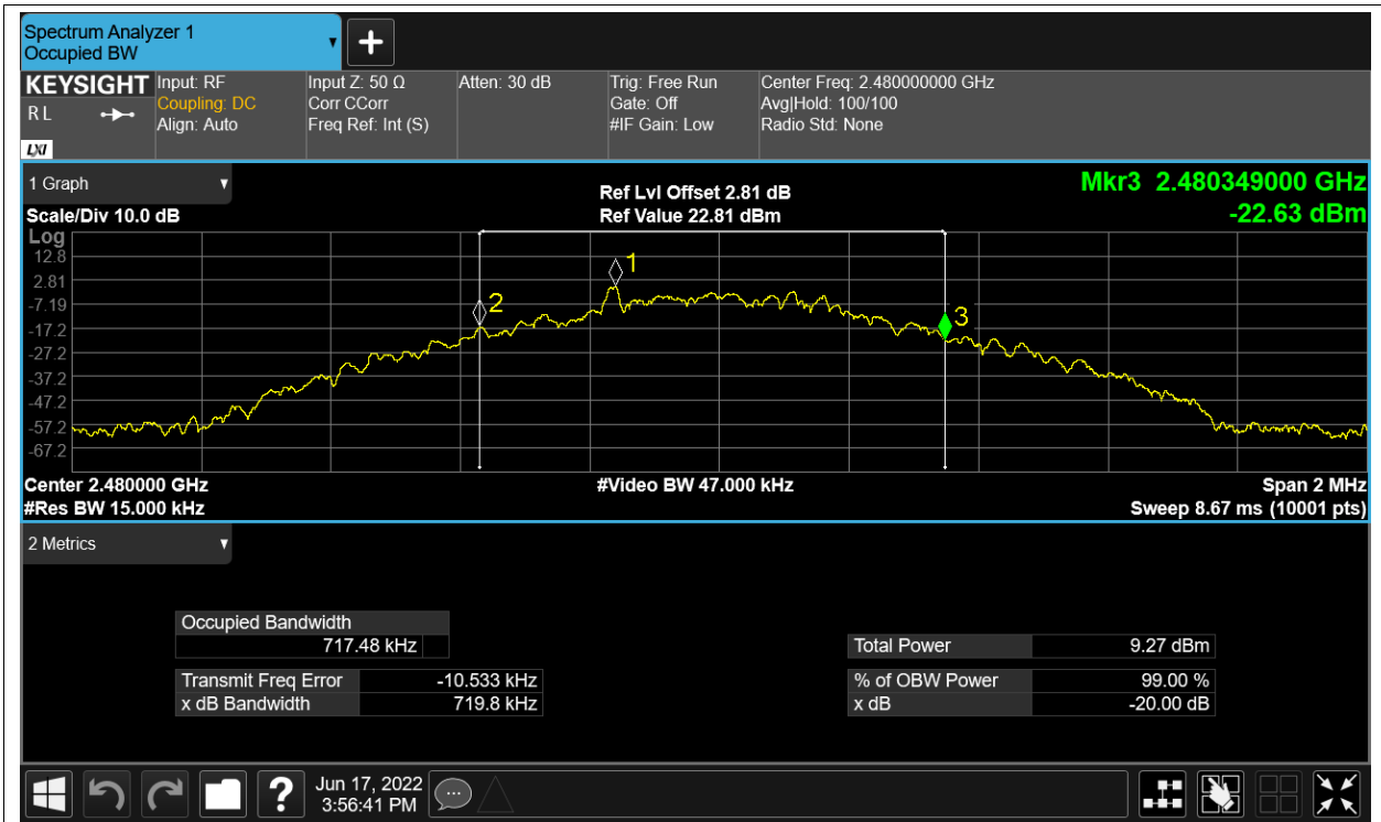
-20dB Bandwidth NVNT 2-DH1 2402MHz Ant2
