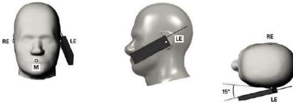
Fig.11.4 Illustration for Tilted Position
