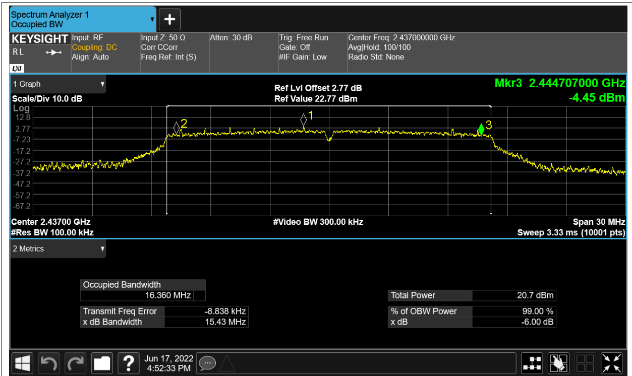
-6dB Bandwidth NVNT g 2462MHz Ant2
