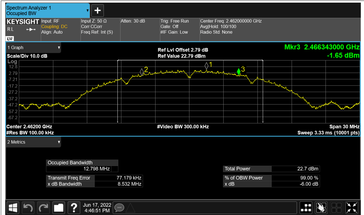
-6dB Bandwidth NVNT g 2412MHz Ant2
