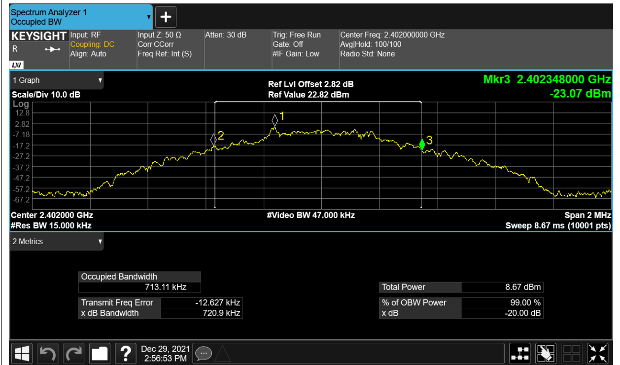
-20dB Bandwidth NVNT 1-DH1 2441MHz Ant1
