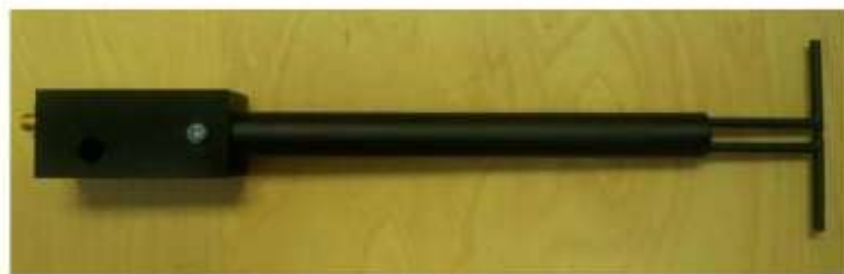
Figure 1 – MVG COMOSAR Validation Dipole
