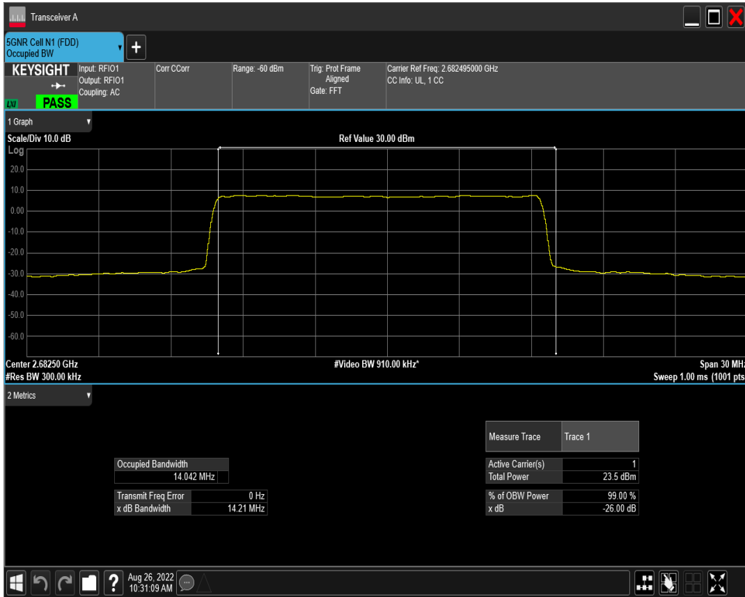
n41 SCS=15kHz DFT_QAM64 BW=15MHz Channel=536499 RB=75@0
