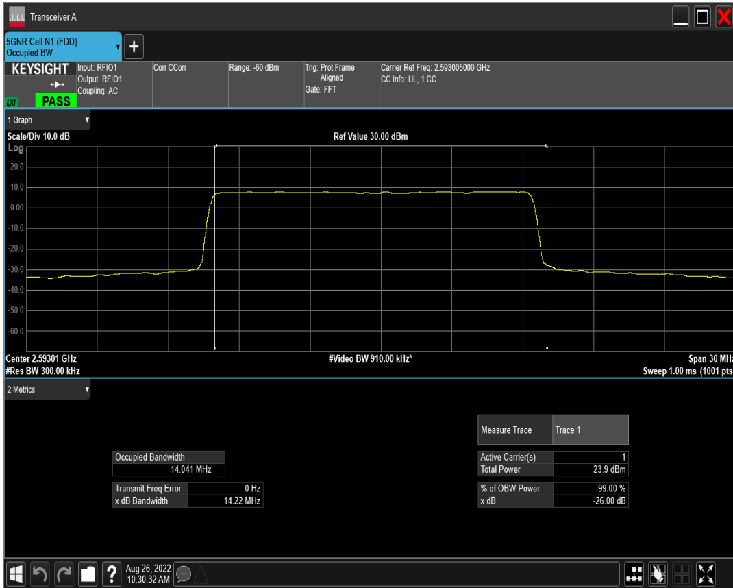
n41 SCS=15kHz DFT_QAM64 BW=15MHz Channel=518601 RB=75@0
