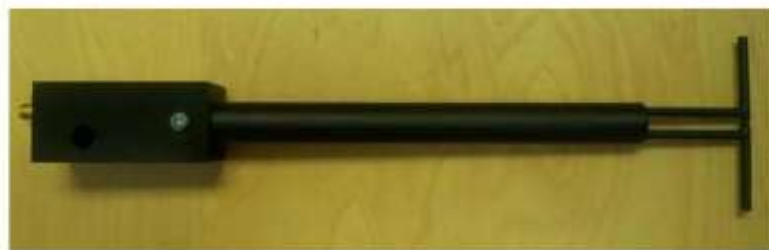
Figure 1 – MVG COMOSAR Validation Dipole
