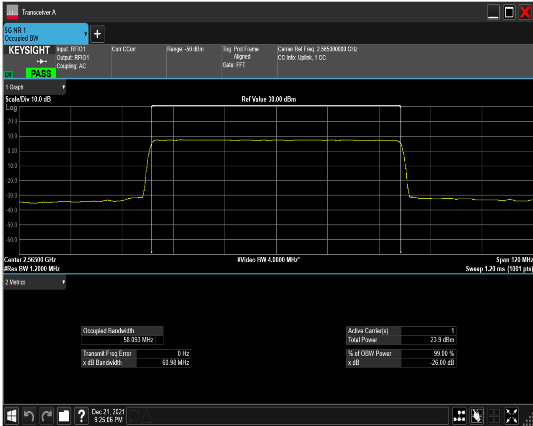
n41(2535-2655) SCS=30kHz DFT_QAM64 BW=60MHz Channel=513000 RB=162@0
