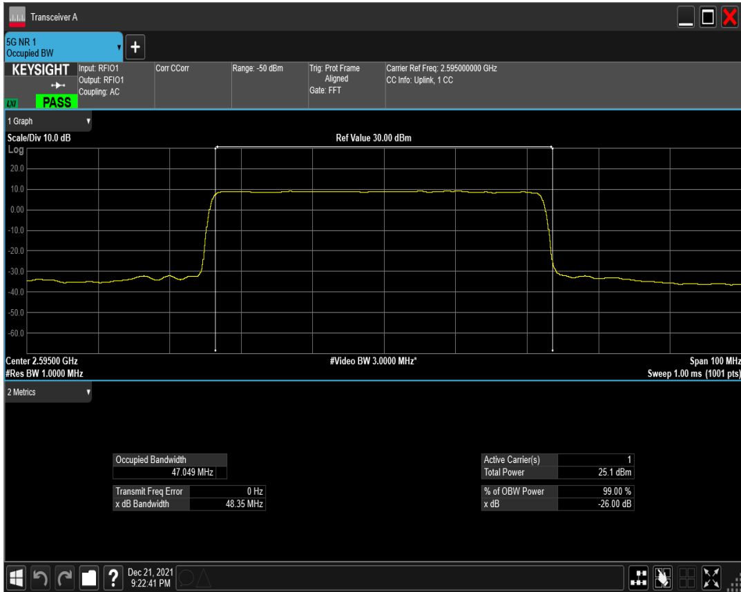
n41(2535-2655) SCS=30kHz DFT_QAM16 BW=50MHz Channel=519000 RB=128@0
