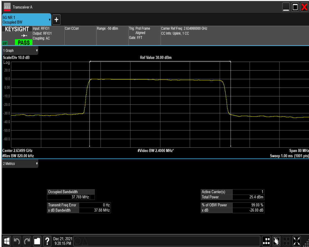
n41(2535-2655) SCS=30kHz DFT_QAM16 BW=40MHz Channel=526998 RB=100@0
