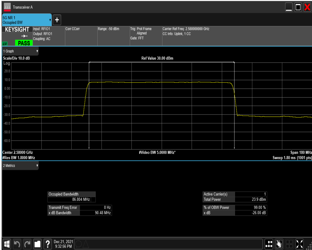
n41(2535-2655) SCS=30kHz DFT_QAM64 BW=90MHz Channel=516000 RB=240@0
