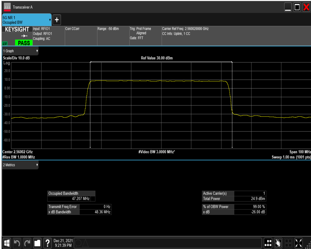
n41(2535-2655) SCS=30kHz DFT_QAM16 BW=50MHz Channel=512004 RB=128@0
