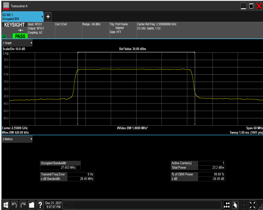
n41(2535-2655) SCS=30kHz DFT_QAM256 BW=30MHz Channel=509004 RB=75@0
