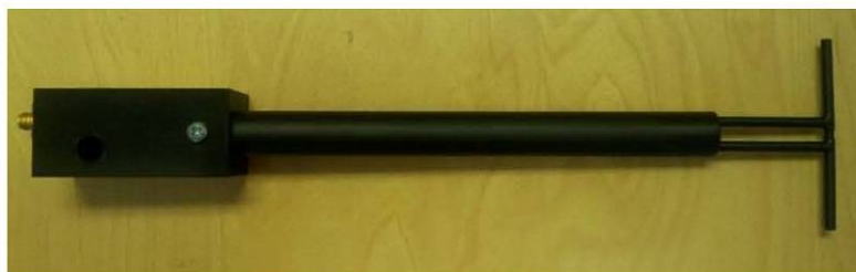
Figure 1 – MVG COMOSAR Validation Dipole
