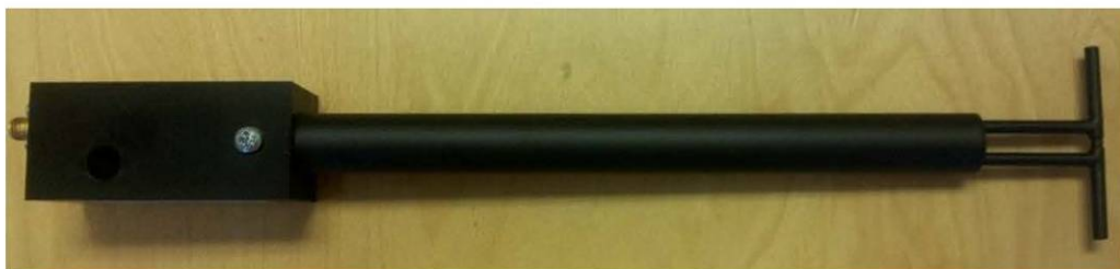
Figure 1 – MVG COMOSAR Validation Dipole
