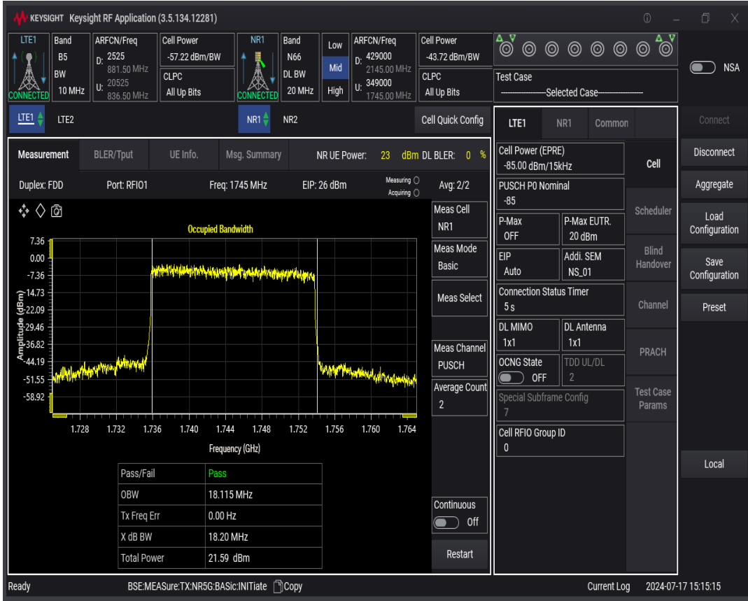
n66 SCS=30kHz DFT_QAM256 BW=40MHz Channel=349000 RB=100@0
