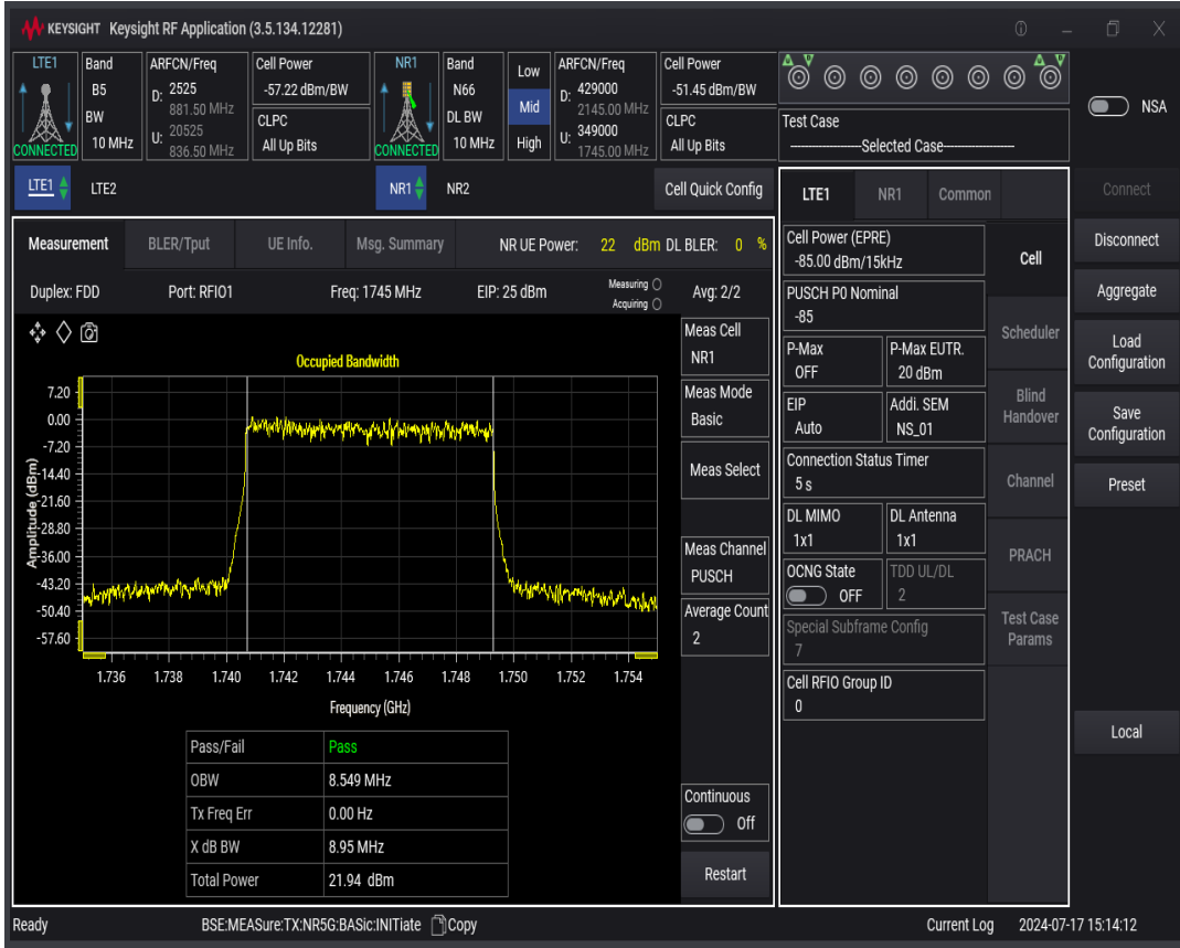
n66 SCS=30kHz DFT_QAM64 BW=15MHz Channel=349000 RB=36@0
