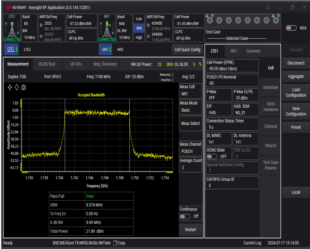
n66 SCS=30kHz DFT_QPSK BW=15MHz Channel=349000 RB=36@0
