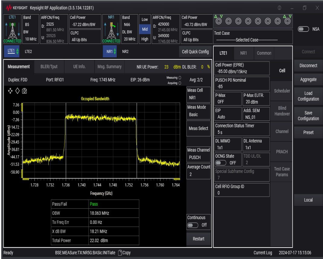
n66 SCS=30kHz DFT_QAM16 BW=40MHz Channel=349000 RB=100@0
