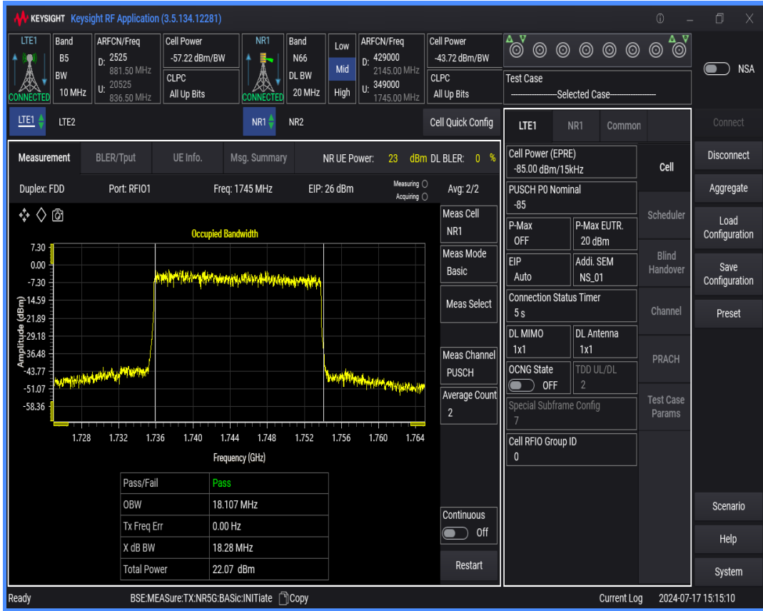
n66 SCS=30kHz DFT_QAM64 BW=40MHz Channel=349000 RB=100 @0
