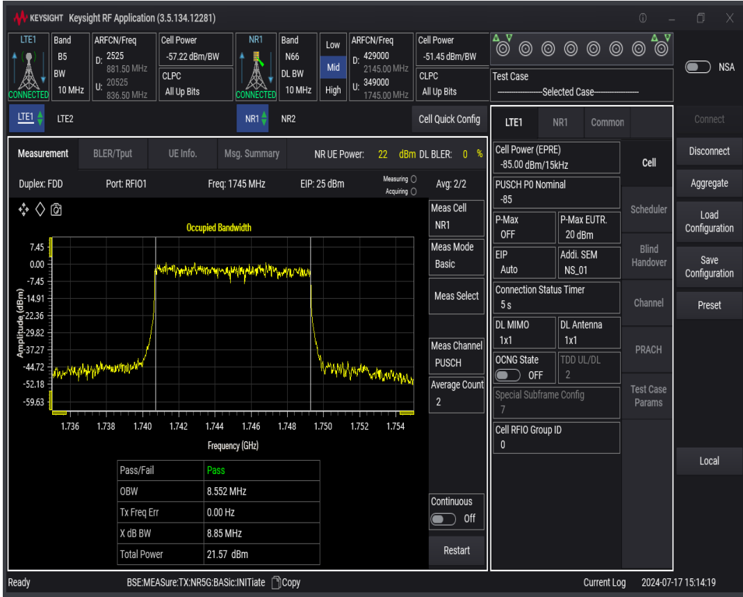
n66 SCS=30kHz DFT_QAM256 BW=15MHz Channel=349000 RB=36 @0
