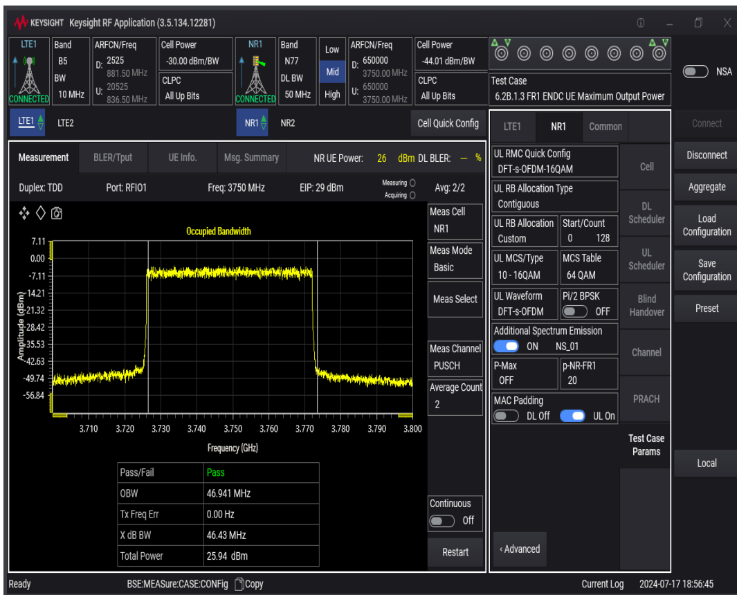
n77 SCS=30kHz DFT_QAM16 BW=60MHz Channel=650000 RB=162 @0
