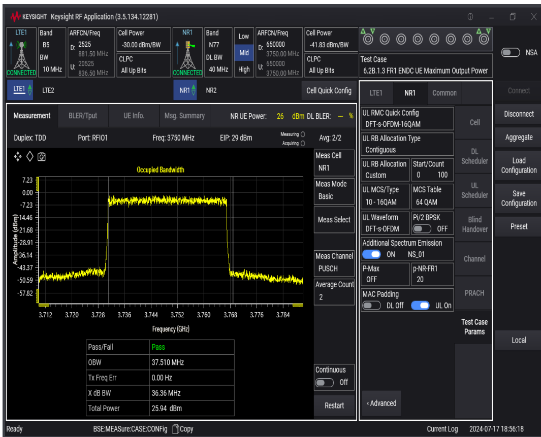
n77 SCS=30kHz DFT_QAM16 BW=50MHz Channel=650000 RB=128 @0
