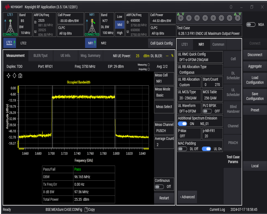
n77 SCS=30kHz DFT_QAM256 BW=10MHz Channel=650000 RB=24 @0
