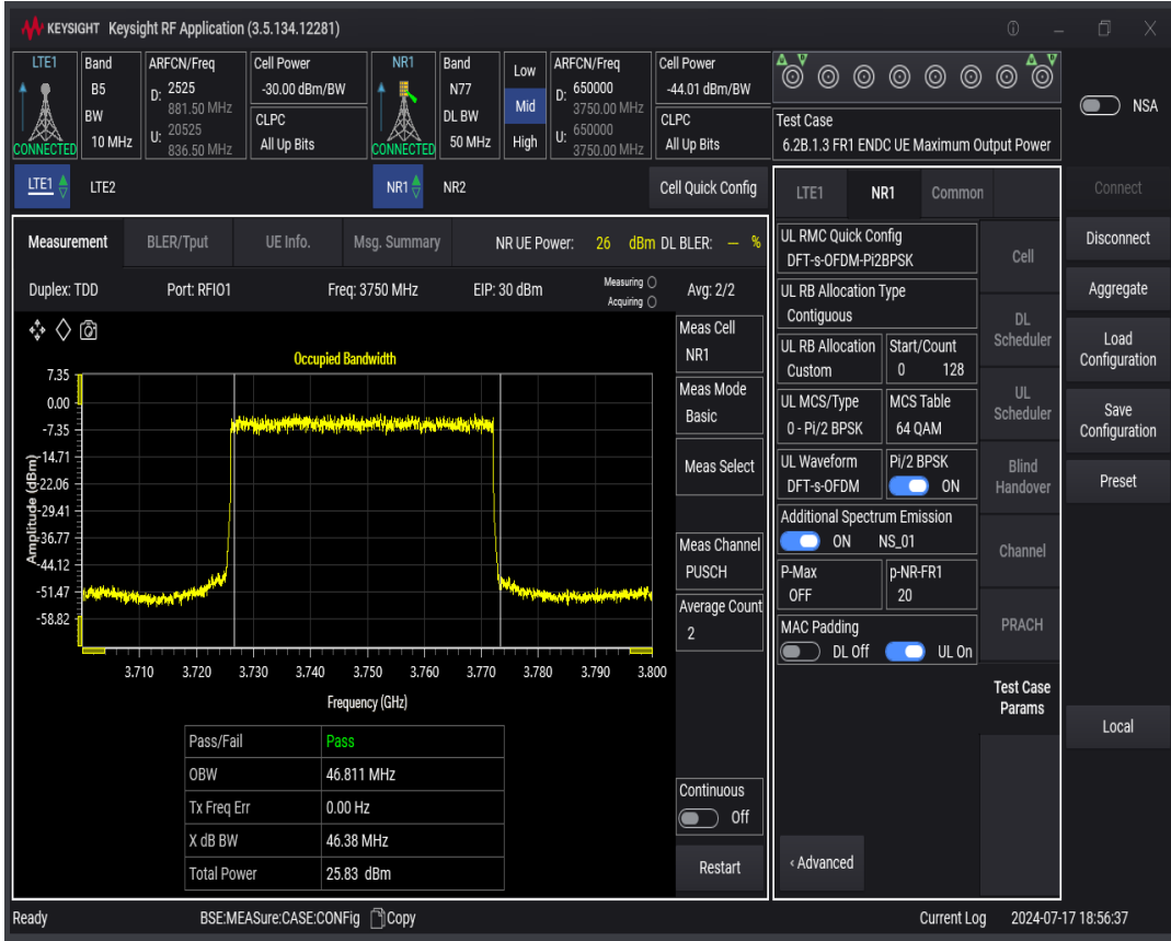
n77 SCS=30kHz DFT_BPSK BW=60MHz Channel=650000 RB=162@0
