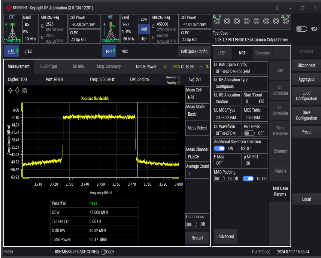
n77 SCS=30kHz DFT_QAM256 BW=60MHz Channel=650000 RB=162 @0
