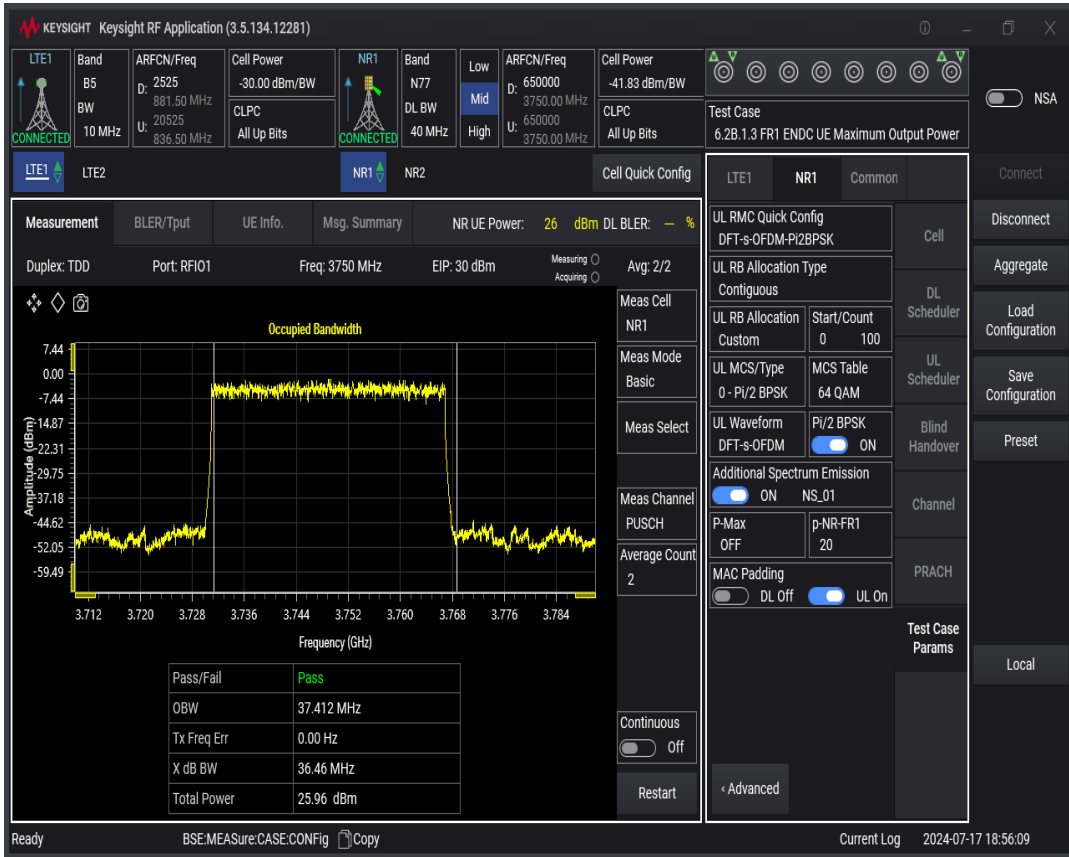
n77 SCS=30kHz DFT_BPSK BW=50MHz Channel=650000 RB=128@0
