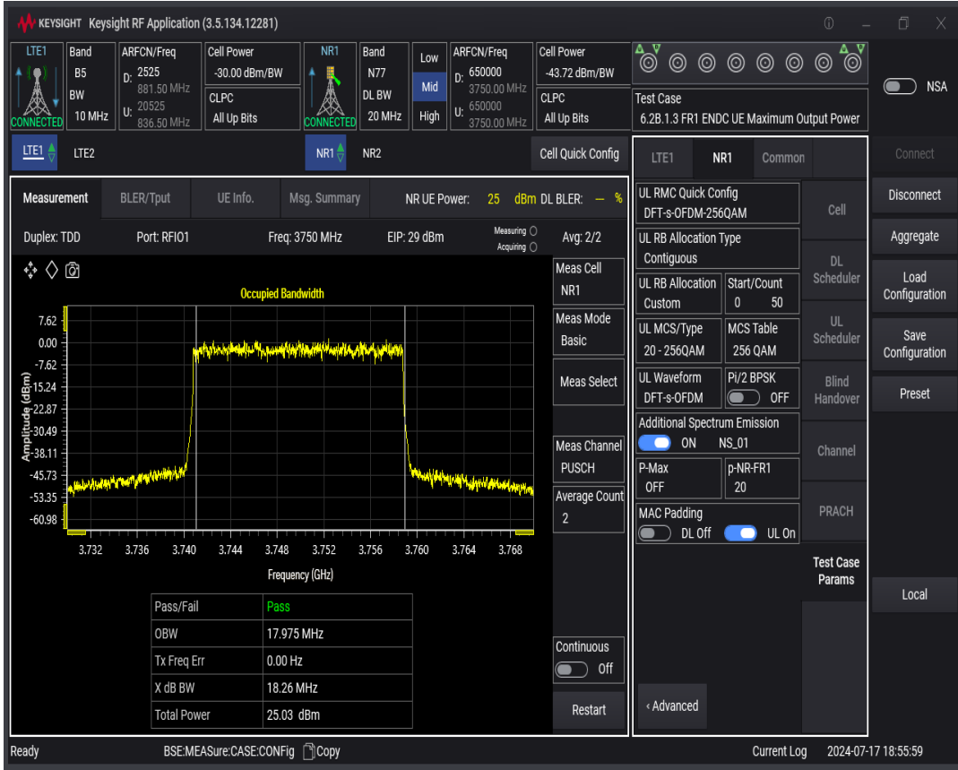
n77 SCS=30kHz DFT_QAM256 BW=40MHz Channel=65000 RB=100@0
