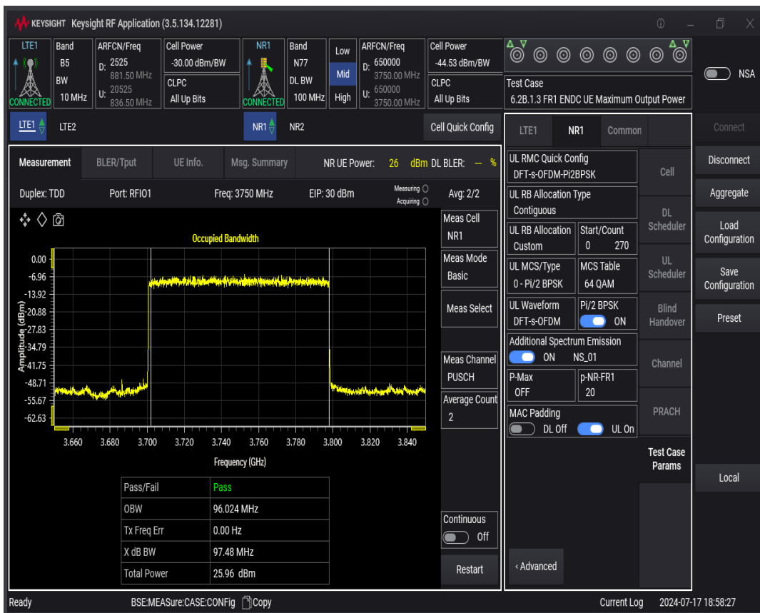
n77 SCS=30kHz DFT_BPSK BW=10MHz Channel=650000 RB=24@0
