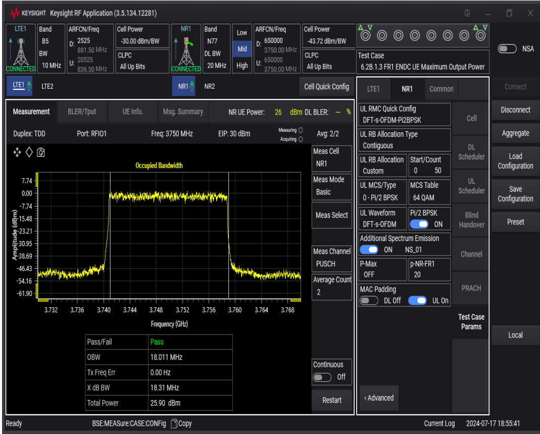
n77 SCS=30kHz DFT_BPSK BW=40MHz Channel=650000 RB=100@0
