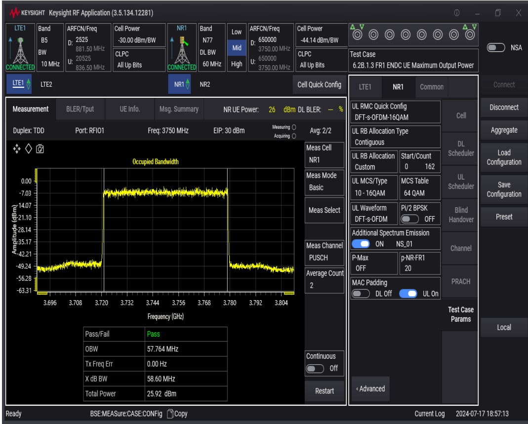
n77 SCS=30kHz DFT_QAM16 BW=80MHz Channel=650000 RB=216 @0
