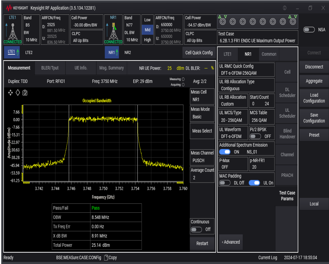
n77 SCS=30kHz DFT_QAM256 BW=15MHz Channel=650000 RB=36@0
