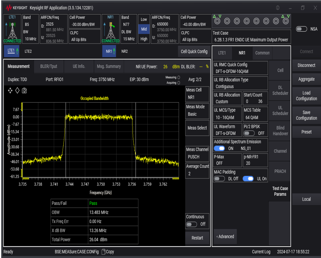
n77 SCS=30kHz DFT_QAM16 BW=20MHz Channel=650000 RB=50@0
