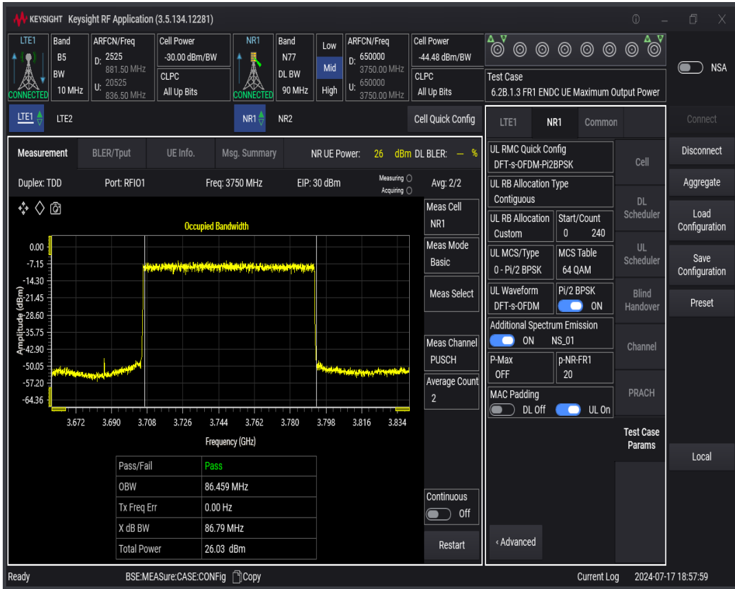
n77 SCS=30kHz DFT_QAM16 BW=100MHz Channel=650000 RB=270@0
