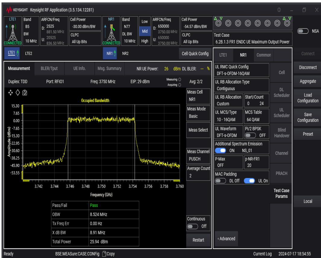
n77 SCS=30kHz DFT_QAM16 BW=15MHz Channel=65000 RB=36@0
