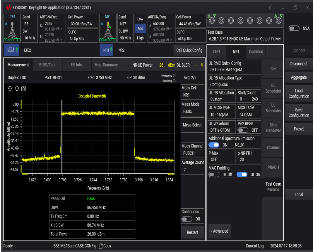
n77 SCS=30kHz DFT_QAM256 BW=100MHz Channel=650000 RB=270 @0
