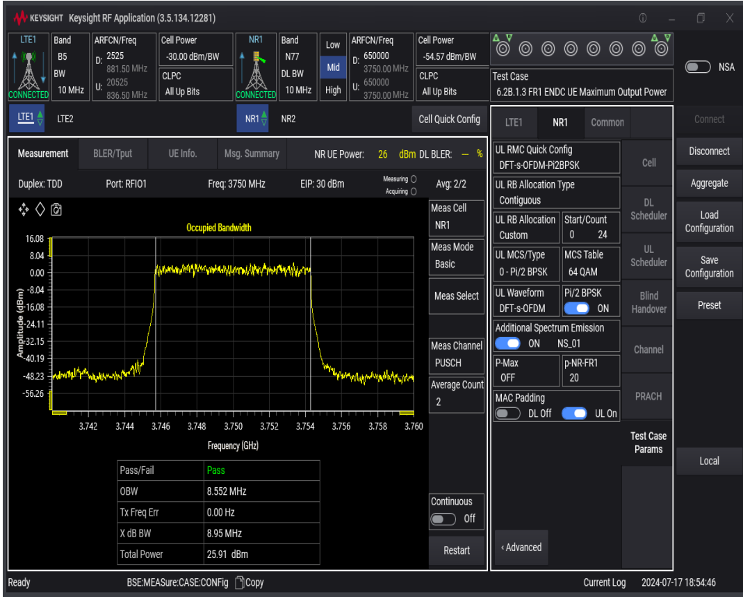
n77 SCS=30kHz DFT_BPSK BW=15MHz Channel=650000 RB=36@0
