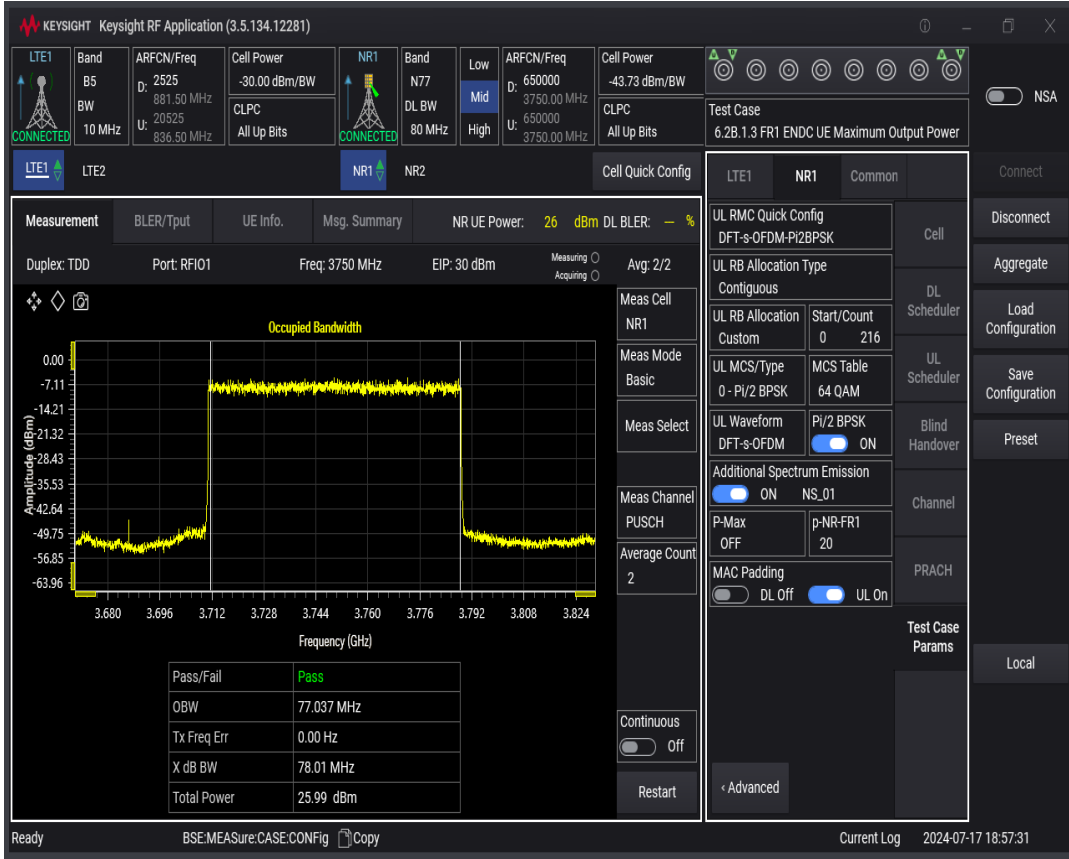
n77 SCS=30kHz DFT_BPSK BW=90MHz Channel=650000 RB=240@0
