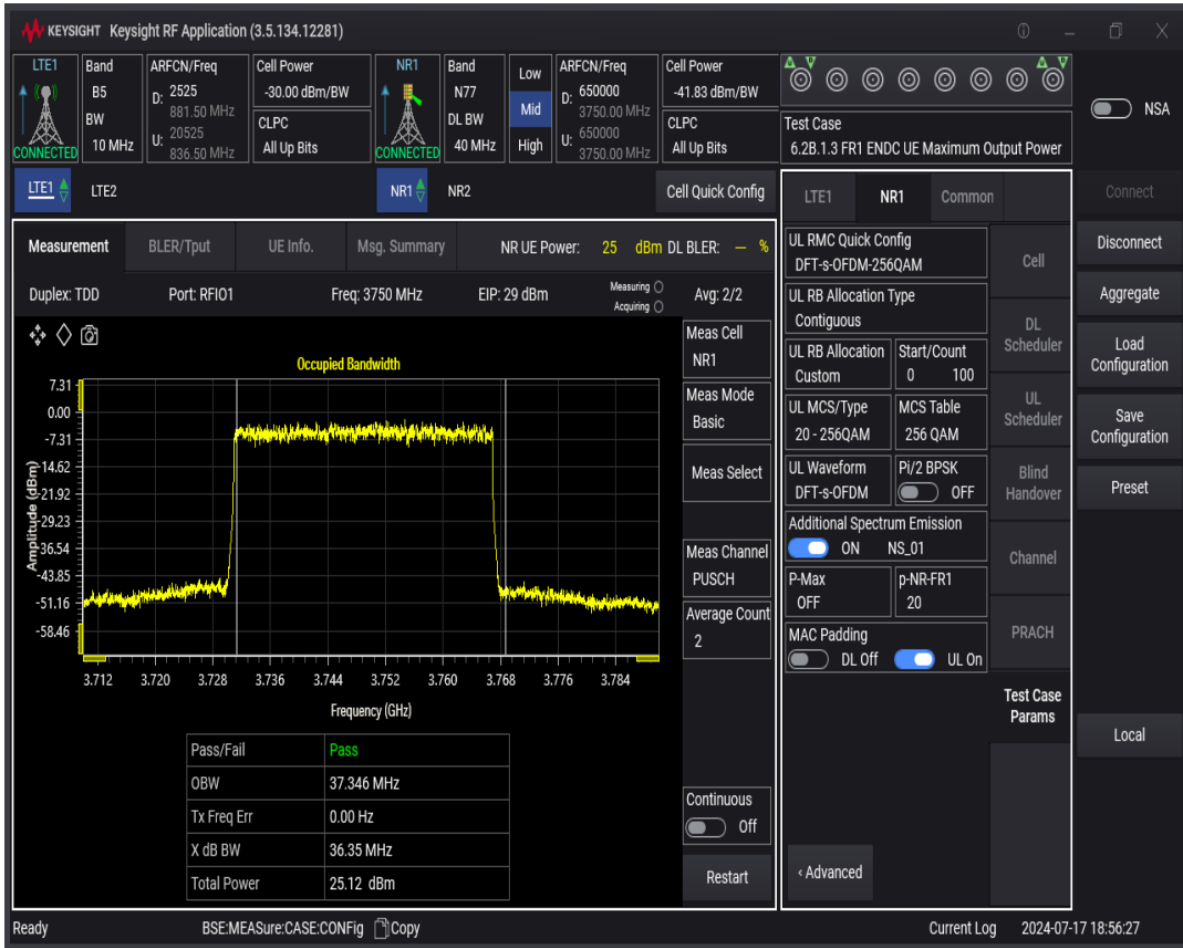
n77 SCS=30kHz DFT_QAM256 BW=50MHz Channel=65000 RB=128@0
