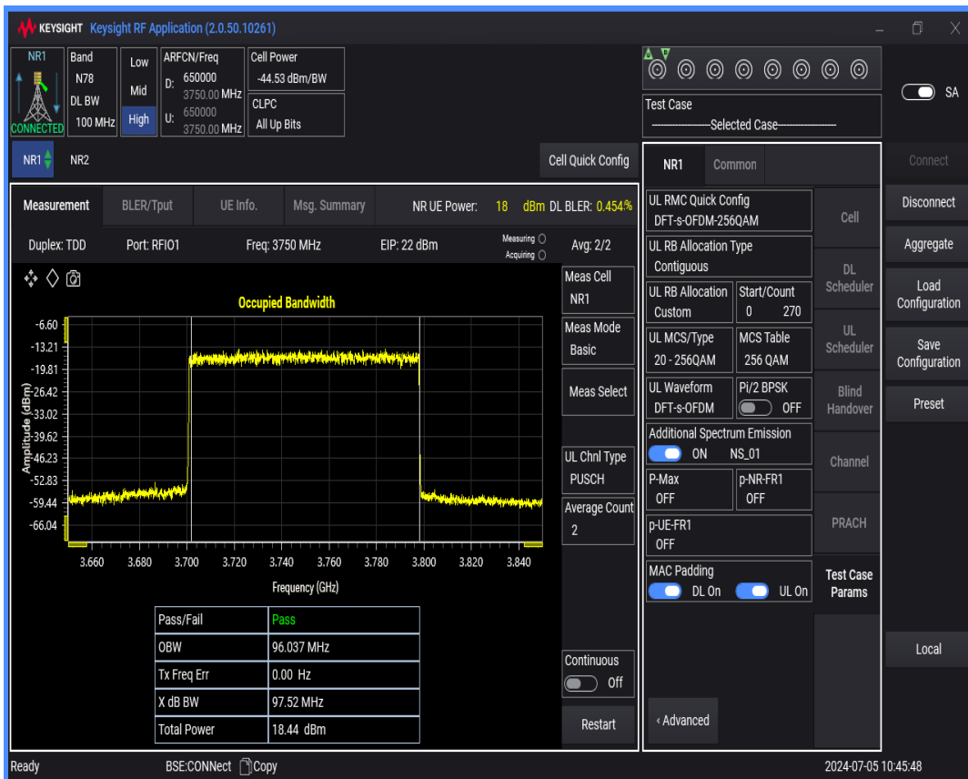
n78(3700-3800) SCS=30kHz DFT_QAM256 BW=10MHz Channel=650000 RB=24@0
