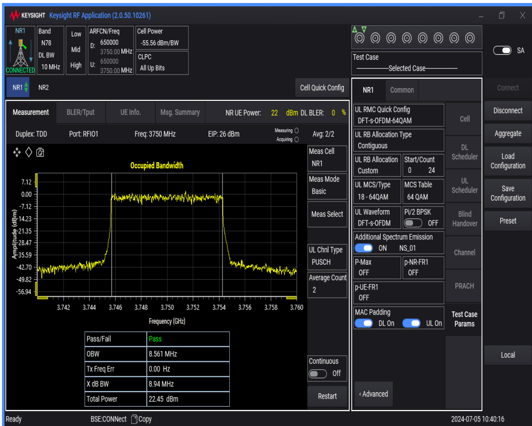
n78(3700-3800) SCS=30kHz DFT_QAM64 BW=15MHz Channel=650000 RB=36@0
