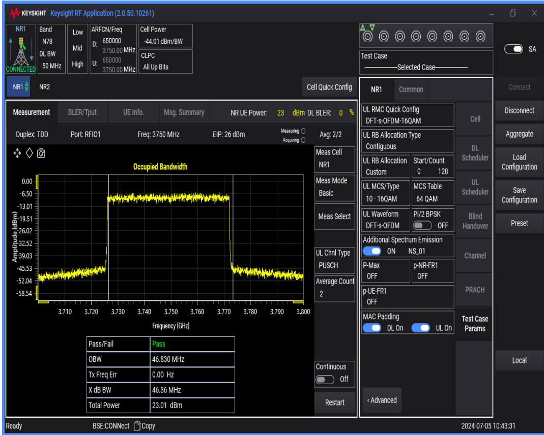
n78(3700-3800) SCS=30kHz DFT_QAM16 BW=60MHz Channel=650000 RB=162@0
