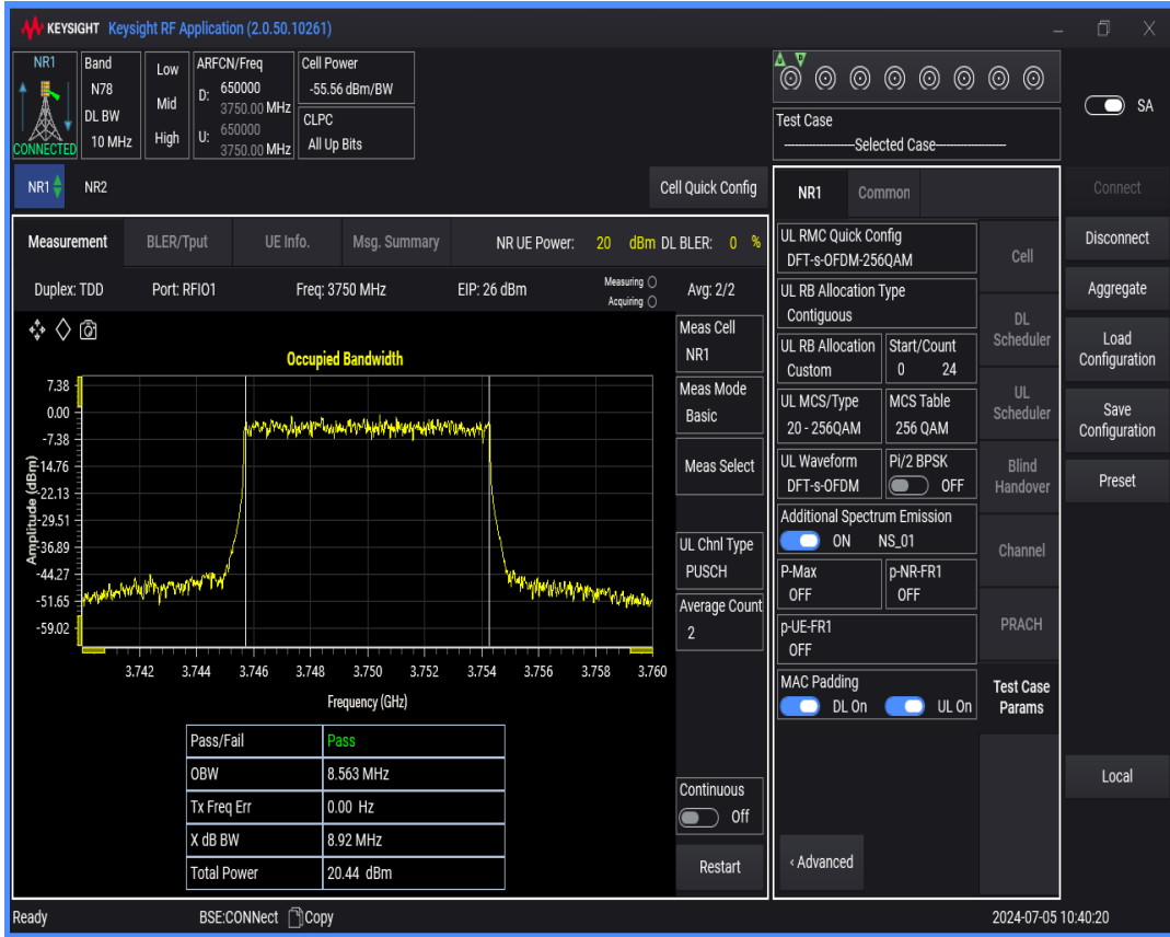
n78(3700-3800) SCS=30kHz DFT_QAM256 BW=15MHz Channel=65000 RB=36@0
