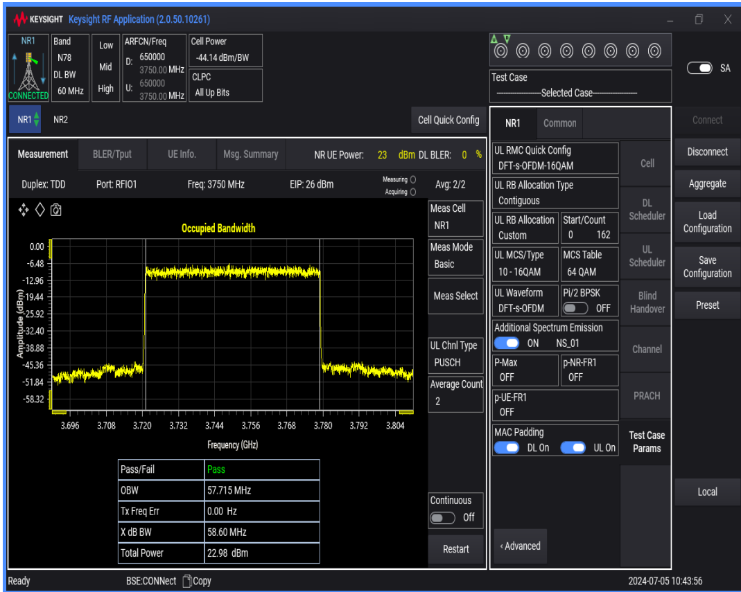
n78(3700-3800) SCS=30kHz DFT_QAM16 BW=70MHz Channel=650000 RB=180@0
