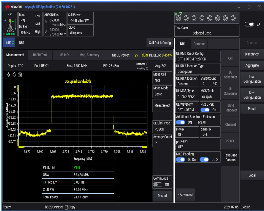
n78(3700-3800) SCS=30kHz DFT_QAM16 BW=100MHz Channel=650000 RB=270@0
