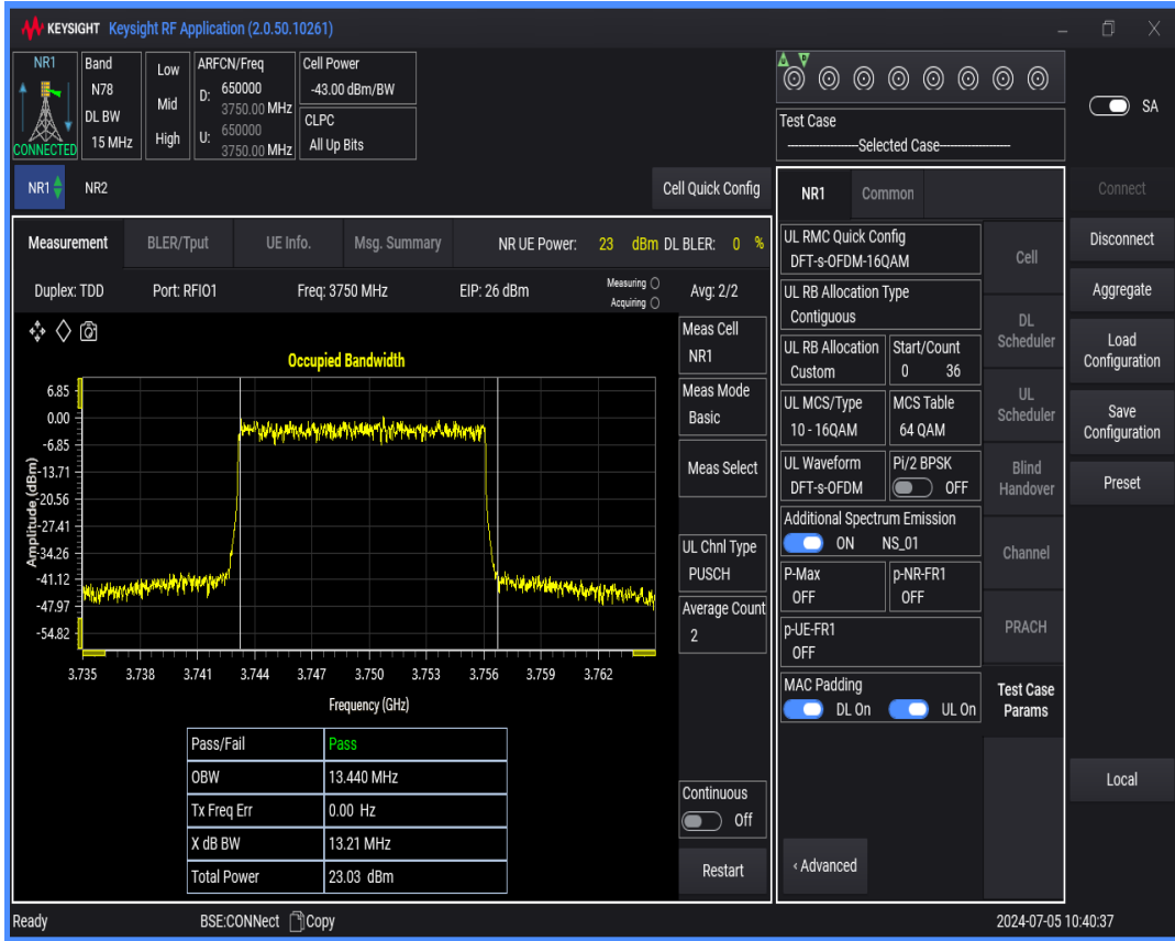
n78(3700-3800) SCS=30kHz DFT_QAM16 BW=20MHz Channel=650000 RB=50@0
