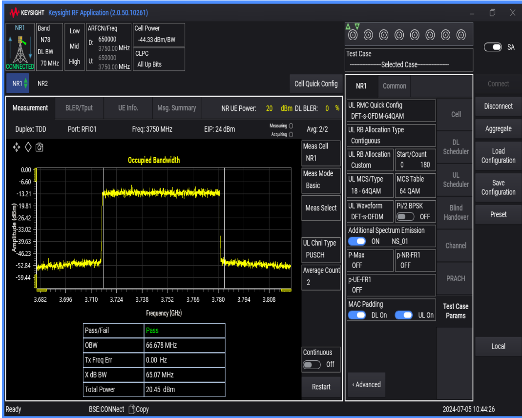
n78(3700-3800) SCS=30kHz DFT_QAM64 BW=80MHz Channel=650000 RB=216@0
