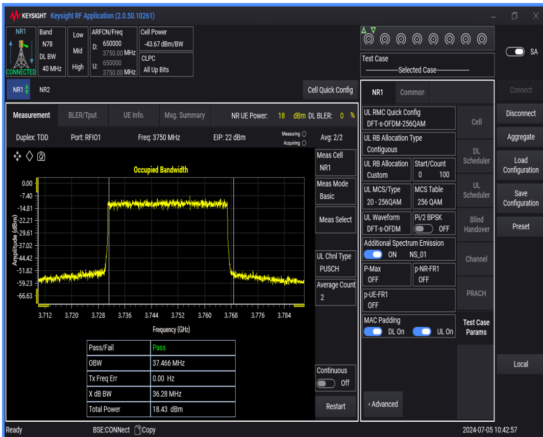
n78(3700-3800) SCS=30kHz DFT_QAM256 BW=50MHz Channel=650000 RB=128@0
