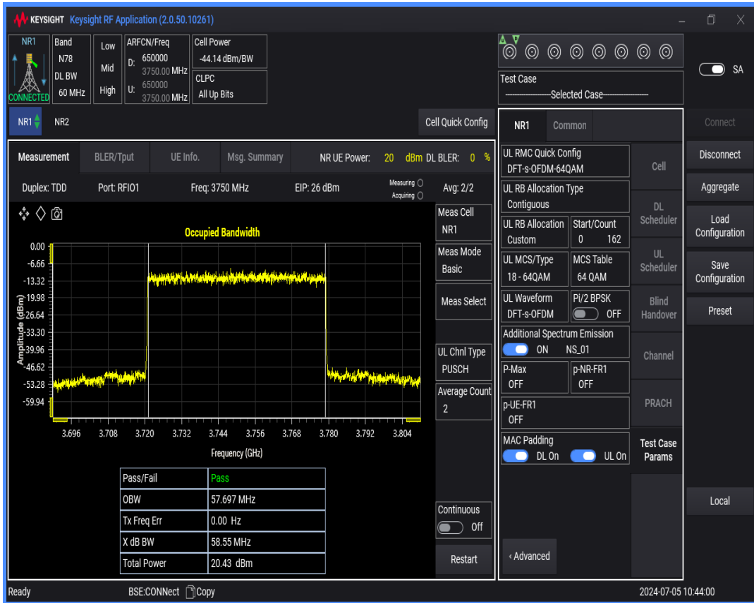
n78(3700-3800) SCS=30kHz DFT_QAM64 BW=70MHz Channel=650000 RB=180@0
