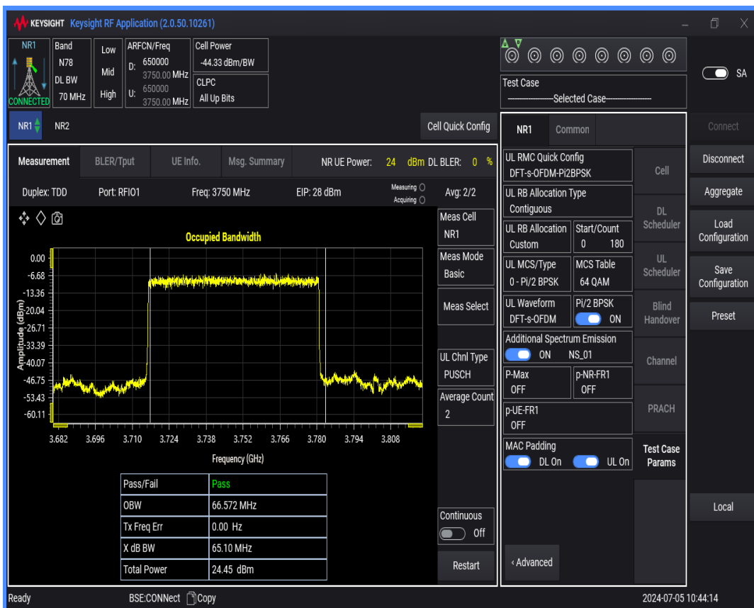
n78(3700-3800) SCS=30kHz DFT_BPSK BW=80MHz Channel=650000 RB=216@0
