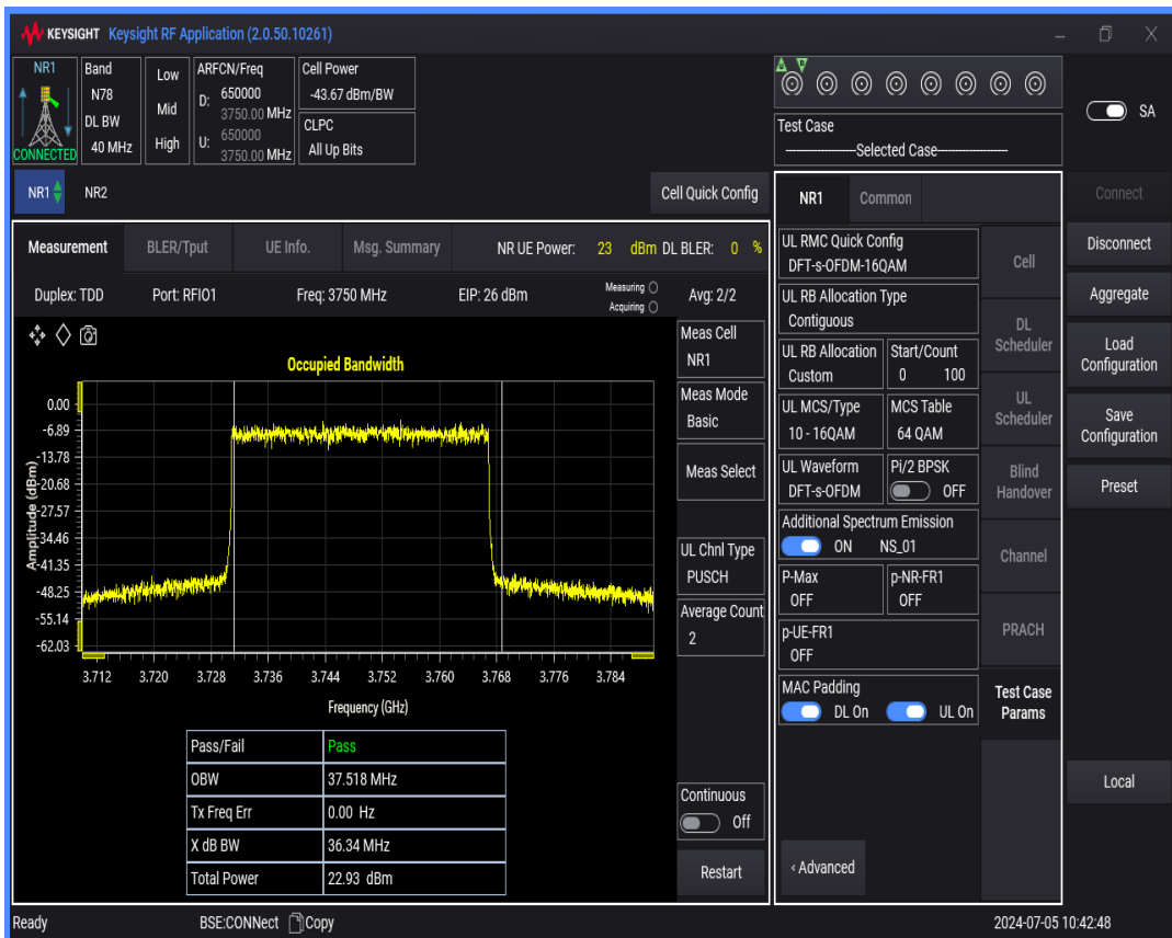
n78(3700-3800) SCS=30kHz DFT_QAM16 BW=50MHz Channel=650000 RB=128@0
