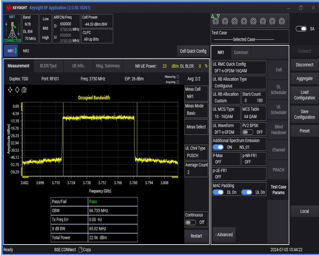
n78(3700-3800) SCS=30kHz DFT_QAM16 BW=80MHz Channel=650000 RB=216@0
