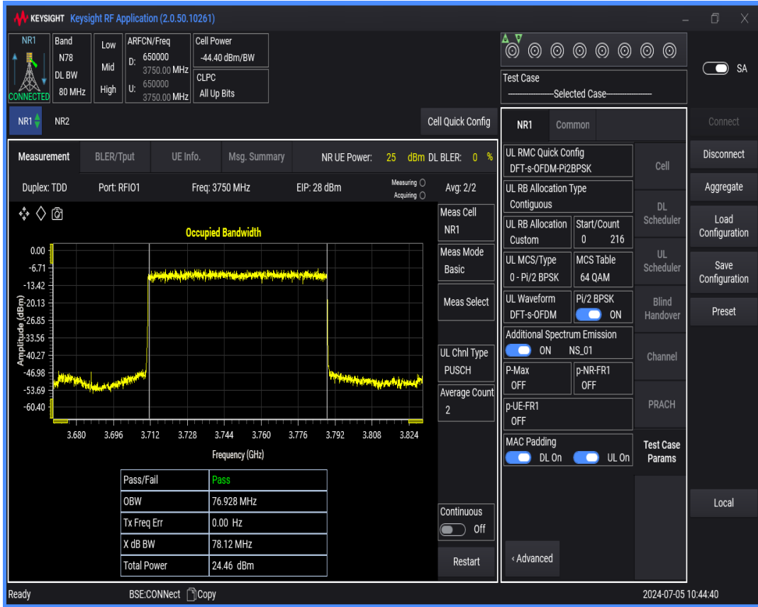
n78(3700-3800) SCS=30kHz DFT_BPSK BW=90MHz Channel=650000 RB=240@0
