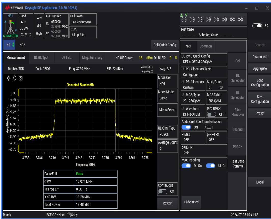
n78(3700-3800) SCS=30kHz DFT_QAM256 BW=30MHz Channel=650000 RB=75@0
