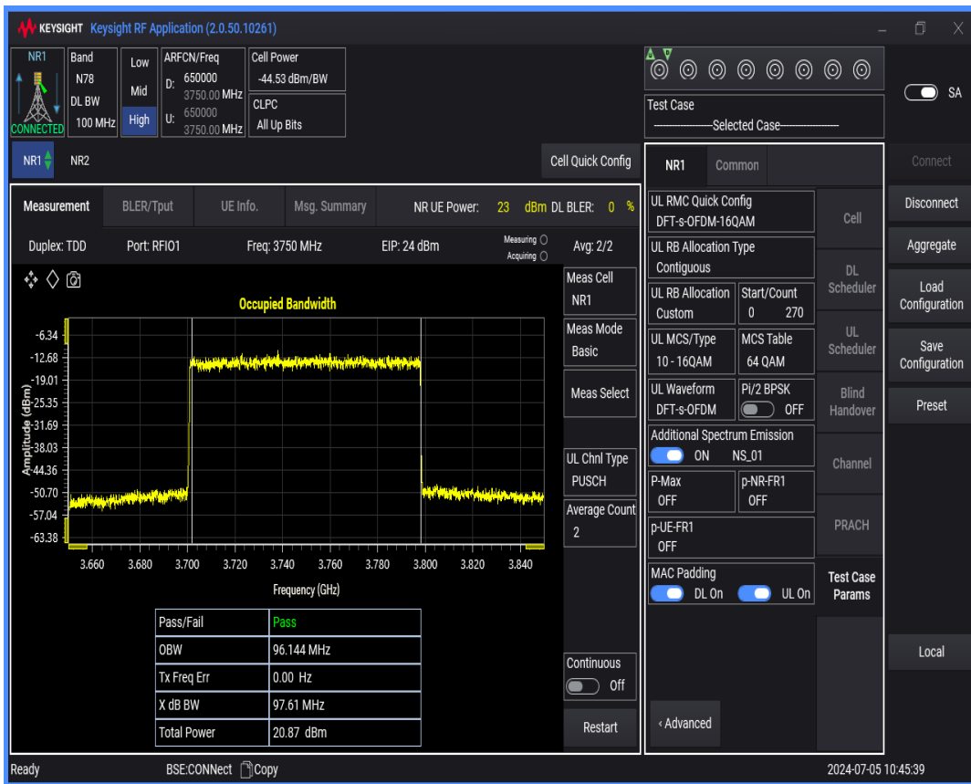
n78(3700-3800) SCS=30kHz DFT_QAM16 BW=10MHz Channel=650000 RB=24@0
