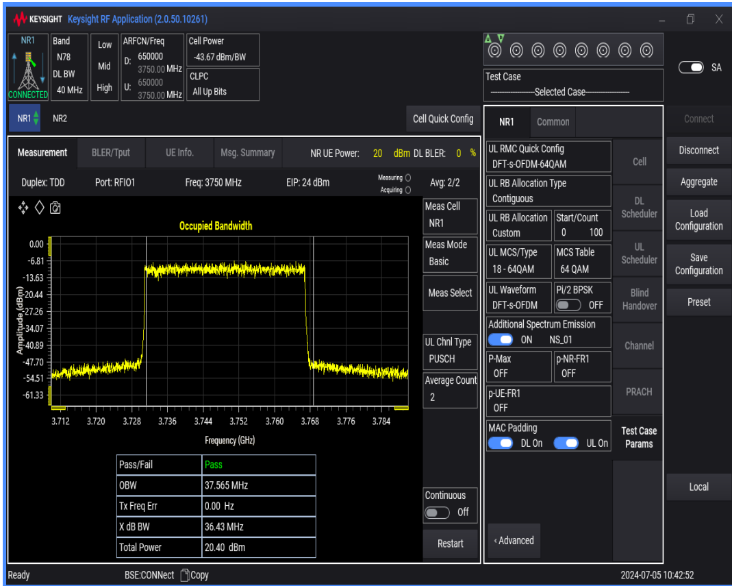
n78(3700-3800) SCS=30kHz DFT_QAM64 BW=50MHz Channel=650000 RB=128@0
