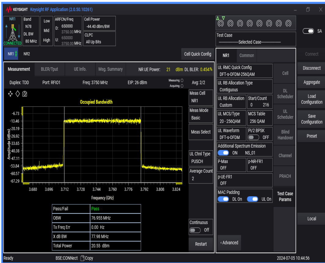
n78(3700-3800) SCS=30kHz DFT_QAM256 BW=90MHz Channel=650000 RB=240@0
