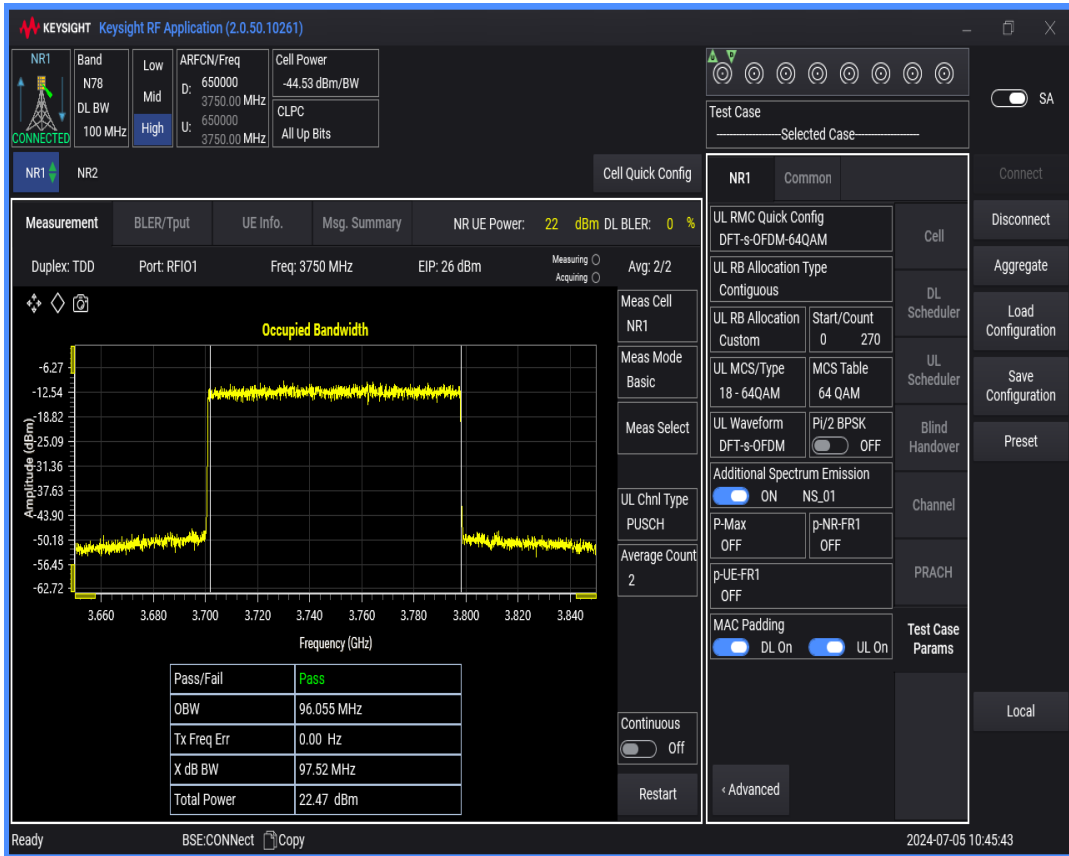
n78(3700-3800) SCS=30kHz DFT_QAM64 BW=10MHz Channel=650000 RB=24@0
