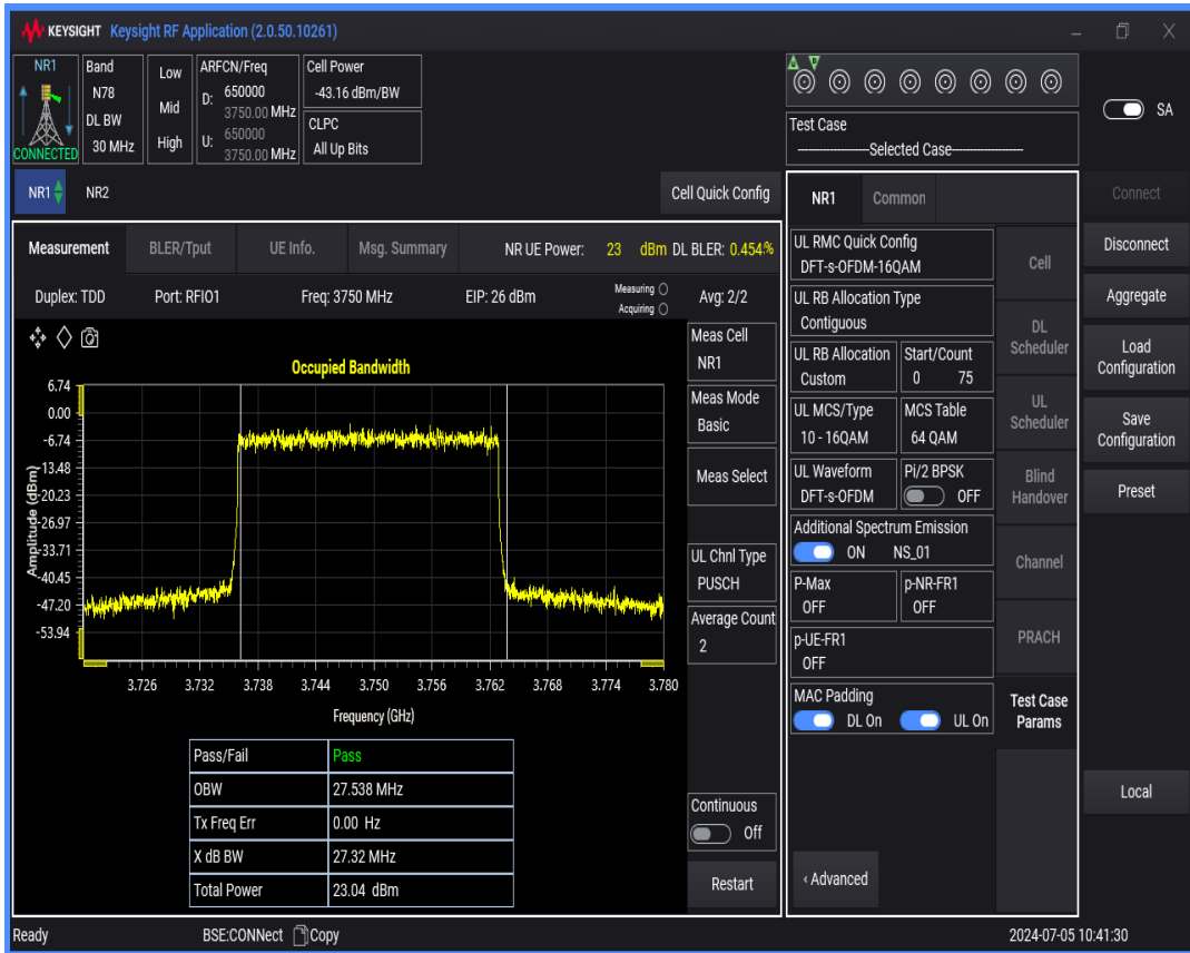
n78(3700-3800) SCS=30kHz DFT_QAM16 BW=40MHz Channel=650000 RB=100@0
