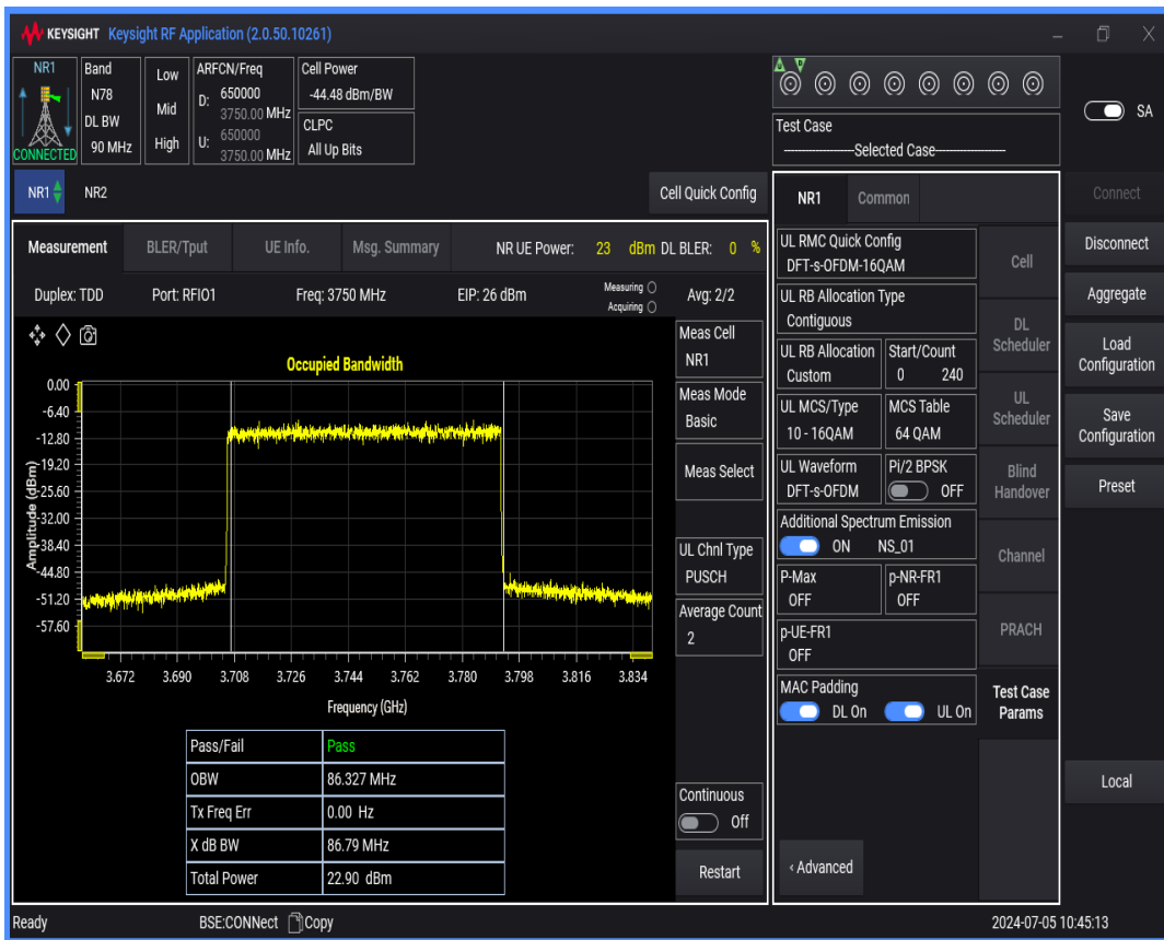
n78(3700-3800) SCS=30kHz DFT_QAM256 BW=100MHz Channel=650000 RB=270@0
