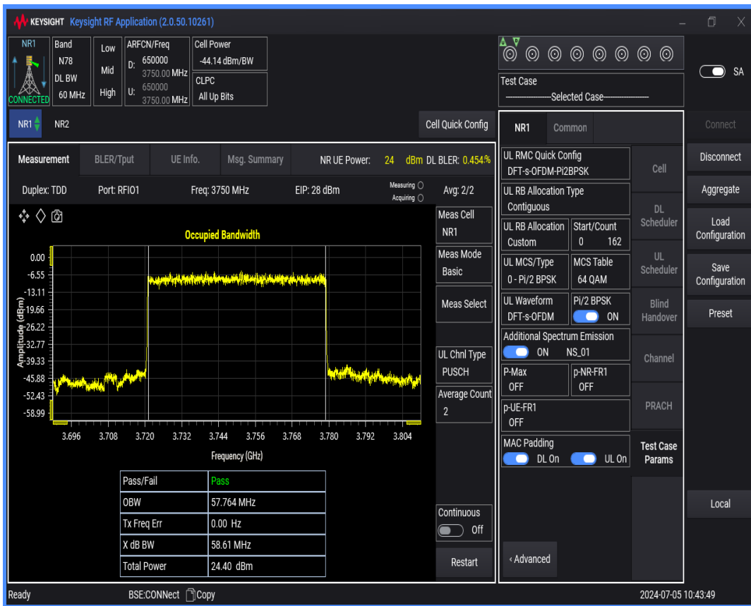
n78(3700-3800) SCS=30kHz DFT_BPSK BW=70MHz Channel=650000 RB=180@0
