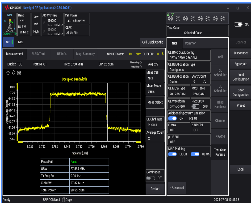
n78(3700-3800) SCS=30kHz DFT_QAM256 BW=40MHz Channel=650000 RB=100@0
