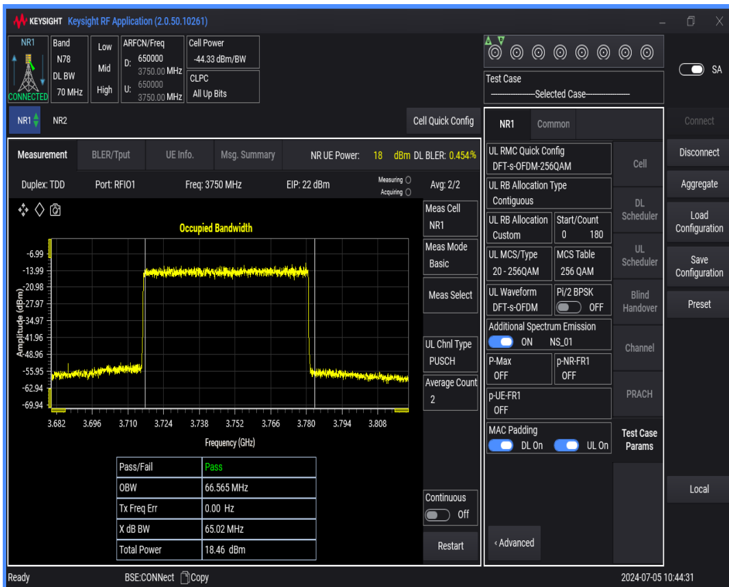
n78(3700-3800) SCS=30kHz DFT_QAM256 BW=80MHz Channel=650000 RB=216@0
