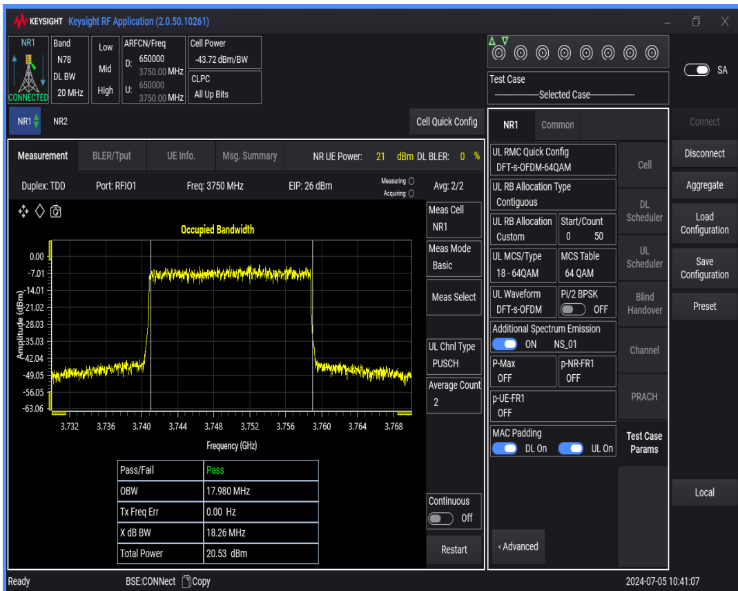
n78(3700-3800) SCS=30kHz DFT_QAM64 BW=30MHz Channel=650000 RB=75@0
