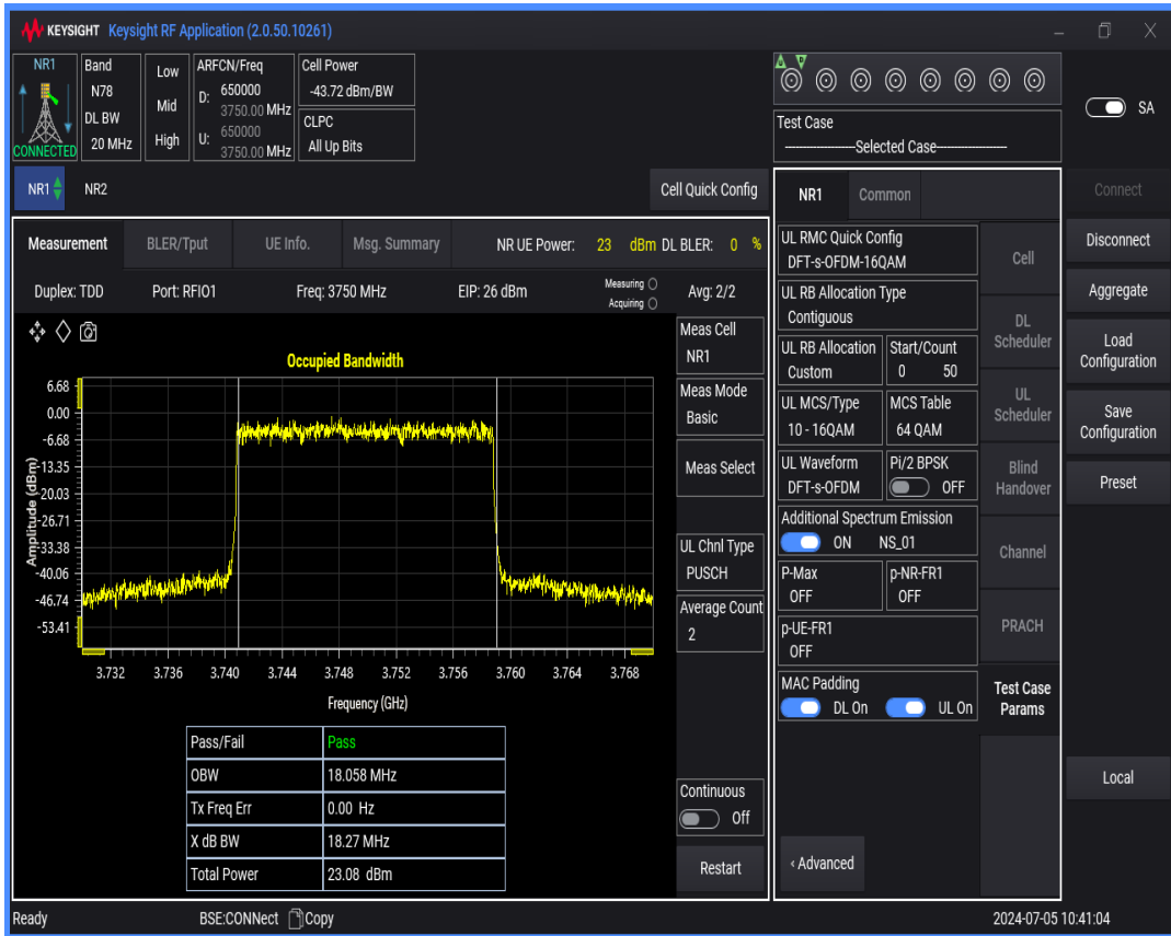
n78(3700-3800) SCS=30kHz DFT_QAM16 BW=30MHz Channel=650000 RB=75@0
