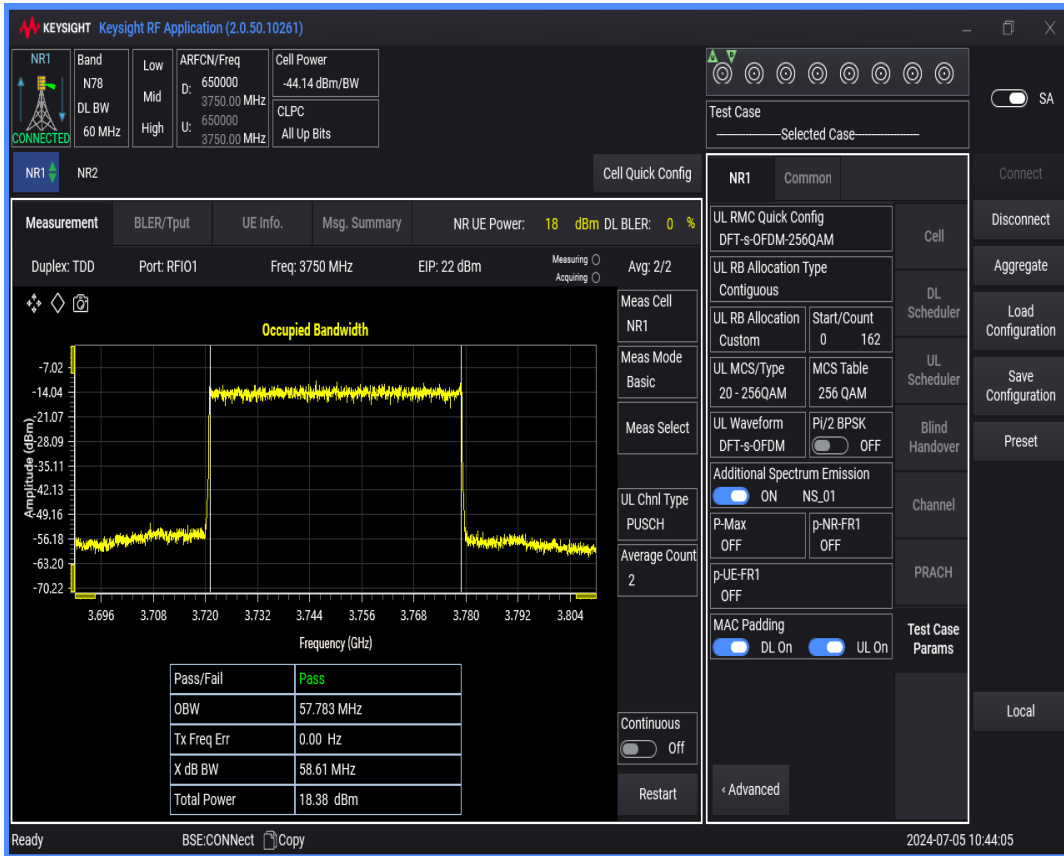
n78(3700-3800) SCS=30kHz DFT_QAM256 BW=70MHz Channel=650000 RB=180@0
