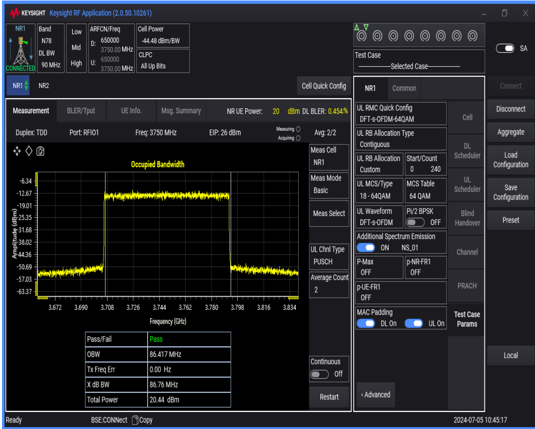
n78(3700-3800) SCS=30kHz DFT_QPSK BW=100MHz Channel=650000 RB=270@0
