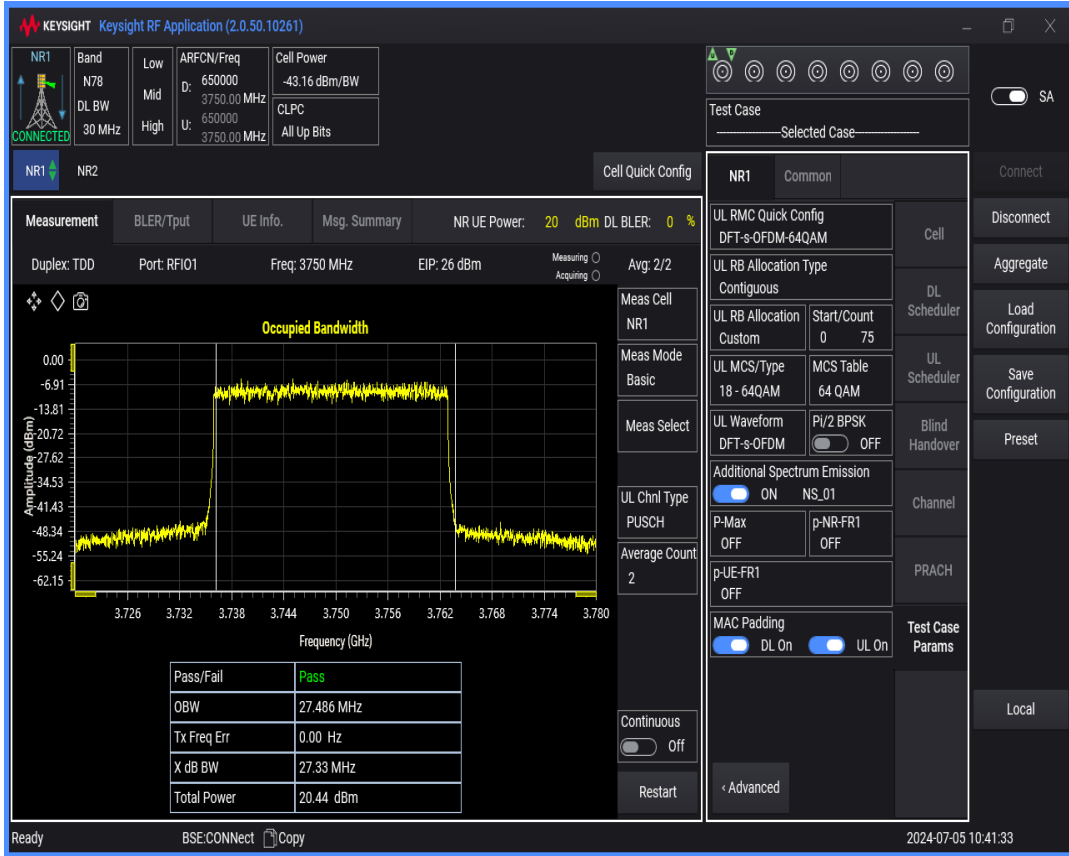
n78(3700-3800) SCS=30kHz DFT_QAM64 BW=40MHz Channel=650000 RB=100@0
