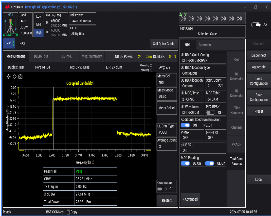
n78(3700-3800) SCS=30kHz DFT_QPSK BW=10MHz Channel=650000 RB=24@0
