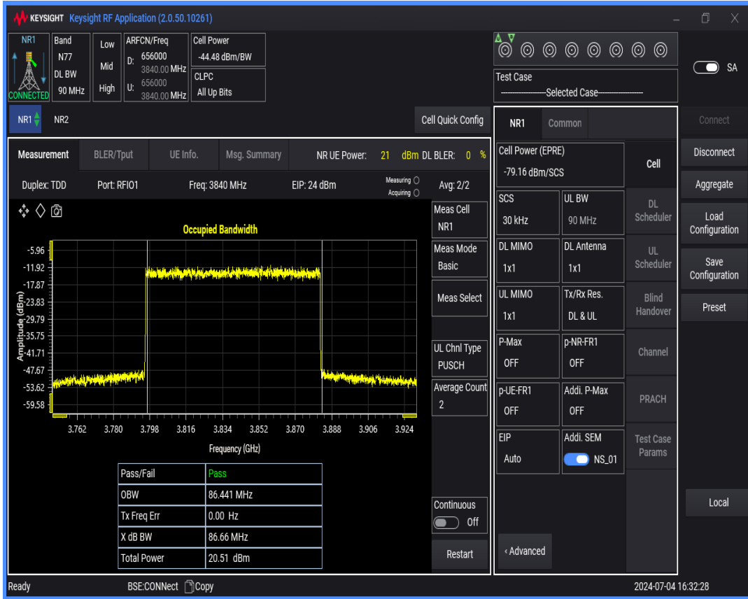
n77(3700-3980) SCS=30kHz DFT_QPSK BW=100MHz Channel=656000 RB=270 @0
