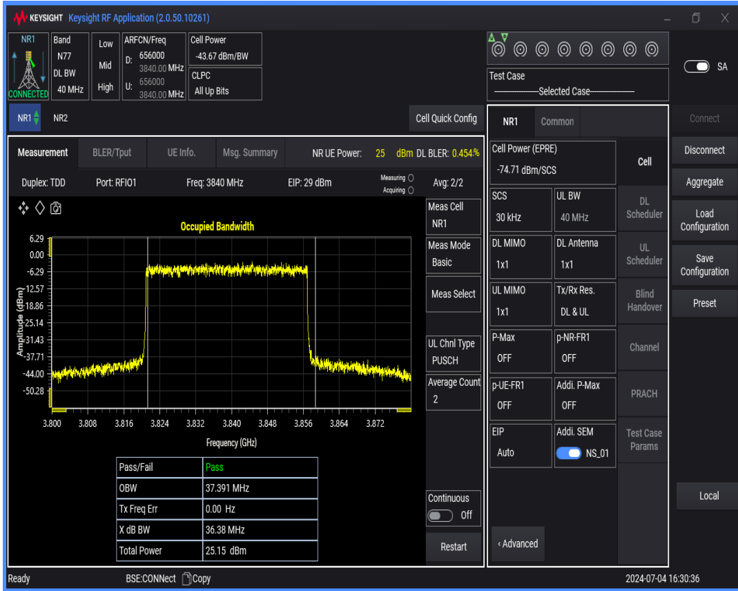
n77(3700-3980) SCS=30kHz DFT_QPSK BW=50MHz Channel=656000 RB=128@0
