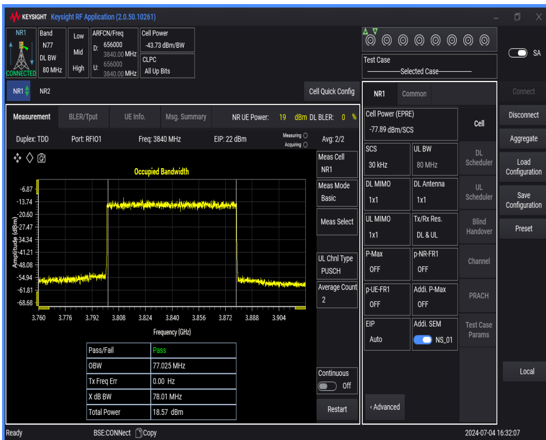
n77(3700-3980) SCS=30kHz DFT_QAM256 BW=90MHz Channel=656000 RB=240@0
