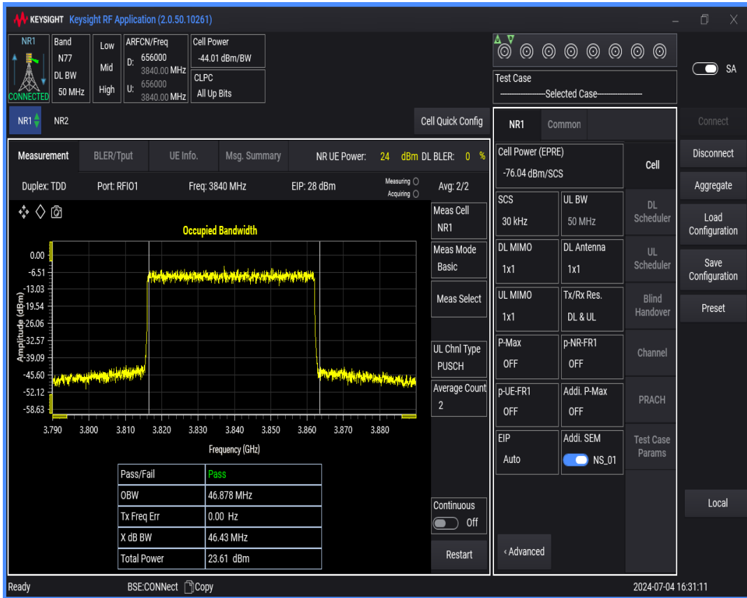
n77(3700-3980) SCS=30kHz DFT_QAM64 BW=60MHz Channel=656000 RB=162@0
