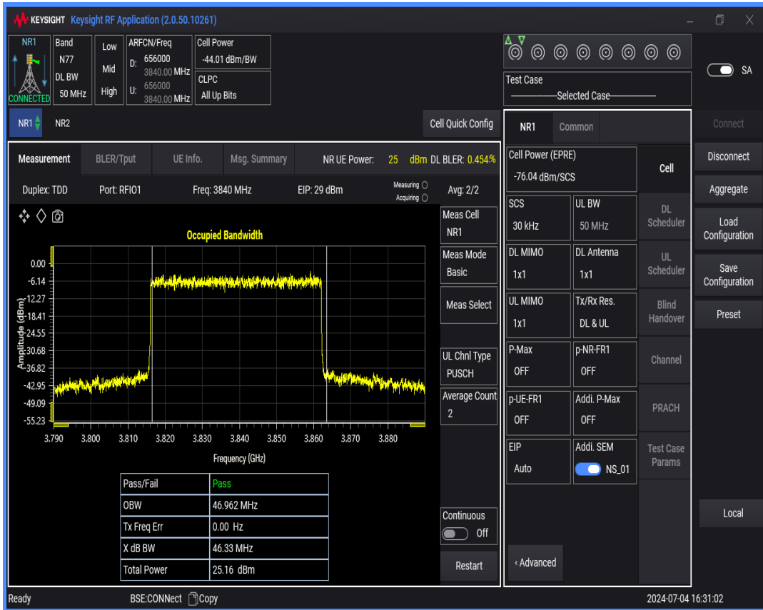
n77(3700-3980) SCS=30kHz DFT_QPSK BW=60MHz Channel=656000 RB=162@0
