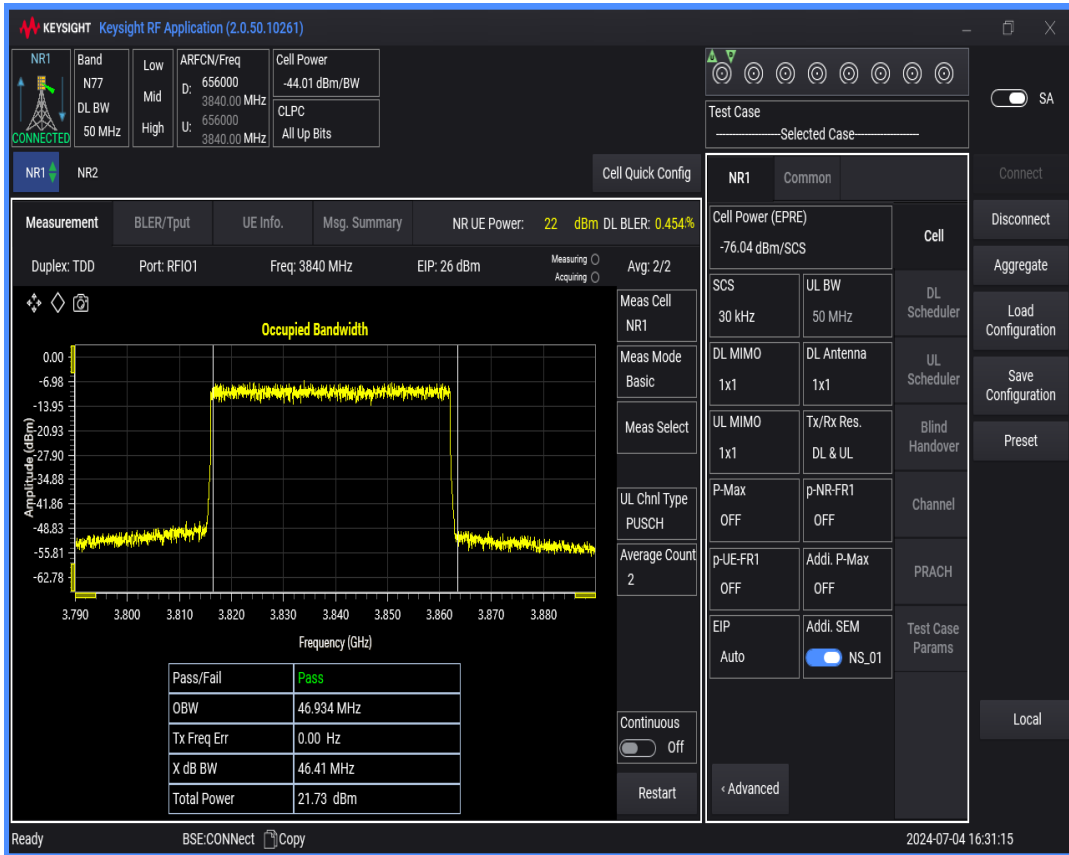
n77(3700-3980) SCS=30kHz DFT_QAM256 BW=60MHz Channel=656000 RB=162@0
