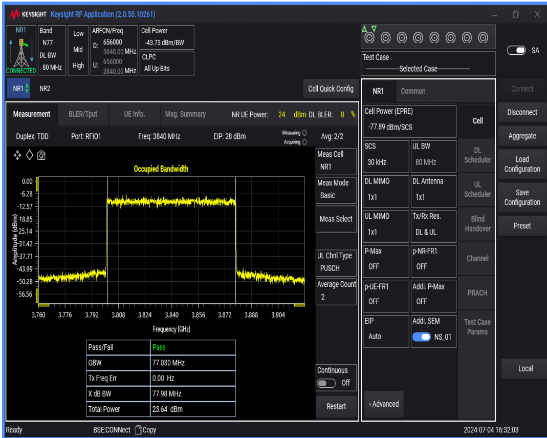
n77(3700-3980) SCS=30kHz DFT_QAM64 BW=90MHz Channel=656000 RB=240@0
