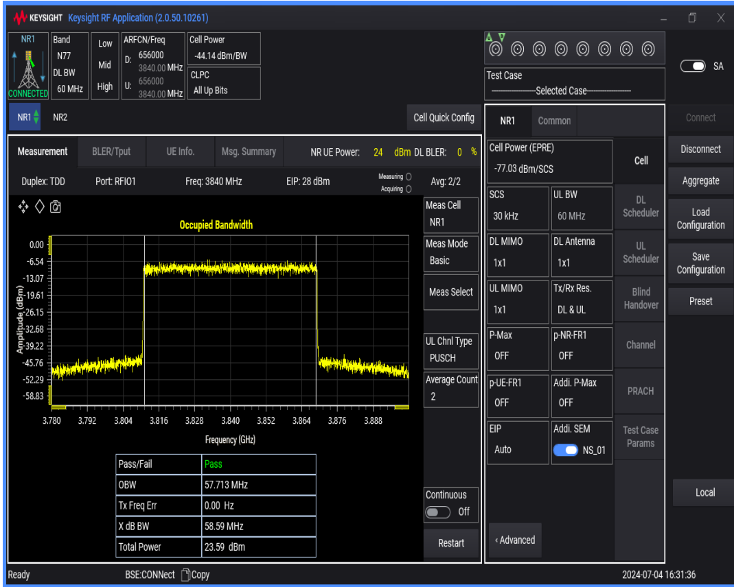
n77(3700-3980) SCS=30kHz DFT_QAM64 BW=80MHz Channel=656000 RB=216@0
