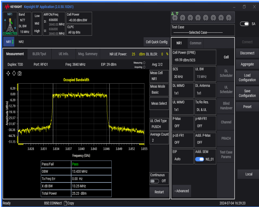
n77(3700-3980) SCS=30kHz DFT_QPSK BW=20MHz Channel=656000 RB=50 @0
