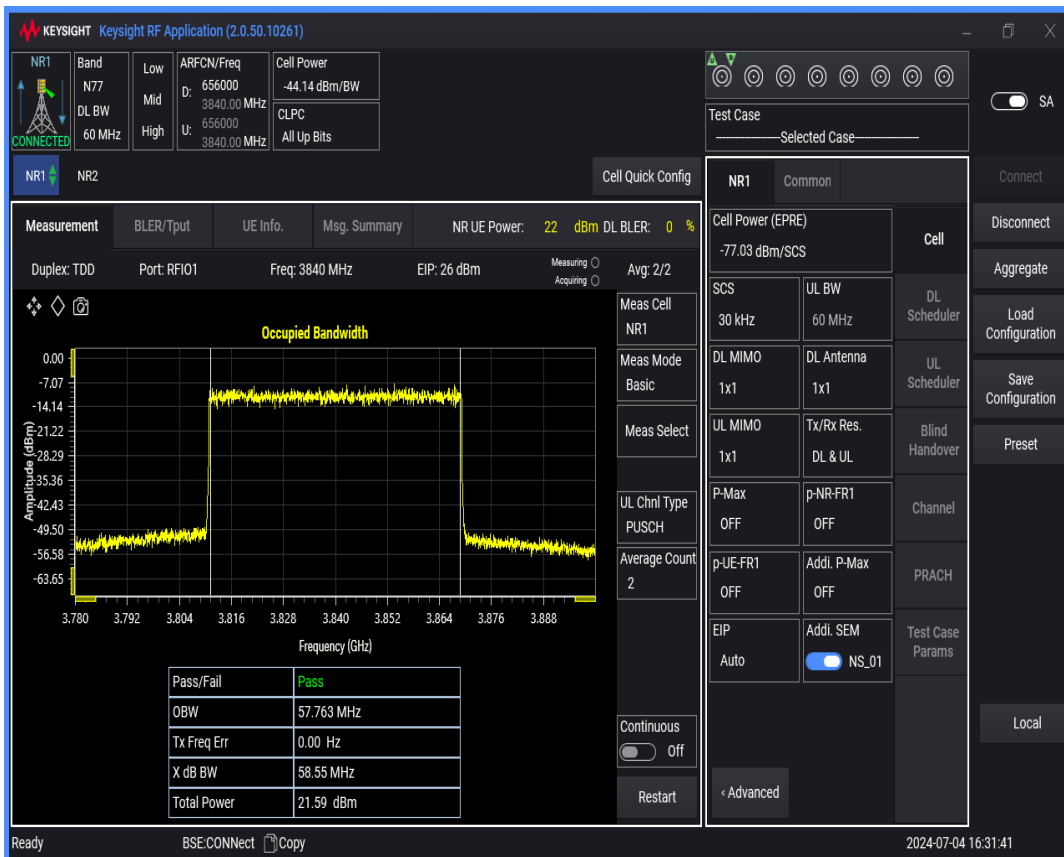
n77(3700-3980) SCS=30kHz DFT_QAM256 BW=80MHz Channel=656000 RB=216@0
