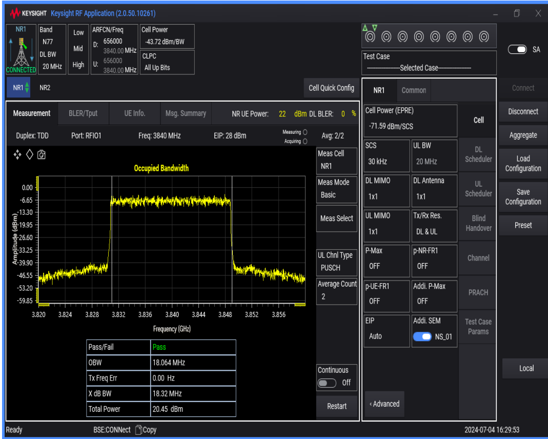
n77(3700-3980) SCS=30kHz DFT_QAM64 BW=30MHz Channel=656000 RB=75@0
