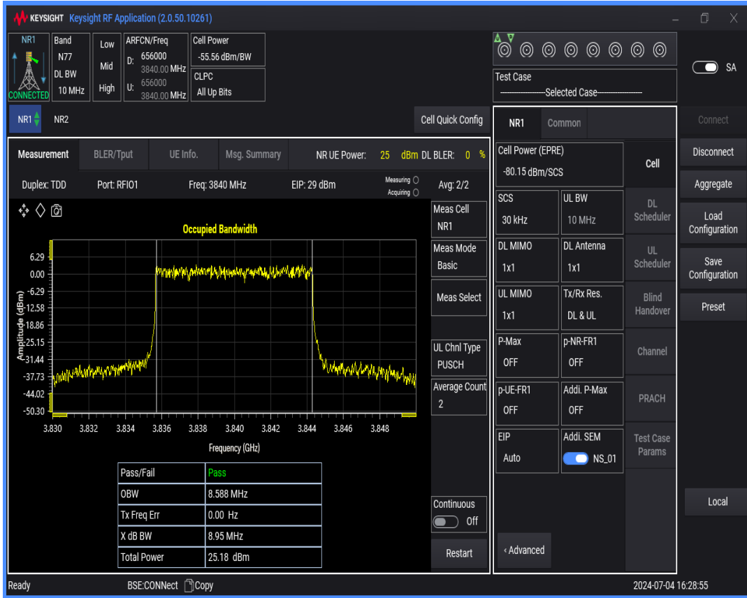
n77(3700-3980) SCS=30kHz DFT_QPSK BW=15MHz Channel=656000 RB=36 @0
