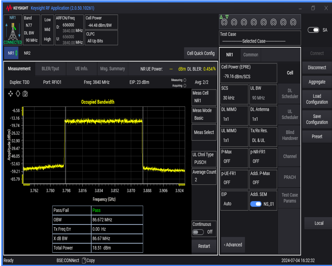
n77(3700-3980) SCS=30kHz DFT_QAM64 BW=100MHz Channel=656000 RB=270@0
