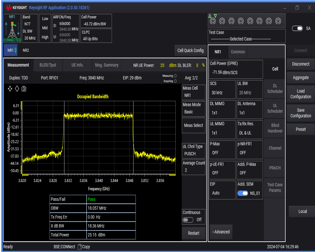
n77(3700-3980) SCS=30kHz DFT_QPSK BW=30MHz Channel=656000 RB=75 @0
