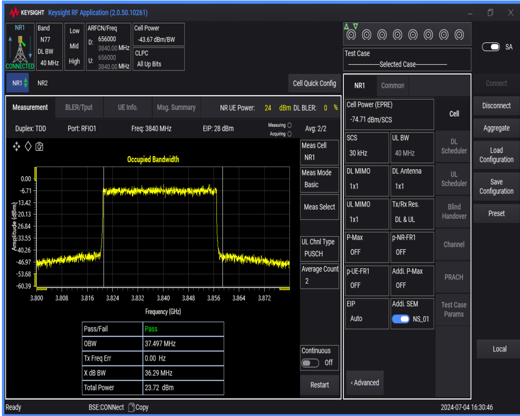
n77(3700-3980) SCS=30kHz DFT_QAM64 BW=50MHz Channel=656000 RB=128@0
