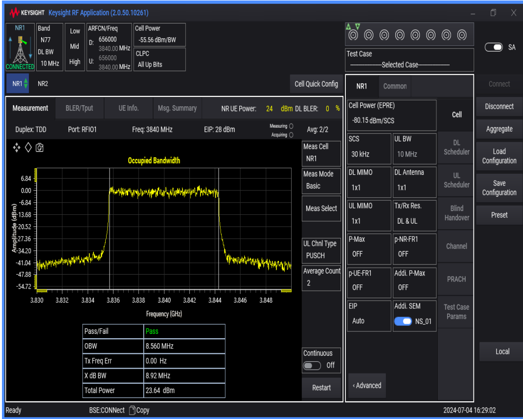
n77(3700-3980) SCS=30kHz DFT_QAM64 BW=15MHz Channel=656000 RB=36@0
