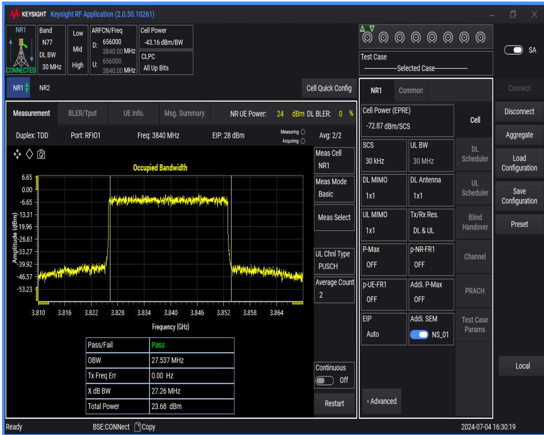
n77(3700-3980) SCS=30kHz DFT_QAM64 BW=40MHz Channel=656000 RB=100@0
