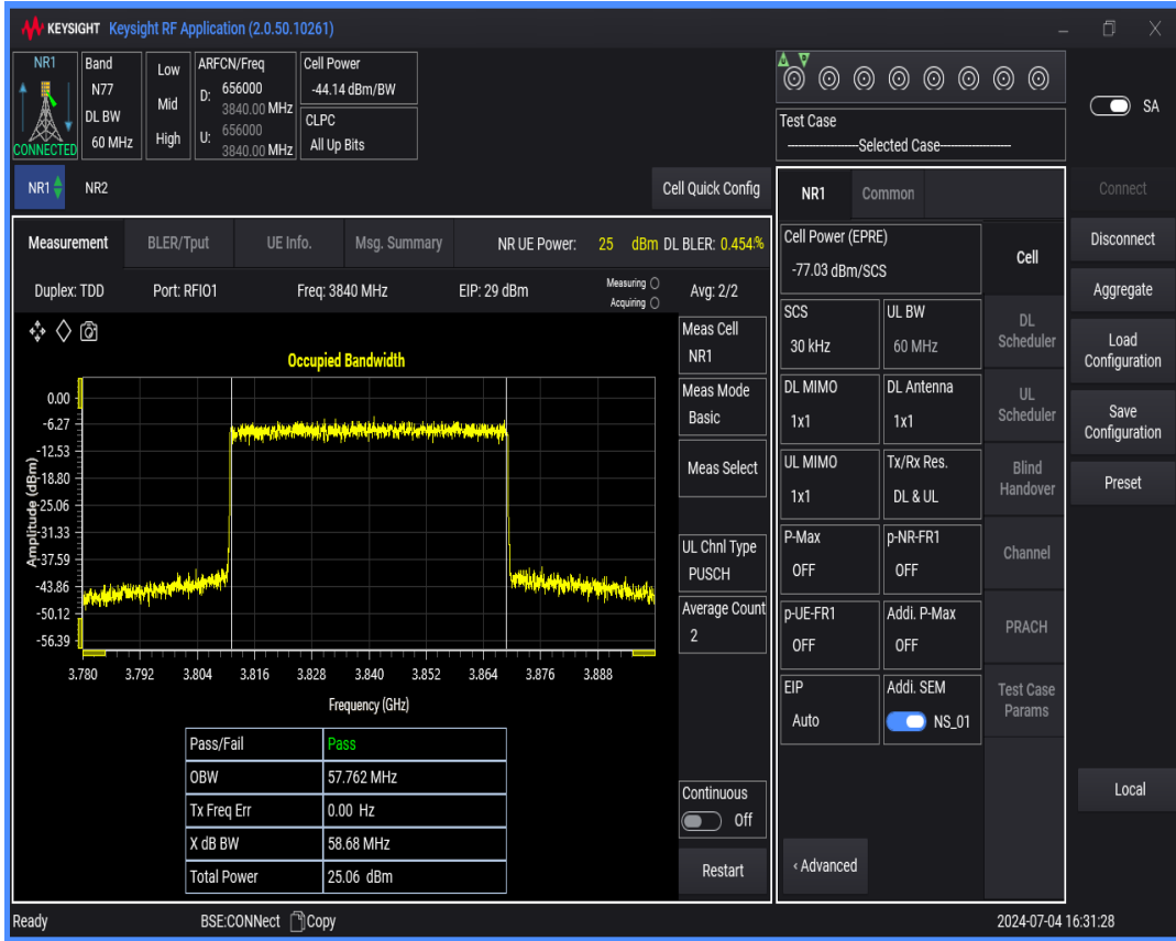
n77(3700-3980) SCS=30kHz DFT_QPSK BW=80MHz Channel=656000 RB=216@0
