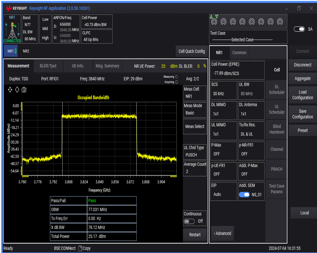
n77(3700-3980) SCS=30kHz DFT_QPSK BW=90MHz Channel=656000 RB=240@0
