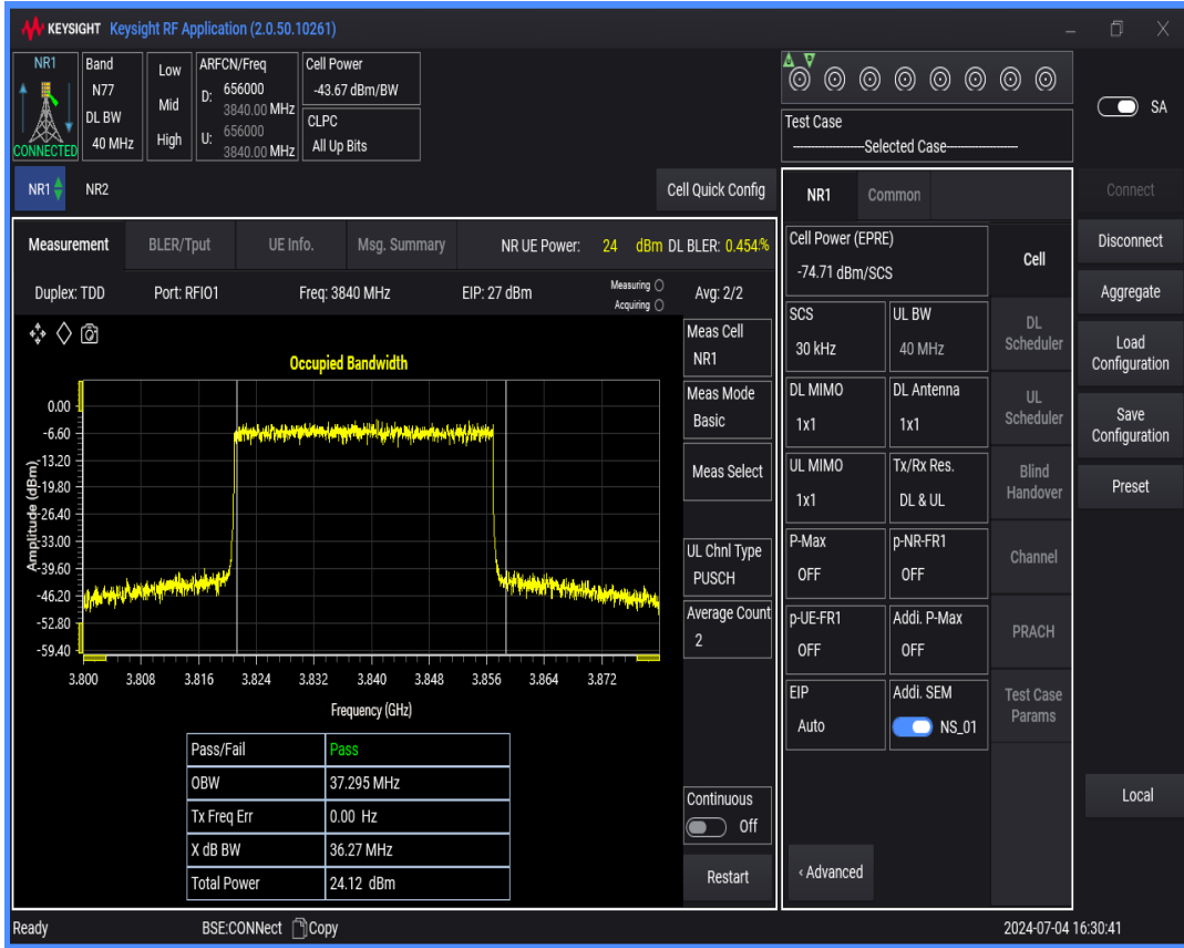
n77(3700-3980) SCS=30kHz DFT_QAM16 BW=50MHz Channel=656000 RB=128@0
