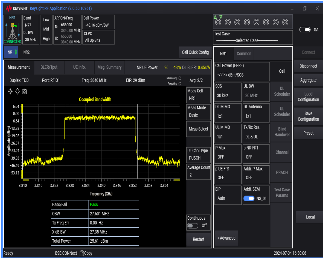
n77(3700-3980) SCS=30kHz DFT_BPSK BW=40MHz Channel=656000 RB=100 @0
