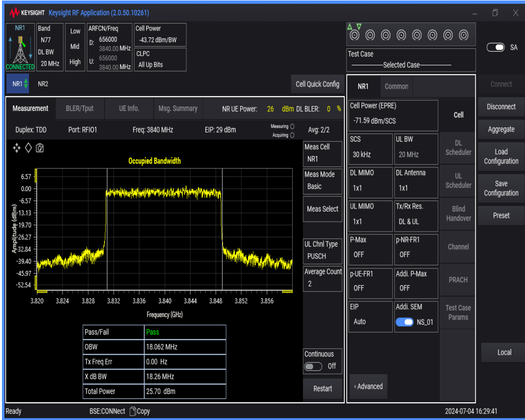
n77(3700-3980) SCS=30kHz DFT_BPSK BW=30MHz Channel=656000 RB=75 @0
