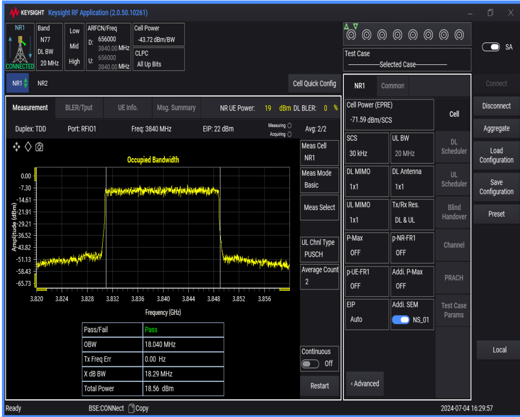
n77(3700-3980) SCS=30kHz DFT_QAM256 BW=30MHz Channel=656000 RB=75 @0
