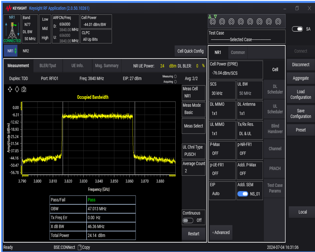
n77(3700-3980) SCS=30kHz DFT_QAM16 BW=60MHz Channel=656000 RB=162@0
