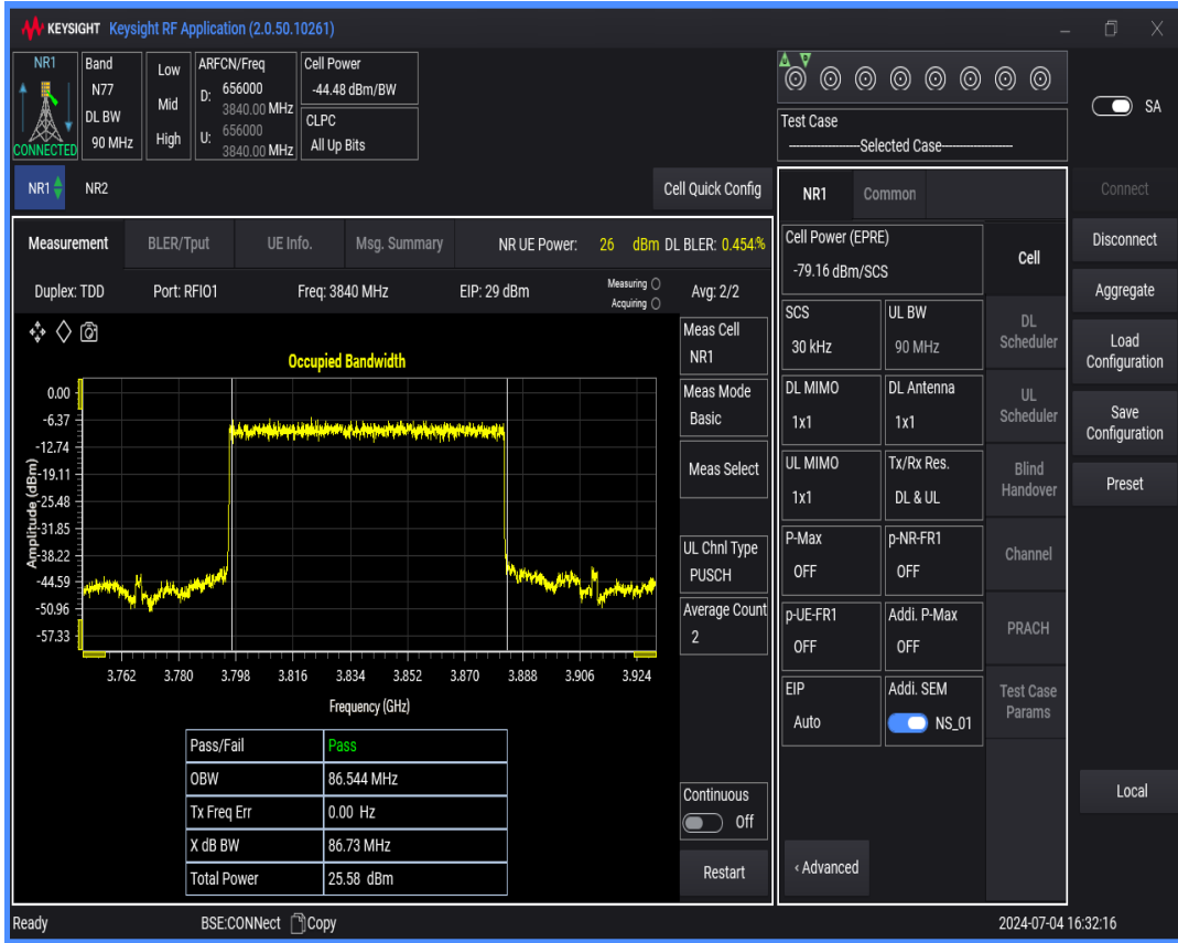
n77(3700-3980) SCS=30kHz DFT_QAM16 BW=100MHz Channel=656000 RB=270@0
