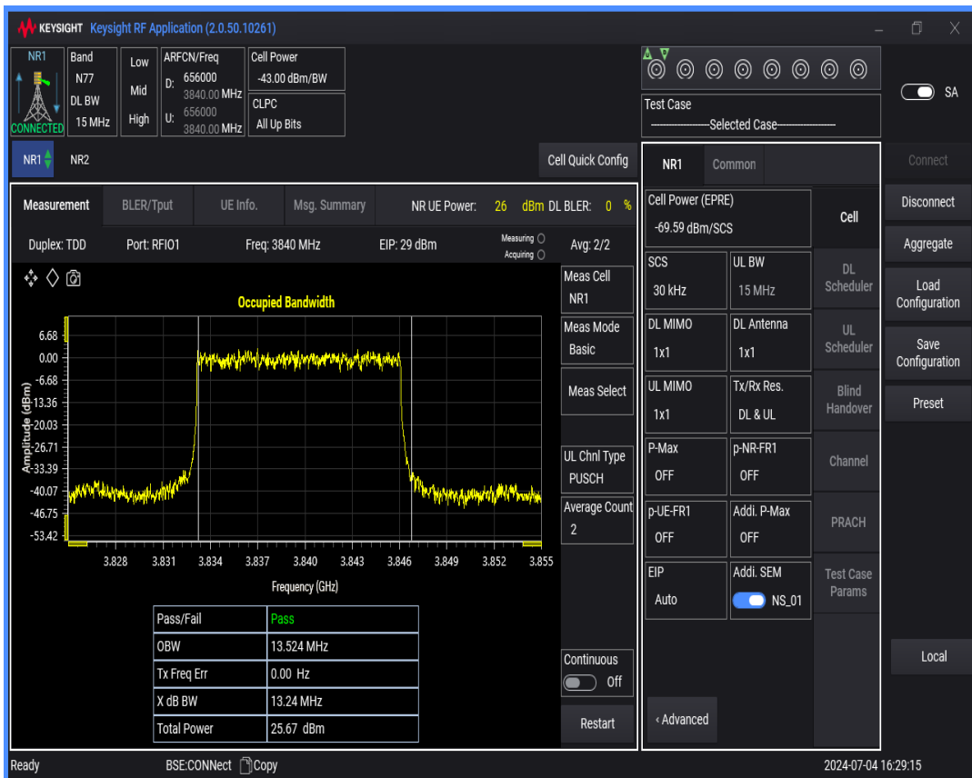
n77(3700-3980) SCS=30kHz DFT_BPSK BW=20MHz Channel=656000 RB=50 @0
