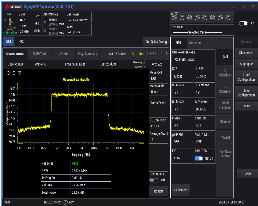
n77(3700-3980) SCS=30kHz DFT_QAM256 BW=40MHz Channel=656000 RB=100 @0
