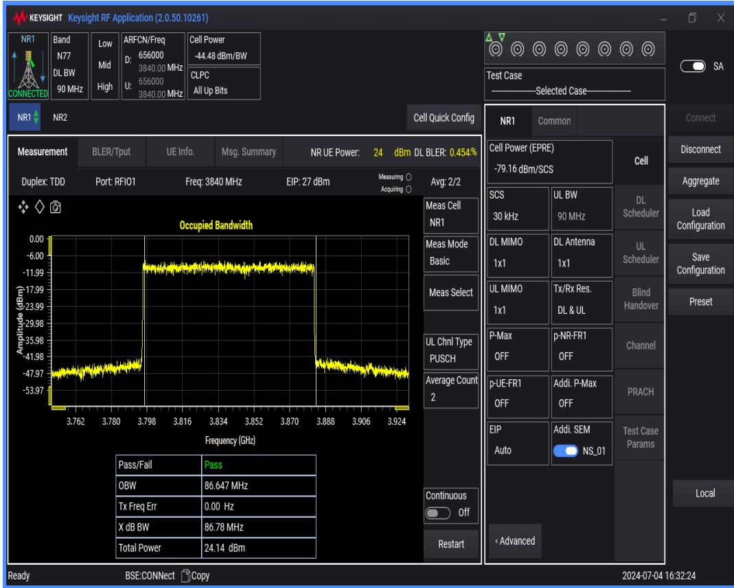
n77(3700-3980) SCS=30kHz DFT_QAM256 BW=100MHz Channel=656000 RB=270@0
