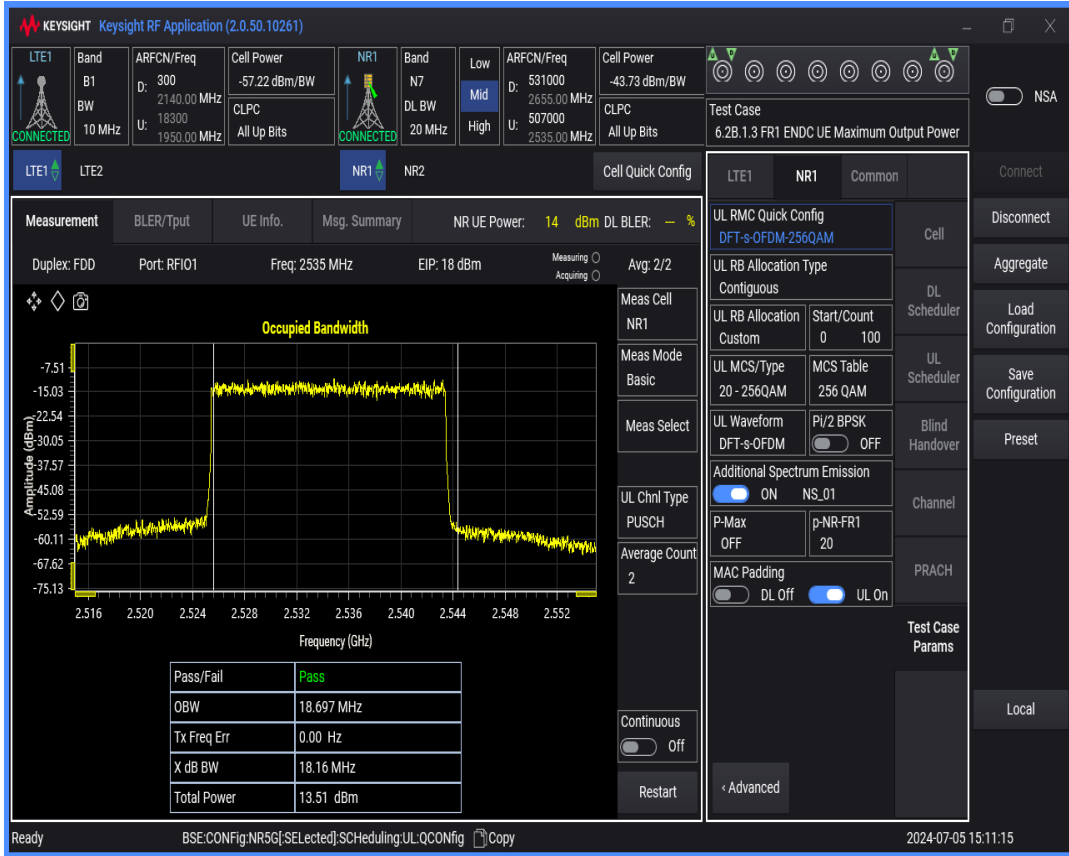
n7 SCS=15kHz DFT_QAM256 BW=5MHz Channel=507000 RB=25@0
