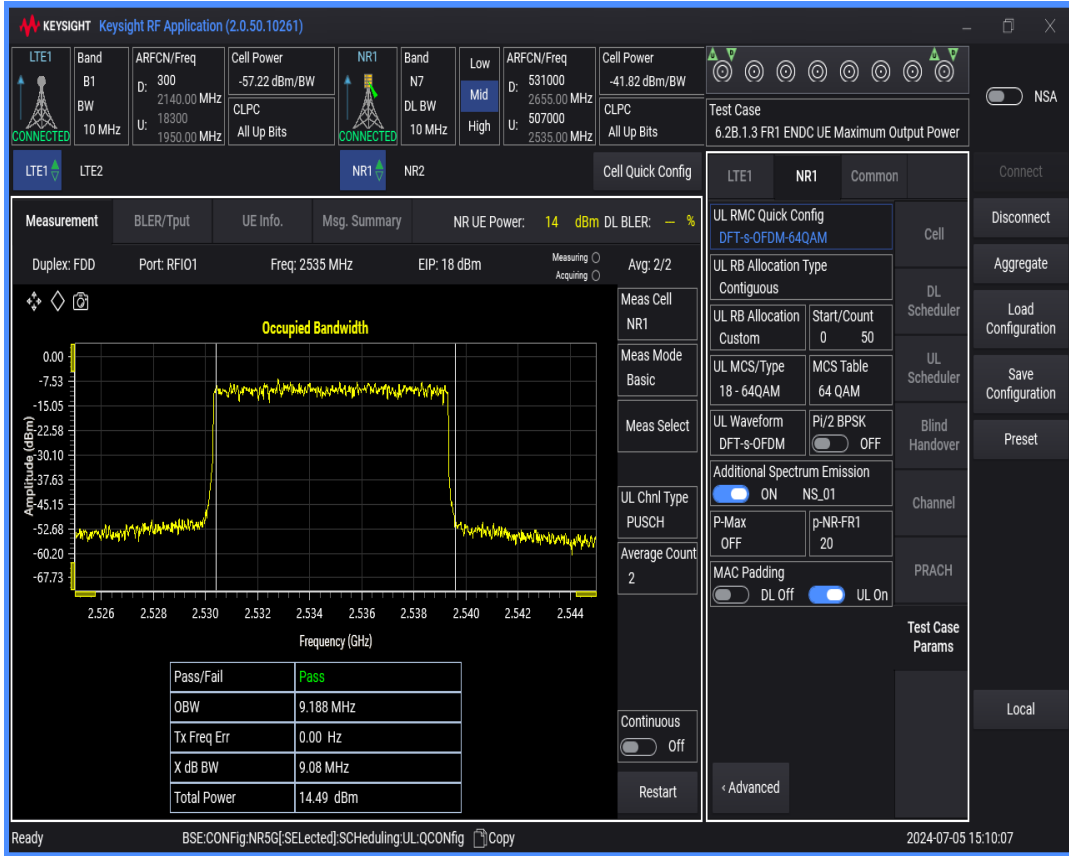
n7 SCS=15kHz DFT_QAM64 BW=15MHz Channel=507000 RB=75@0
