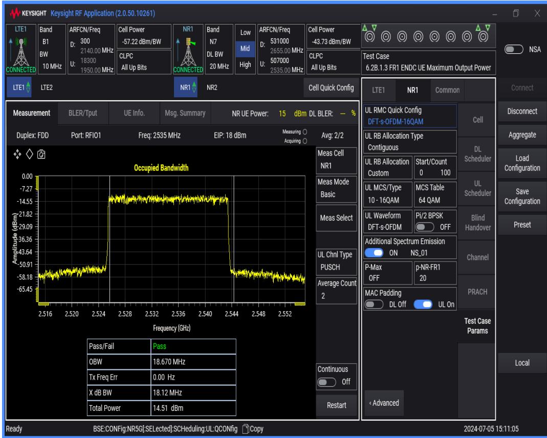
n7 SCS=15kHz DFT_QAM16 BW=5MHz Channel=507000 RB=25 @0
