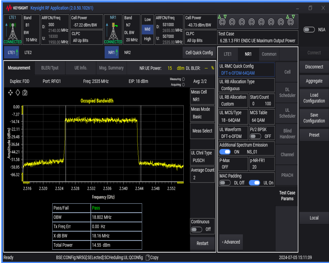
n7 SCS=15kHz DFT_QAM64 BW=5MHz Channel=507000 RB=25 @0
