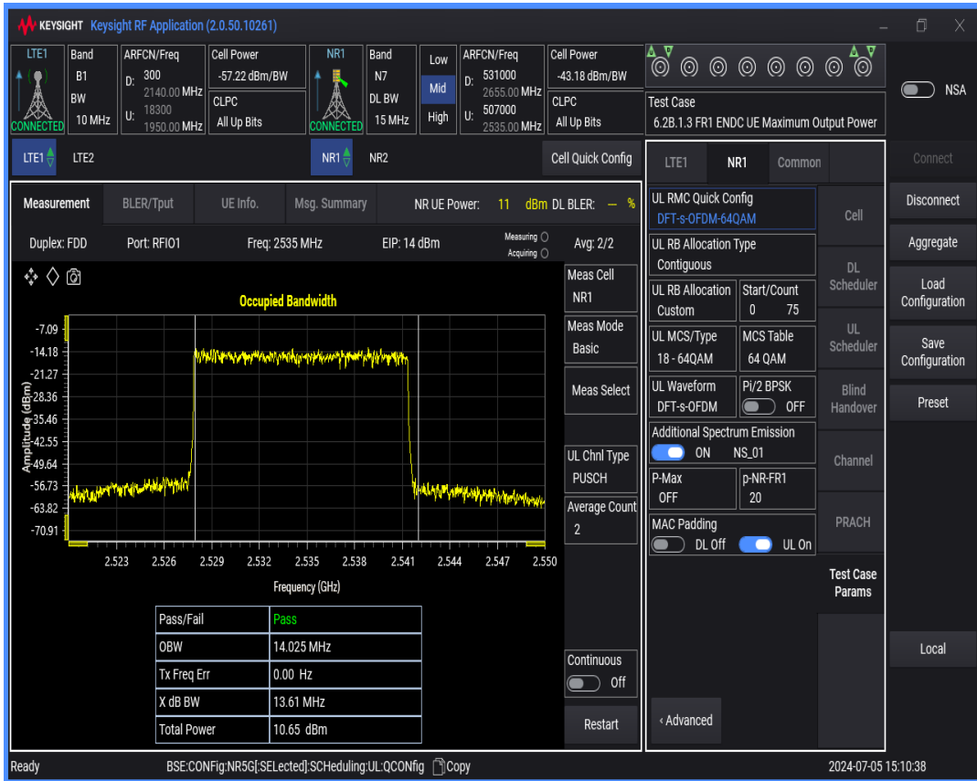
n7 SCS=15kHz DFT_QAM64 BW=20MHz Channel=507000 RB=100@0
