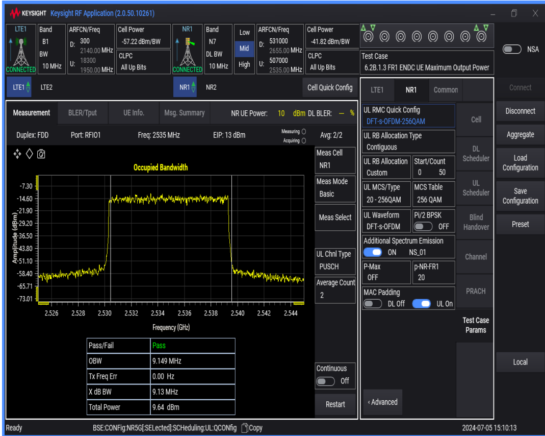
n7 SCS=15kHz DFT_QAM256 BW=15MHz Channel=507000 RB=75@0
