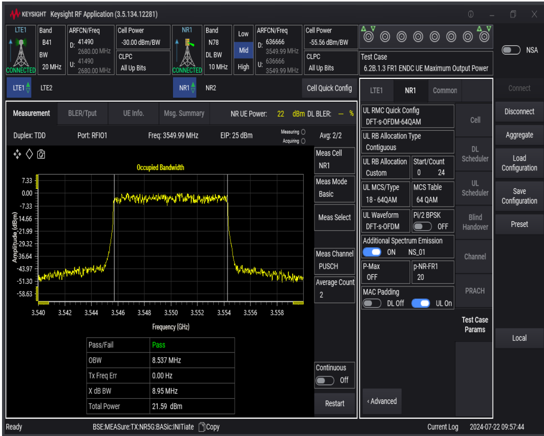
n78 SCS=30kHz DFT_QAM64 BW=15MHz Channel=636666 RB=36@0
