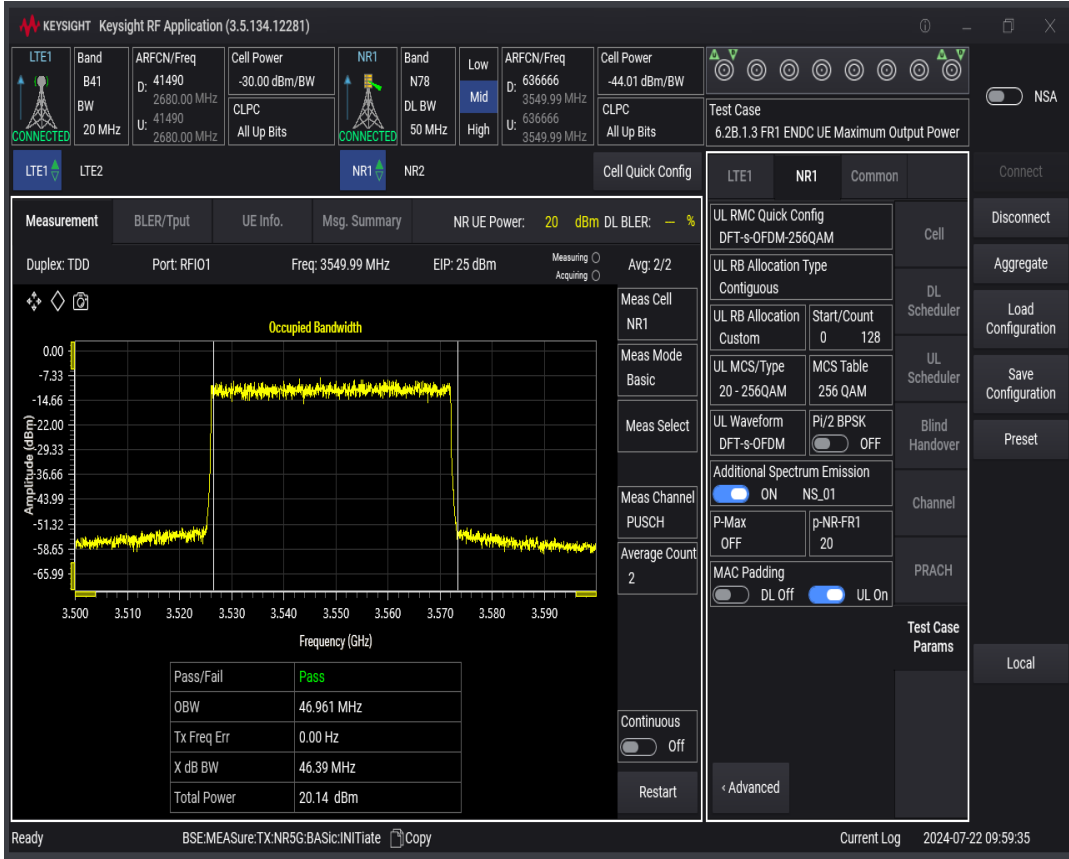
n78 SCS=30kHz DFT_QAM256 BW=60MHz Channel=636666 RB=162 @0
