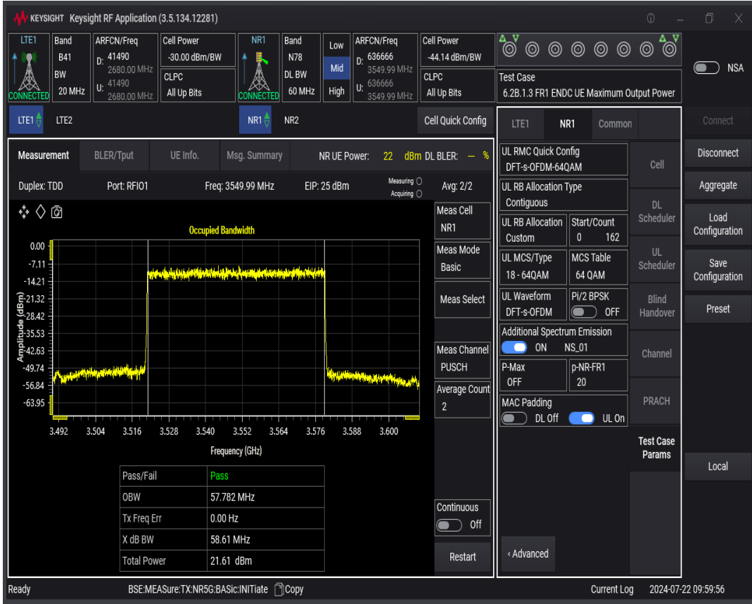
n78 SCS=30kHz DFT_QAM64 BW=80MHz Channel=636666 RB=216@0
