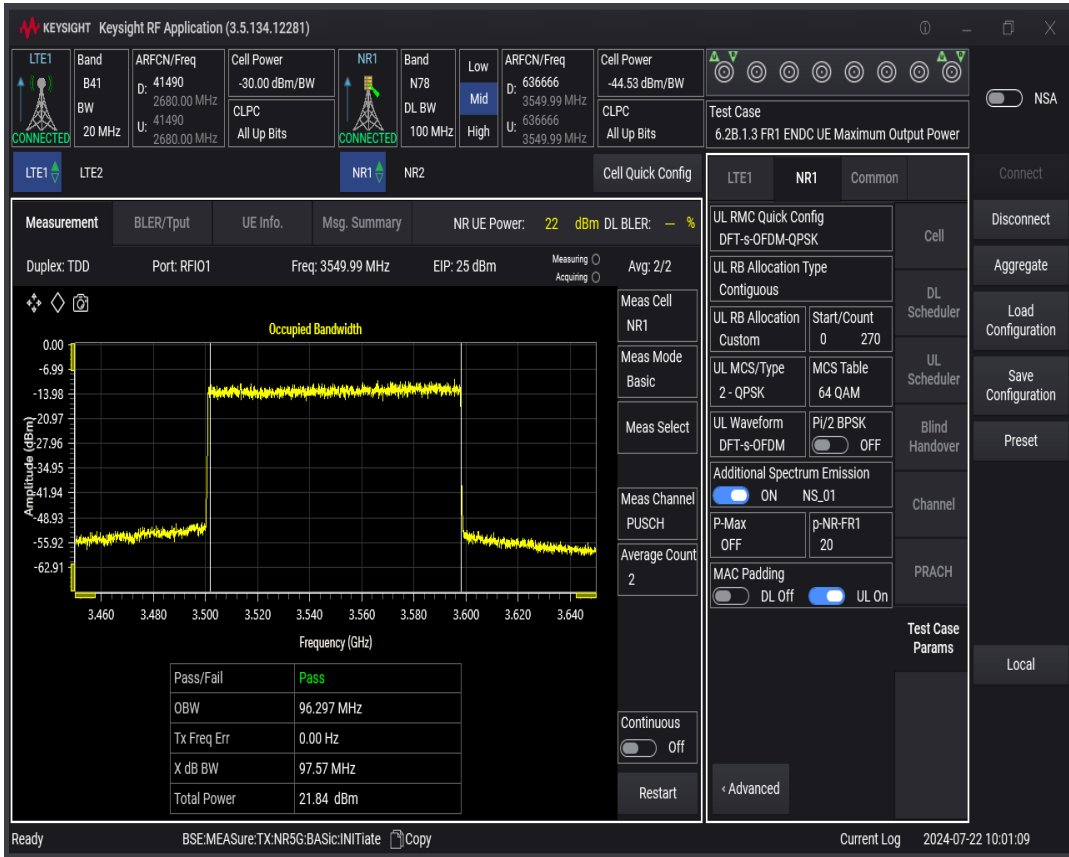
n78 SCS=30kHz DFT_QPSK BW=10MHz Channel=636666 RB=24 @0
