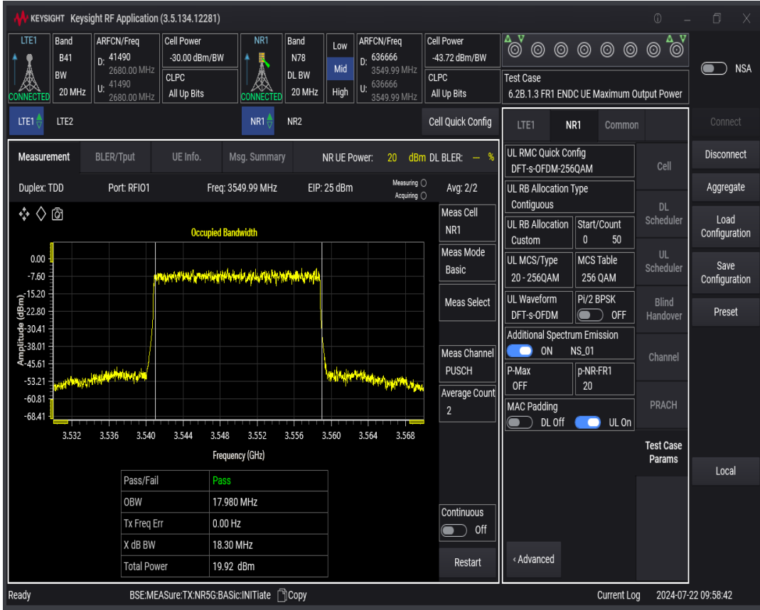
n78 SCS=30kHz DFT_QAM256 BW=40MHz Channel=636666 RB=100@0
