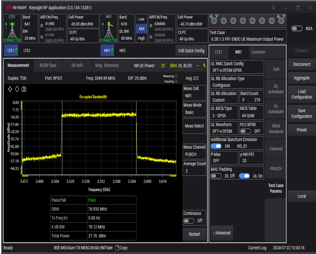
n78 SCS=30kHz DFT_QPSK BW=90MHz Channel=636666 RB=240@0
