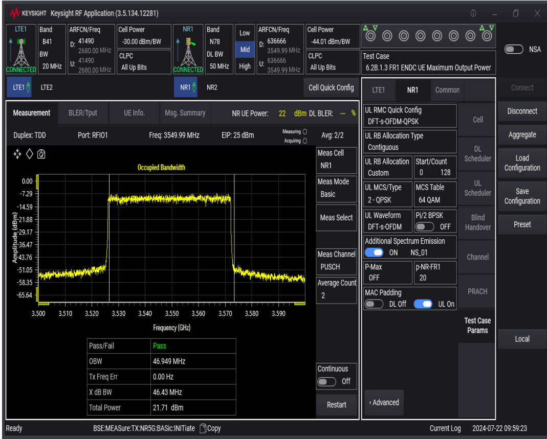
n78 SCS=30kHz DFT_QPSK BW=60MHz Channel=636666 RB=162@0
