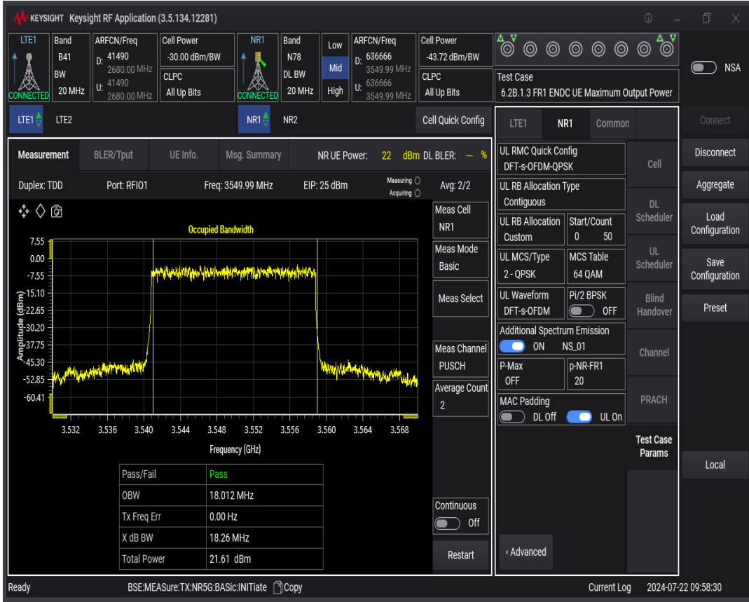
n78 SCS=30kHz DFT_QPSK BW=40MHz Channel=636666 RB=100@0
