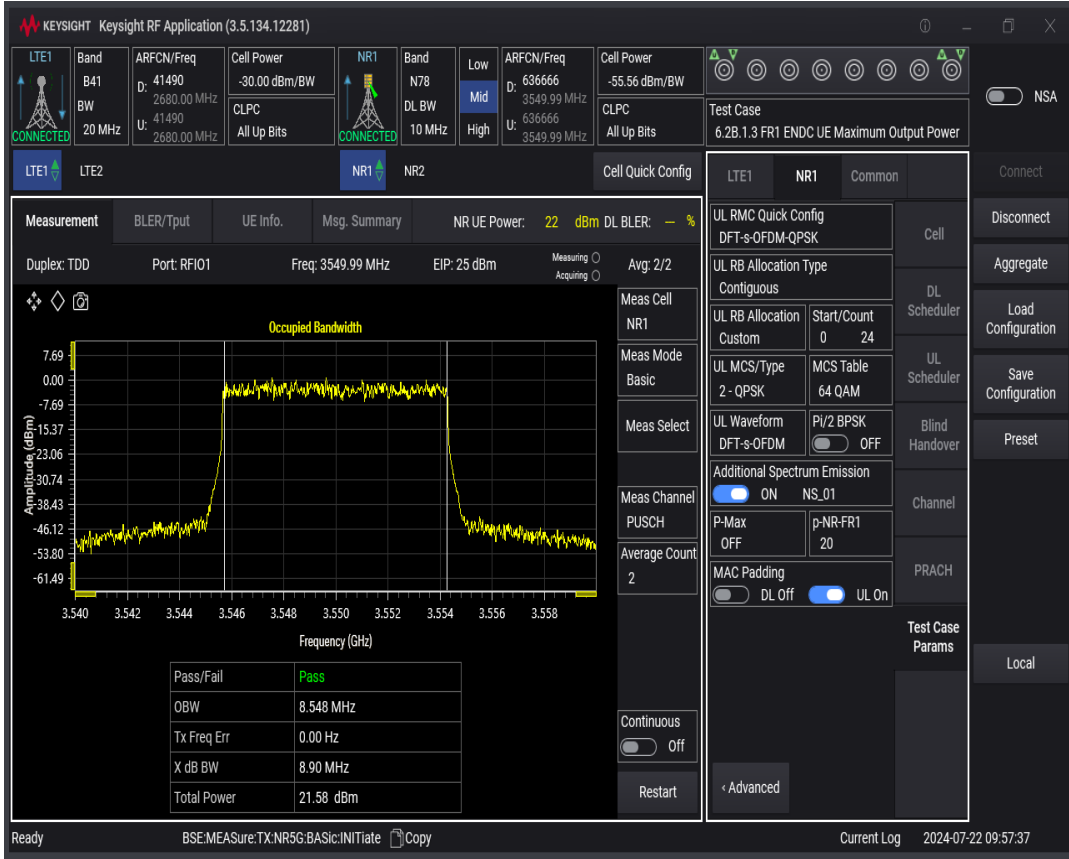
n78 SCS=30kHz DFT_QPSK BW=15MHz Channel=636666 RB=36@0
