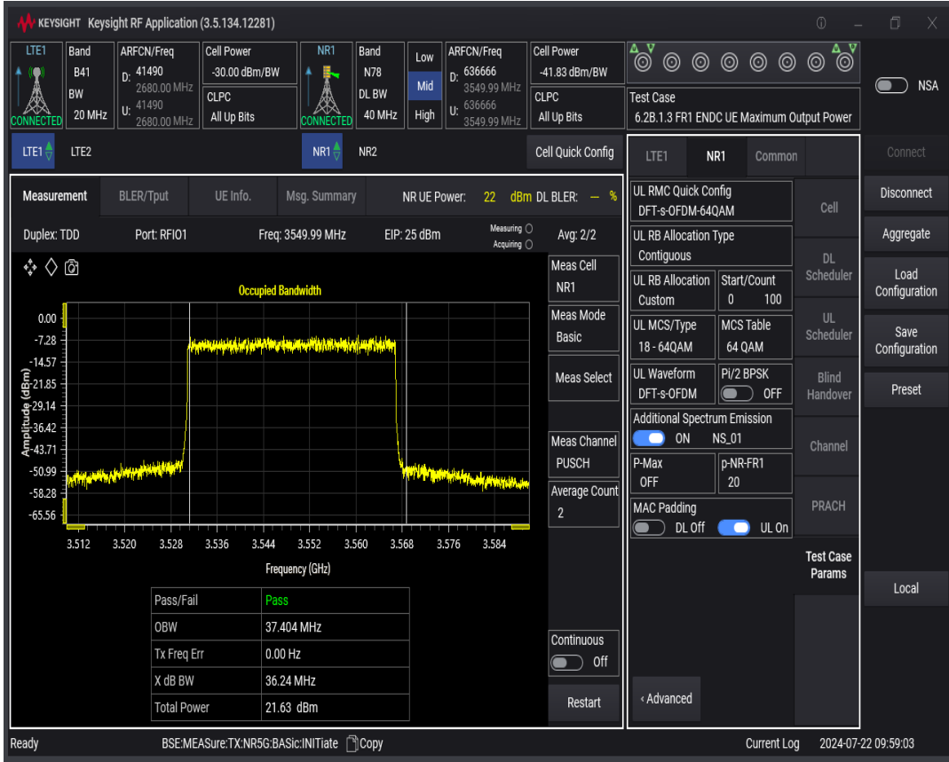
n78 SCS=30kHz DFT_QAM64 BW=50MHz Channel=636666 RB=128 @0
