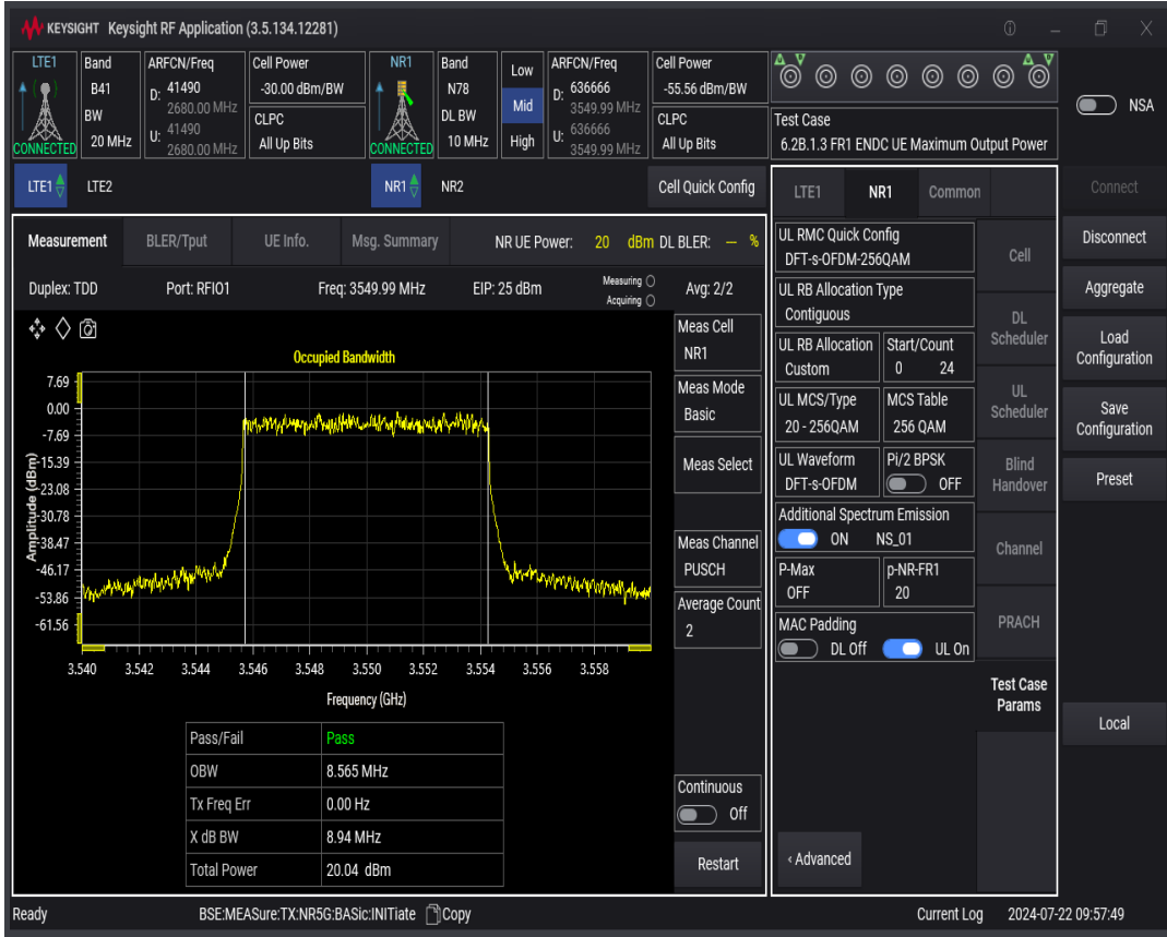
n78 SCS=30kHz DFT_QAM256 BW=15MHz Channel=636666 RB=36@0
