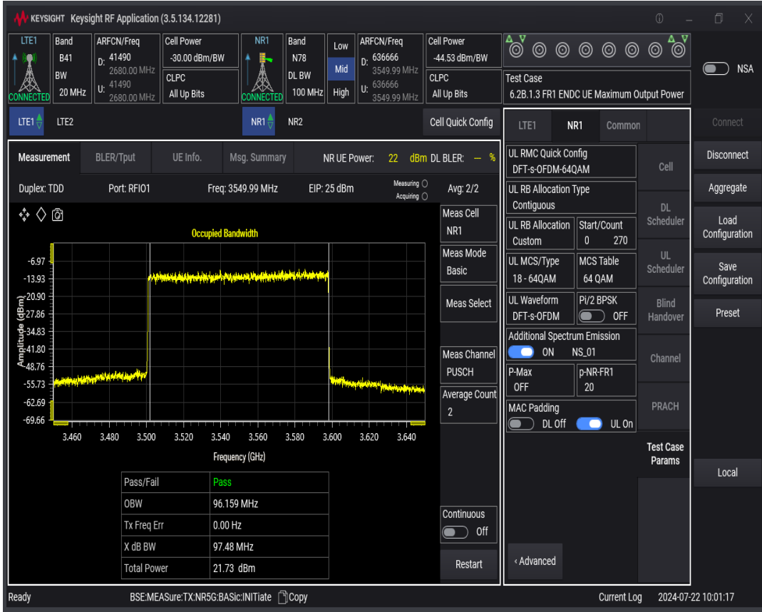
n78 SCS=30kHz DFT_QAM64 BW=10MHz Channel=636666 RB=24@0
