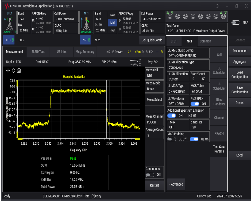
n78 SCS=30kHz DFT_BPSK BW=40MHz Channel=636666 RB=100@0
