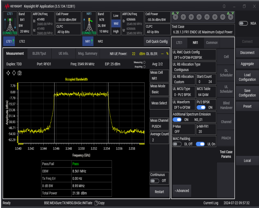
n78 SCS=30kHz DFT_BPSK BW=15MHz Channel=636666 RB=36@0
