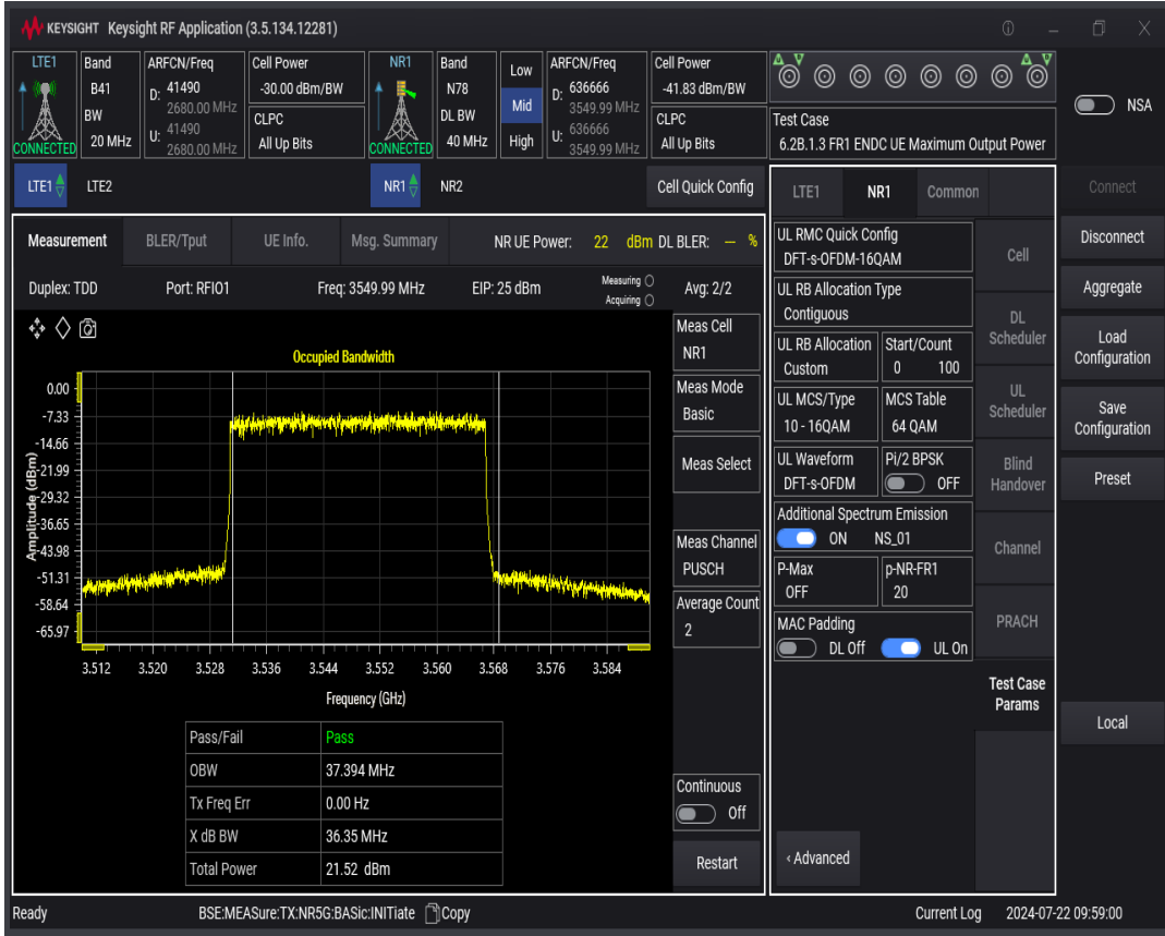
n78 SCS=30kHz DFT_QAM16 BW=50MHz Channel=636666 RB=128 @0
