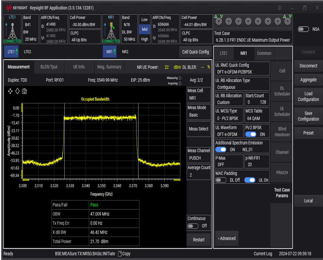
n78 SCS=30kHz DFT_BPSK BW=60MHz Channel=636666 RB=162@0
