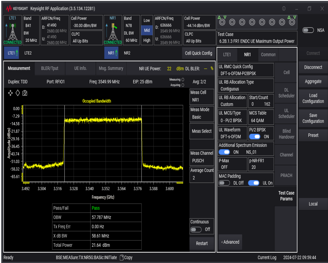
n78 SCS=30kHz DFT_BPSK BW=80MHz Channel=636666 RB=216@0
