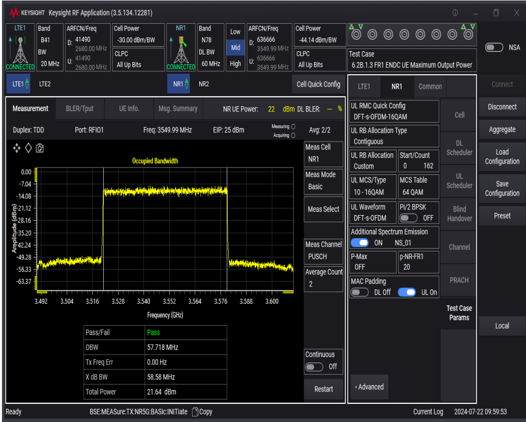
n78 SCS=30kHz DFT_QAM16 BW=80MHz Channel=636666 RB=216 @0
