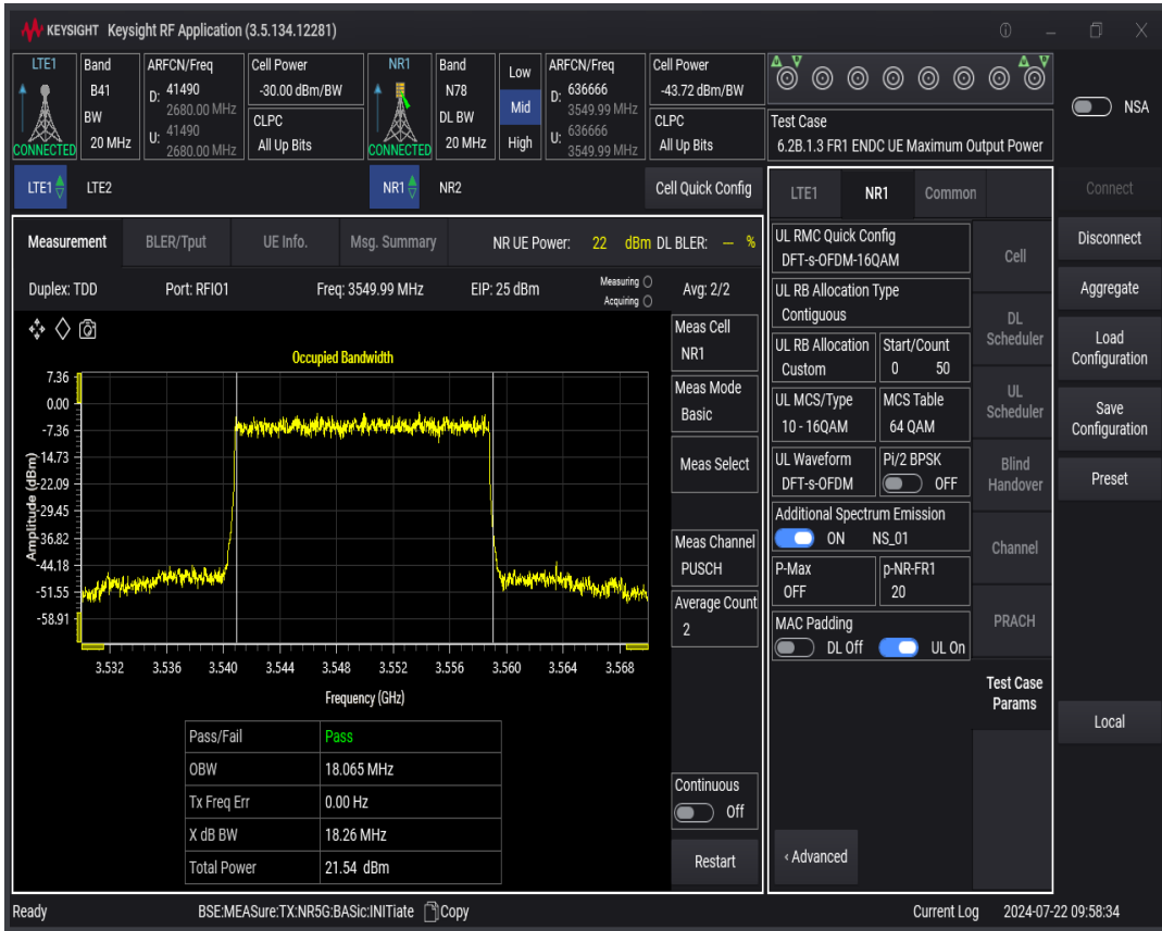
n78 SCS=30kHz DFT_QAM16 BW=40MHz Channel=636666 RB=100@0
