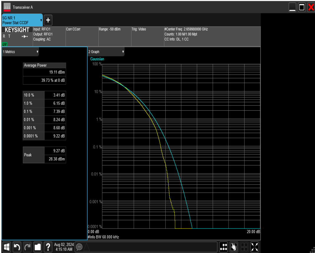
n41 SCS=30kHz DFT_QAM256 BW=80MHz Channel=507204 RB=216@0
