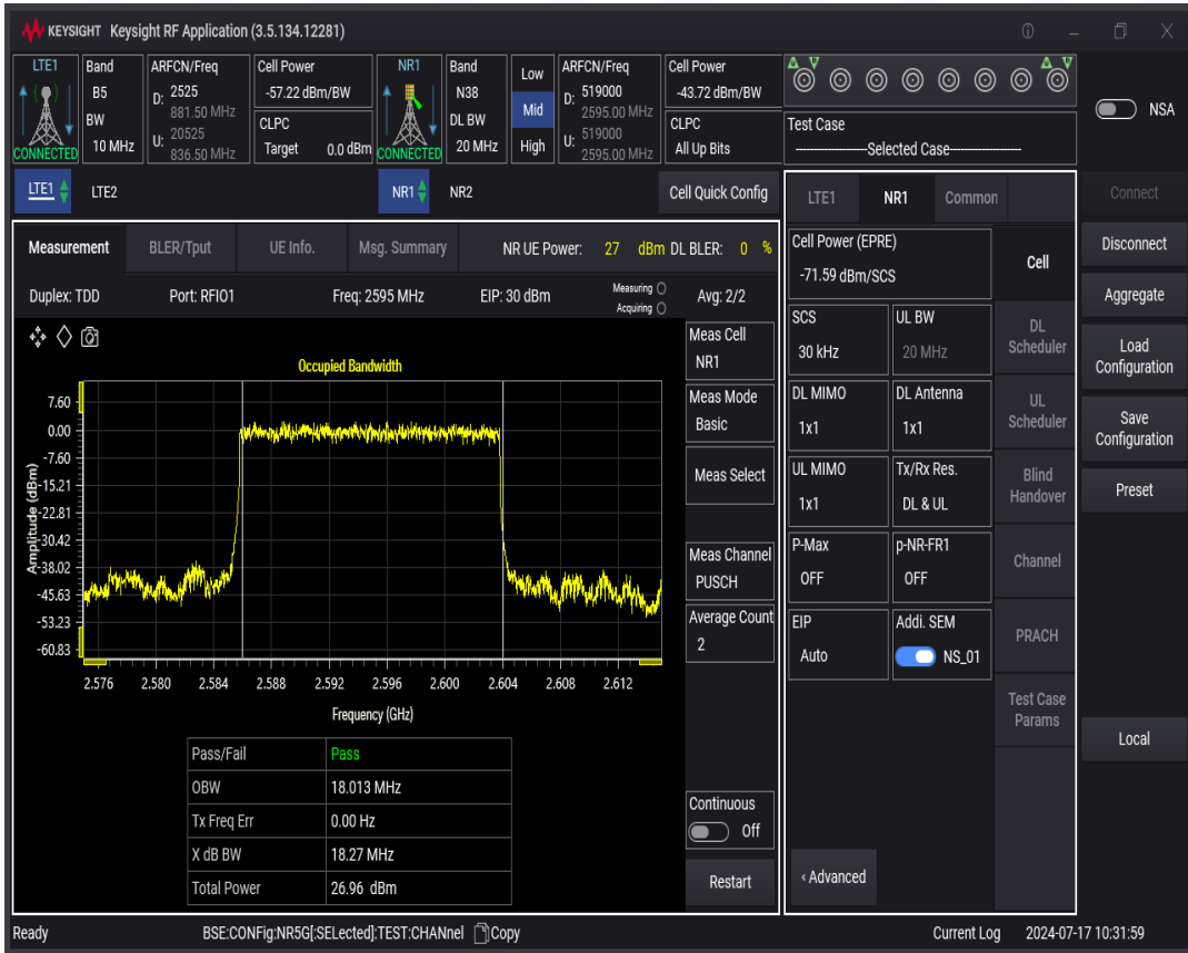
n38 SCS=30kHz DFT_QAM16 BW=10MHz Channel=519000 RB=24@0
