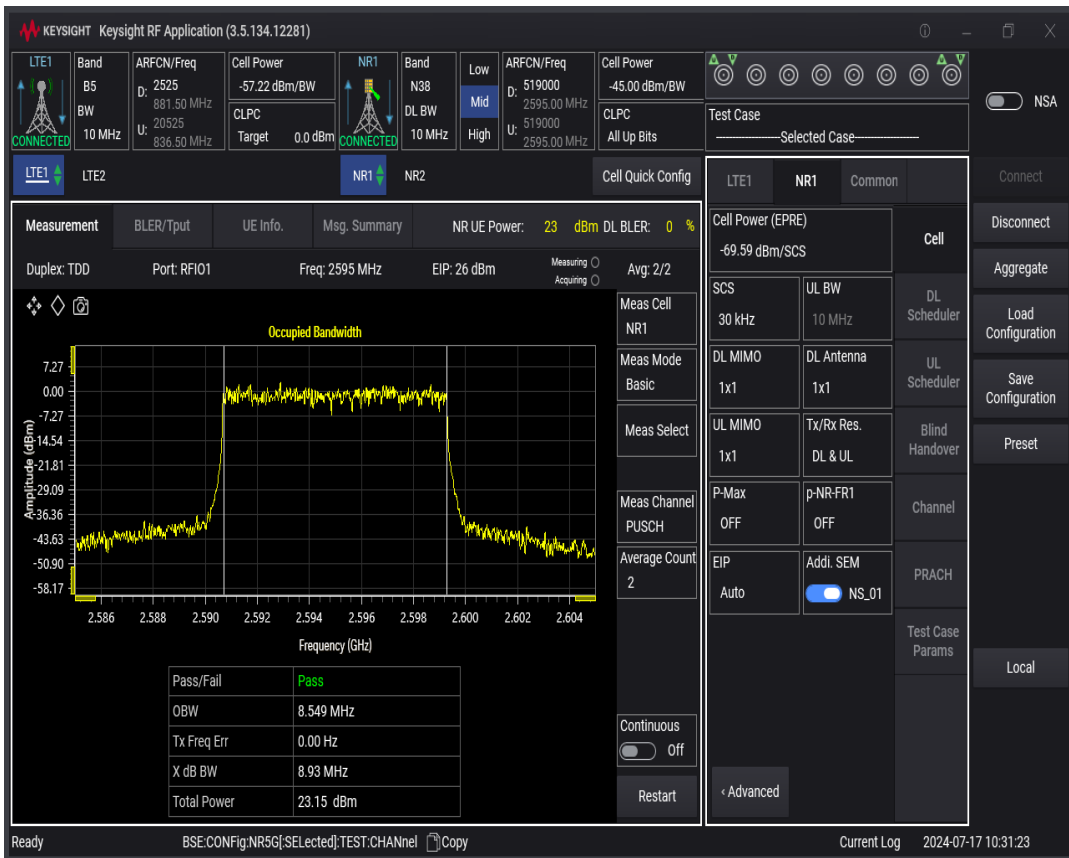
n38 SCS=30kHz DFT_QAM256 BW=15MHz Channel=519000 RB=36@0
