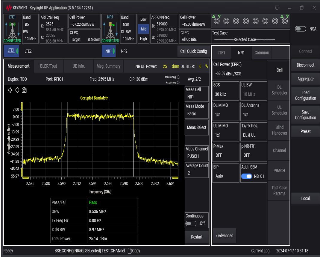
n38 SCS=30kHz DFT_QAM64 BW=15MHz Channel=519000 RB=36@0
