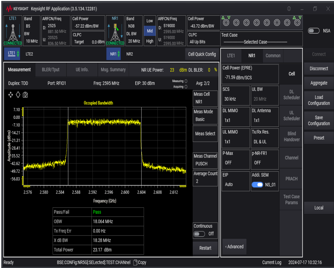
n38 SCS=30kHz DFT_QAM64 BW=10MHz Channel=519000 RB=24 @0
