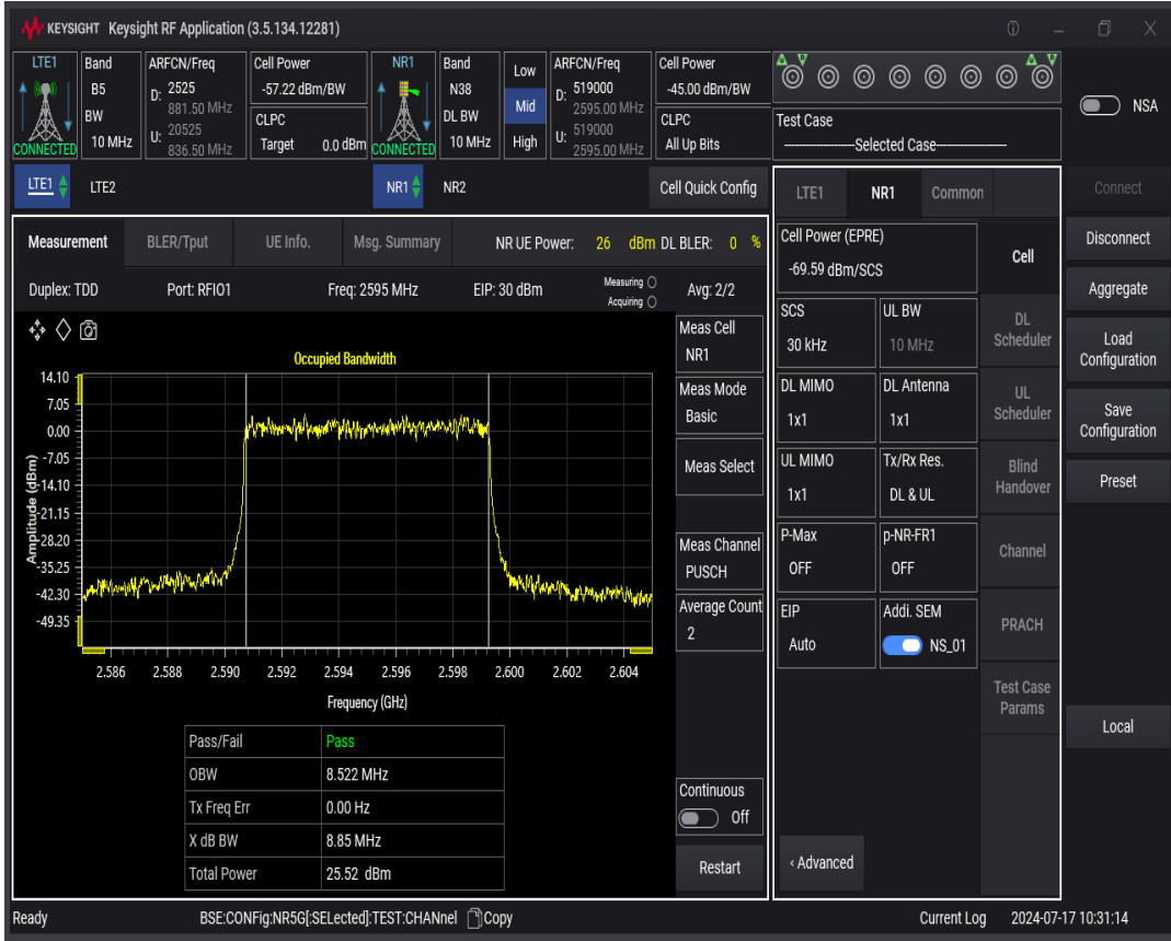
n38 SCS=30kHz DFT_QAM16 BW=15MHz Channel=519000 RB=36@0
