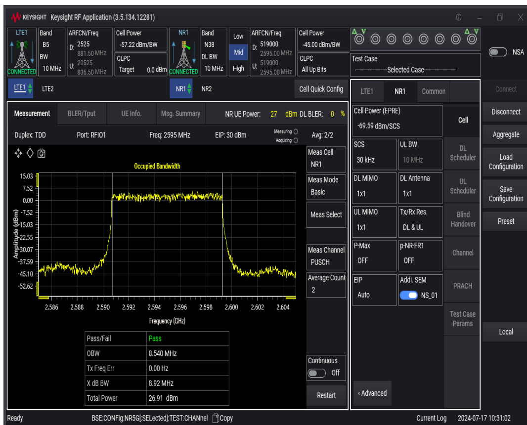
n38 SCS=30kHz DFT_BPSK BW=15MHz Channel=519000 RB=36@0
