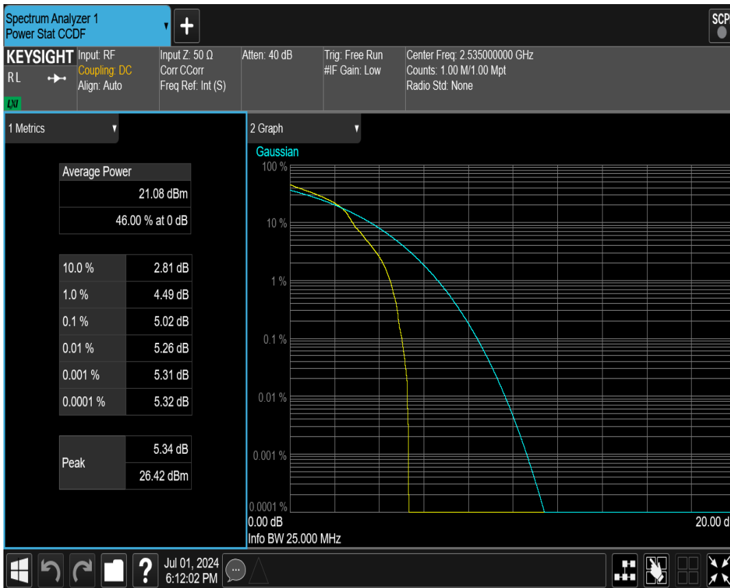
Band7 QPSK BW=10MHz Channel=21100 RB Size=1 Position=#0
