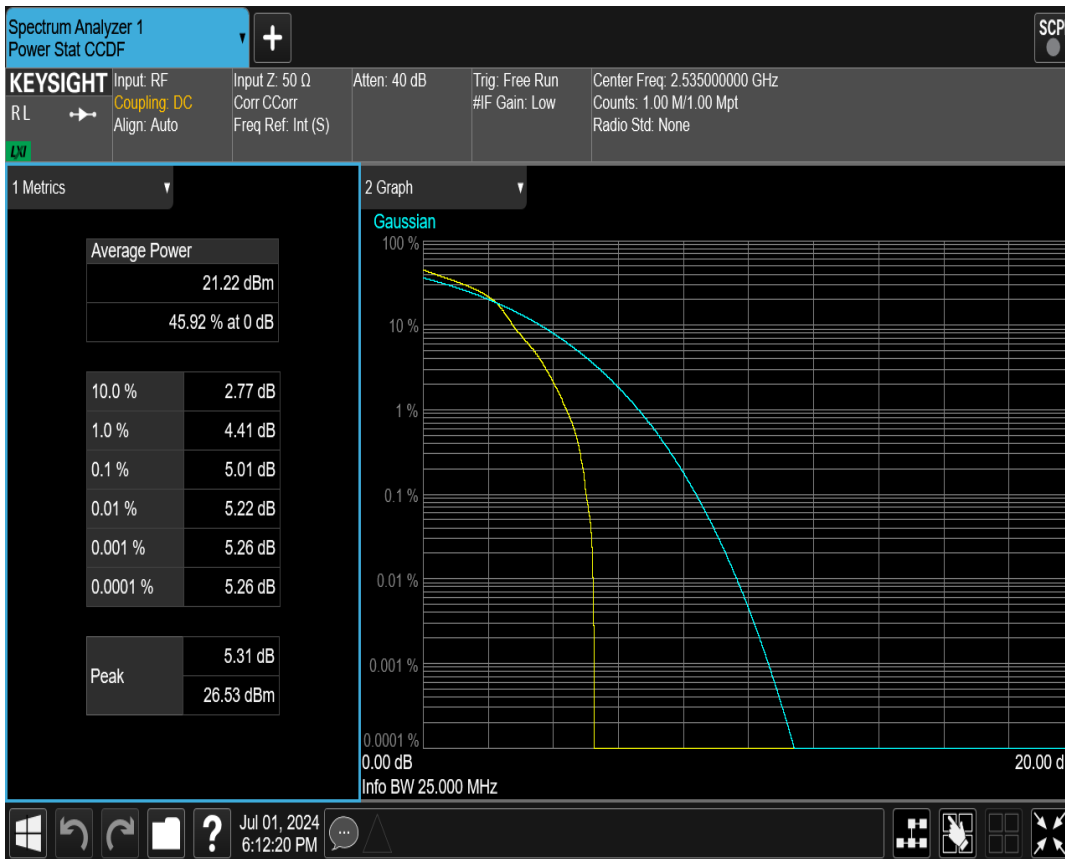
Band7 QAM16 BW=20MHz Channel=21100 RB Size=1 Position=#0
