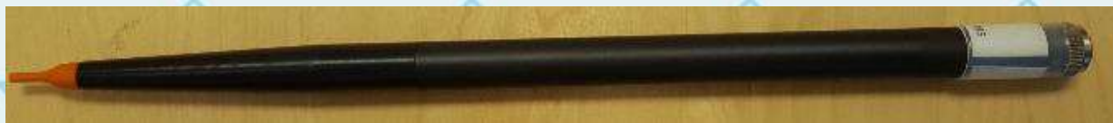
Figure 2 – MVG COMOSAR Dosimetric E field Dipole
