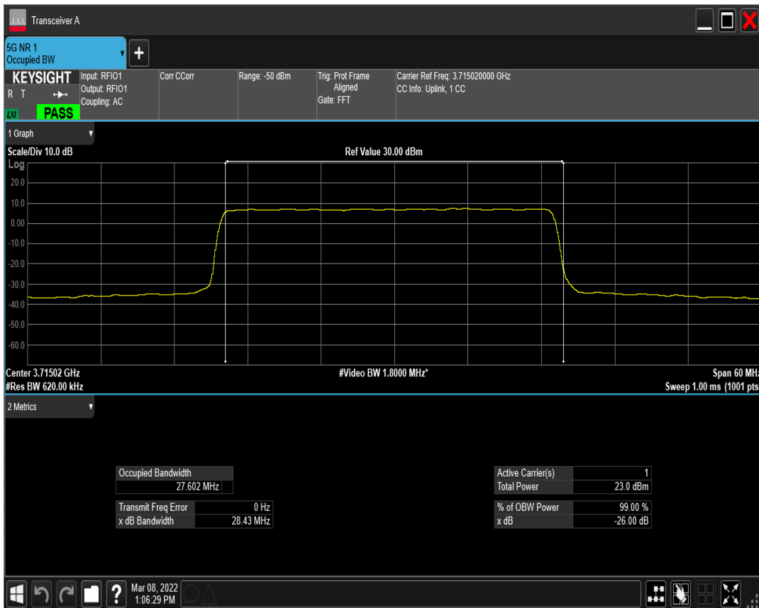
n77(3700-3980) SCS=30kHz DFT_QAM16 BW=30MHz Channel=647668 RB=75@0
