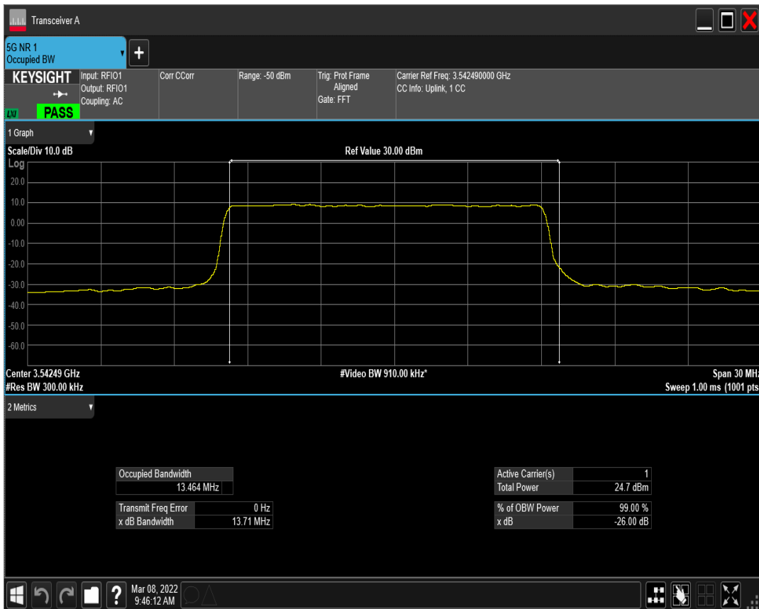
n77(3450-3550) SCS=30kHz DFT_QPSK BW=15MHz Channel=636166 RB=36@0
