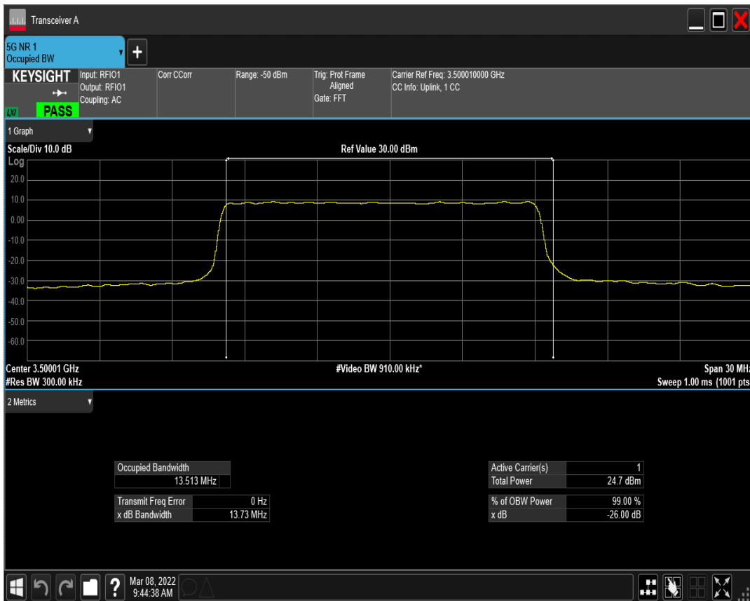
n77(3450-3550) SCS=30kHz DFT_QPSK BW=15MHz Channel=633334 RB=36@0
