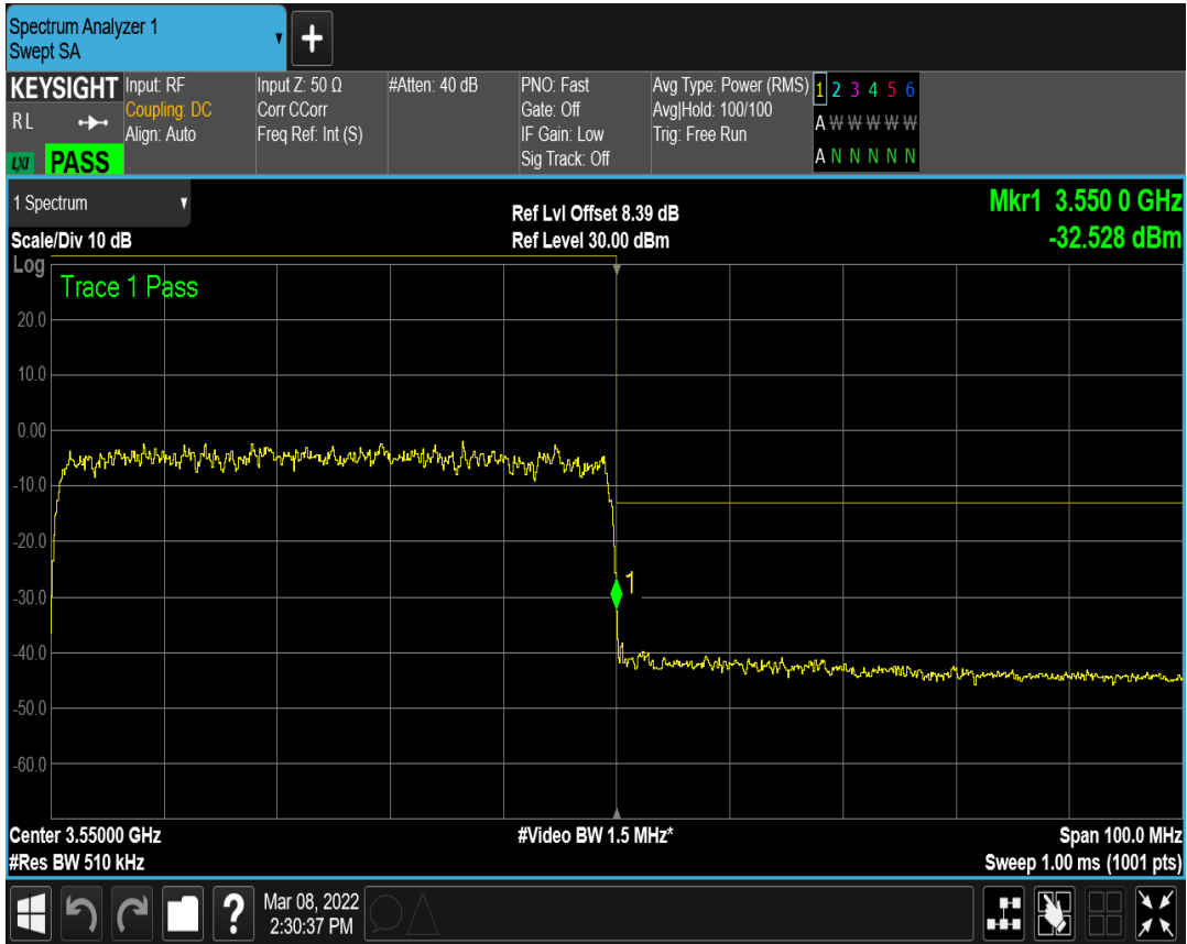
n77(3450-3550) SCS=15kHz DFT_QPSK BW=50MHz Channel=635000 RB=1@269
