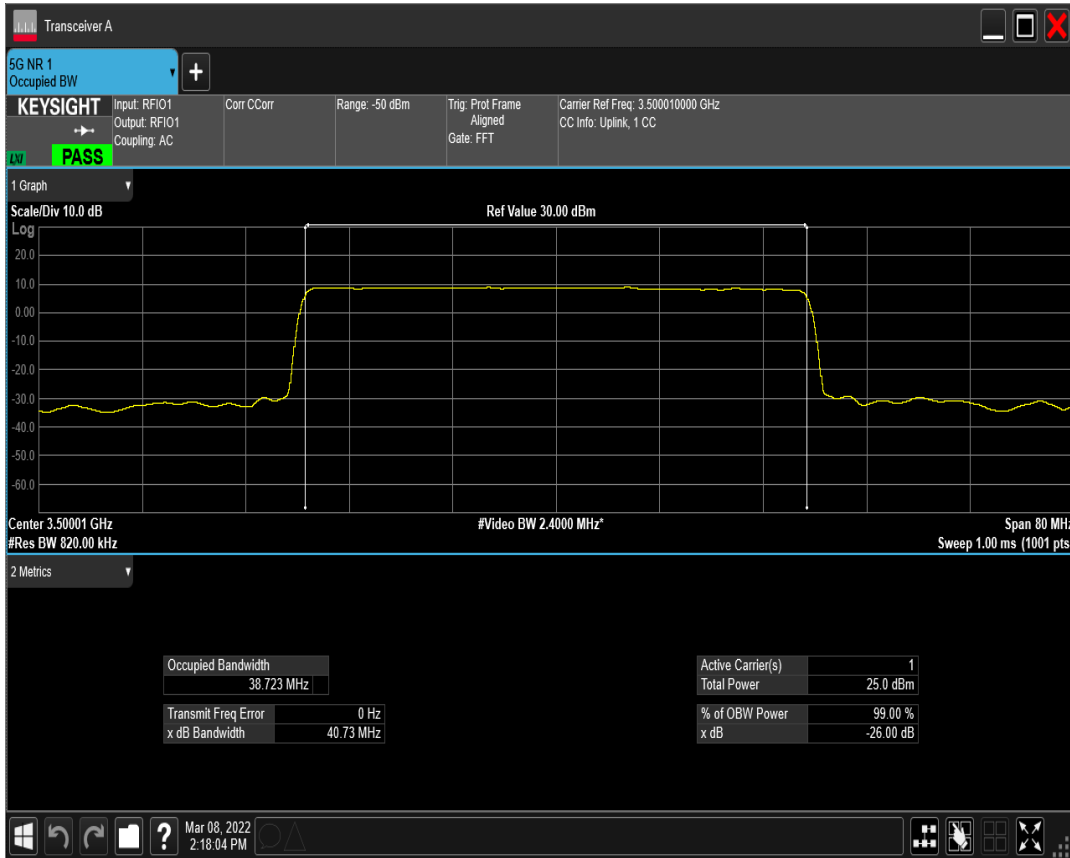
n77(3450-3550) SCS=15kHz DFT_QPSK BW=40MHz Channel=633334 RB=216@0
