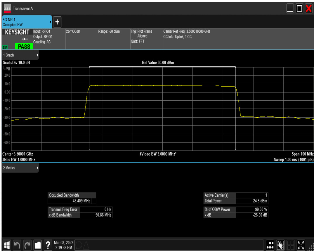
n77(3450-3550) SCS=15kHz DFT_QPSK BW=50MHz Channel=633334 RB=270@0
