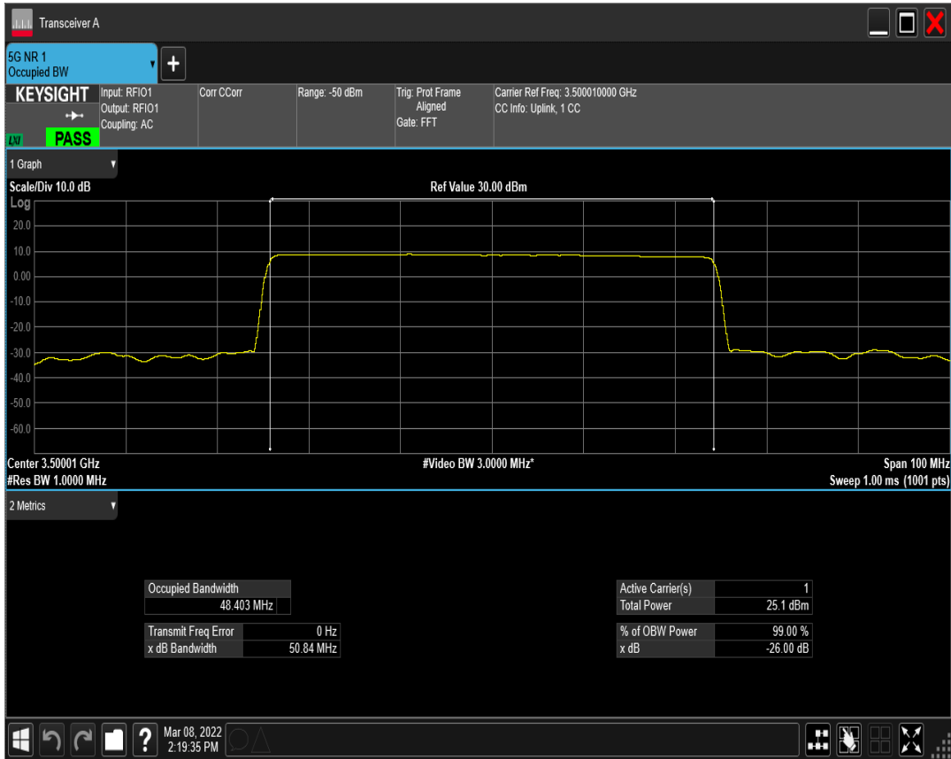
n77(3450-3550) SCS=15kHz DFT_QPSK BW=50MHz Channel=633334 RB=270@0
