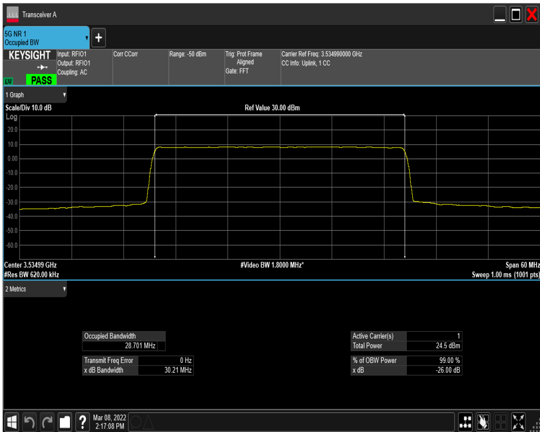
n77(3450-3550) SCS=15kHz DFT_QPSK BW=30MHz Channel=635666 RB=160@0
