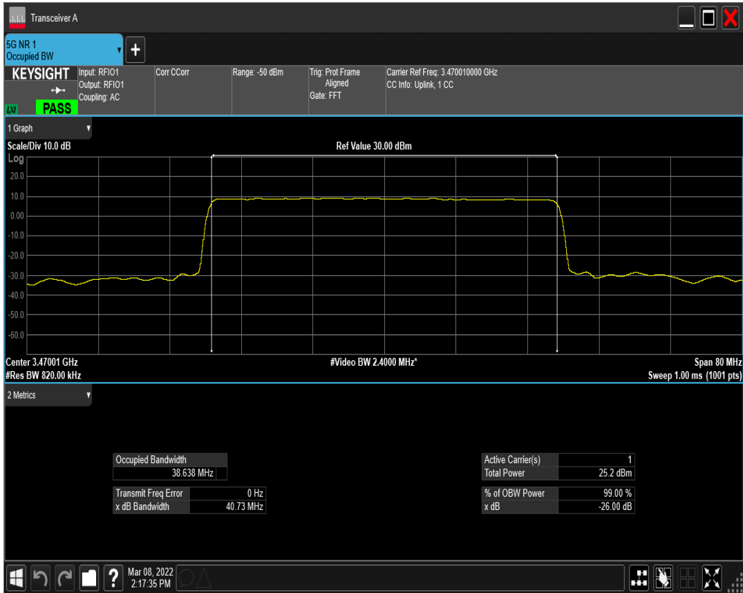
n77(3450-3550) SCS=15kHz DFT_QPSK BW=40MHz Channel=631334 RB=216@0
