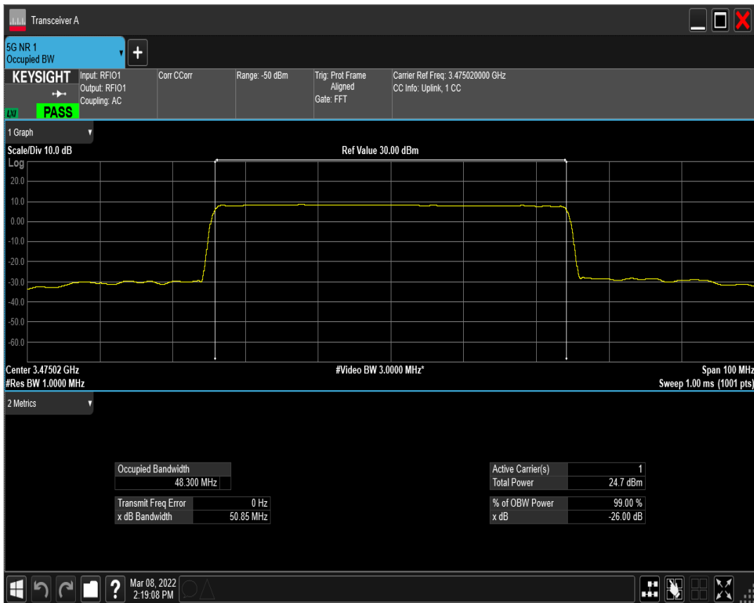
n77(3450-3550) SCS=15kHz DFT_QPSK BW=50MHz Channel=631668 RB=270@0
