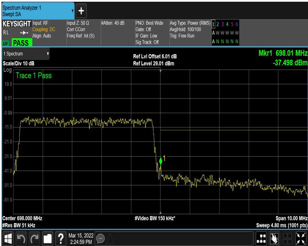
n71 SCS=15kHz DFT_QPSK BW=5MHz Channel=139100 RB=25@0
