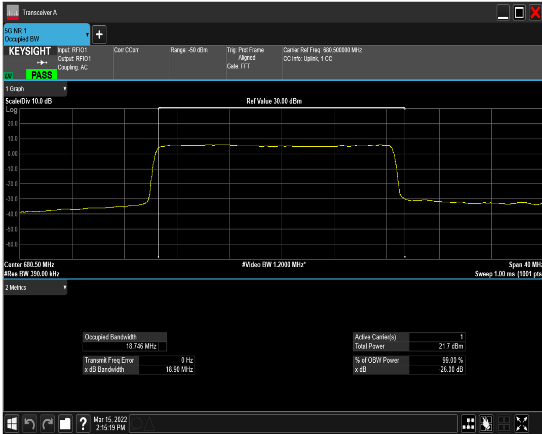
n71 SCS=15kHz DFT_QAM16 BW=20MHz Channel=136100 RB=100@0
