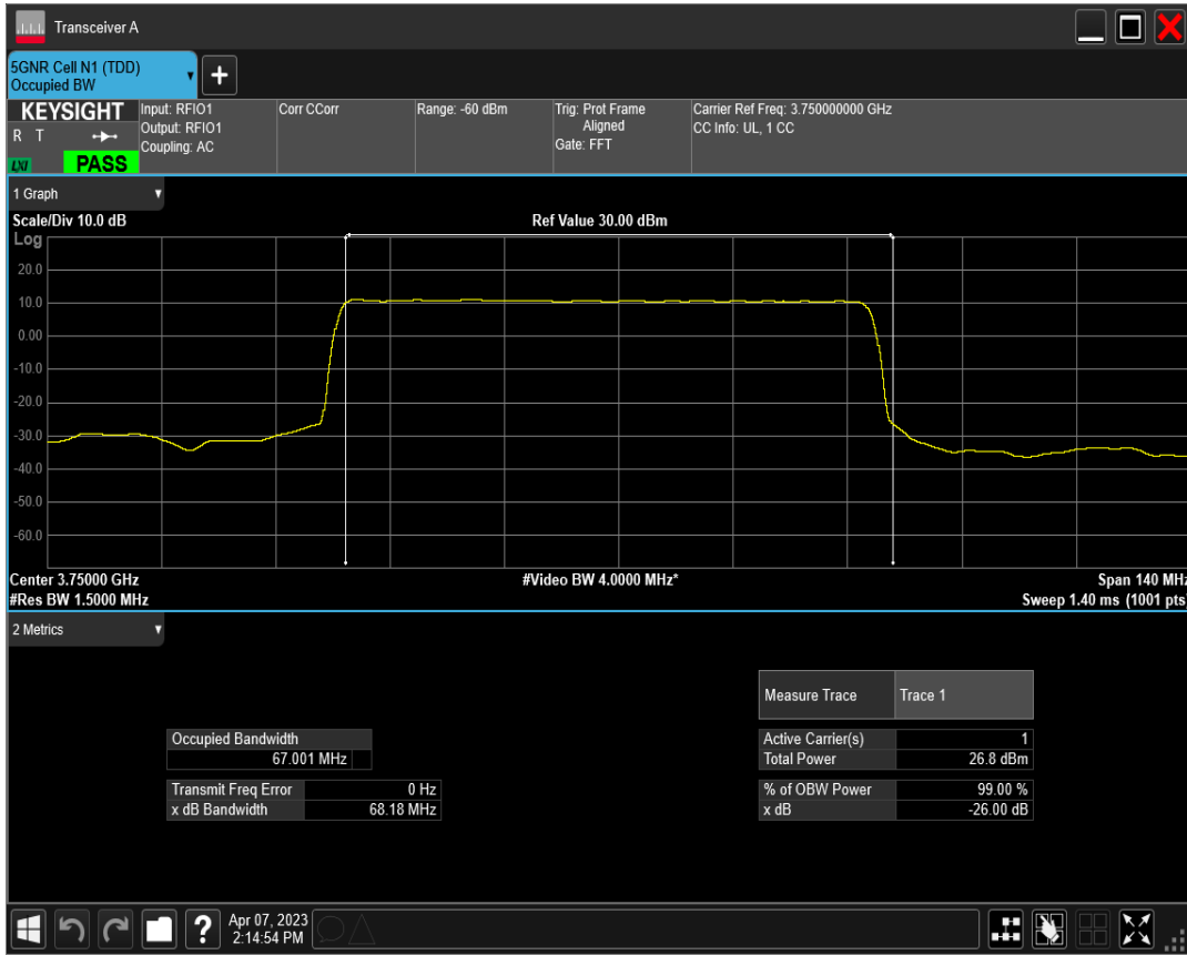
n78(3700-3800) SCS=30kHz DFT_QPSK BW=70MHz Channel=650000 RB=180@0
