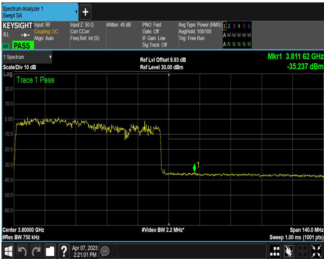
n78(3700-3800) SCS=30kHz DFT_QPSK BW=70MHz Channel=651000 RB=1@188
