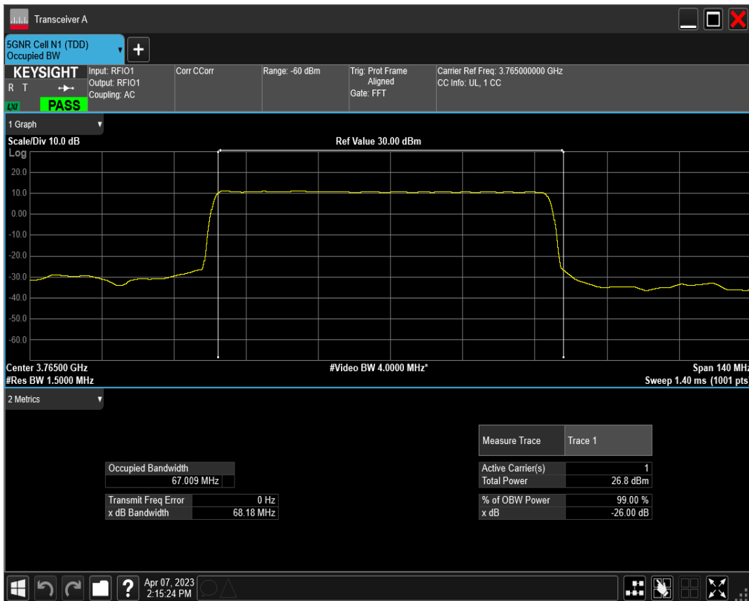
n78(3700-3800) SCS=30kHz DFT_QPSK BW=70MHz Channel=651000 RB=180@0
