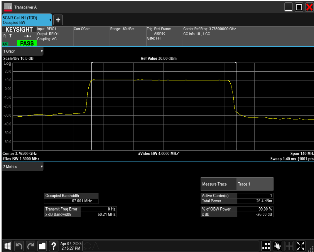
n78(3700-3800) SCS=30kHz DFT_QAM16 BW=70MHz Channel=651000 RB=180@0
