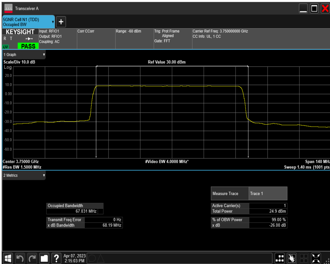
n78(3700-3800) SCS=30kHz CP_QPSK BW=70MHz Channel=650000 RB=189@0
