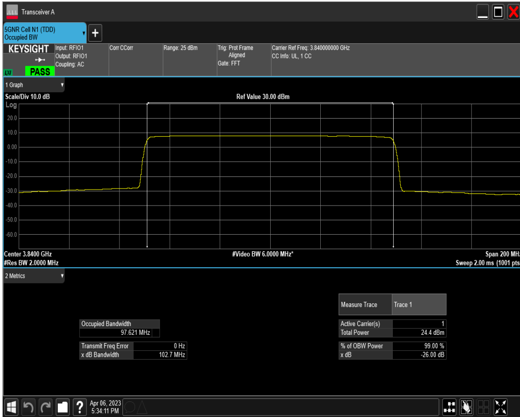
n77(3700-3980) SCS=30kHz DFT_BPSK BW=100MHz Channel=662000 RB=270@0
