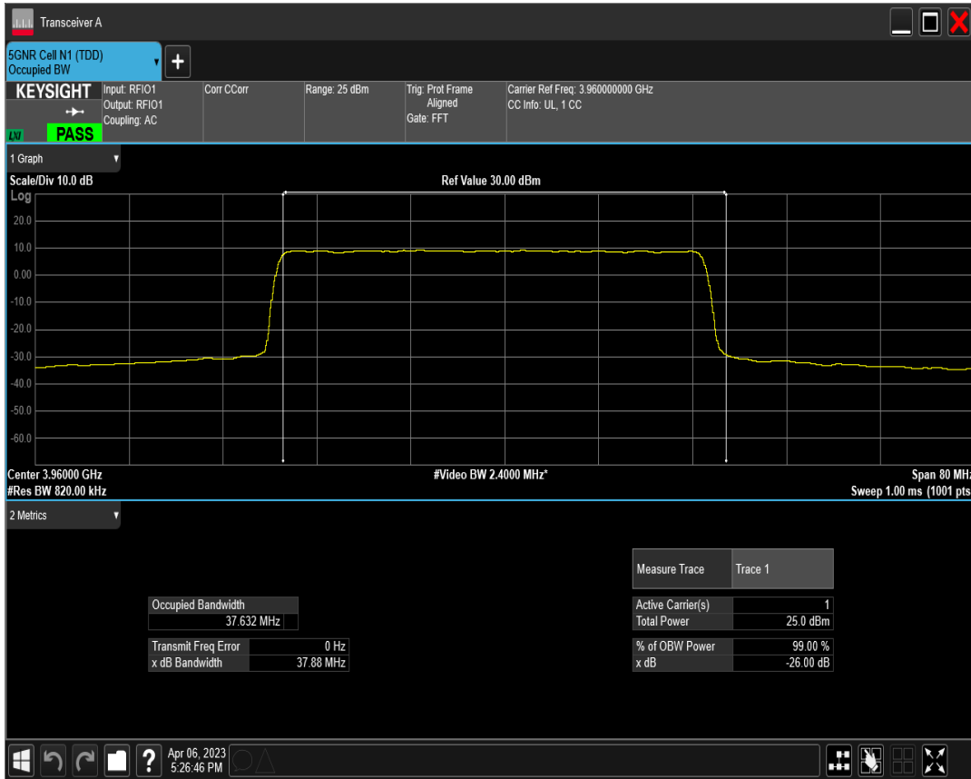
n77(3700-3980) SCS=30kHz DFT_QAM256 BW=40MHz Channel=664000 RB=100@0
