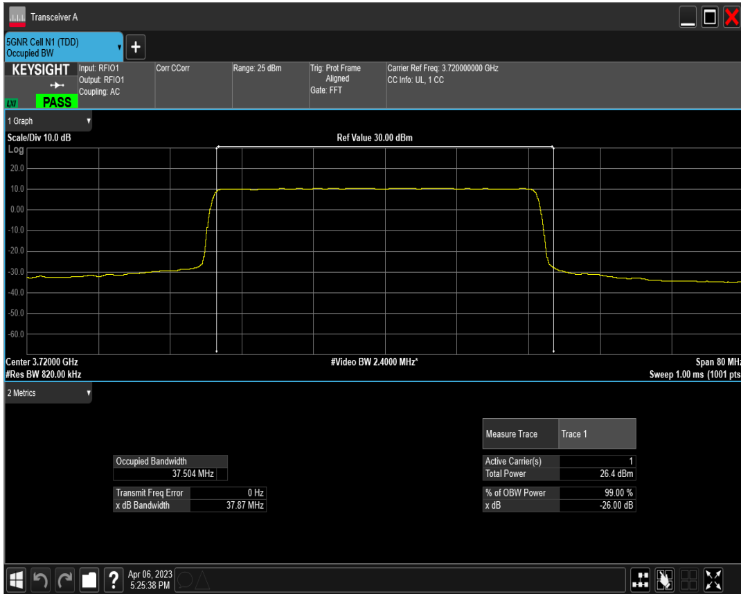
n77(3700-3980) SCS=30kHz DFT_QAM16 BW=40MHz Channel=648000 RB=100@0
