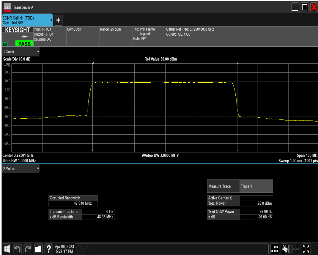
n77(3700-3980) SCS=30kHz DFT_QAM256 BW=50MHz Channel=648334 RB=128@0
