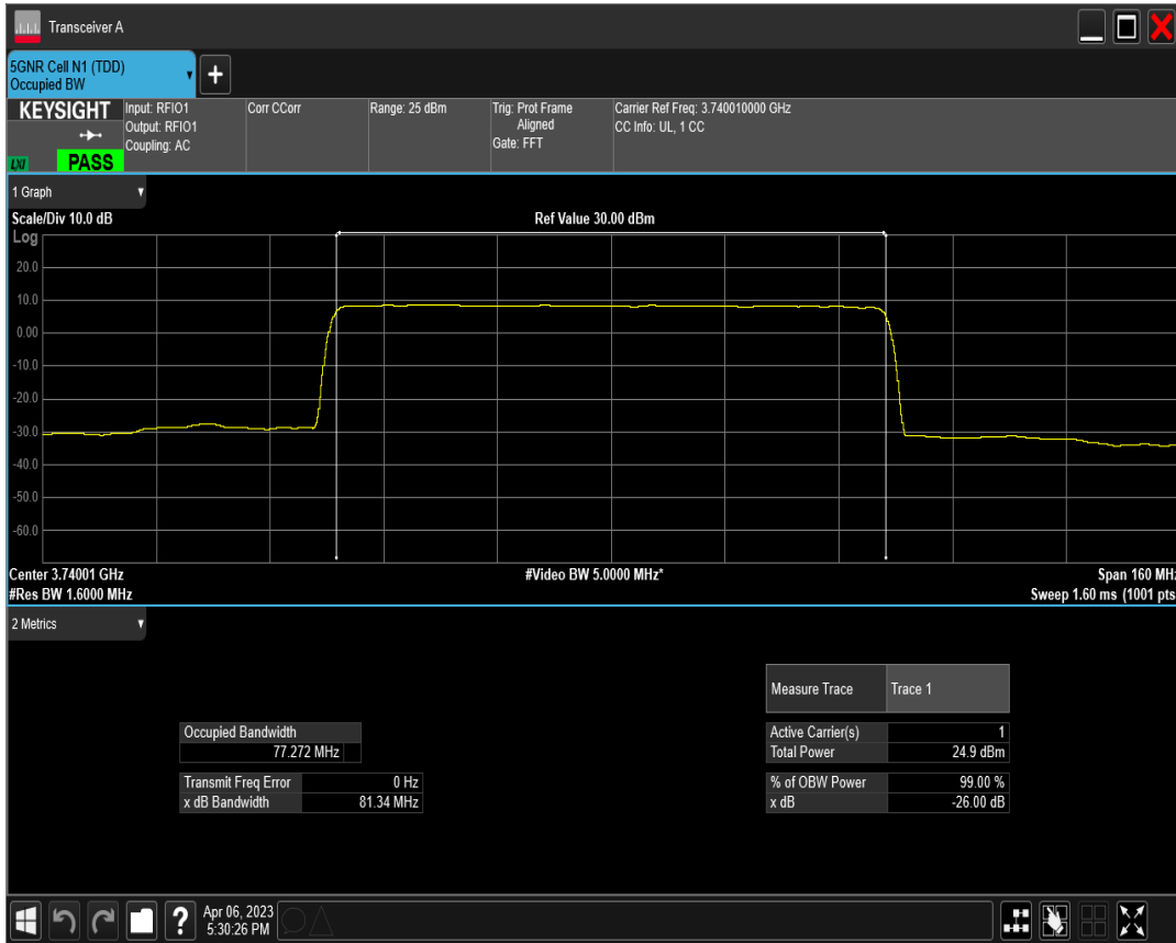
n77(3700-3980) SCS=30kHz DFT_QAM256 BW=80MHz Channel=649334 RB=216@0
