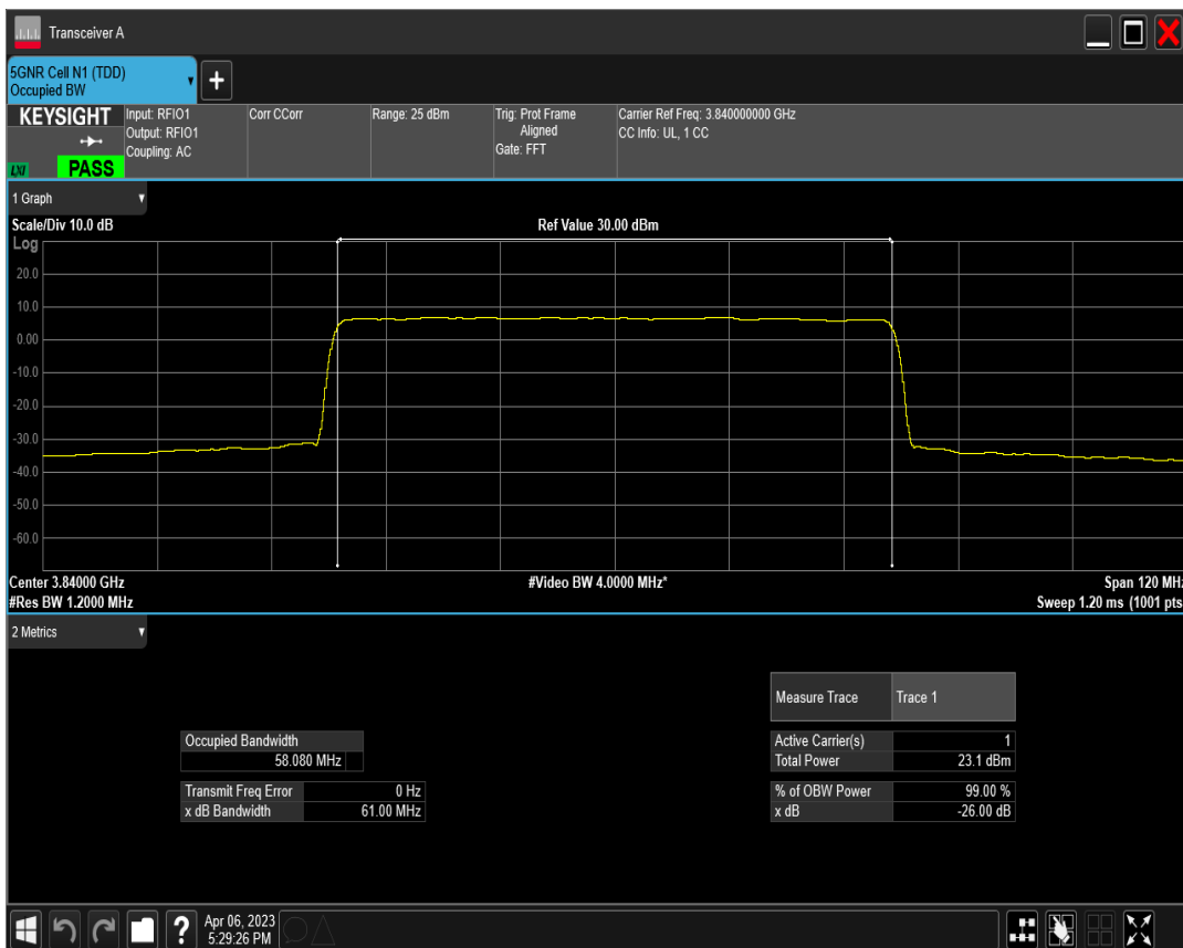
n77(3700-3980) SCS=30kHz CP_QPSK BW=60MHz Channel=656000 RB=162@0
