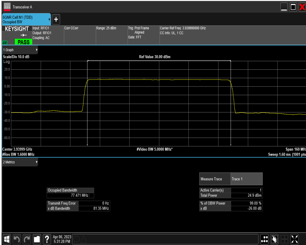
n77(3700-3980) SCS=30kHz DFT_QAM256 BW=80MHz Channel=662666 RB=216@0
