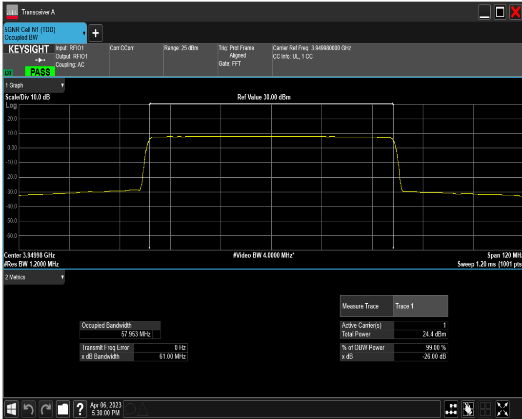
n77(3700-3980) SCS=30kHz DFT_BPSK BW=80MHz Channel=649334 RB=216@0
