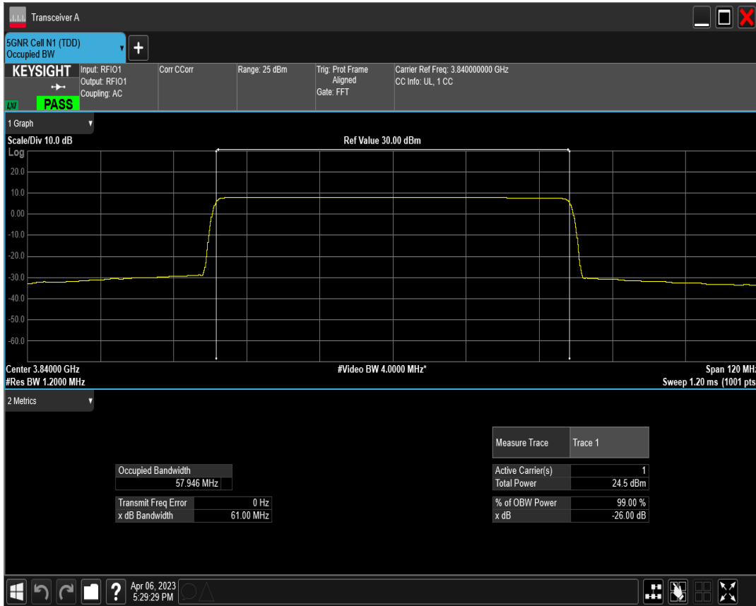
n77(3700-3980) SCS=30kHz DFT_BPSK BW=60MHz Channel=663332 RB=162@0
