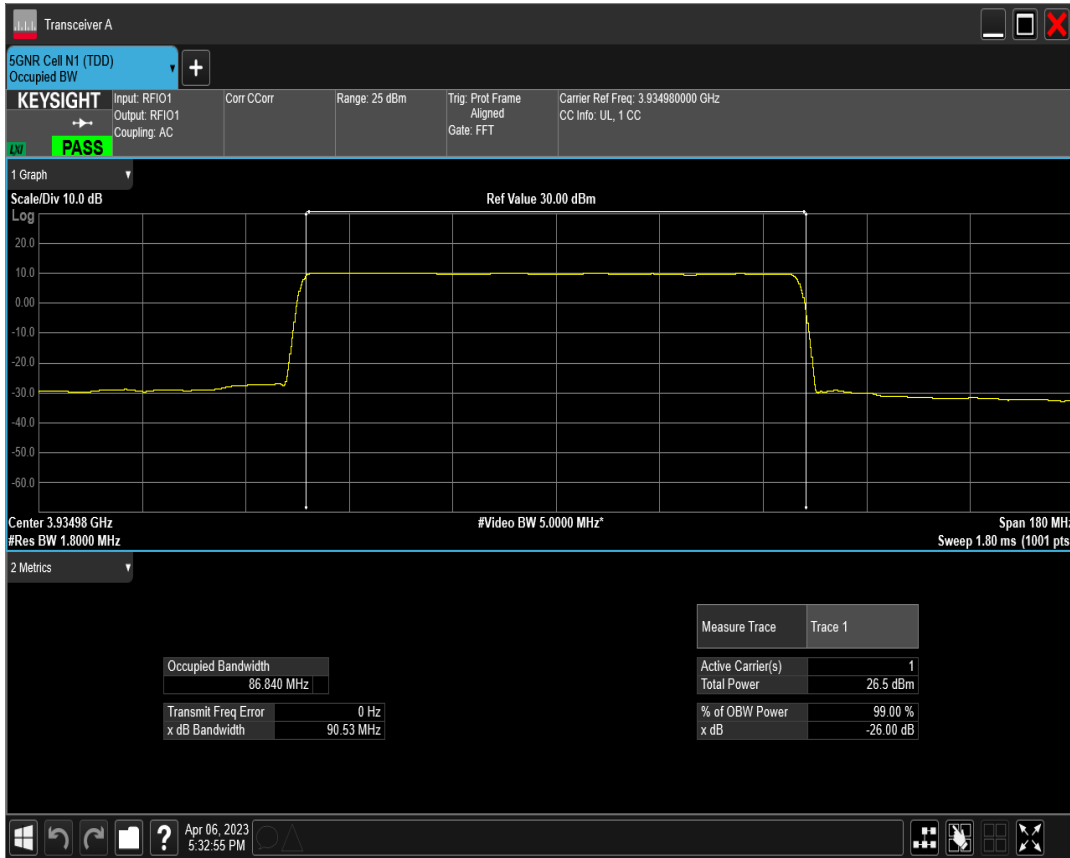
n77(3700-3980) SCS=30kHz DFT_QAM16 BW=90MHz Channel=662332 RB=240@0
