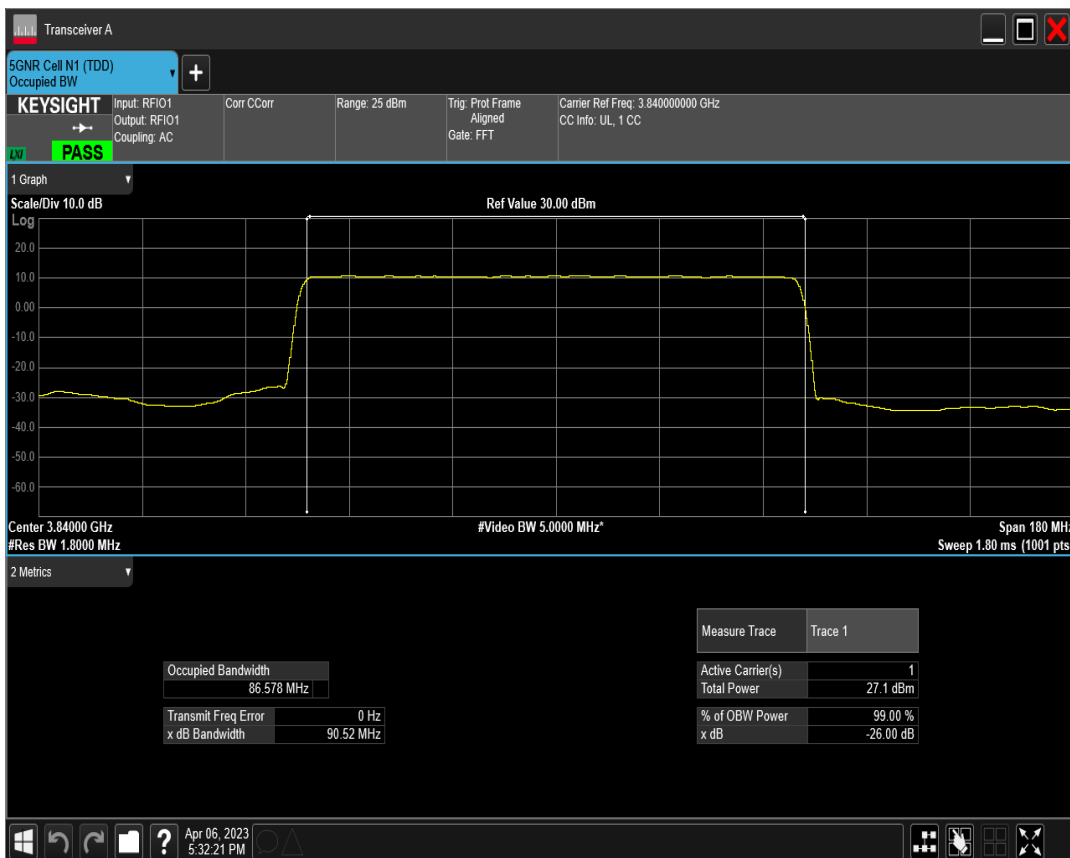
n77(3700-3980) SCS=30kHz DFT_QPSK BW=90MHz Channel=656000 RB=240@0
