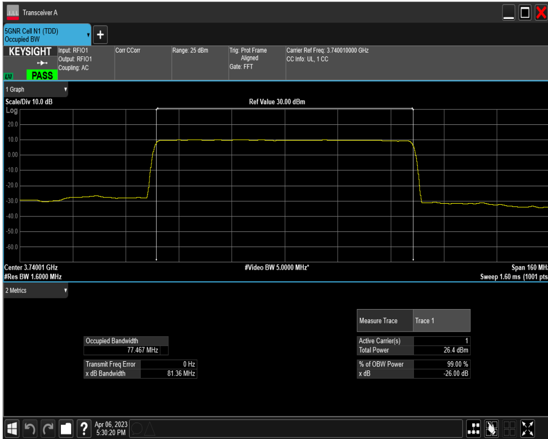
n77(3700-3980) SCS=30kHz DFT_QAM16 BW=80MHz Channel=649334 RB=216@0
