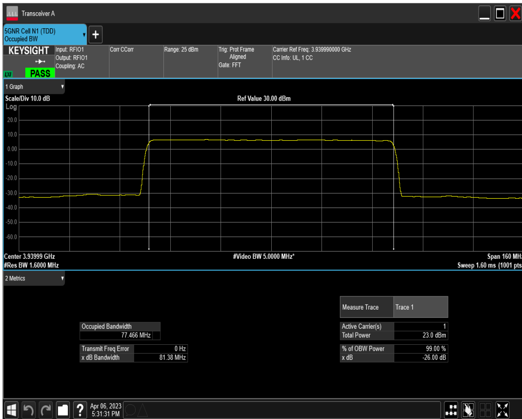
n77(3700-3980) SCS=30kHz CP_QPSK BW=80MHz Channel=662666 RB=217@0
