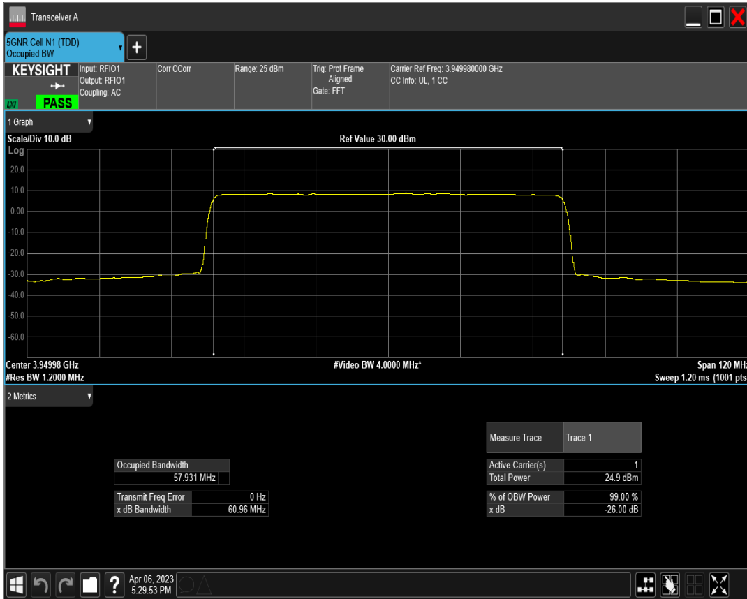
n77(3700-3980) SCS=30kHz DFT_QAM256 BW=60MHz Channel=663332 RB=162@0
