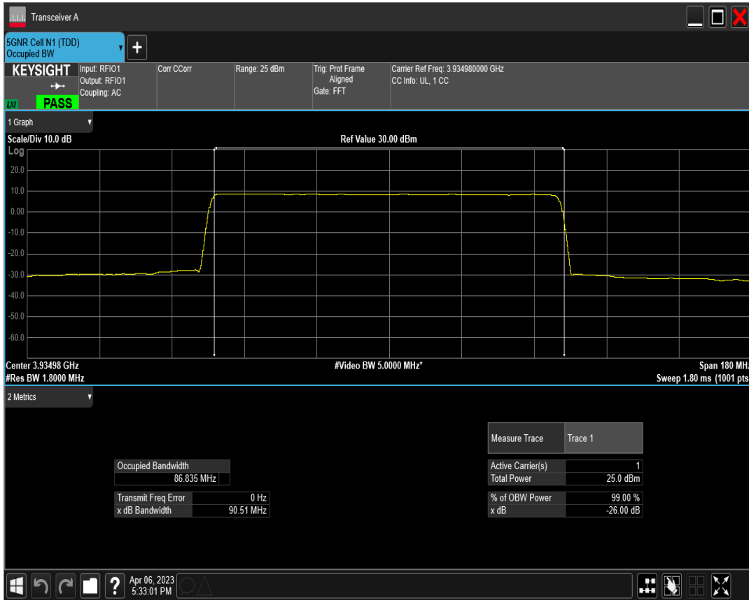
n77(3700-3980) SCS=30kHz DFT_QAM256 BW=90MHz Channel=662332 RB=240@0
