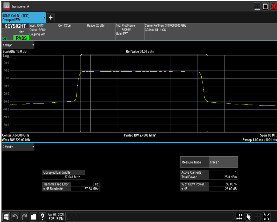
n77(3700-3980) SCS=30kHz DFT_QAM256 BW=40MHz Channel=656000 RB=100@0
