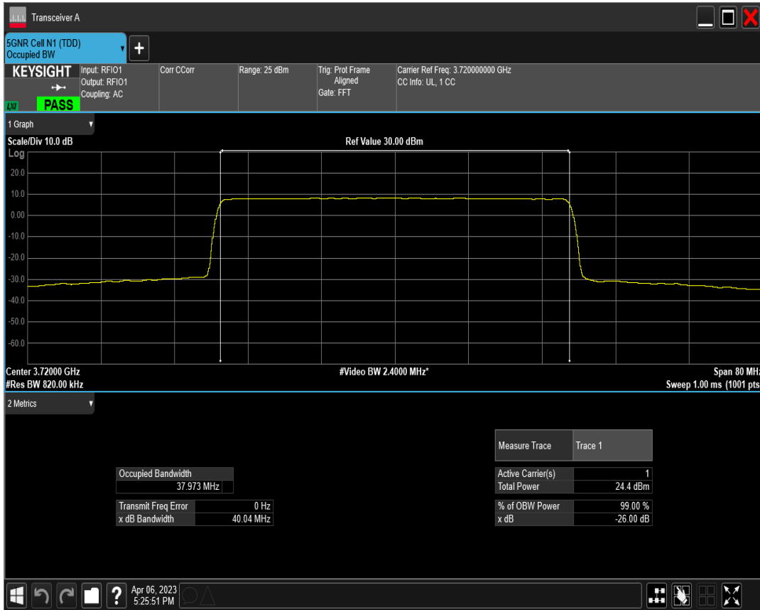
n77(3700-3980) SCS=30kHz DFT_BPSK BW=40MHz Channel=656000 RB=100@0
