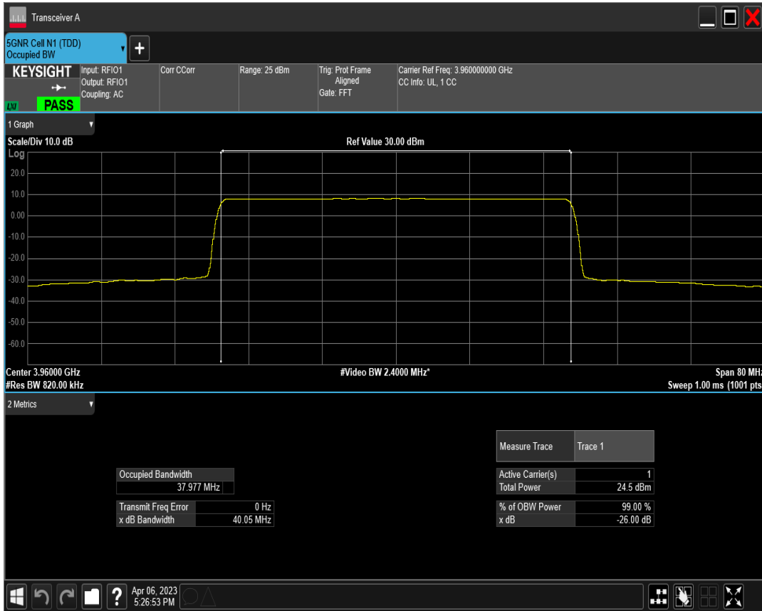
n77(3700-3980) SCS=30kHz DFT_BPSK BW=50MHz Channel=648334 RB=128@0
