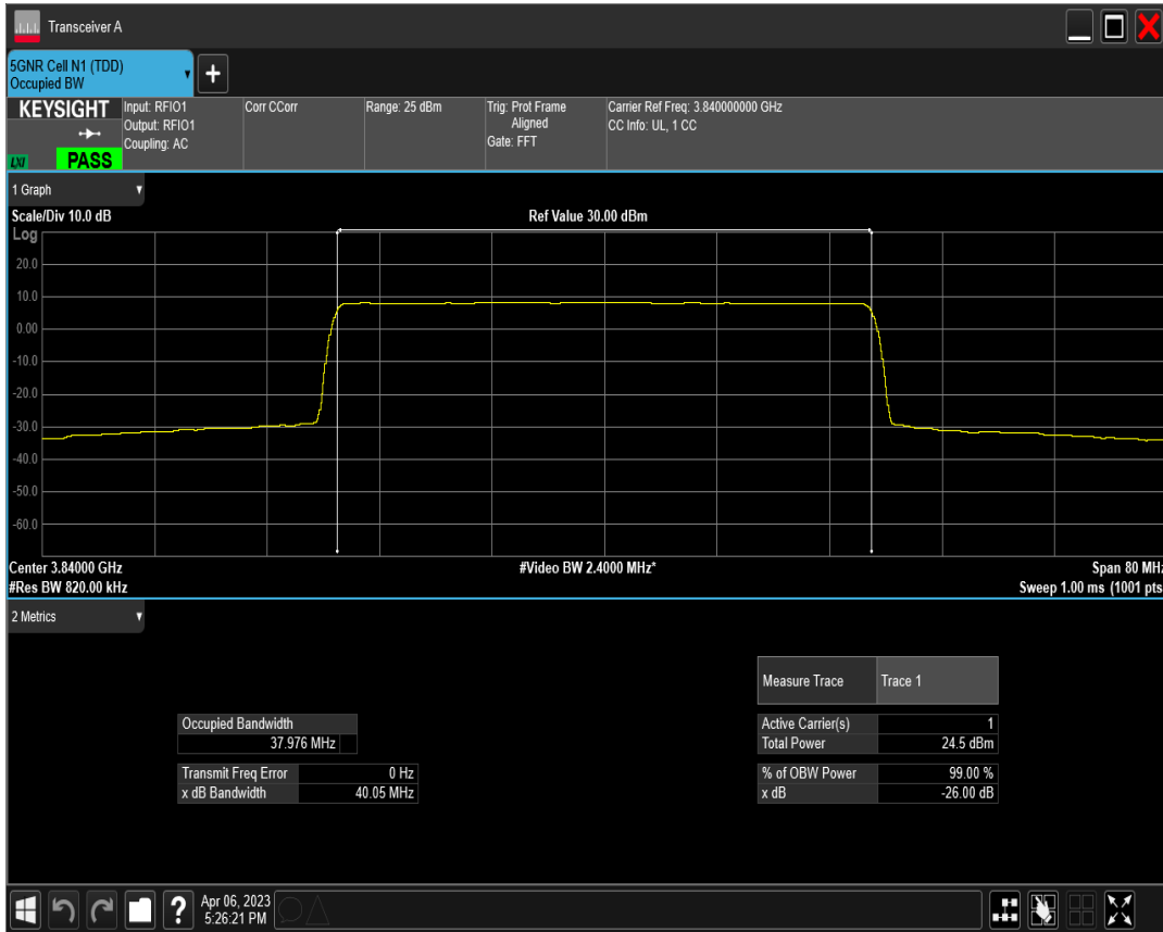
n77(3700-3980) SCS=30kHz DFT_BPSK BW=40MHz Channel=664000 RB=100@0
