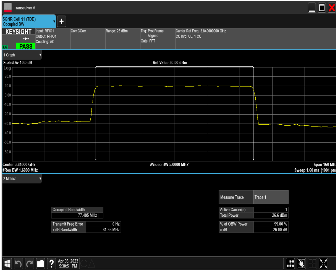
n77(3700-3980) SCS=30kHz DFT_QAM16 BW=80MHz Channel=656000 RB=216@0
