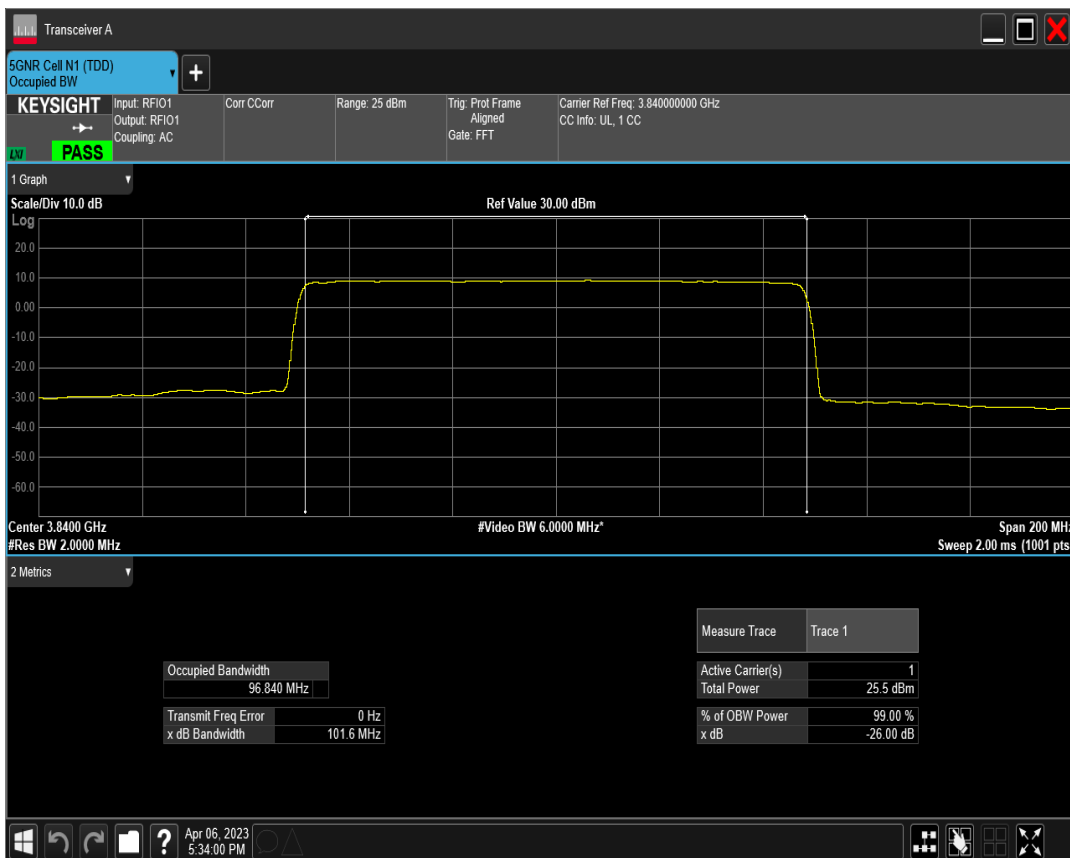
n77(3700-3980) SCS=30kHz DFT_QAM64 BW=100MHz Channel=656000 RB=270@0
