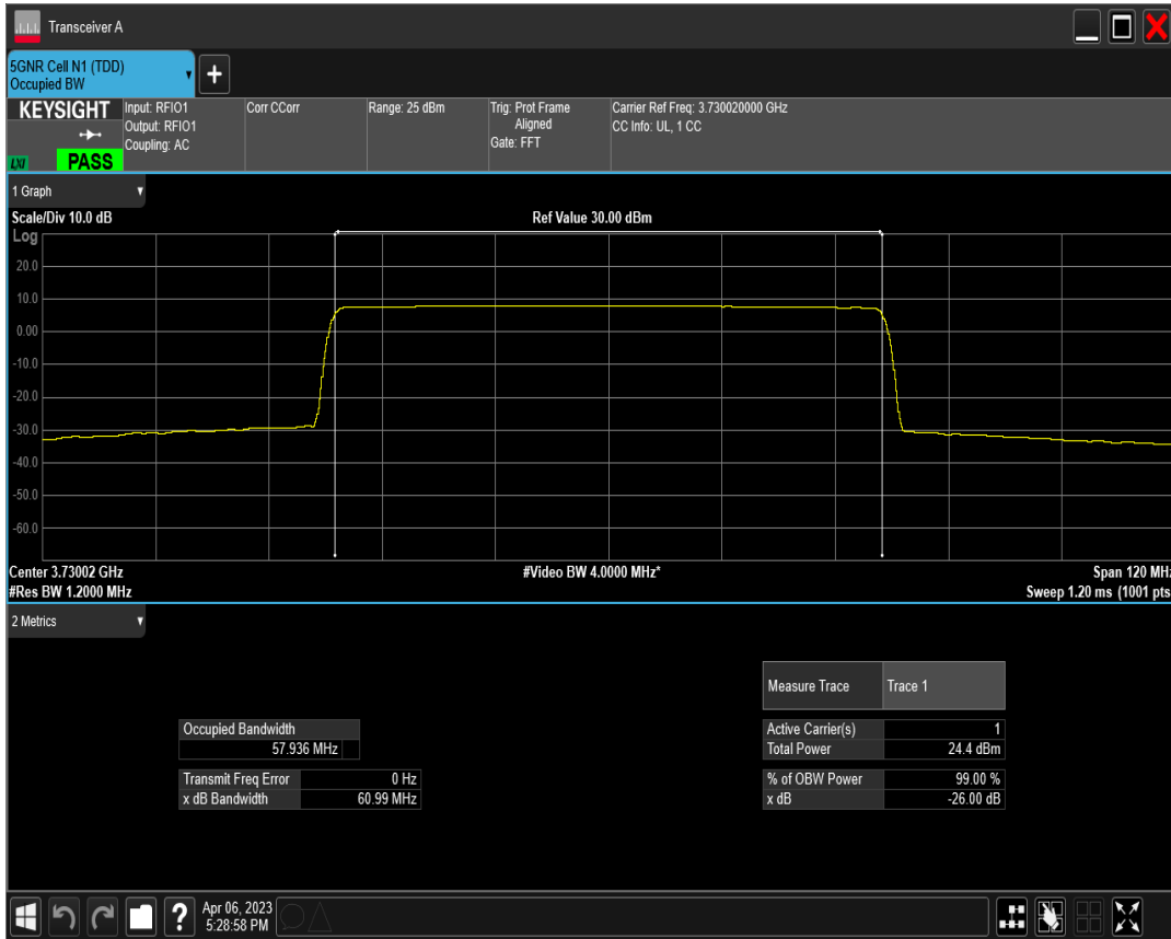
n77(3700-3980) SCS=30kHz DFT_BPSK BW=60MHz Channel=656000 RB=162@0
