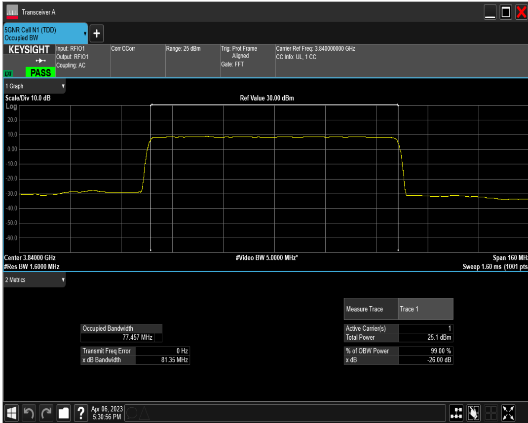
n77(3700-3980) SCS=30kHz DFT_QAM256 BW=80MHz Channel=656000 RB=216@0
