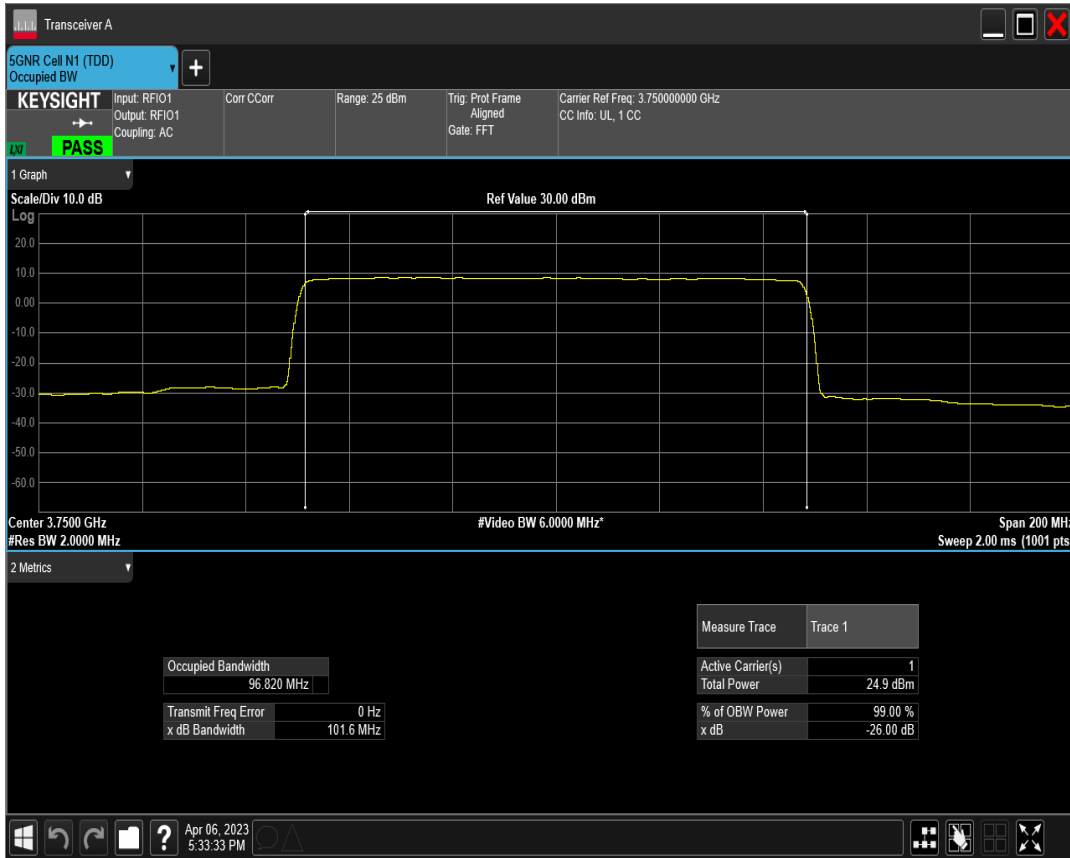
n77(3700-3980) SCS=30kHz DFT_QAM256 BW=100MHz Channel=650000 RB=270@0
