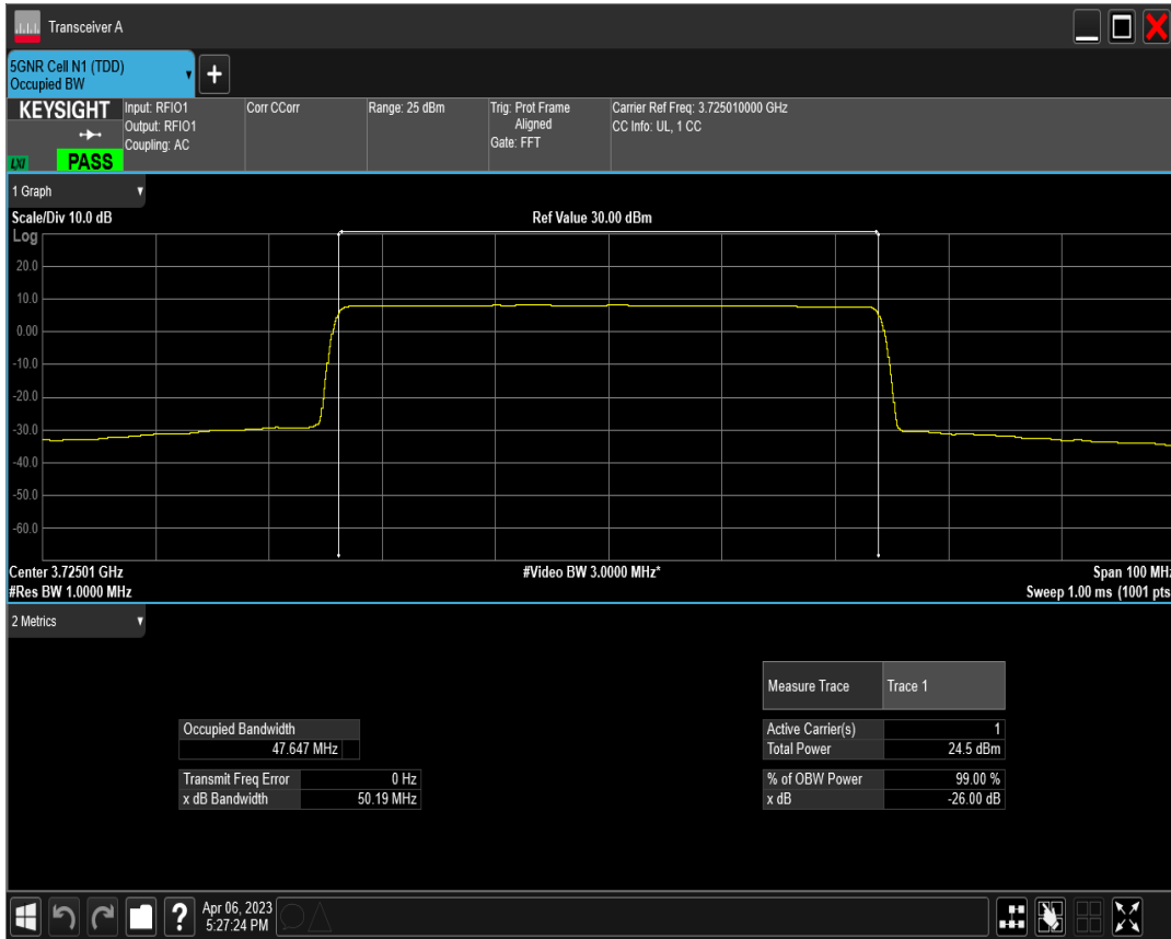
n77(3700-3980) SCS=30kHz DFT_BPSK BW=50MHz Channel=656000 RB=128@0
