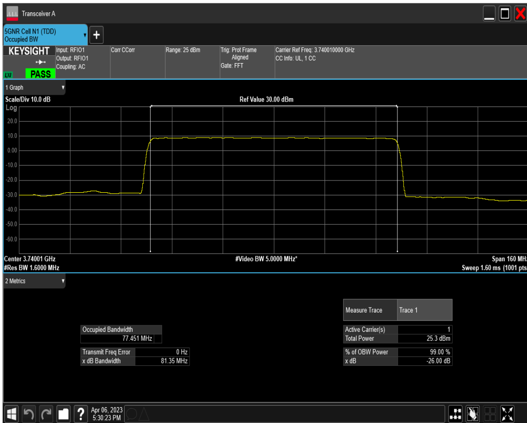
n77(3700-3980) SCS=30kHz DFT_QAM64 BW=80MHz Channel=649334 RB=216@0
