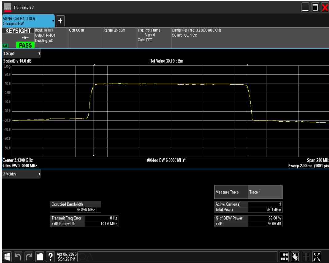
n77(3700-3980) SCS=30kHz DFT_QAM16 BW=100MHz Channel=662000 RB=270@0
