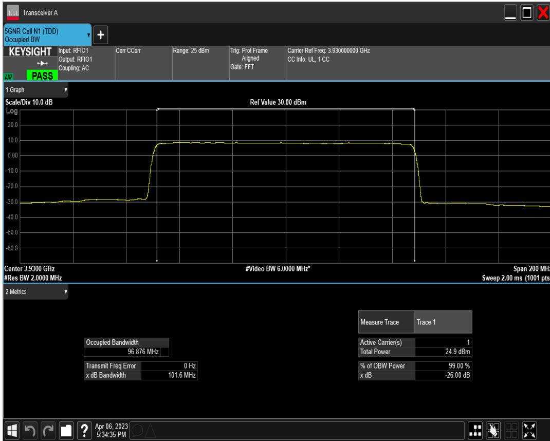
n77(3700-3980) SCS=30kHz DFT_QAM256 BW=100MHz Channel=662000 RB=270@0
