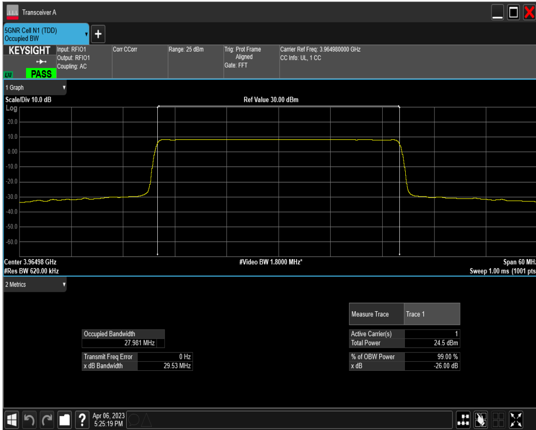
n77(3700-3980) SCS=30kHz DFT_BPSK BW=40MHz Channel=648000 RB=100@0
