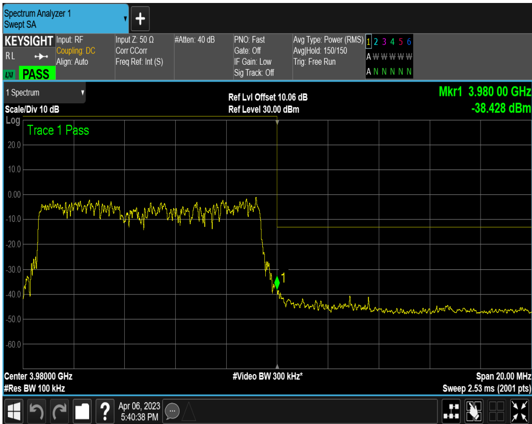
n77(3700-3980) SCS=30kHz DFT_QPSK BW=10MHz Channel=665000 RB=1@23
