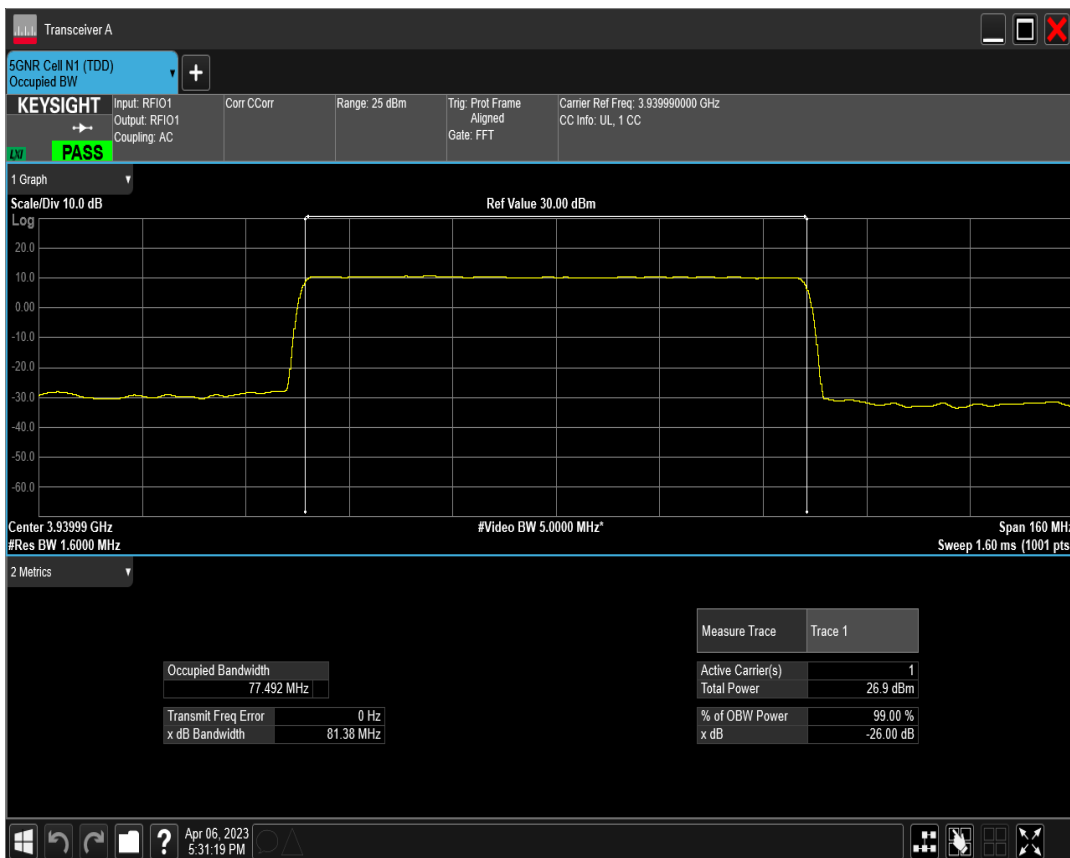
n77(3700-3980) SCS=30kHz DFT_QPSK BW=80MHz Channel=662666 RB=216@0
