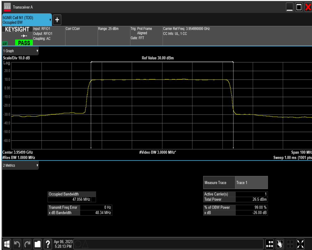
n77(3700-3980) SCS=30kHz DFT_QAM16 BW=50MHz Channel=663666 RB=128@0
