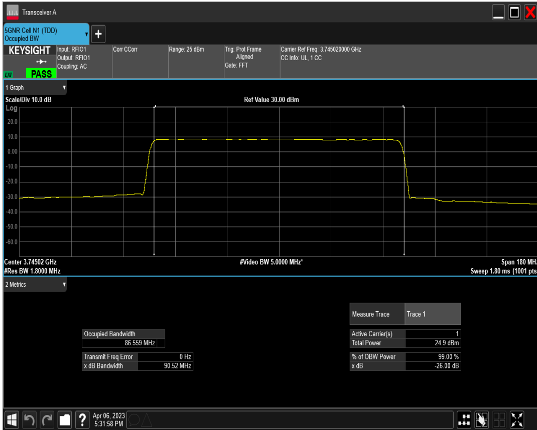
n77(3700-3980) SCS=30kHz DFT_QAM256 BW=90MHz Channel=649668 RB=240@0
