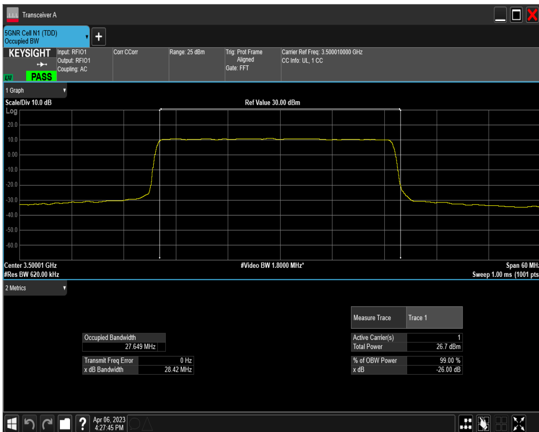
n77(3450-3550) SCS=30kHz DFT_QAM16 BW=30MHz Channel=633334 RB=75@0
