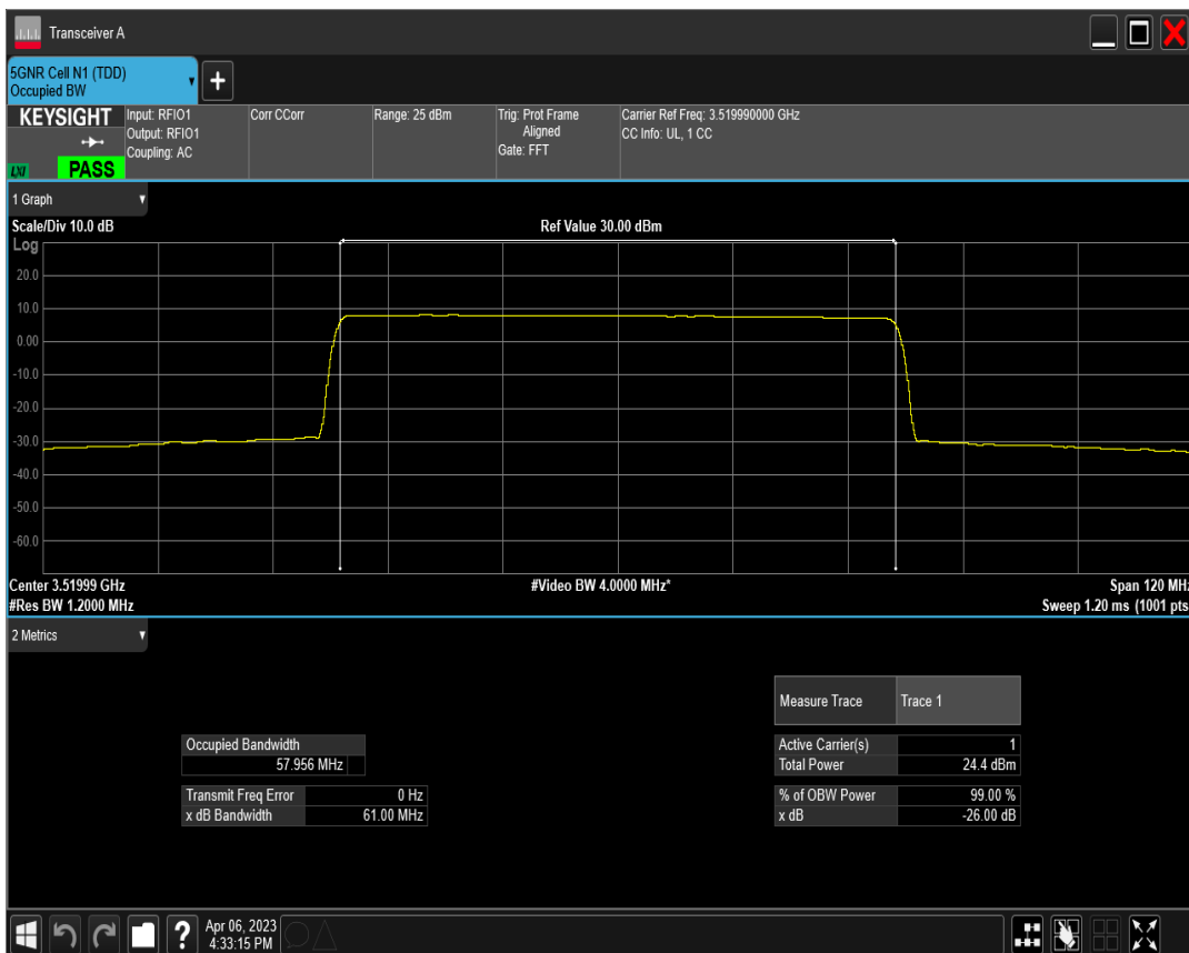
n77(3450-3550) SCS=30kHz DFT_BPSK BW=80MHz Channel=632668 RB=216@0
