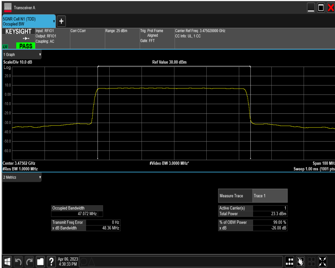
n77(3450-3550) SCS=30kHz CP_QPSK BW=50MHz Channel=631668 RB=133@0
