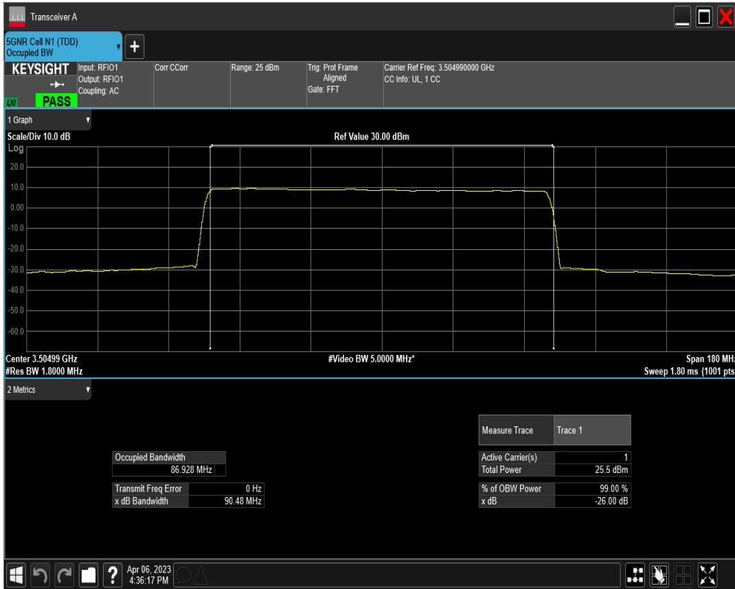
n77(3450-3550) SCS=30kHz DFT_QAM64 BW=90MHz Channel=633666 RB=240@0
