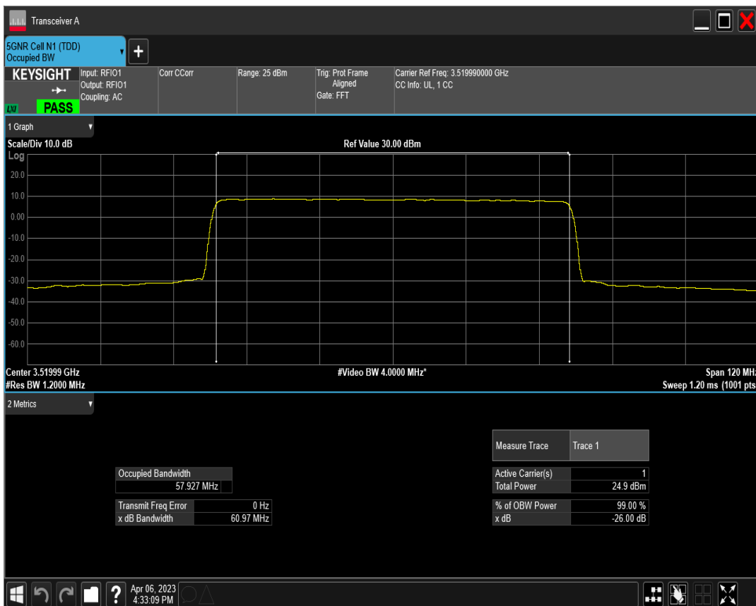
n77(3450-3550) SCS=30kHz DFT_QAM256 BW=60MHz Channel=634666 RB=162@0
