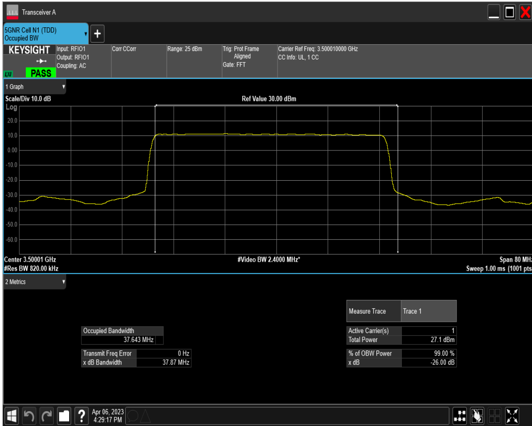
n77(3450-3550) SCS=30kHz DFT_QPSK BW=40MHz Channel=633334 RB=100@0
