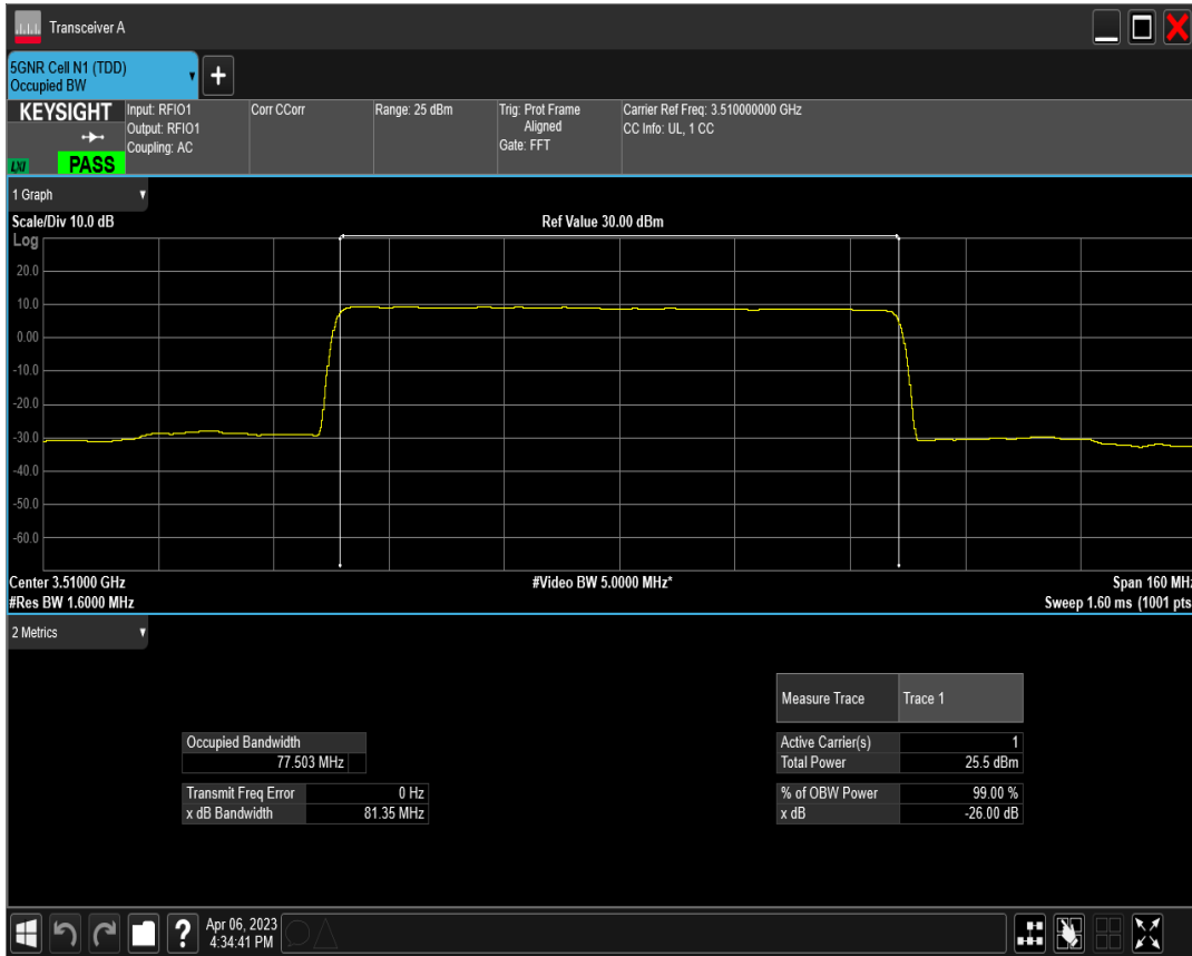
n77(3450-3550) SCS=30kHz DFT_QAM64 BW=80MHz Channel=634000 RB=216@0
