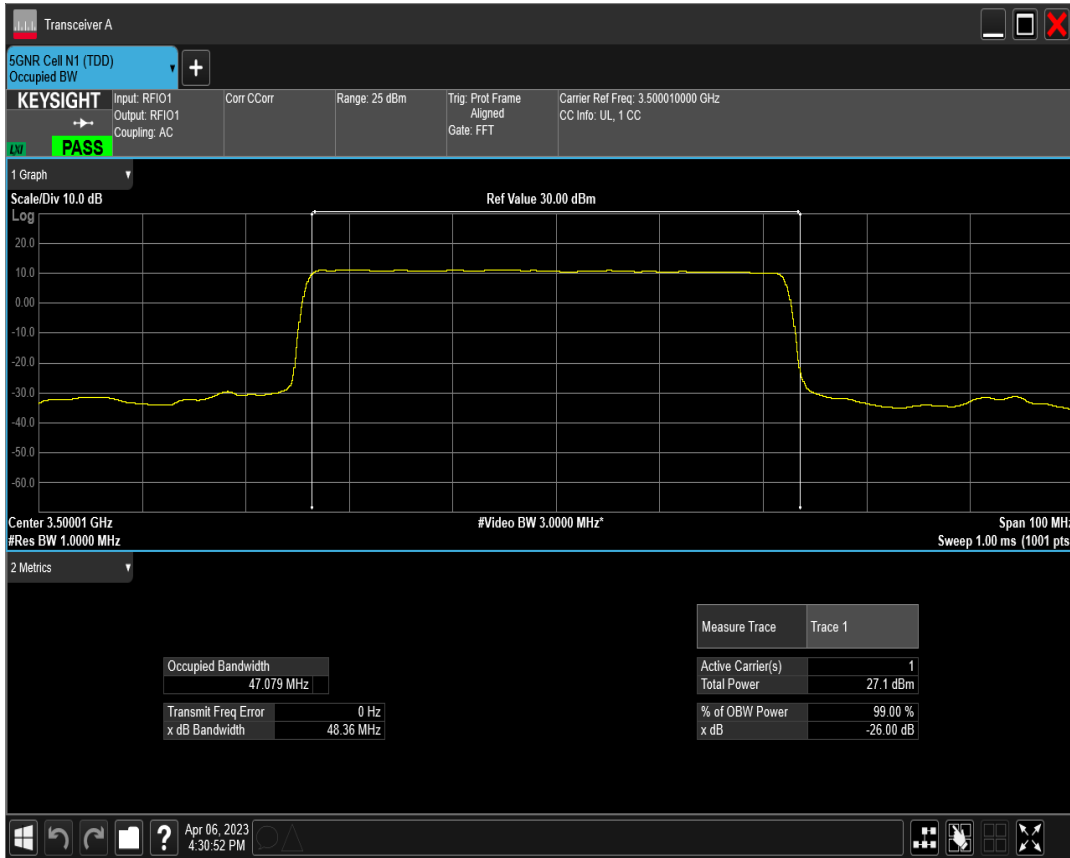
n77(3450-3550) SCS=30kHz DFT_QPSK BW=50MHz Channel=633334 RB=128@0
