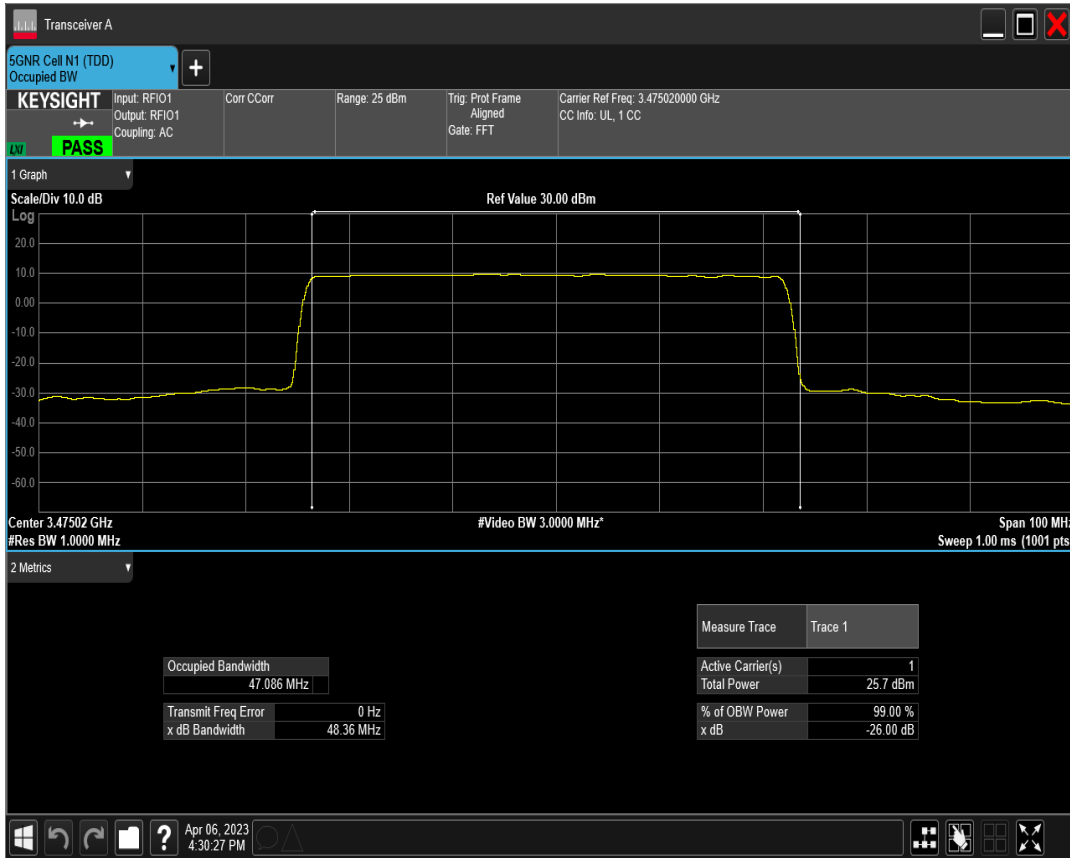
n77(3450-3550) SCS=30kHz DFT_QAM64 BW=50MHz Channel=631668 RB=128@0
