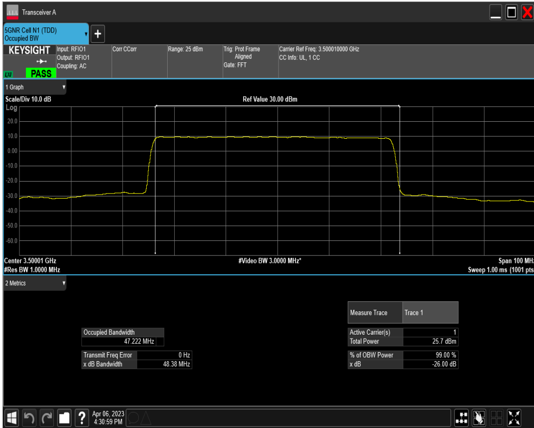
n77(3450-3550) SCS=30kHz DFT_QAM64 BW=50MHz Channel=633334 RB=128@0
