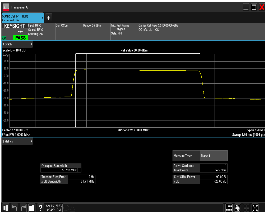
n77(3450-3550) SCS=30kHz DFT_BPSK BW=90MHz Channel=633000 RB=240@0
