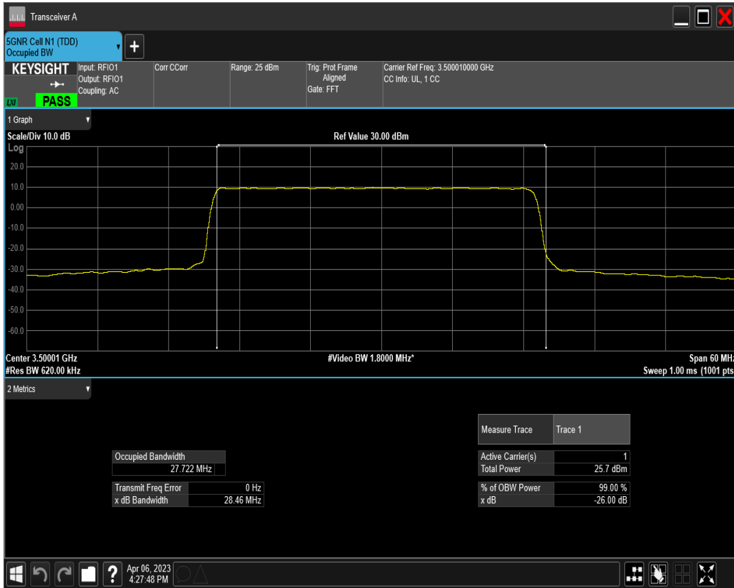
n77(3450-3550) SCS=30kHz DFT_QAM64 BW=30MHz Channel=633334 RB=75@0
