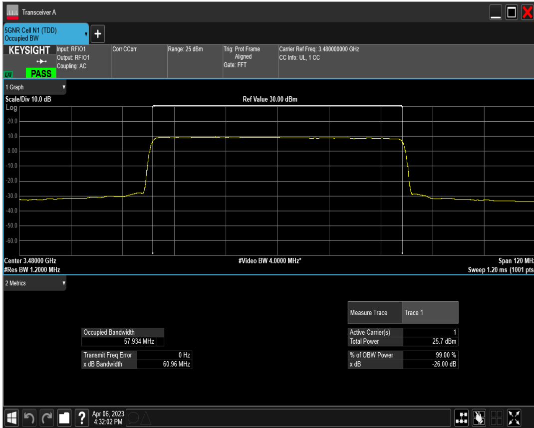
n77(3450-3550) SCS=30kHz DFT_QAM64 BW=60MHz Channel=632000 RB=162@0
