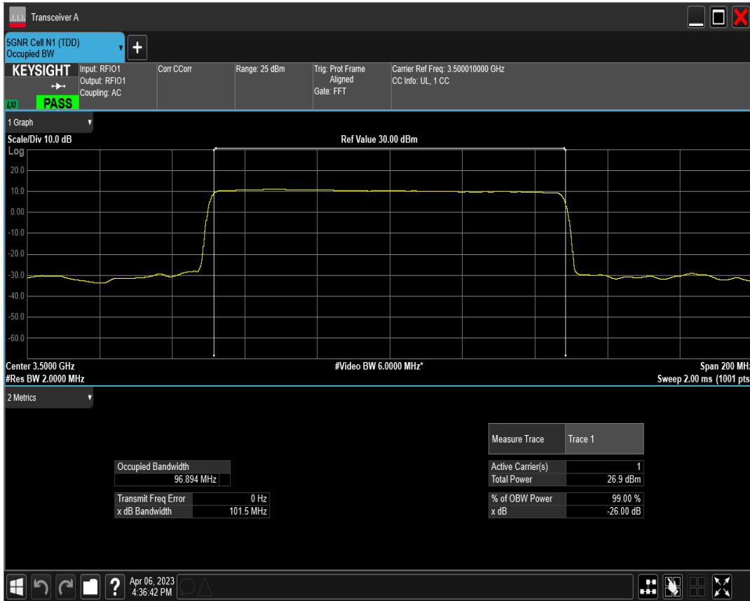
n77(3450-3550) SCS=30kHz DFT_QPSK BW=100MHz Channel=633334 RB=270@0
