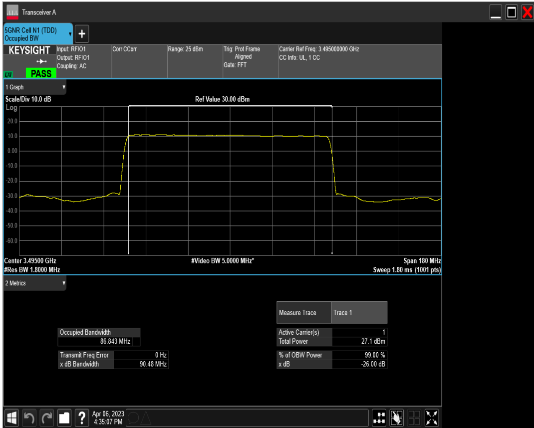
n77(3450-3550) SCS=30kHz DFT_QPSK BW=90MHz Channel=633000 RB=240@0
