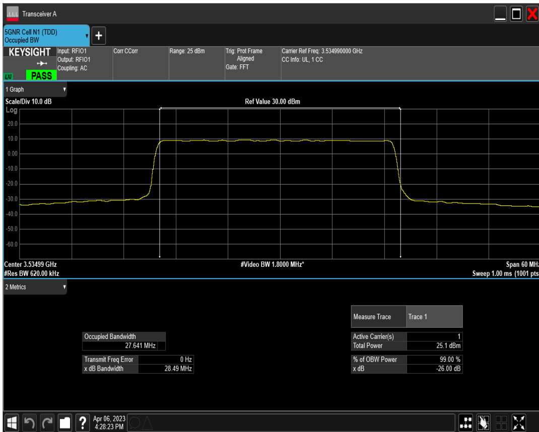
n77(3450-3550) SCS=30kHz DFT_QAM256 BW=30MHz Channel=635666 RB=75@0
