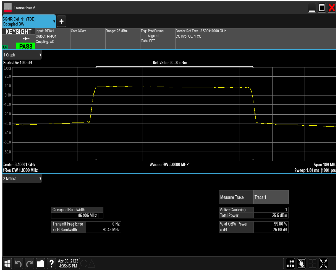
n77(3450-3550) SCS=30kHz DFT_QAM64 BW=90MHz Channel=633334 RB=240@0
