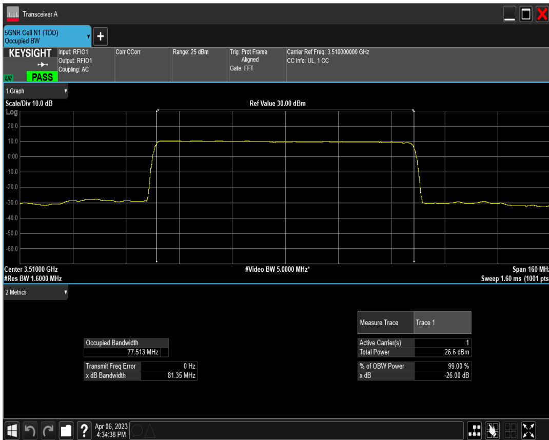
n77(3450-3550) SCS=30kHz DFT_QAM16 BW=80MHz Channel=634000 RB=216@0
