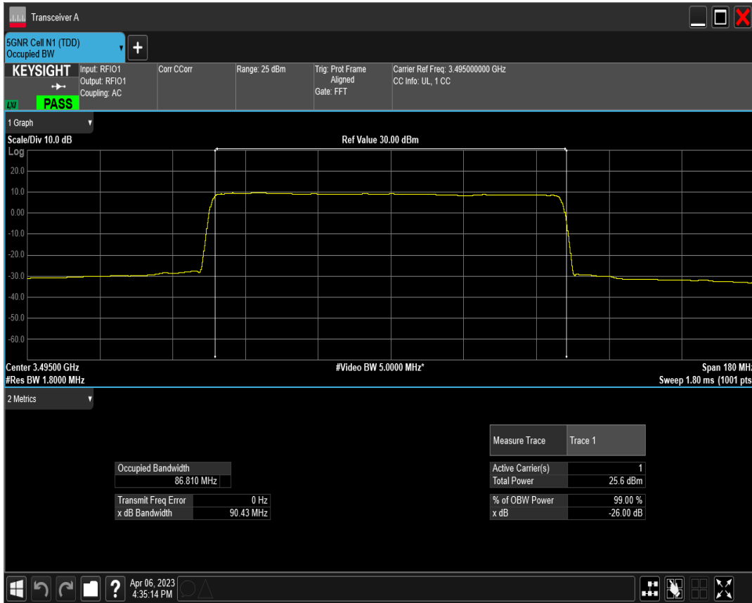
n77(3450-3550) SCS=30kHz DFT_QAM64 BW=90MHz Channel=633000 RB=240@0
