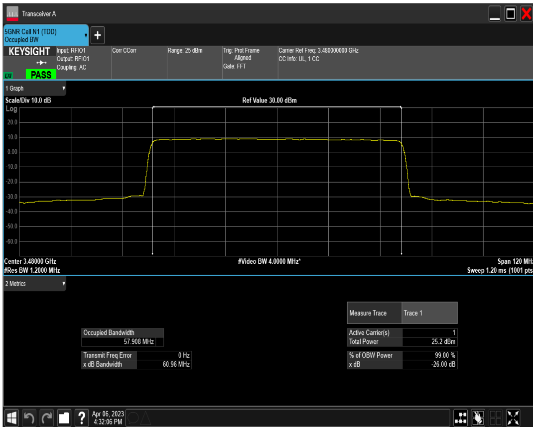
n77(3450-3550) SCS=30kHz DFT_QAM256 BW=60MHz Channel=632000 RB=162@0
