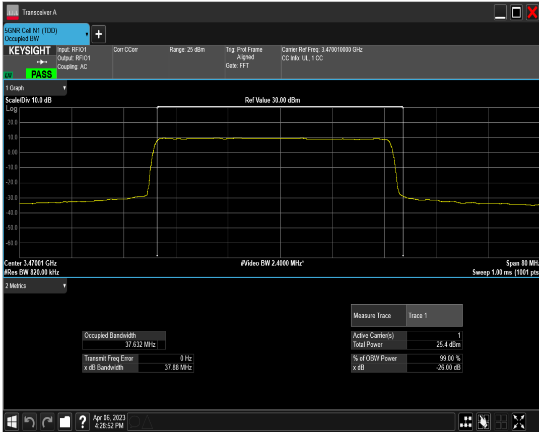
n77(3450-3550) SCS=30kHz DFT_QAM64 BW=40MHz Channel=631334 RB=100@0
