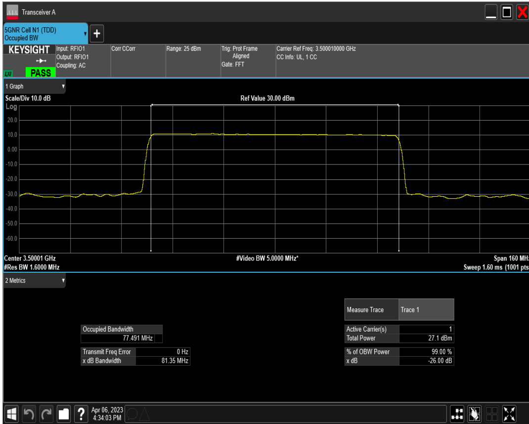
n77(3450-3550) SCS=30kHz DFT_QPSK BW=80MHz Channel=633334 RB=216@0
