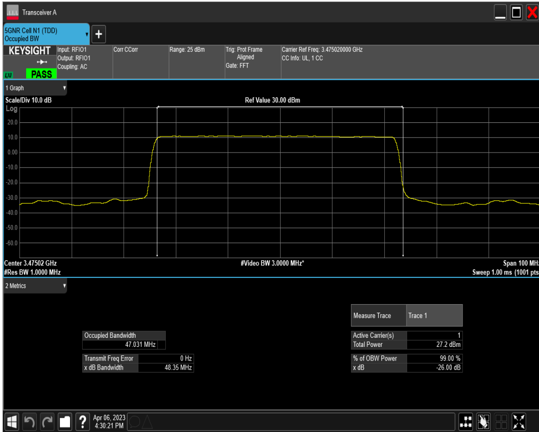
n77(3450-3550) SCS=30kHz DFT_QPSK BW=50MHz Channel=631668 RB=128@0
