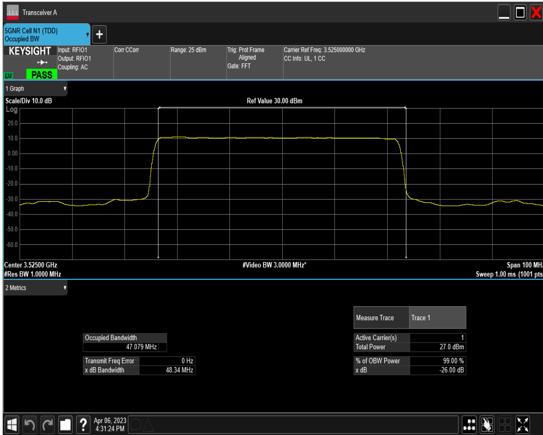
n77(3450-3550) SCS=30kHz DFT_QPSK BW=50MHz Channel=635000 RB=128@0
