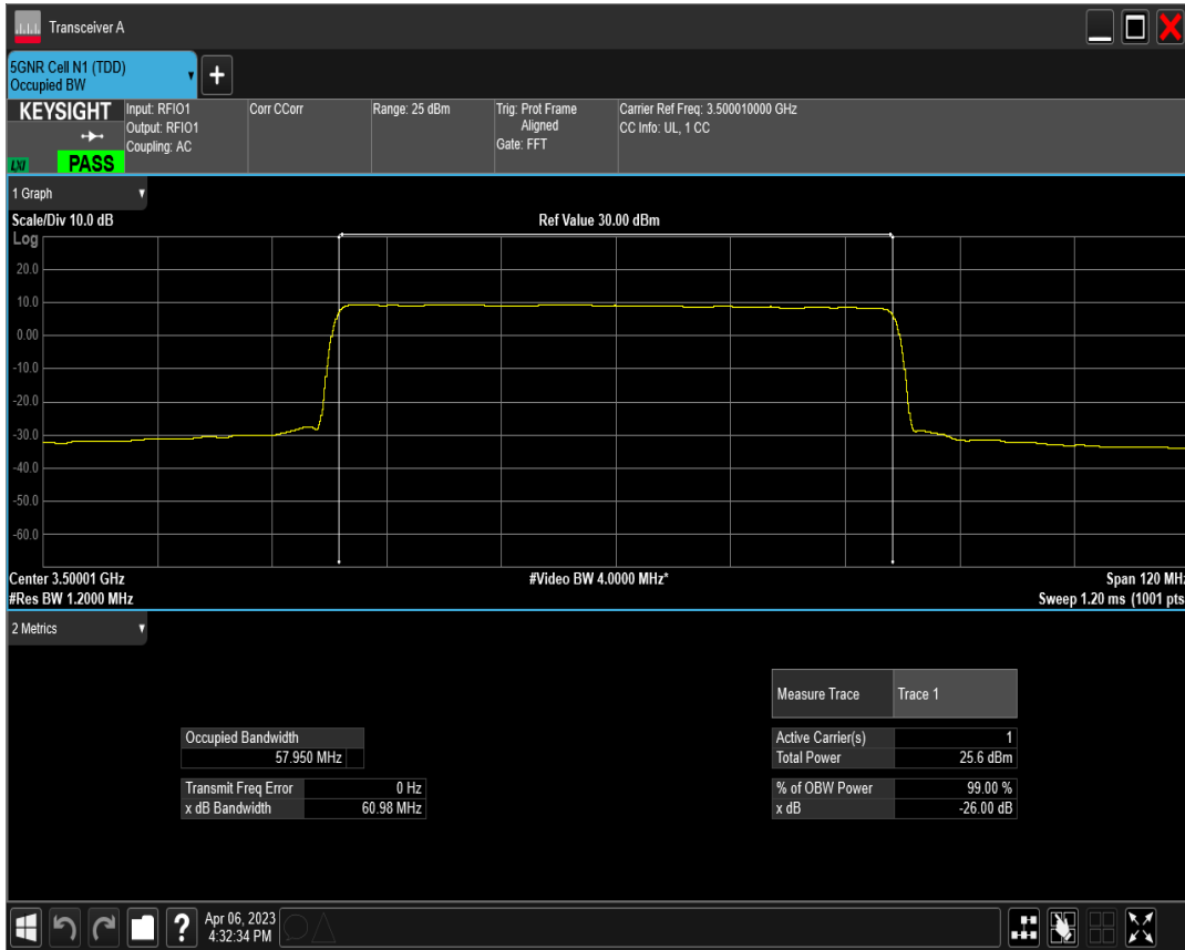
n77(3450-3550) SCS=30kHz DFT_QAM64 BW=60MHz Channel=633334 RB=162@0
