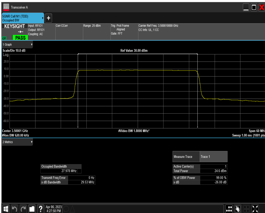
n77(3450-3550) SCS=30kHz DFT_BPSK BW=30MHz Channel=635666 RB=75@0
