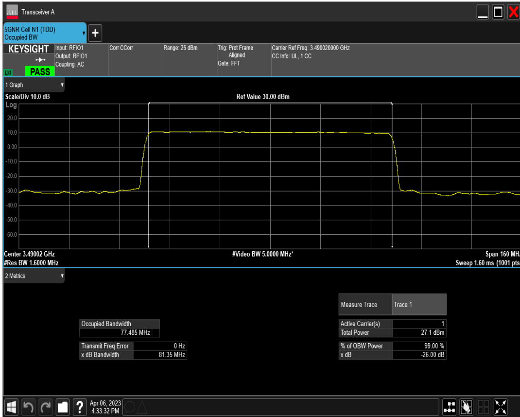
n77(3450-3550) SCS=30kHz DFT_QPSK BW=80MHz Channel=632668 RB=216@0
