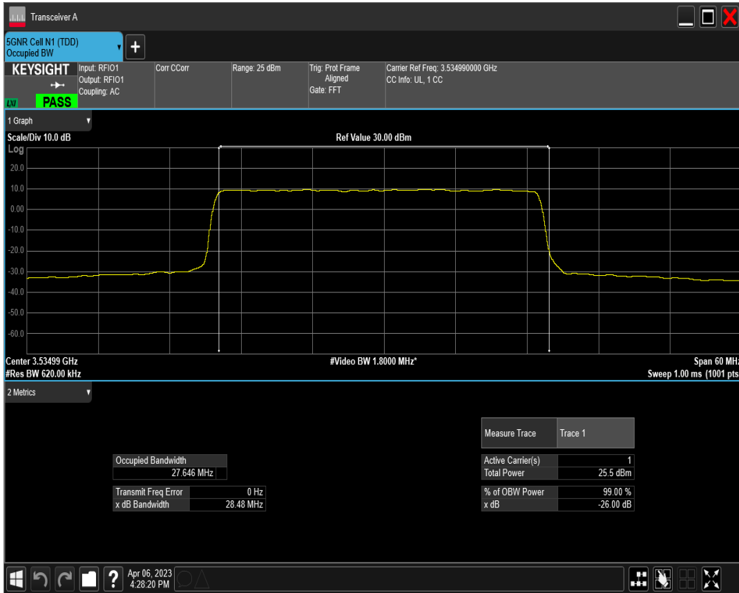
n77(3450-3550) SCS=30kHz DFT_QAM64 BW=30MHz Channel=635666 RB=75@0
