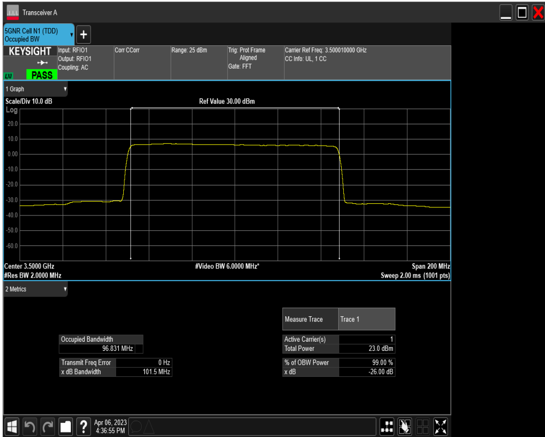
n77(3450-3550) SCS=30kHz CP_QPSK BW=100MHz Channel=633334 RB=273@0
