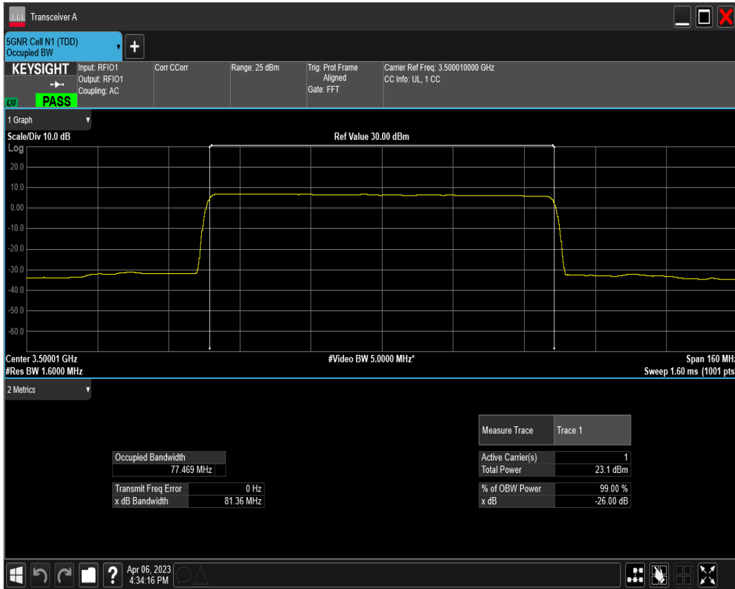
n77(3450-3550) SCS=30kHz CP_QPSK BW=80MHz Channel=633334 RB=217@0
