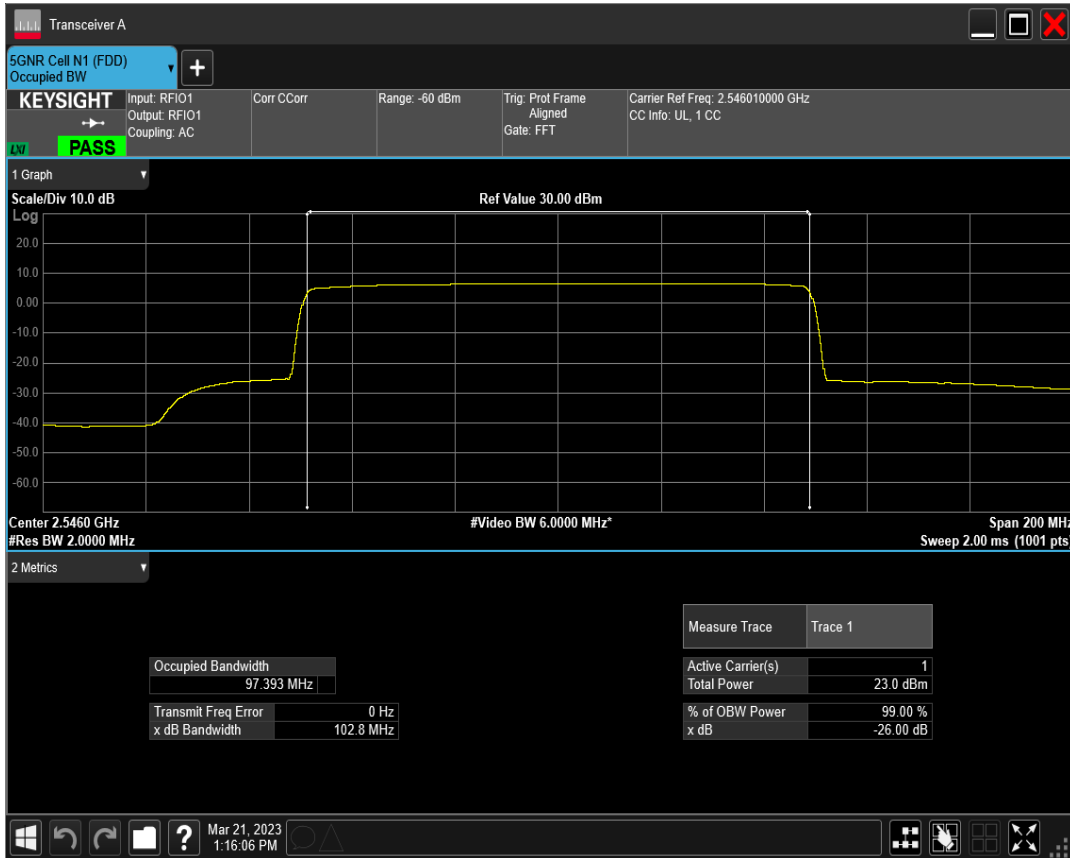
n41 SCS=30kHz DFT_BPSK BW=100MHz Channel=518598 RB=270@0
