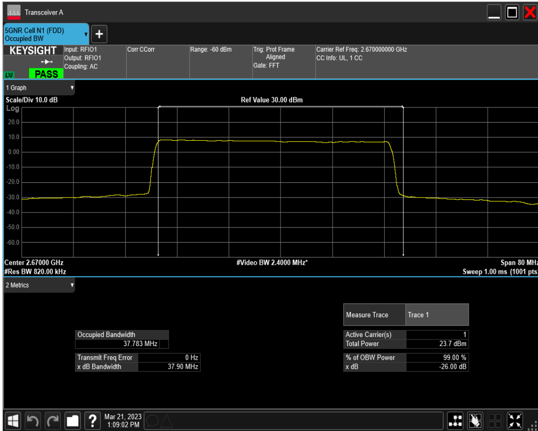
n41 SCS=30kHz DFT_QAM256 BW=40MHz Channel=534000 RB=100@0
