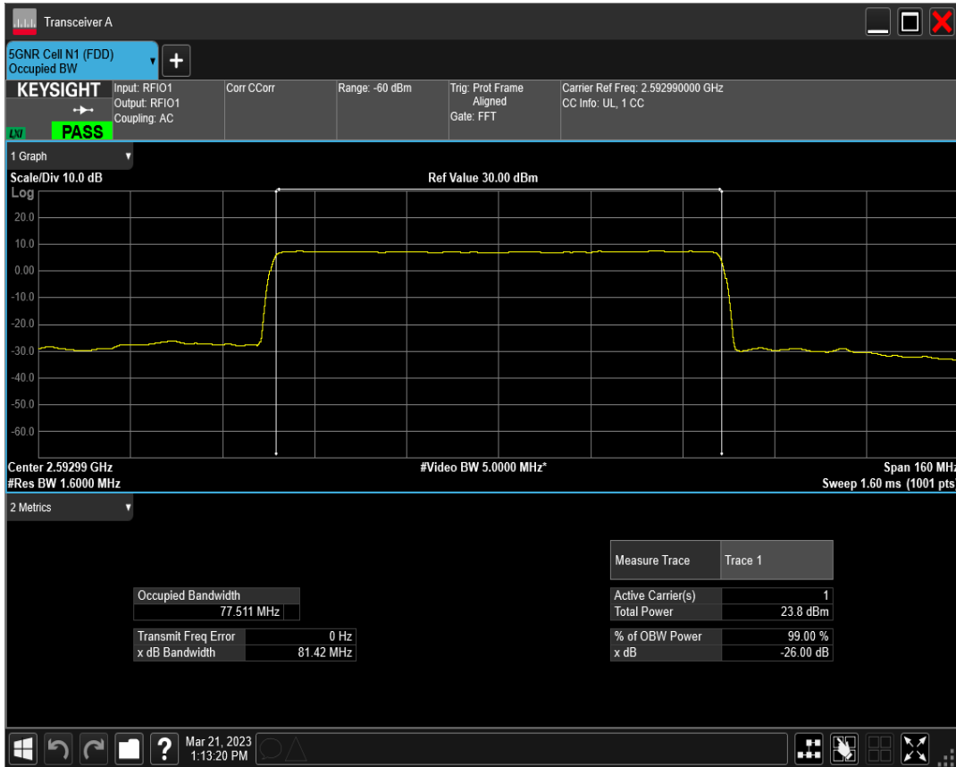
n41 SCS=30kHz DFT_QAM256 BW=80MHz Channel=518598 RB=216@0
