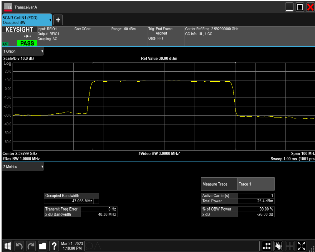
n41 SCS=30kHz DFT_QAM16 BW=50MHz Channel=518598 RB=128@0
