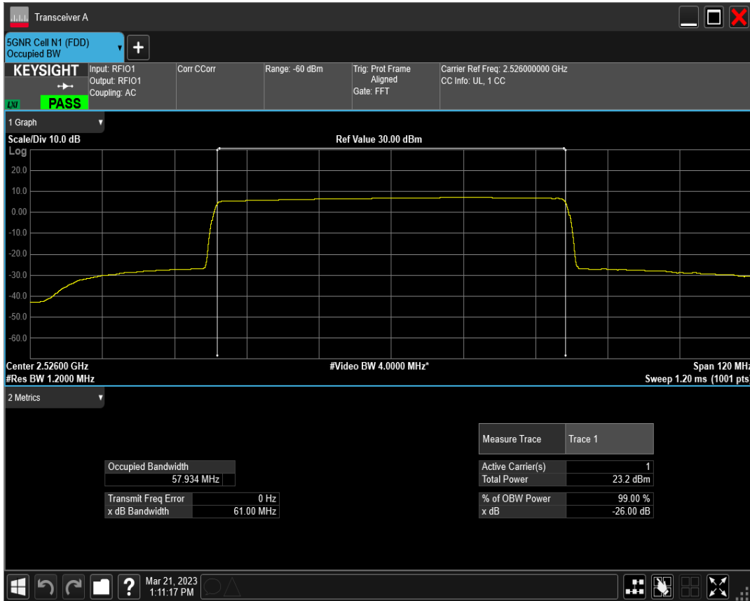
n41 SCS=30kHz DFT_BPSK BW=60MHz Channel=518598 RB=162@0
