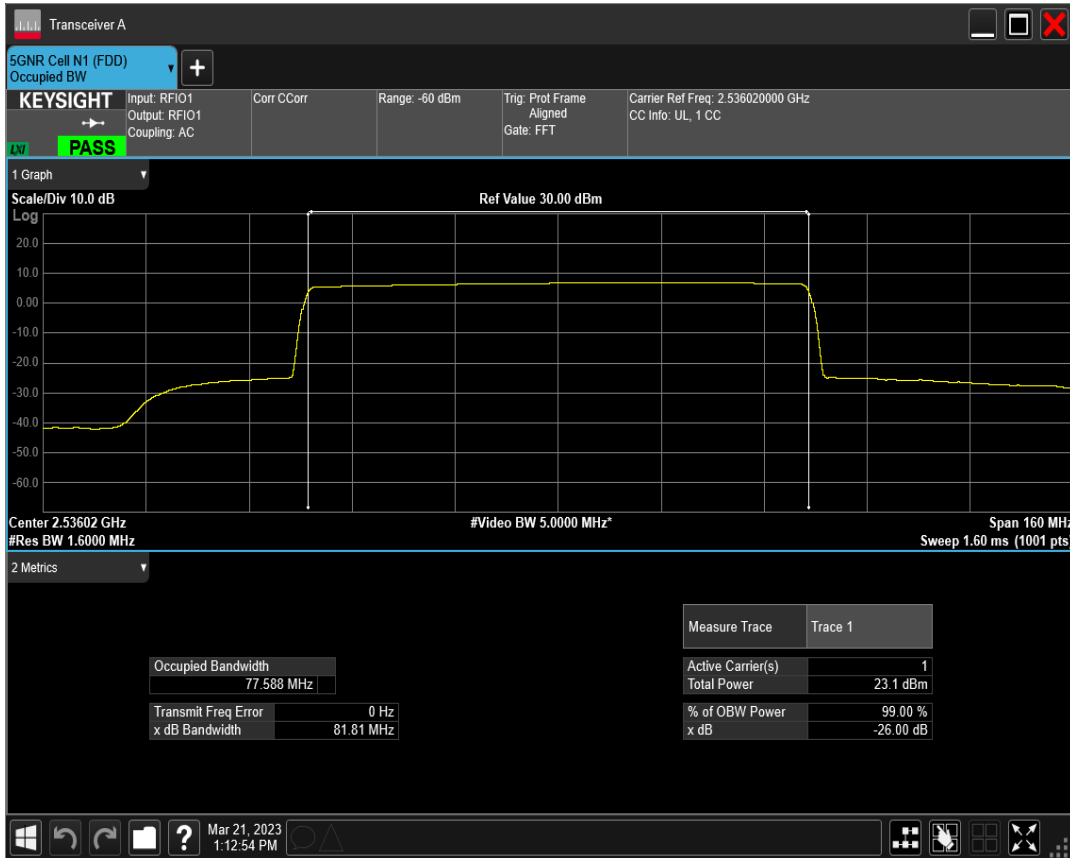
n41 SCS=30kHz DFT_BPSK BW=80MHz Channel=518598 RB=216@0
