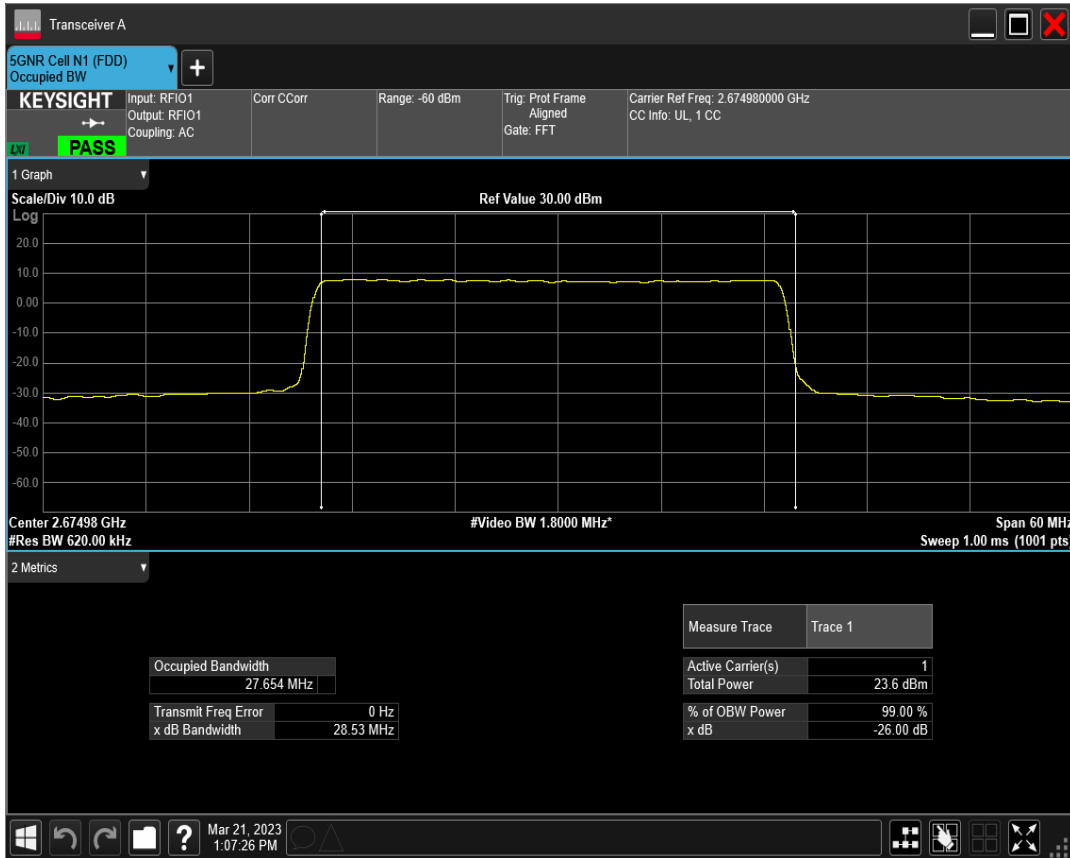
n41 SCS=30kHz DFT_QAM256 BW=30MHz Channel=534996 RB=75@0
