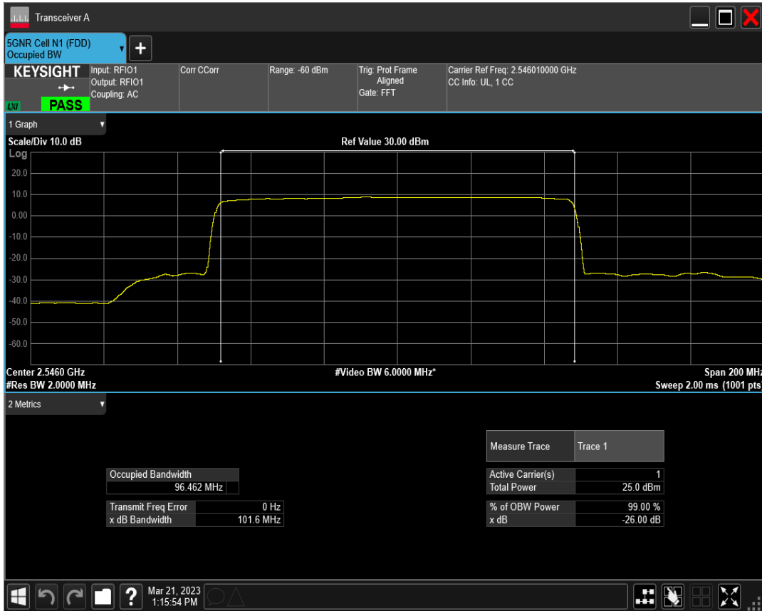
n41 SCS=30kHz DFT_QAM16 BW=100MHz Channel=509202 RB=270@0
