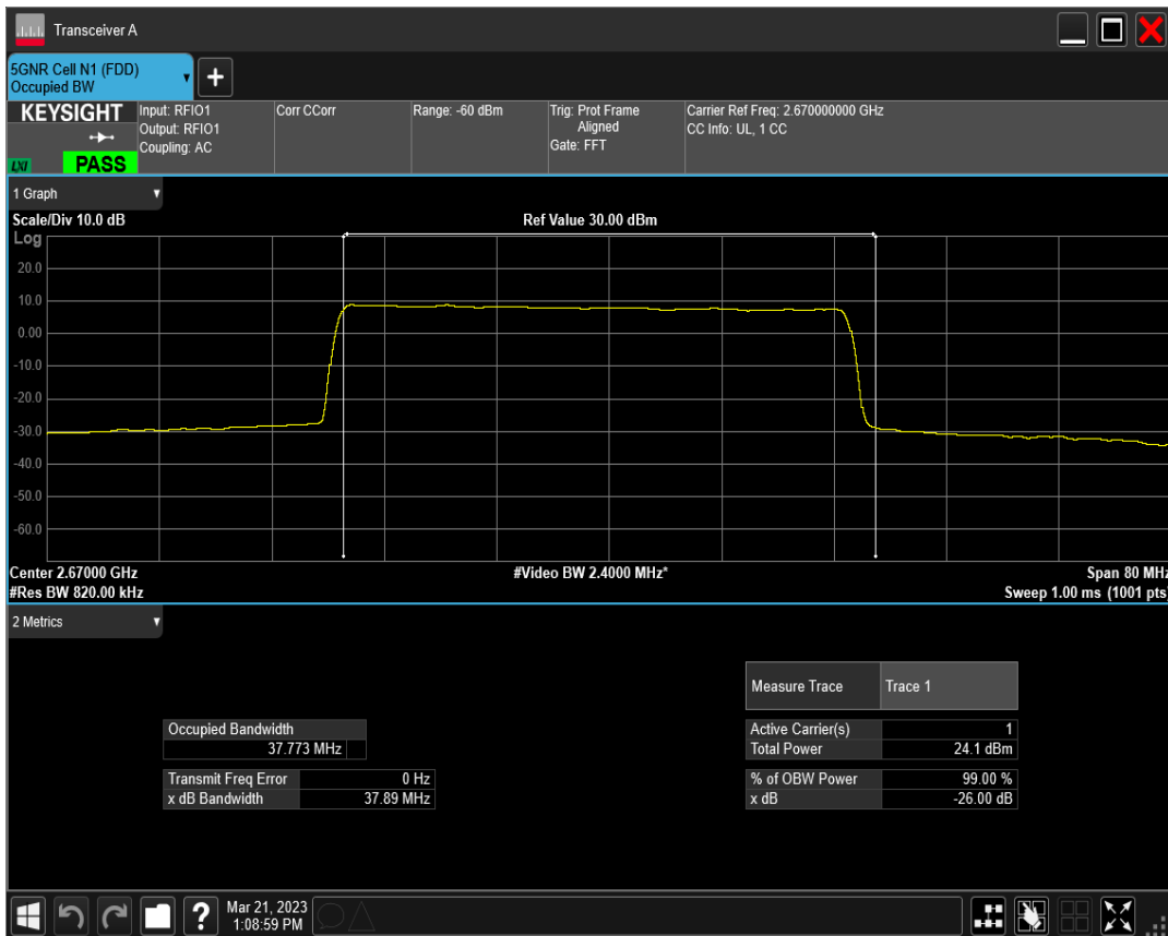
n41 SCS=30kHz DFT_QAM64 BW=40MHz Channel=534000 RB=100@0
