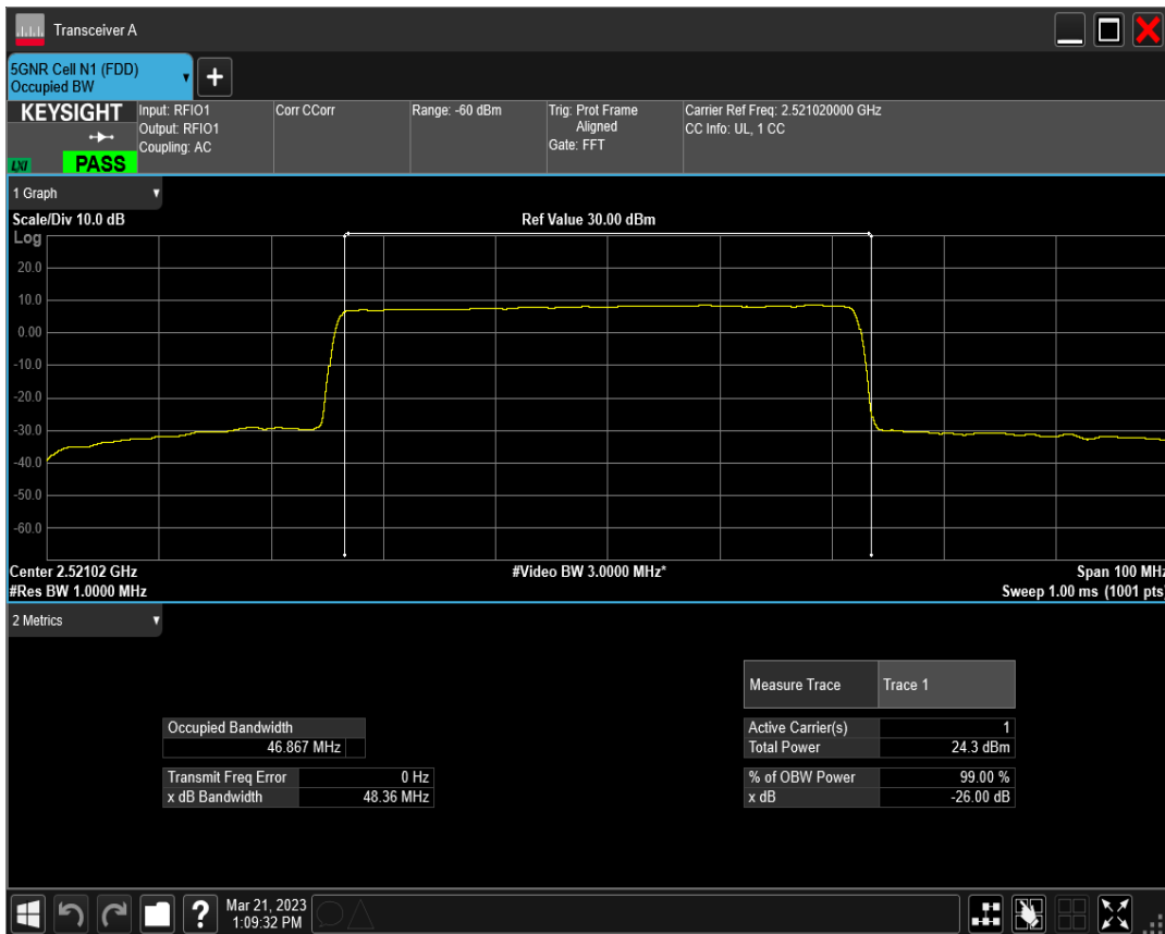
n41 SCS=30kHz DFT_QAM64 BW=50MHz Channel=504204 RB=128@0
