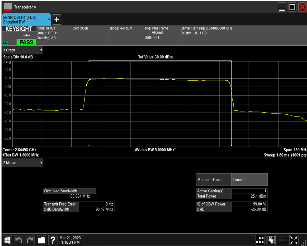
n41 SCS=30kHz DFT_QAM16 BW=90MHz Channel=528996 RB=240@0
