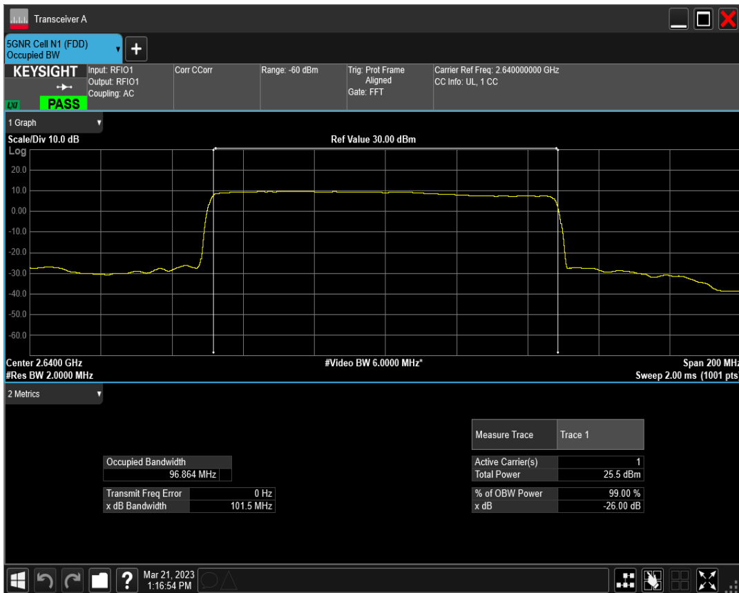
n41 SCS=30kHz DFT_QPSK BW=100MHz Channel=528000 RB=270@0
