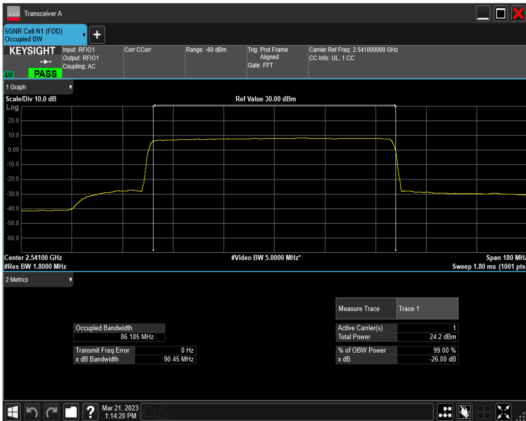
n41 SCS=30kHz DFT_QAM64 BW=90MHz Channel=508200 RB=240@0
