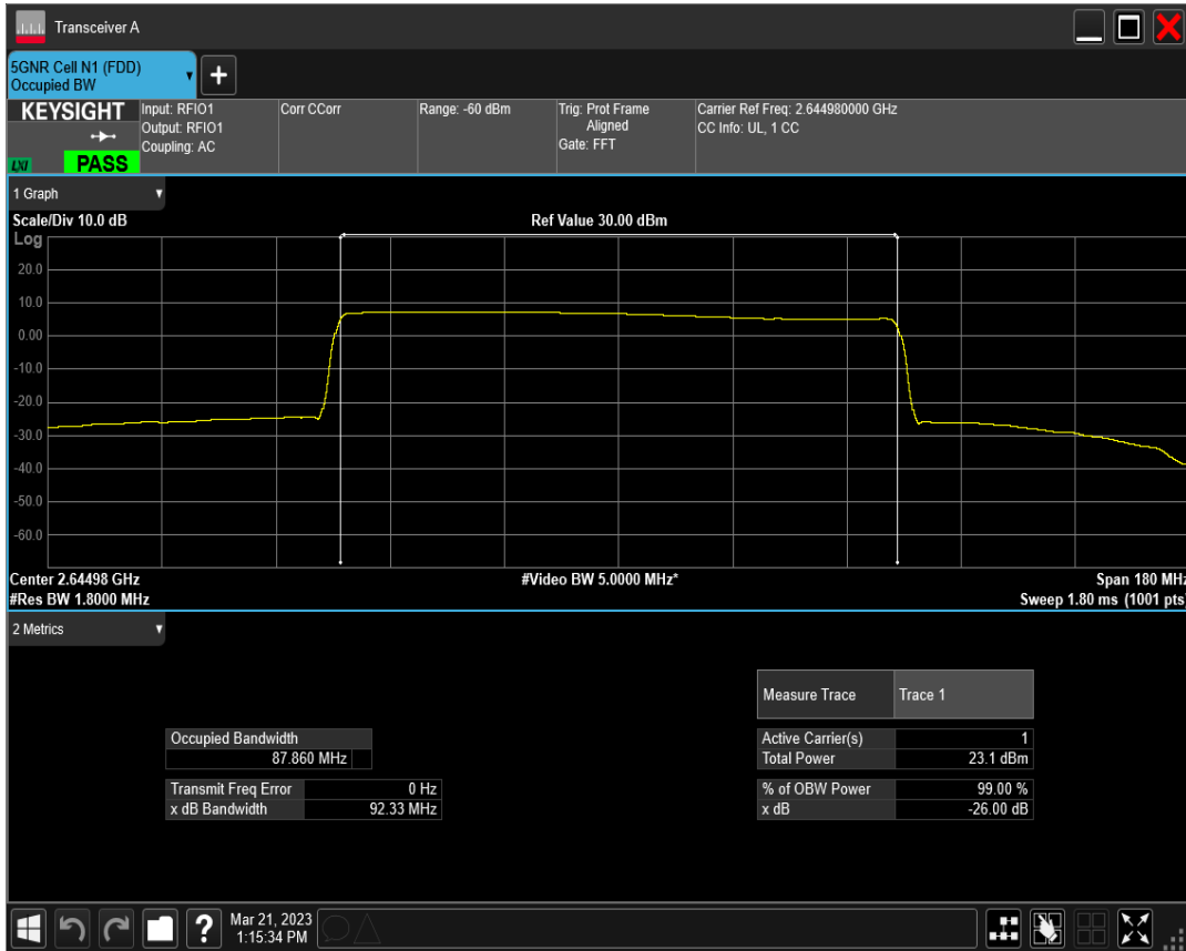
n41 SCS=30kHz DFT_BPSK BW=100MHz Channel=509202 RB=270@0
