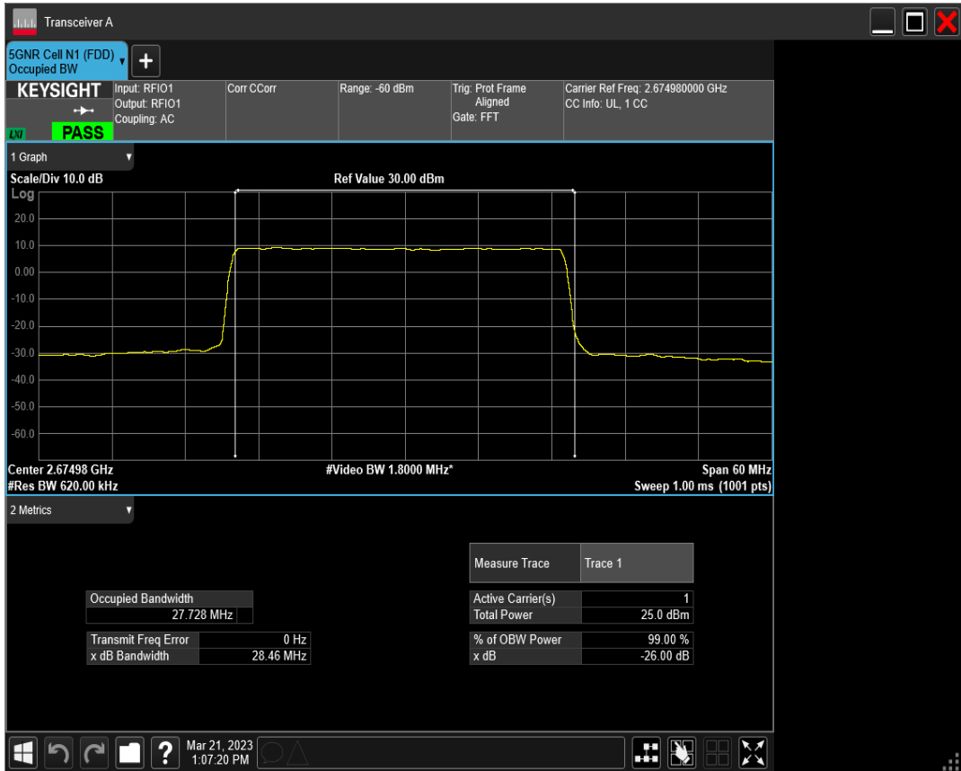
n41 SCS=30kHz DFT_QAM16 BW=30MHz Channel=534996 RB=75@0
