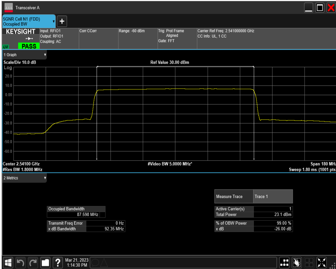
n41 SCS=30kHz DFT_BPSK BW=90MHz Channel=518598 RB=240@0
