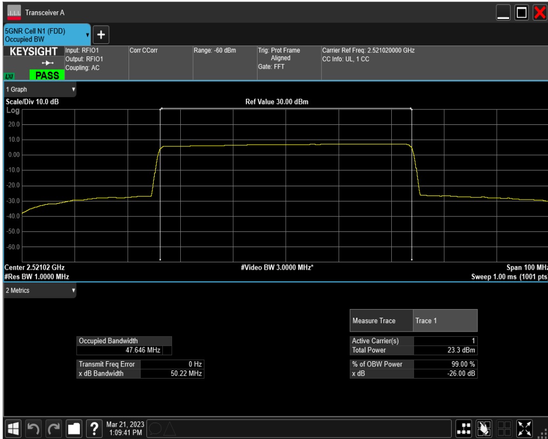
n41 SCS=30kHz DFT_BPSK BW=50MHz Channel=518598 RB=128@0
