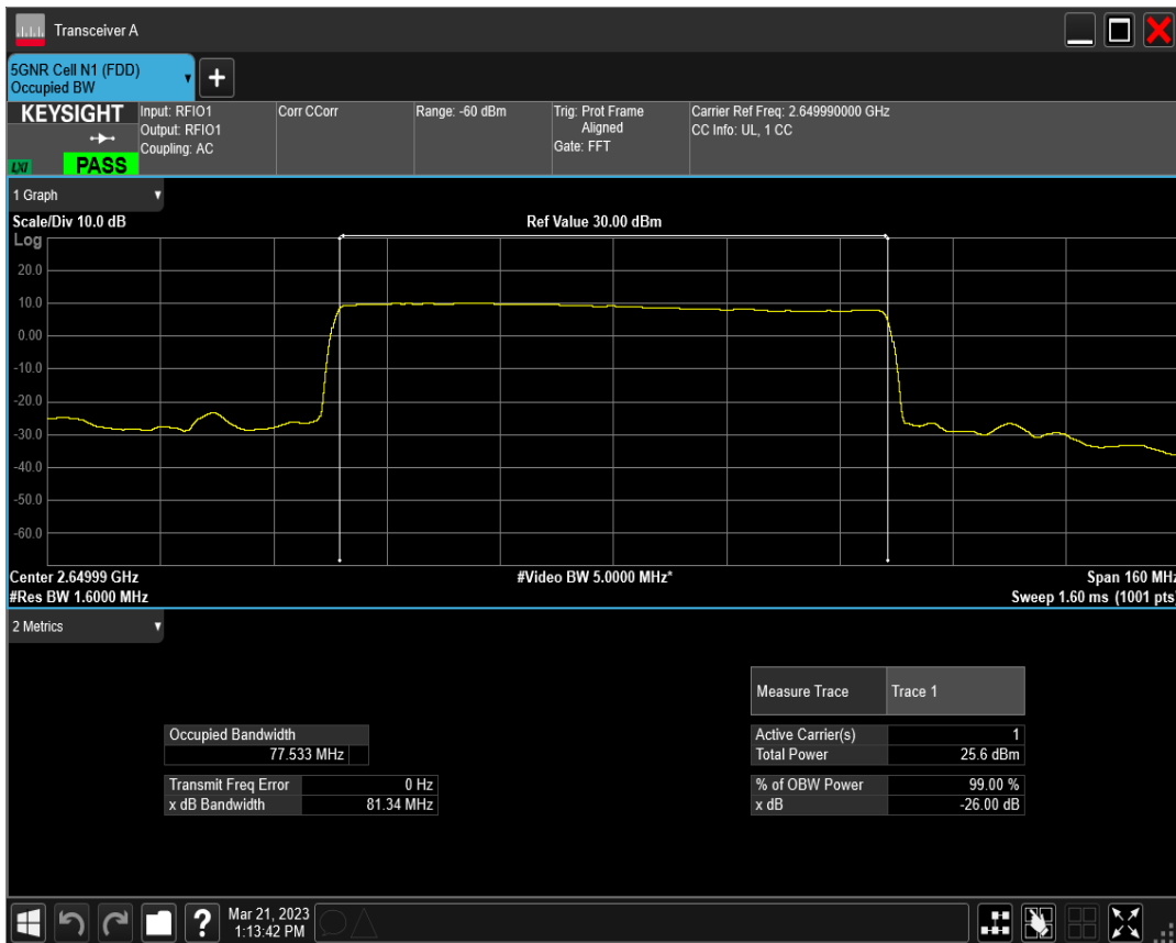
n41 SCS=30kHz DFT_QPSK BW=80MHz Channel=529998 RB=216@0
