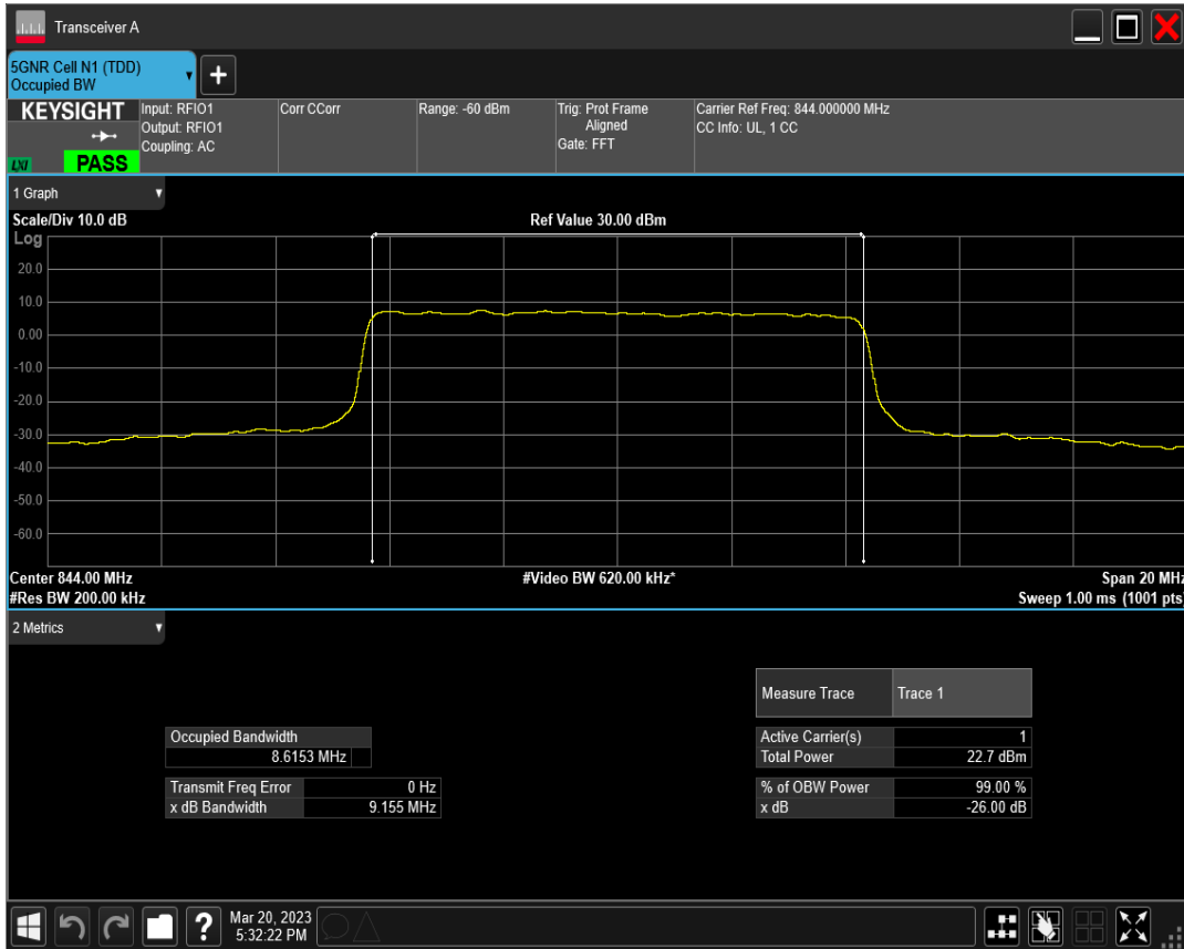
n5 SCS=30kHz DFT_QAM16 BW=10MHz Channel=168800 RB=24@0
