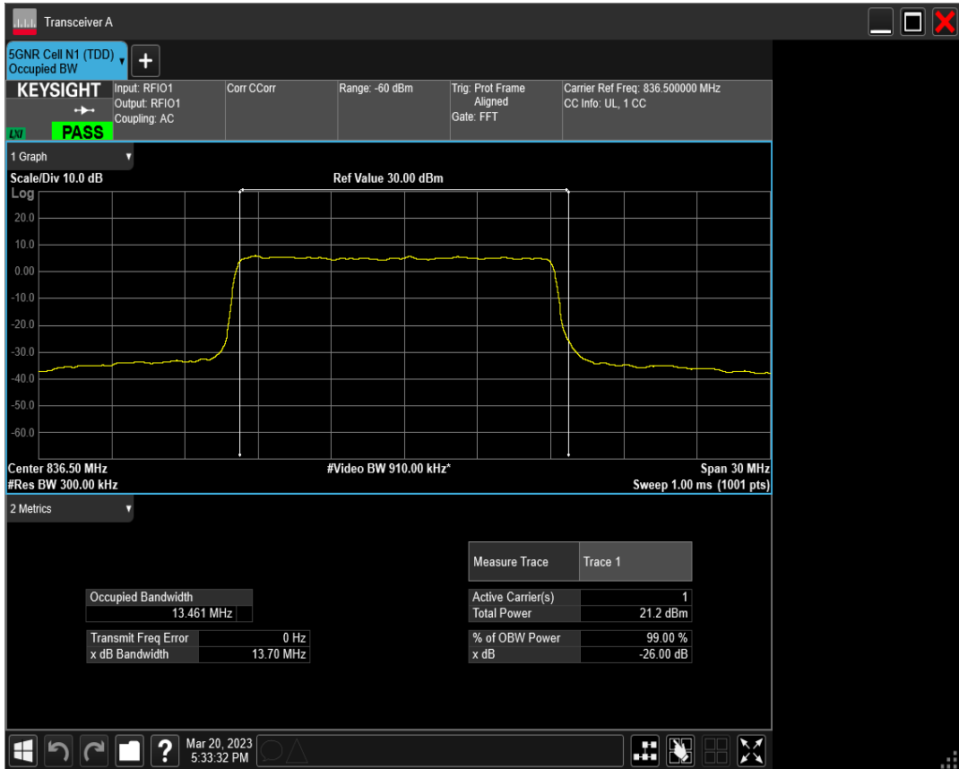
n5 SCS=30kHz DFT_QAM256 BW=15MHz Channel=167300 RB=36@0
