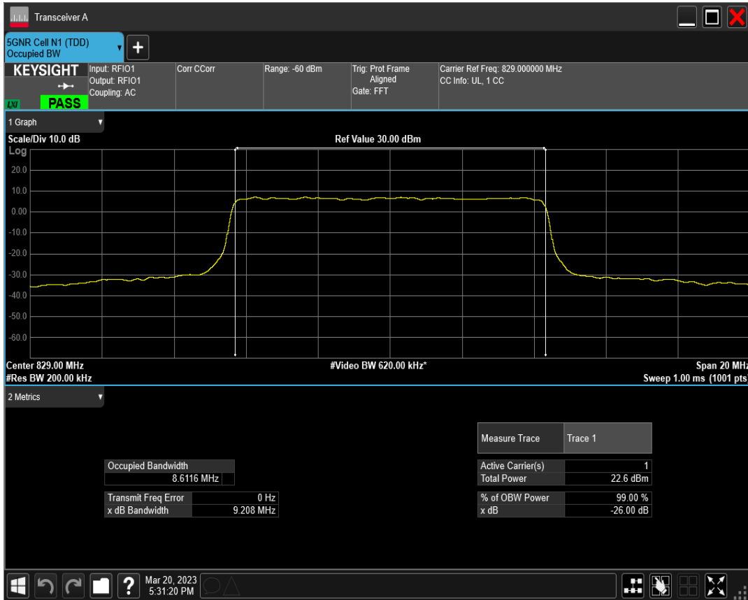
n5 SCS=30kHz DFT_QAM16 BW=10MHz Channel=165800 RB=24@0
