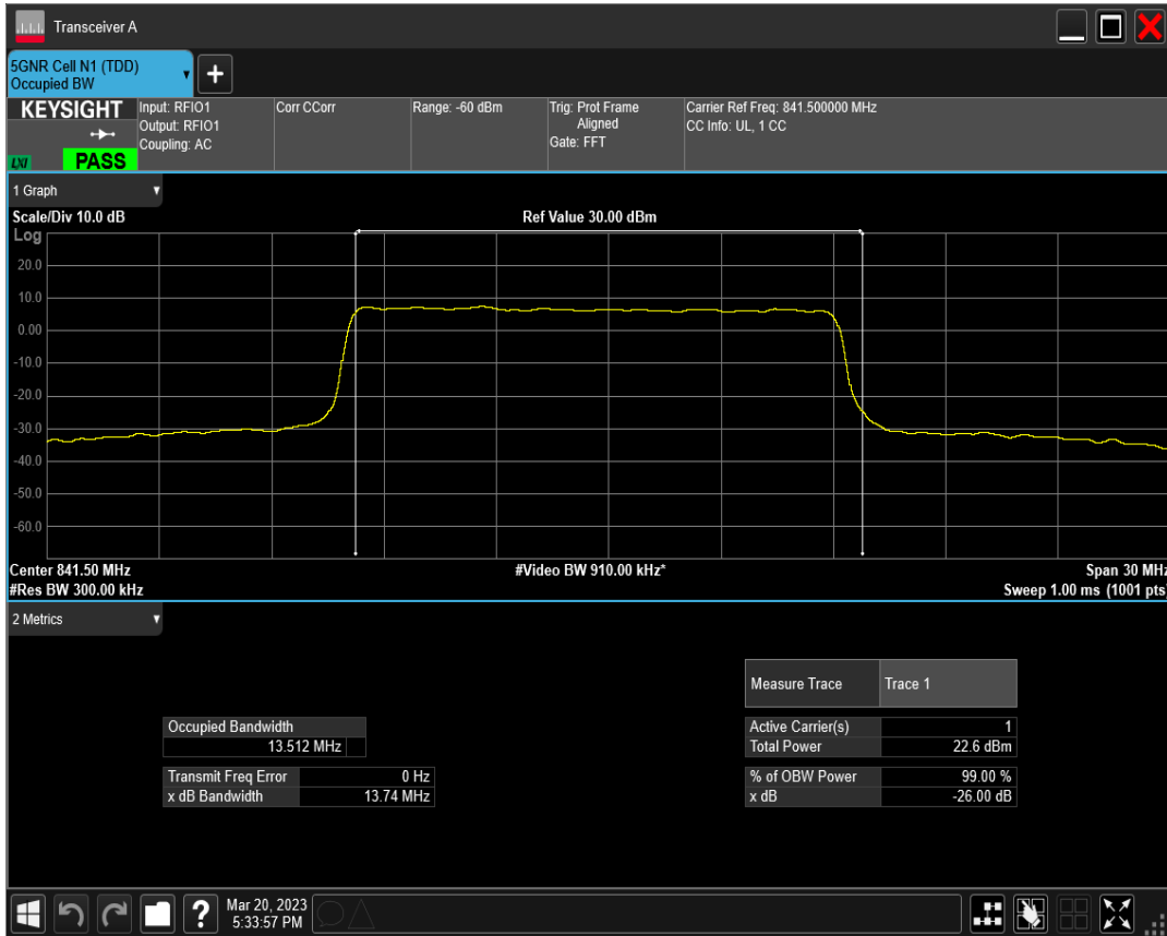
n5 SCS=30kHz DFT_QAM16 BW=15MHz Channel=168300 RB=36@0
