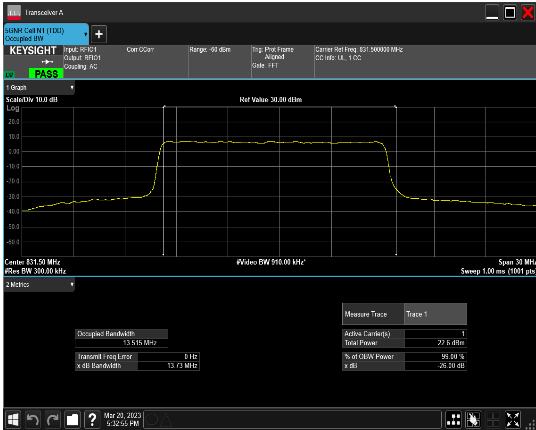
n5 SCS=30kHz DFT_QAM16 BW=15MHz Channel=166300 RB=36@0
