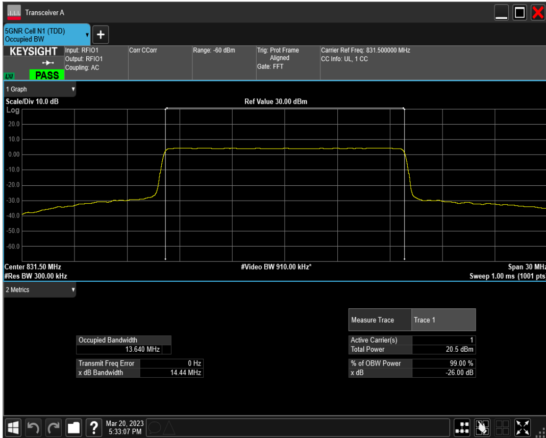
n5 SCS=30kHz DFT_BPSK BW=15MHz Channel=167300 RB=36@0
