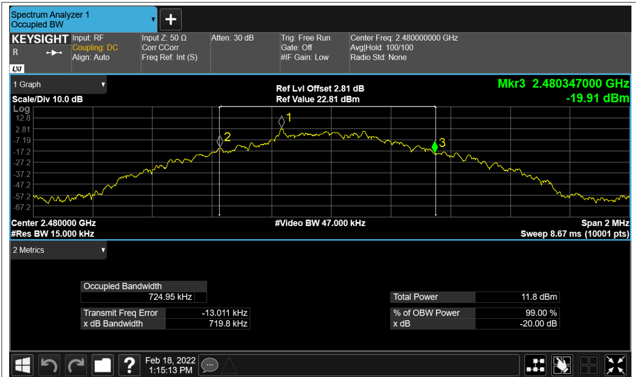
-20dB Bandwidth NVNT 2-DH1 2402MHz Ant1
