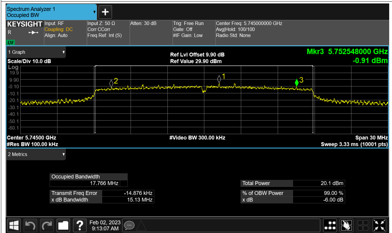
-6dB Bandwidth NVNT n20 5785MHz Ant1
