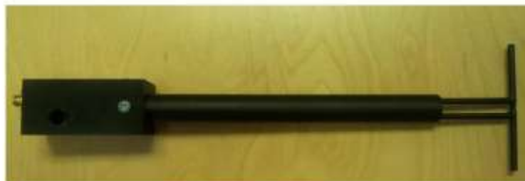
Figure 1 – MVG COMOSAR Validation Dipole
