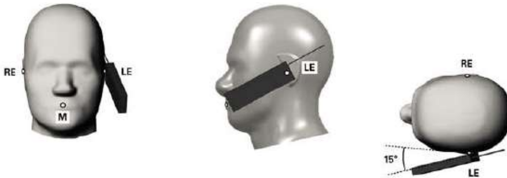
Fig.11.4 Illustration for Tilted Position
