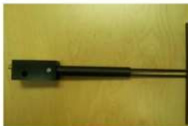
Figure 1 – MVG COMOSAR Validation Dipole
