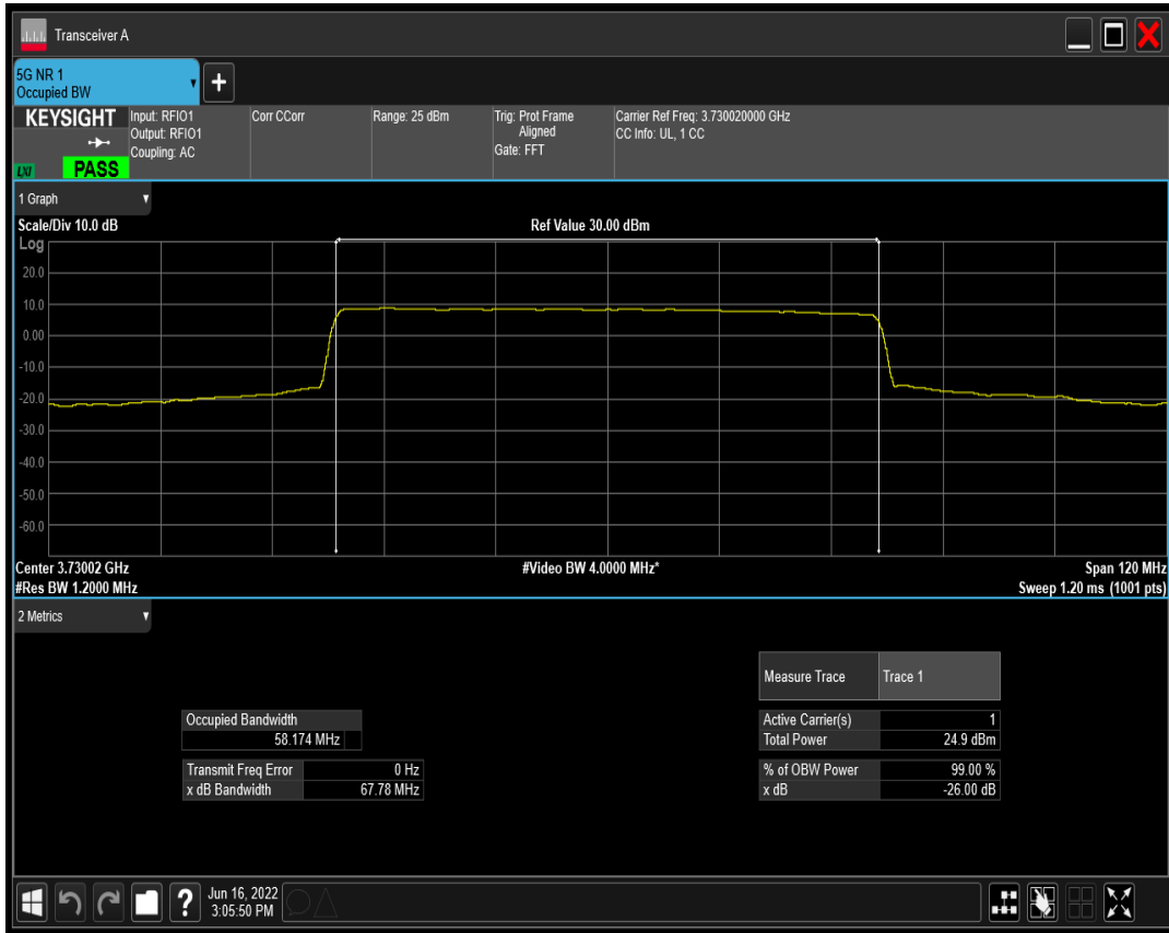
n77(3700-3980) SCS=30kHz DFT_QAM16 BW=60MHz Channel=648668 RB=162@0
