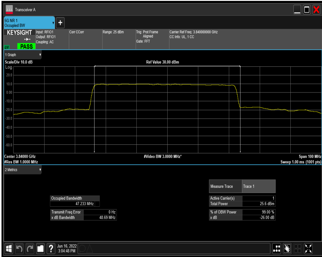
n77(3700-3980) SCS=30kHz DFT_QAM16 BW=50MHz Channel=656000 RB=128@0
