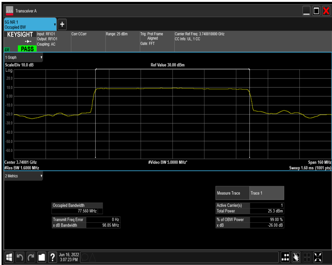
n77(3700-3980) SCS=30kHz DFT_QPSK BW=80MHz Channel=649334 RB=216@0
