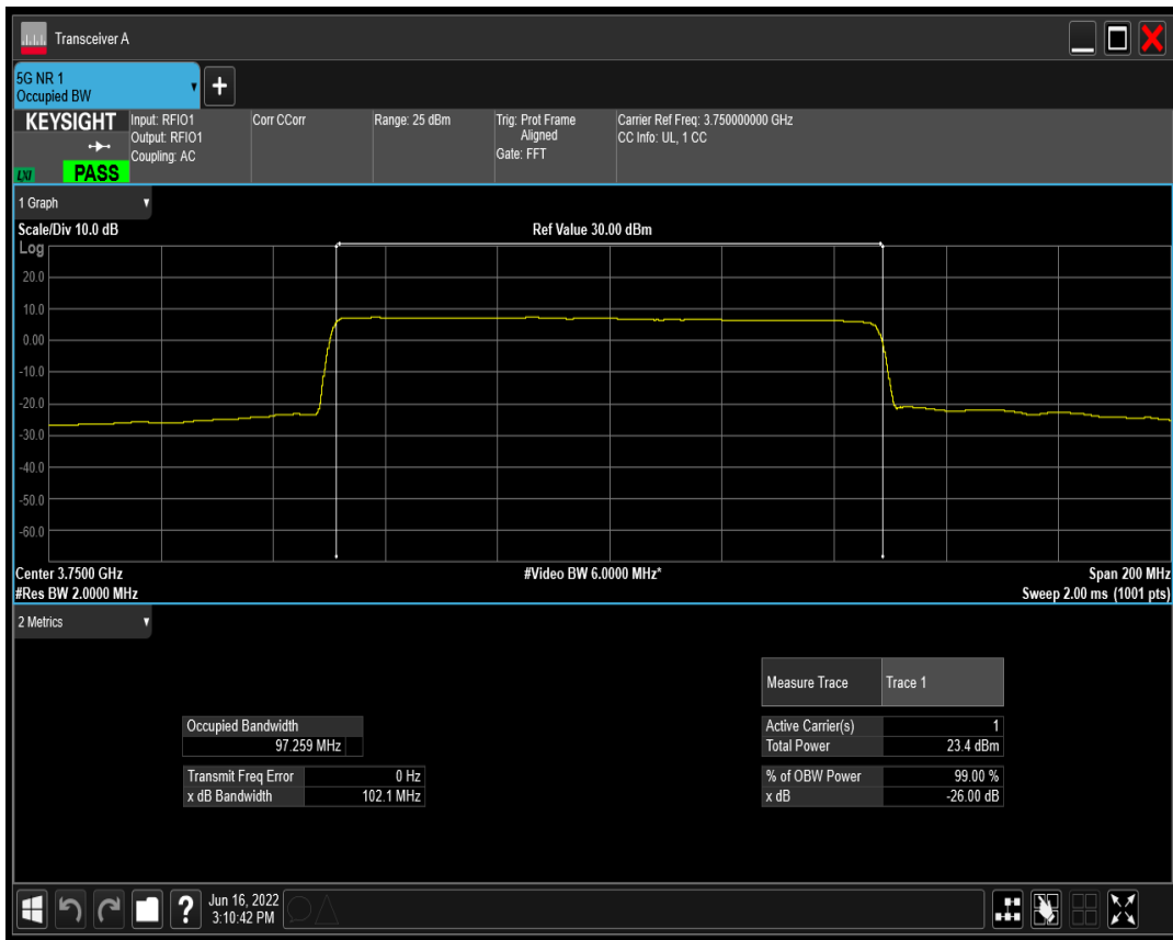
n77(3700-3980) SCS=30kHz DFT_QAM256 BW=100MHz Channel=650000 RB=270@0
