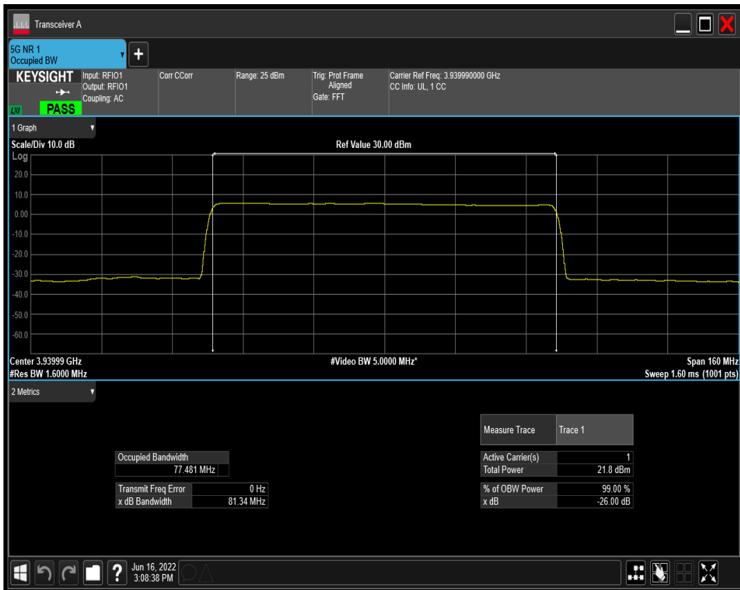
n77(3700-3980) SCS=30kHz CP_QPSK BW=80MHz Channel=662666 RB=217@0
