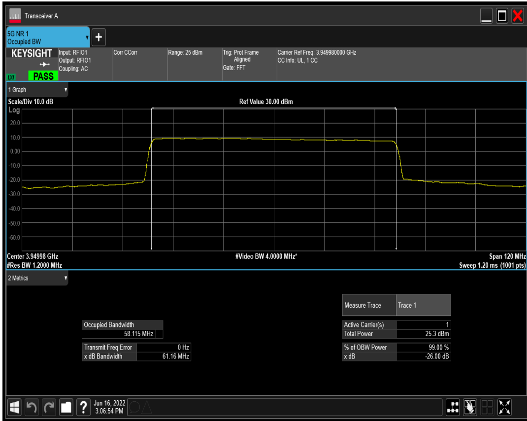
n77(3700-3980) SCS=30kHz DFT_QAM16 BW=60MHz Channel=663332 RB=162@0
