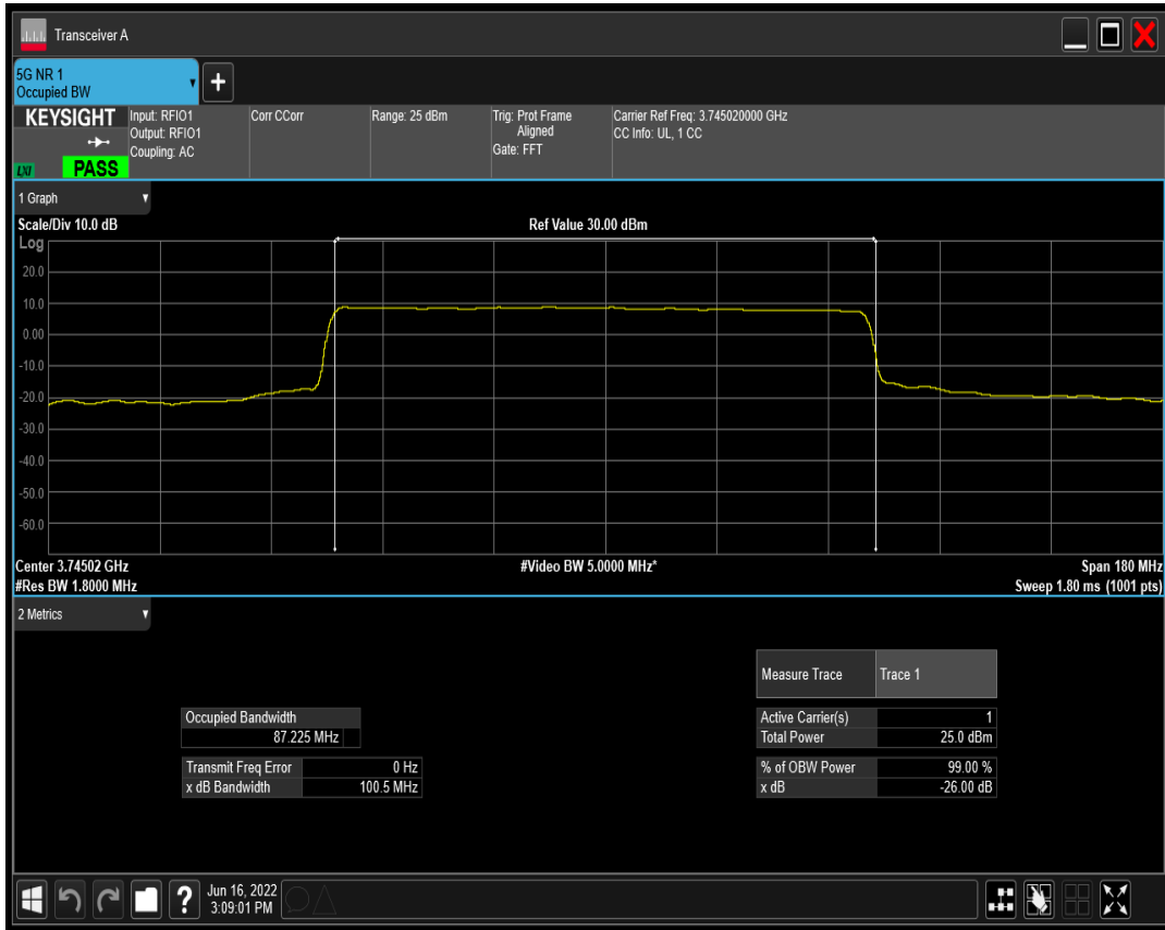
n77(3700-3980) SCS=30kHz DFT_QAM16 BW=90MHz Channel=649668 RB=240@0
