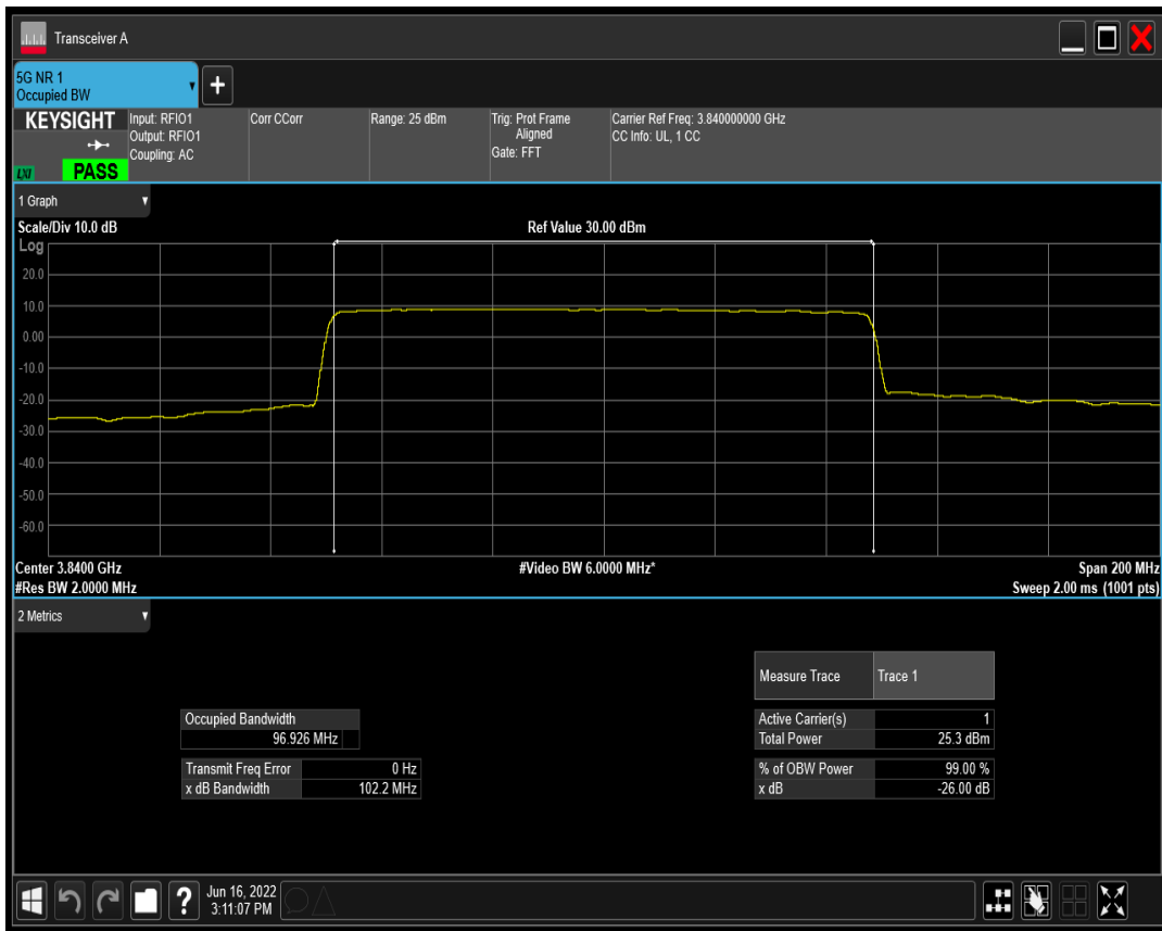
n77(3700-3980) SCS=30kHz DFT_QAM16 BW=100MHz Channel=656000 RB=270@0
