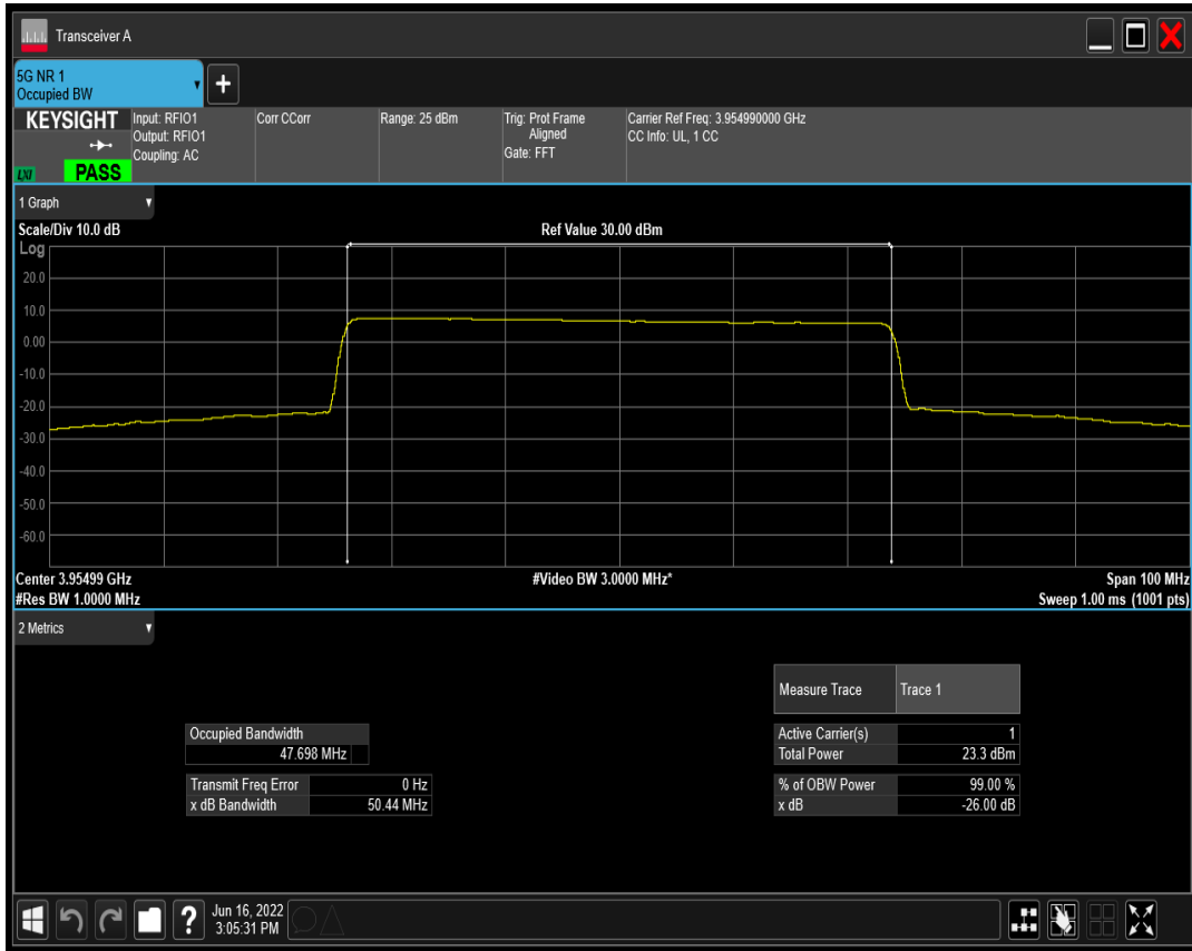
n77(3700-3980) SCS=30kHz DFT_BPSK BW=60MHz Channel=648668 RB=162@0
