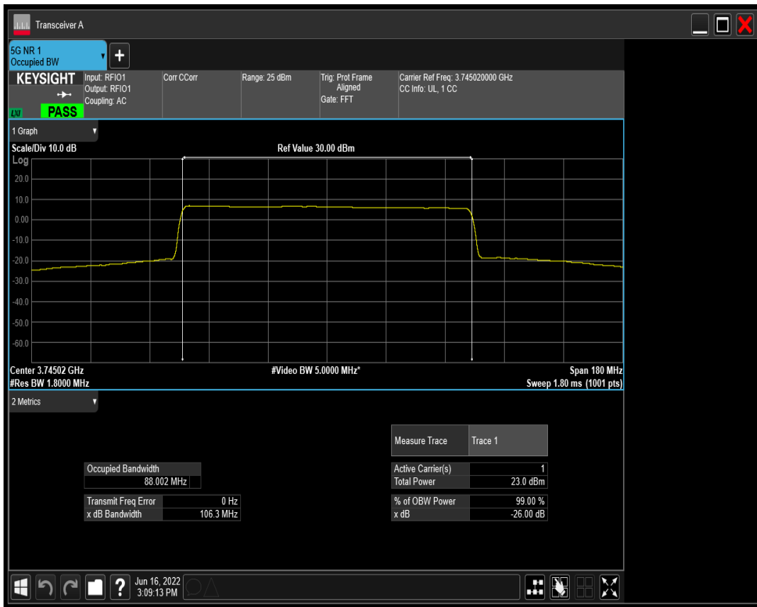
n77(3700-3980) SCS=30kHz DFT_BPSK BW=90MHz Channel=656000 RB=240@0
