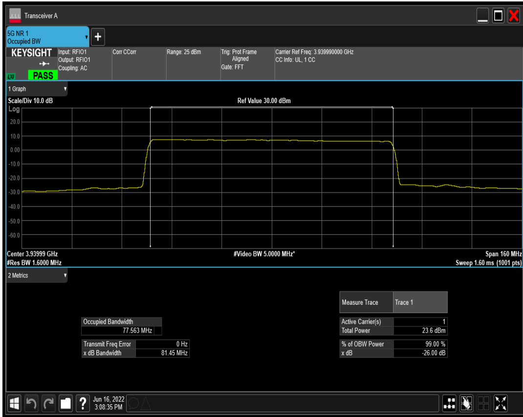
n77(3700-3980) SCS=30kHz DFT_QAM256 BW=80MHz Channel=662666 RB=216@0
