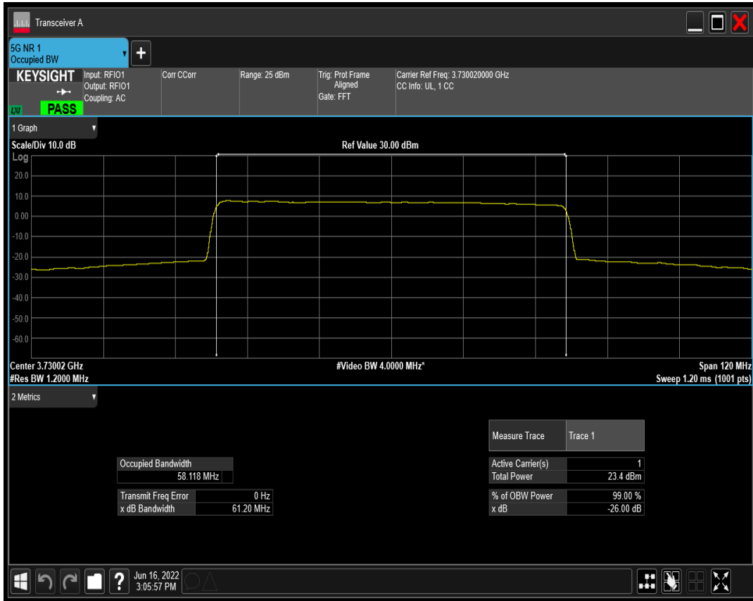
n77(3700-3980) SCS=30kHz DFT_QAM256 BW=60MHz Channel=648668 RB=162@0
