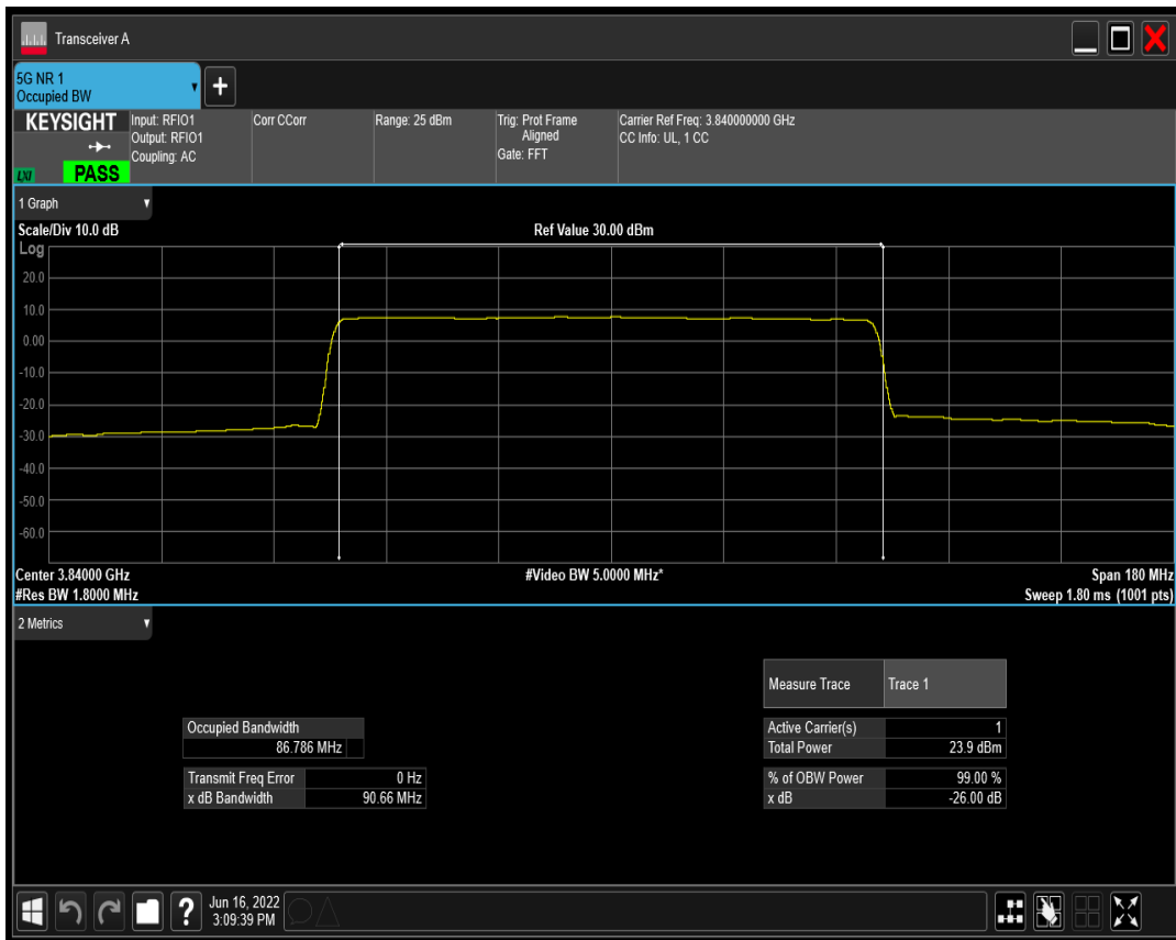
n77(3700-3980) SCS=30kHz DFT_QAM256 BW=90MHz Channel=656000 RB=240@0
