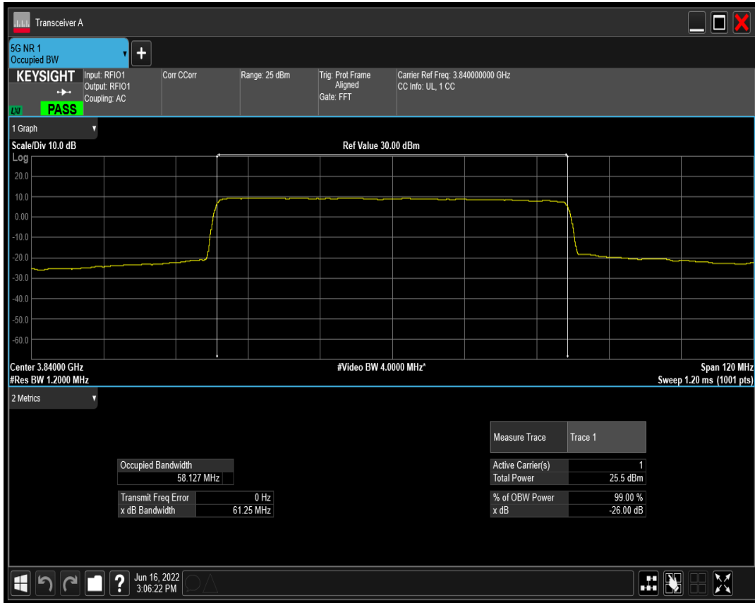
n77(3700-3980) SCS=30kHz DFT_QAM16 BW=60MHz Channel=656000 RB=162@0
