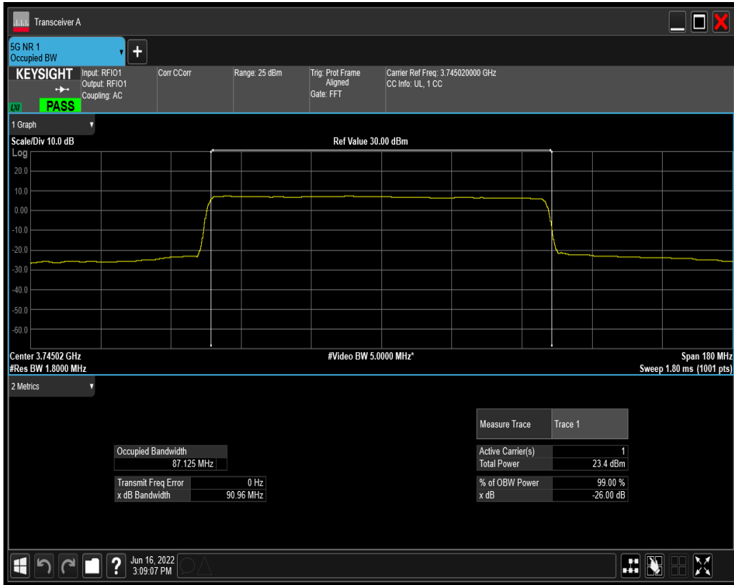
n77(3700-3980) SCS=30kHz DFT_QAM256 BW=90MHz Channel=649668 RB=240@0
