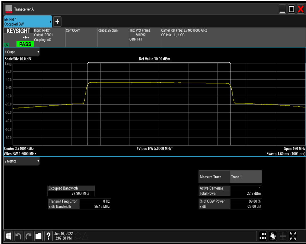
n77(3700-3980) SCS=30kHz DFT_BPSK BW=80MHz Channel=656000 RB=216@0
