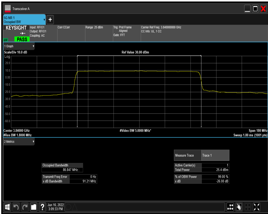
n77(3700-3980) SCS=30kHz DFT_QAM16 BW=90MHz Channel=656000 RB=240@0
