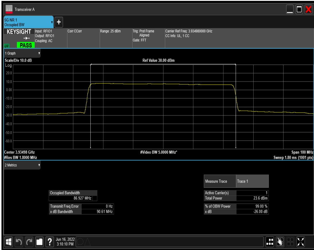
n77(3700-3980) SCS=30kHz DFT_QAM256 BW=90MHz Channel=662332 RB=240@0
