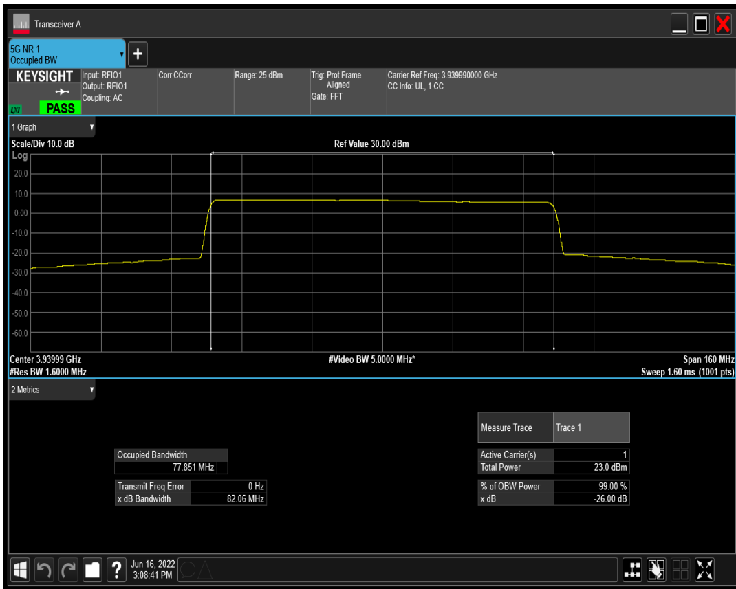
n77(3700-3980) SCS=30kHz DFT_BPSK BW=90MHz Channel=649668 RB=240@0
