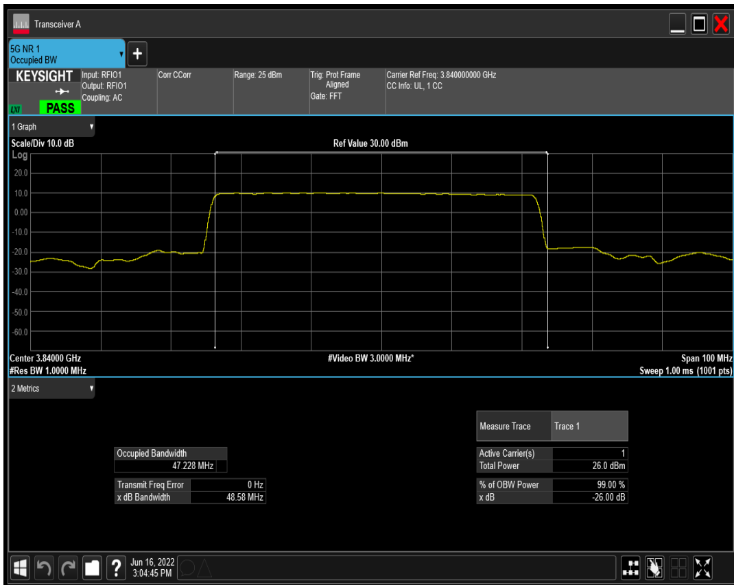
n77(3700-3980) SCS=30kHz DFT_QPSK BW=50MHz Channel=656000 RB=128@0
