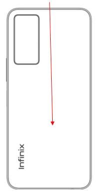
The label shown shall be permanently affixed at a conspicuous location on the device and be readily visible to the user at the time purchase (Labeling requirements per 2.925)
