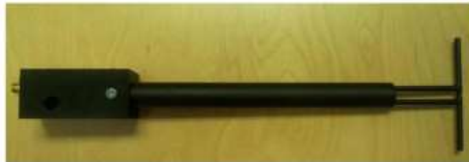
Figure 1 –MVG COMOSAR Validation Dipole
