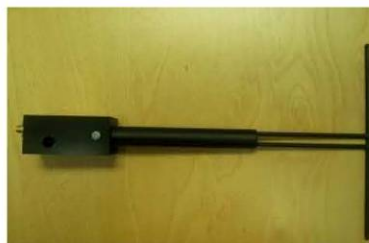
Figure 1 – MVG COMOSAR Validation Dipole
