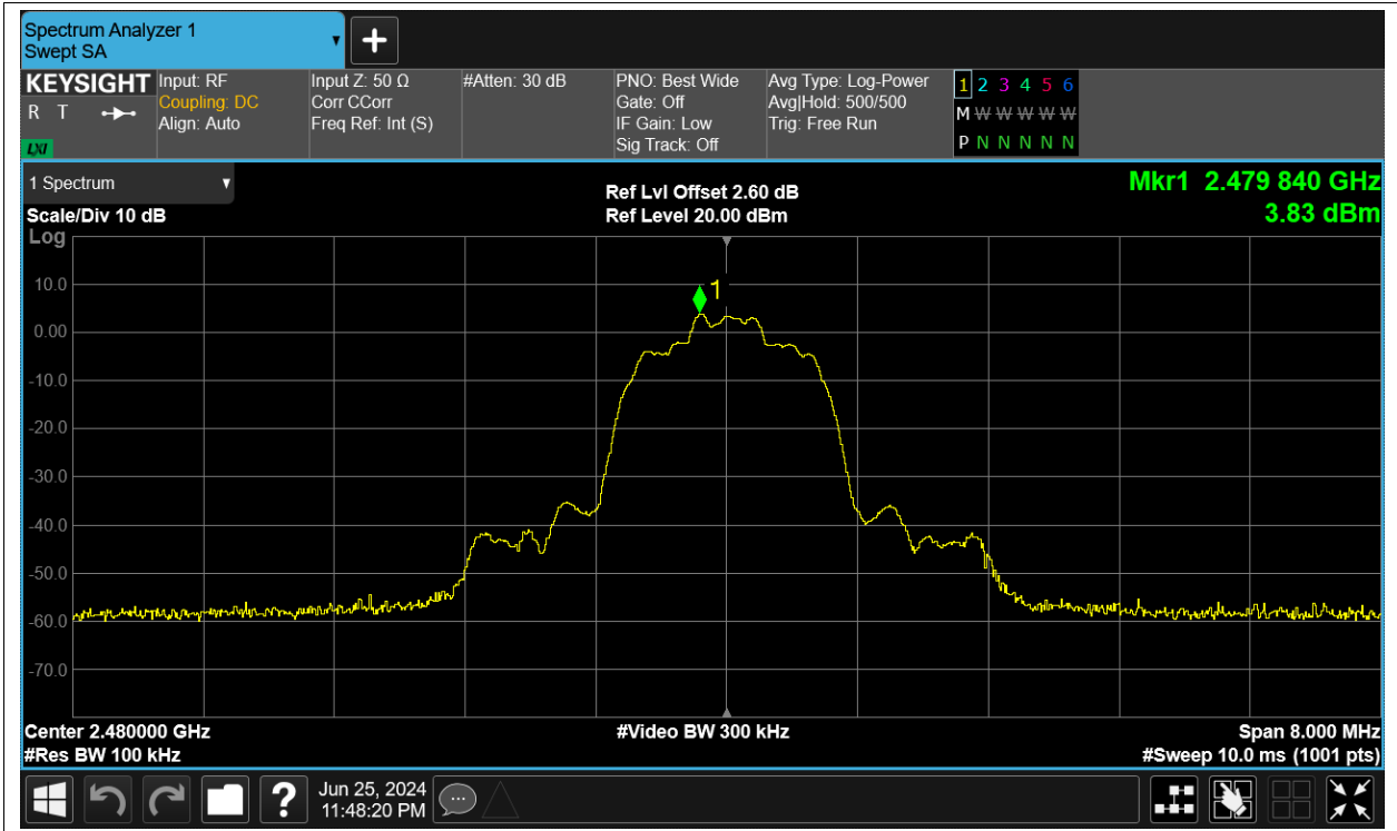
Band Edge NVNT 3-DH1 2480MHz Ant2 No-Hopping Emission
