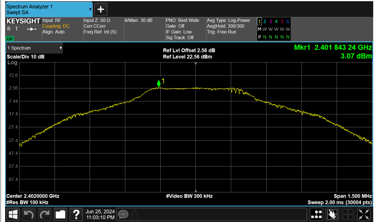
Tx. Spurious NVNT 1-DH1 2402MHz Ant2 Emission
