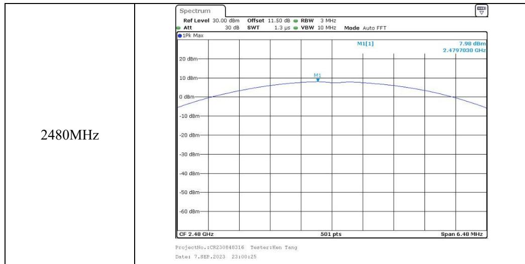
**4.8 100 kHz Bandwidth of Frequency Band Edge**
