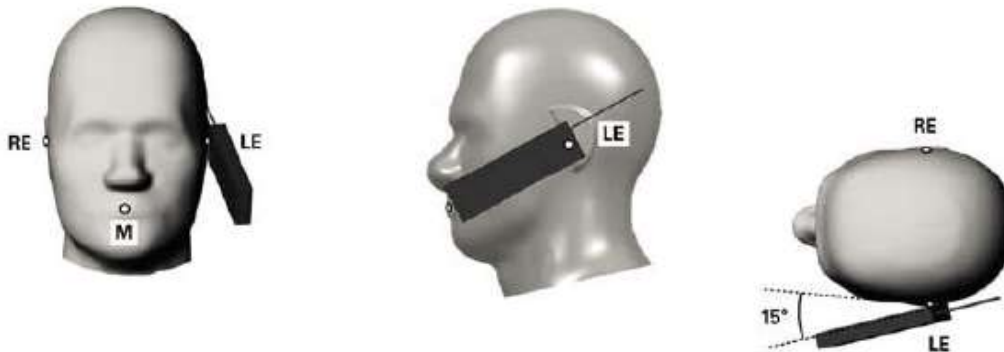
Fig.11.4 Illustration for Tilted Position
