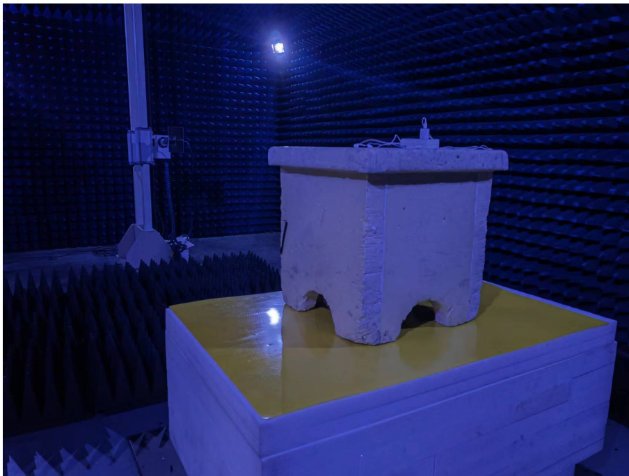
Photo of Radiated Emission Measurement (Above 1G)
