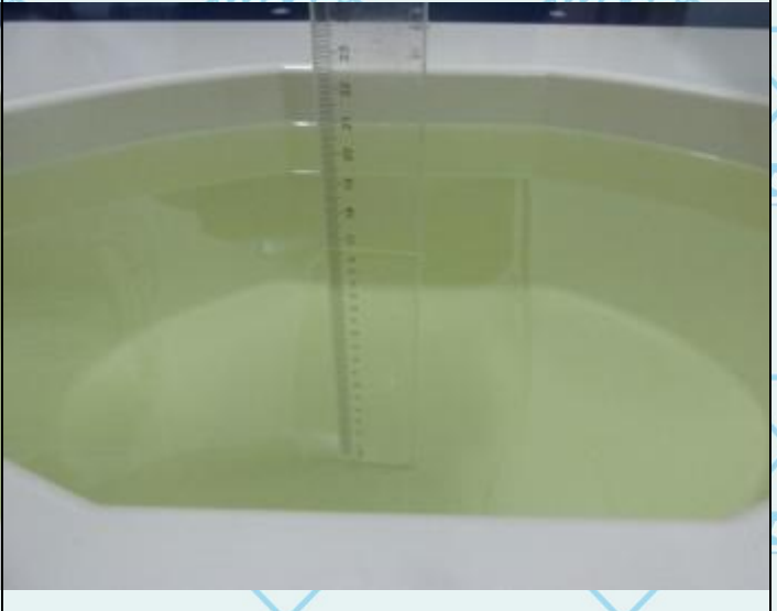
Photo 16: 2450MHz Liquid Depth ≥ 15.0cm
