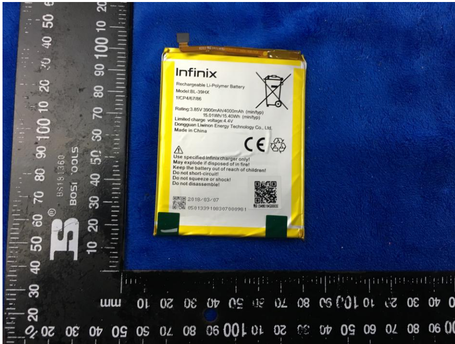
Battery - Front View
