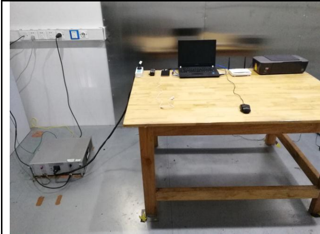
Conducted Emissions Test Setup – Front View
